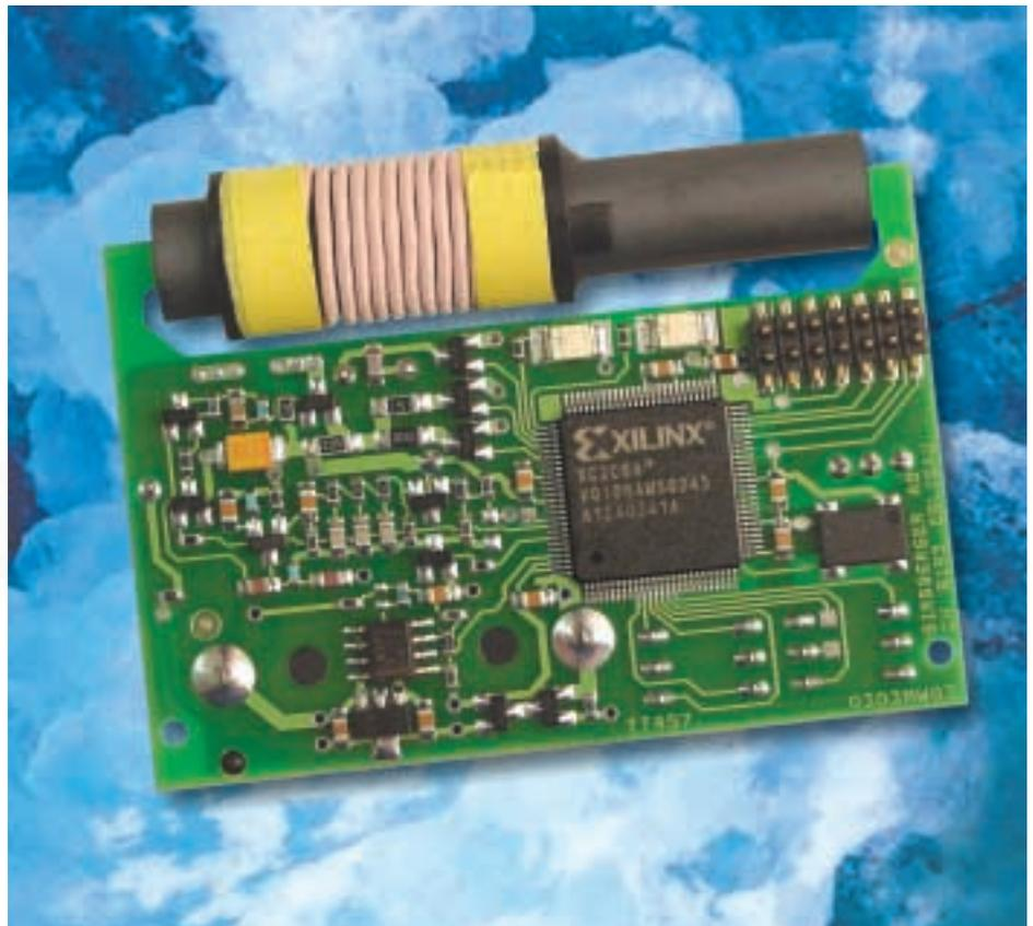
Figure 2 – Internal view of training transmitter
