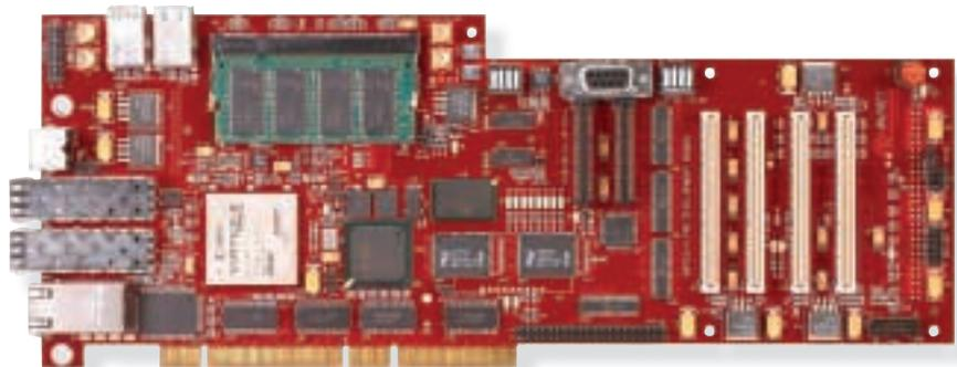
Figure 1 – Avnet-designed Virtex-II Pro XC2VP20 development board
