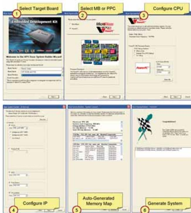
Figure 2 – The Base System Builder wizard enables easy definition of hardware platforms in FPGA-based embedded systems.
