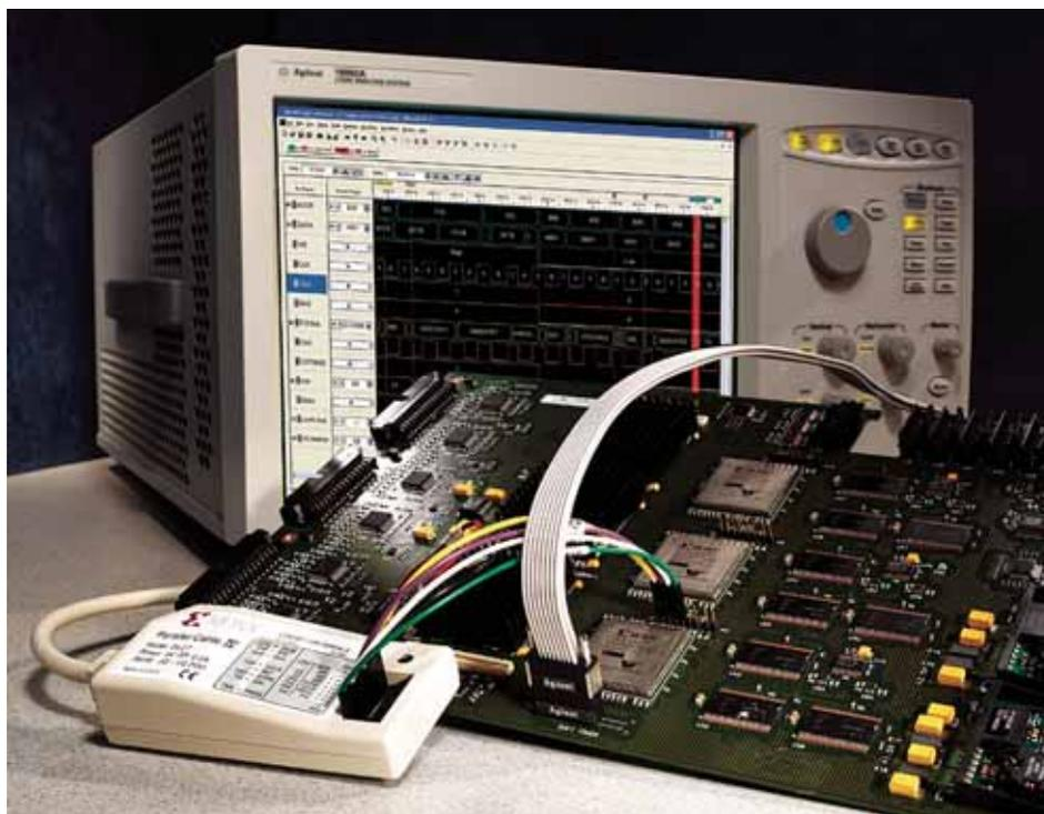
Figure 1 – The FPGA dynamic probe application software can change virtual probe points inside Xilinx FPGAs in less than a second. The logic analysis application communicates to a debug core via JTAG.
