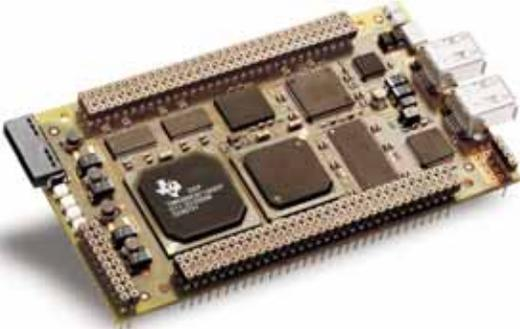
The micro-line C6713Compact is a high performance single board DSP/FPGA solution, offering exceptional capabilities and flexibility.
