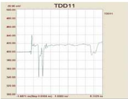
Figure 3 – SDD11 in the time domain for a backplane channel, measured with an Agilent PNA N4421b four-port VNA and PLTS software.
