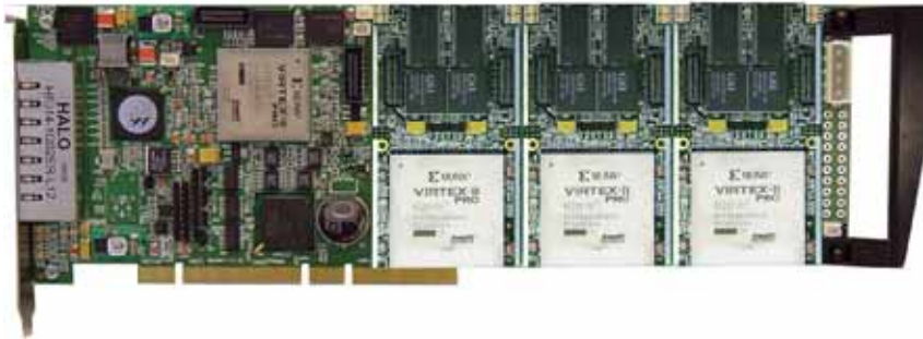
Figure 4 – The BenNUEY-PCI-4E motherboard configured with three BenDATA-II modules
