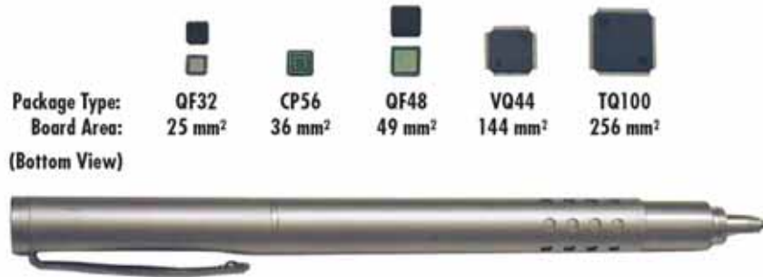
Figure 1 – MLF package comparison
