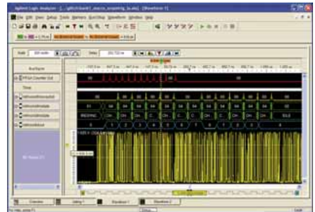
Figure 4 – Zoom-out reveals relationship of glitch to receive state machine stalling after 12 packets
