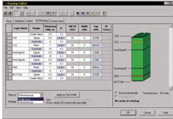
Figure 1 – Careful pre-layout impedance planning using the HyperLynx Stackup Planning tool helps eliminate signal reflections.
