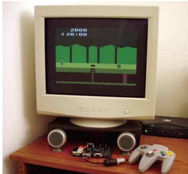
Figure 3 – Hardware emulation of the Atari 2600 VCS running Pitfall by Activision (courtesy of Ed Henciak)
