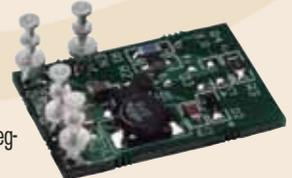
The LM2734 and LM2736 are monolithic, high-frequency (550 kHz and 1.6 MHz) PWM step-down DC/DC converters in tiny six-pin thin SOT-23 packaging. They provide local DC/DC conversion for Xilinx FPGAs with currents up to 1A.
