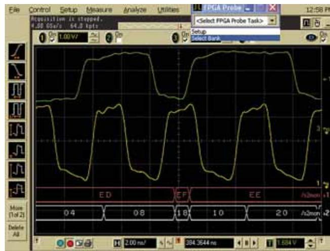
*Figure 1 – In addition to scope channels, mixed-signal oscilloscopes provide 16 digital channels. This gives you the ability to trigger and display as many as 20 signals simultaneously. The width of the digital channels is particularly well suited for measuring signals internal to Xilinx FPGAs.*
