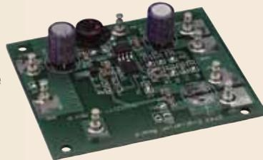
The LM2743 and LM2744 are high-speed synchronous buck regulator controllers that drive external MOSFETs to supply as much as 25A of current. They can provide simple down conversion to output voltages as low as 0.6V. Although the control sections of the ICs are rated for 3 to 6V, the driver sections are designed to accept input supply rails as high as 16V. The use of adaptive non-overlapping MOSFET gate drivers helps avoid potential shoot-through problems while maintaining high efficiency.
