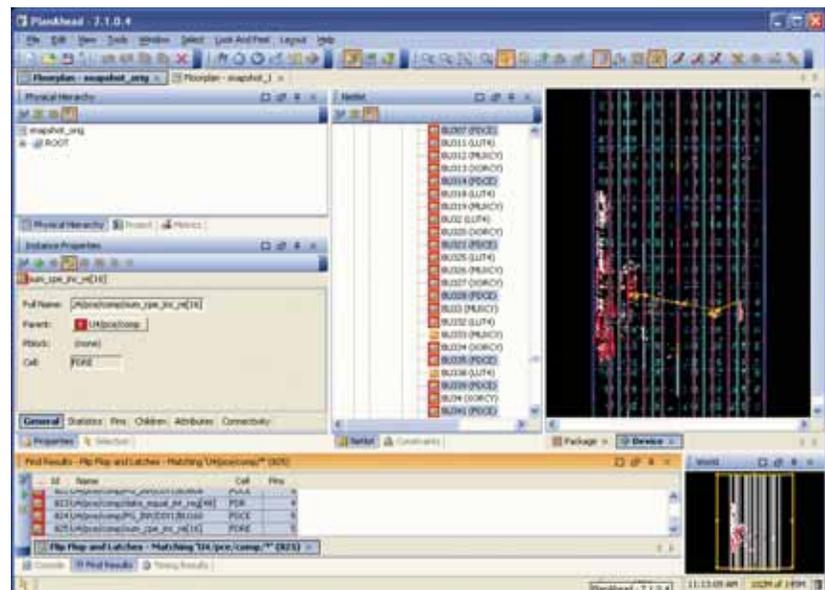
Figure 3 – Initial Virtex-4 FPGA floorplan with the path highlighted that did not initially meet timing
