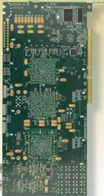
Partitioning your design onto the 3.7 million ASIC gates (LSI measure) of our new board is a lot easier. With three of the biggest, fastest, new Xilinx Virtex-4 FPGAs this PCI hosted logic prototyping system takes full advantage of the integrated ISERDES/OSERDES. 400MHz LVDS differential communication with 10X multiplexing means more than 1800 signals between FPGA A & B. Synplicity Certify™ models are provided for partitioning assistance.
