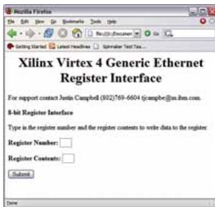
Figure 4 – Example HTML page connection through communication to the Xilinx embedded MAC IP address
