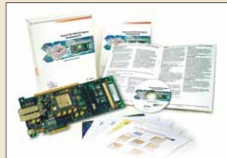
The Virtex-5 LXT FPGA Development kit for PCI Express supports PCIe/PCI-X/PCI. This complete development kit passed PCI-SIG compliance for PCI Express specification v1.1 and enables you to rapidly create and evaluate designs using PCI Express, PCI-X, and PCI interfaces.
