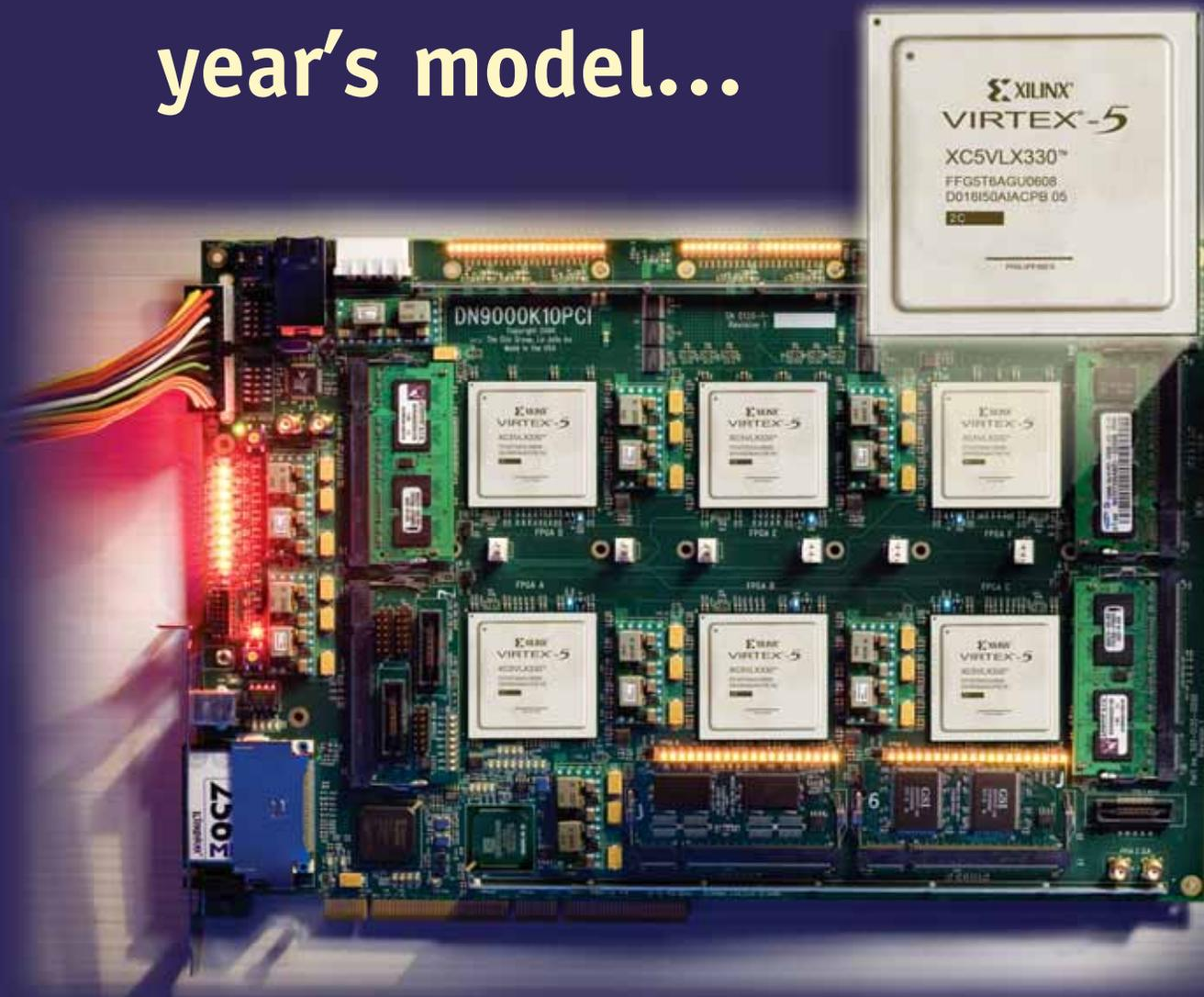
Here are 6 of the new, faster, bigger, Virtex-5 FPGAs on a 12 Million ASIC Gate Board that offers unmatched performance to ASIC Prototypers, IP Designers, and FPGA Developers. The V5 65nm process, with 6 input LUT and advanced interconnect, enables 30% faster clock speeds in your application. The Dini DN9000k10PCI captures this performance on an easy to use board with these handy features:
