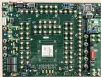
Xilinx ML52x platforms are ideal for characterization and evaluation of Virtex-5 LXT RocketIO GTP transceivers. Each RocketIO GTP transceiver is accessible through four SMA connectors. ML52x platforms are available with XC5VLX50T-FF665 (ML521), XC5VLX110T-FF1136 (ML523), and XC5VLX330T-FF1738 FPGA devices.
