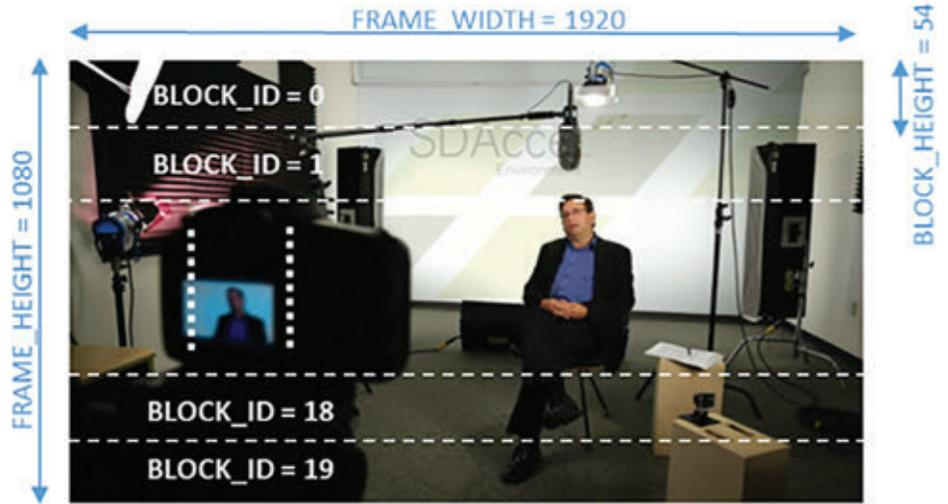
Figure 7 – Video frame partitioning into blocks
