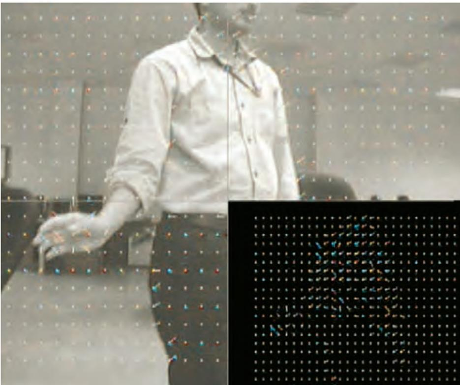
Figure 4 – An actual FPGA-processed frame with motion vector grid overlaid at bottom right
