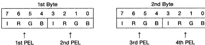
This mode is enabled when GRM1 = '0', GRM0 = '1', and Bit 4 of the Mode Register is '0'. The display colors are identical to those of the 160 x 4 Bit Mode (simultaneous display of 16 colors), and the size of display PELs is identical to that of the 320 x 2 Bit Mode.
