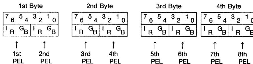
This mode is enabled when GRM1 = '1', GRM0 = '0', and Bit 4 of the Mode Register is '1'. The display colors are identical to those of the 160 x 4 Bit Mode (simultaneous display of 16 colors), and the size of display PELs is identical to that of the 640 x 1 Bit Mode.
