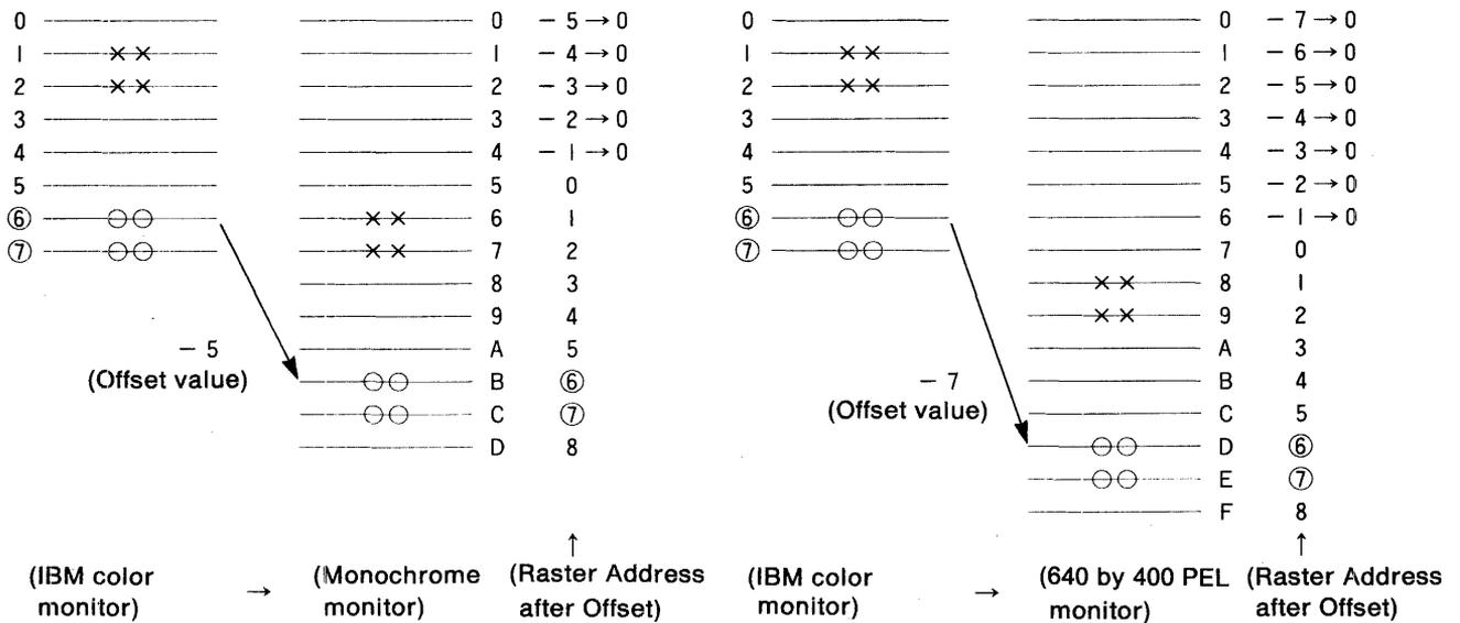
Since the Offset value is expressed in two's complements, the range of its setting is from  $-16$  to  $+15$ . In case an underflow occurs due to the offset, it shall be corrected to "0". If the Offset is unnecessary, write all '0' (the default status upon RESET).
