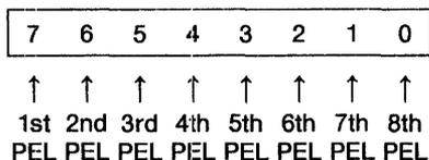
This mode is enabled when GRM1 = GRM0 = '0' and Bit 4 of the Mode Register is '1'. The display PELs have a 1 : 1 correspondence with each bit of the bytes read from VRAM. When data exists (RD = '1'), the color (out of 16 possible colors) selected by Bits 3-0 of the Color Register is displayed. When no data exists (RD = '0'), black (IRGB = "0000") is displayed. The border is similar displayed in black (IRGB = "0000").
