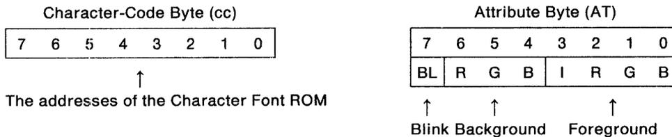
The Font ROM data is input to PCDC by the  $\overline{EC}$  pin via the RD bus. (The leading Display Data is connected for sequential input from RD7 to RD0. If the data consists of nine or more bits, the ninth bit and any consecutive bits are connected in the sequence of R15 to RD8.)
