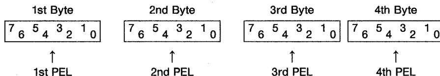
This mode is enabled when GRM1 = '1', GRM0 = '0', and Bit 4 of the Mode Register is '0'. Since the color of each display PEL is specified in byte units, up to 256 colors can be simultaneously displayed. The size of the display PELs is identical to that of the 320 x 2 Bit Mode. The border will be displayed in the color selected by Bits 3-0 of the Color Register (but when BINH = '1', the border will be displayed in black (IRGB = "0000")).
