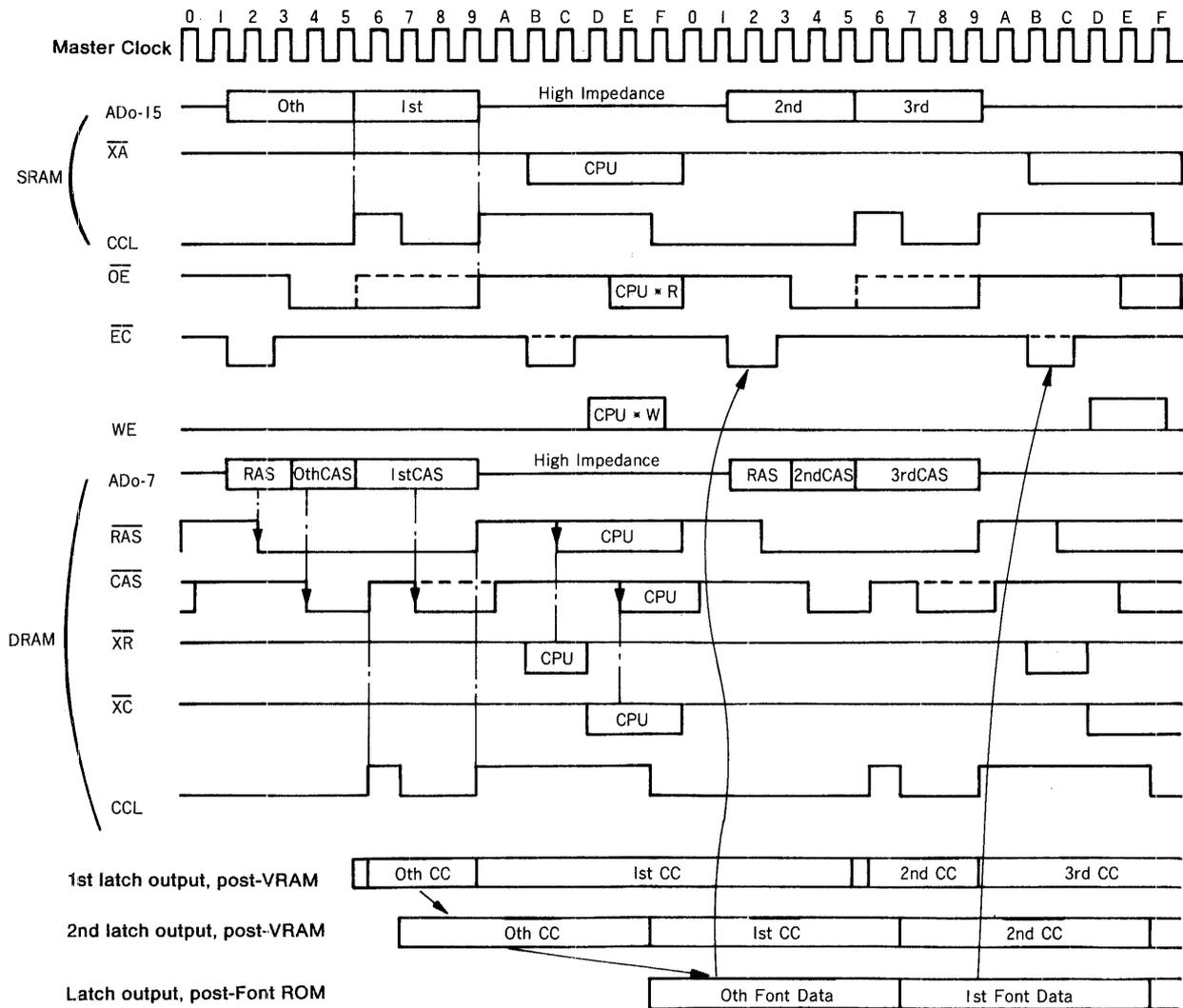
The above figure shows the timing of the various signals in High Resolution Text Mode (in case the horizontal font size is 8 PELs). The Character Codes are latched by an external circuit at the rising edge of CCL, then are latched again at the falling edge of CCL in order to provide leeway in the access time of the Font ROM. After the data from the Font ROM is latched at the falling edge of CCL, it is input to PCDC by  $\overline{EC}$  via the RD bus.
