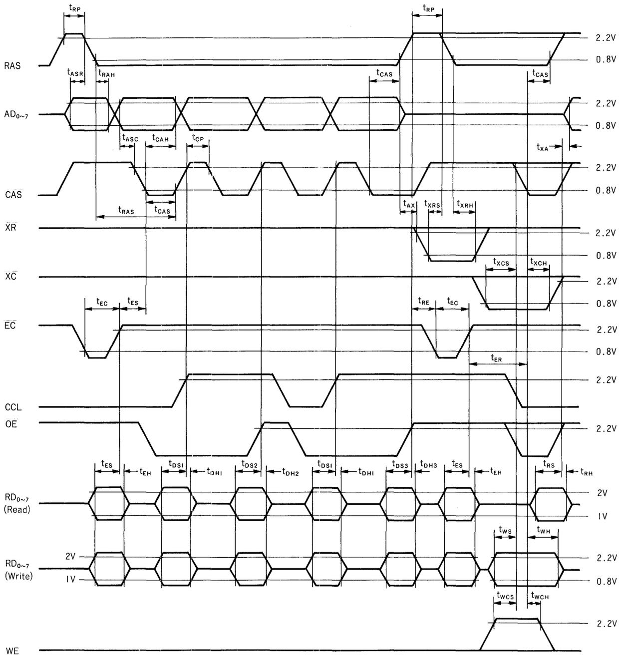
**8-4-3-3. 16-Bit Bus in SRAM Mode (@Cl = 100pF + 2LSTTL)**
