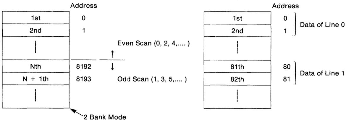
When ACM = '0' (Data is stored in a different bank according to the even/odd status of the Line No.)      When ACM = '1' (Data is sequentially stored from the top line to the bottom line)
