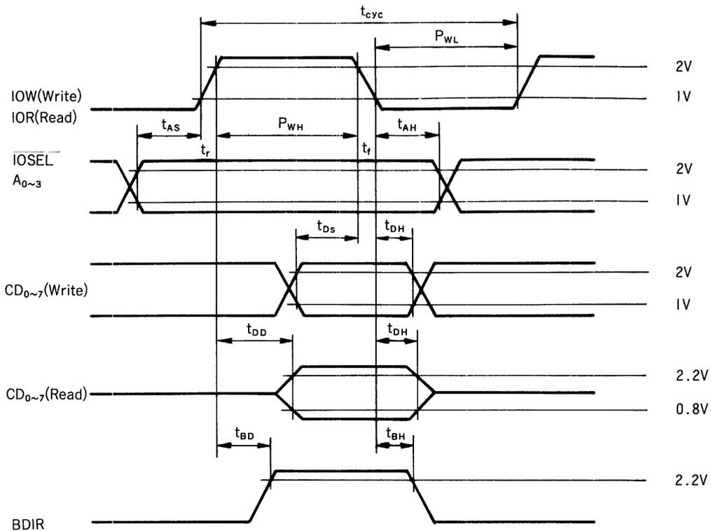
**8-4-2. VRAM-CPU Interface (@CL = 100pF + 2LSTTL (CD0-CD7, BDIR, MEMRDY))**
