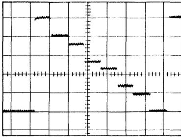
(A Waveform after Digital-to-Analog Conversion)
