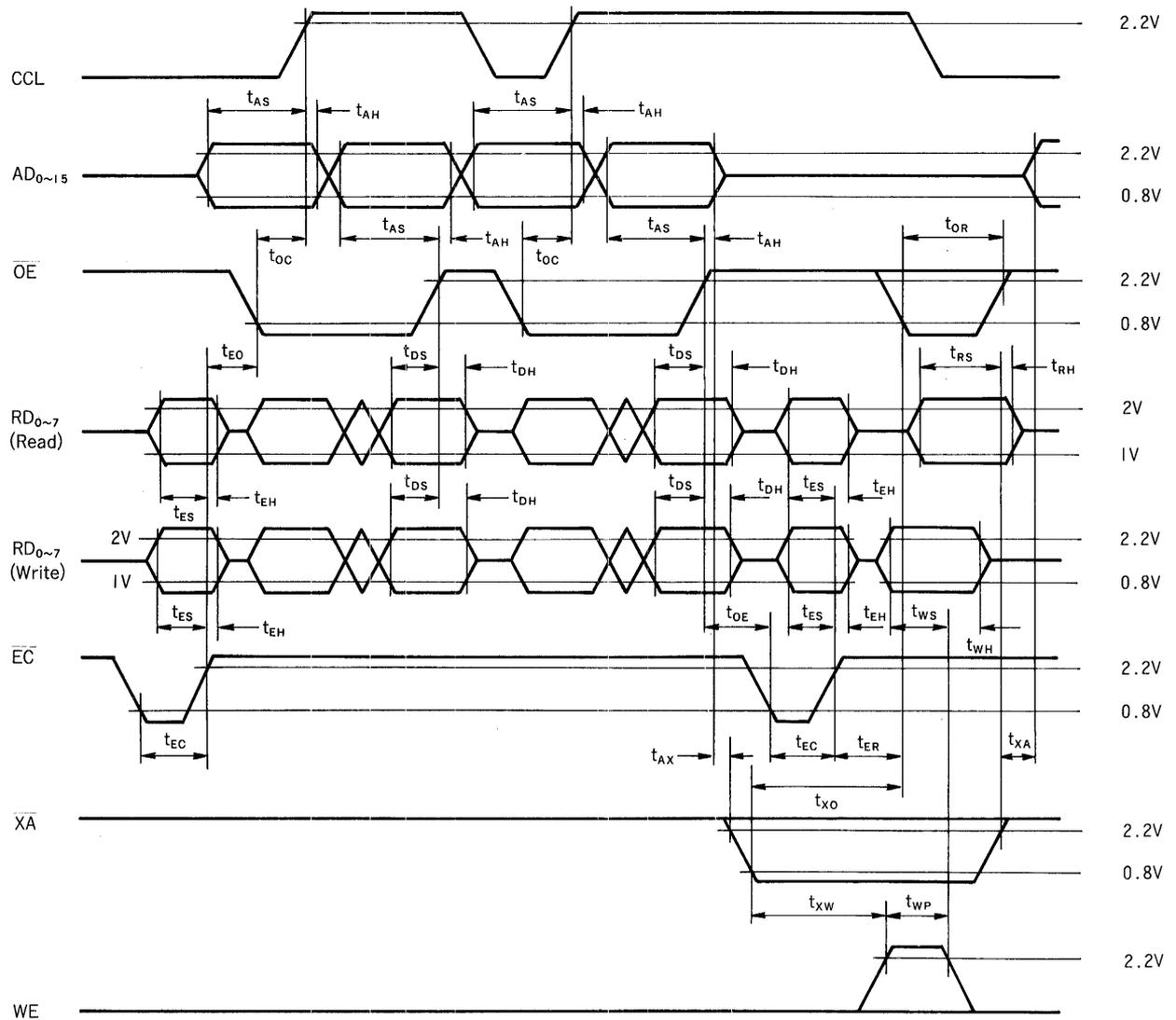
8-4-3-2. 8-Bit Bus in DRAM Mode (@fMaster Clock = 16.257 MHz, Cl = 100pF + 2LSTTL)
