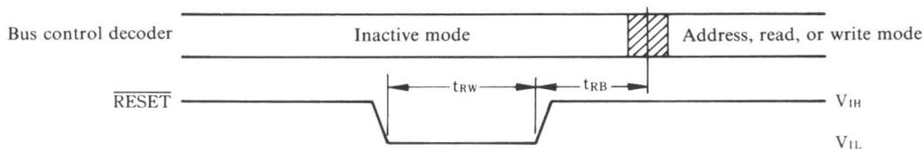
Fig. 6 Reset timing
