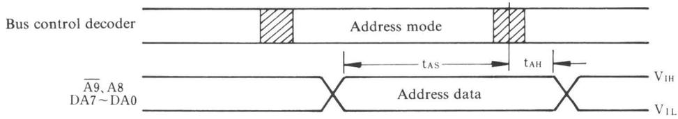
Fig. 7 Address timing
