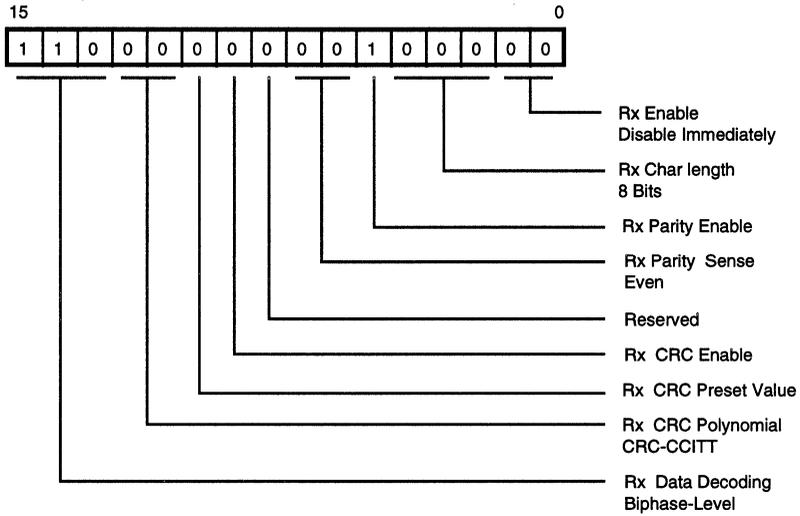
**Figure 6. Receive Mode Register**
