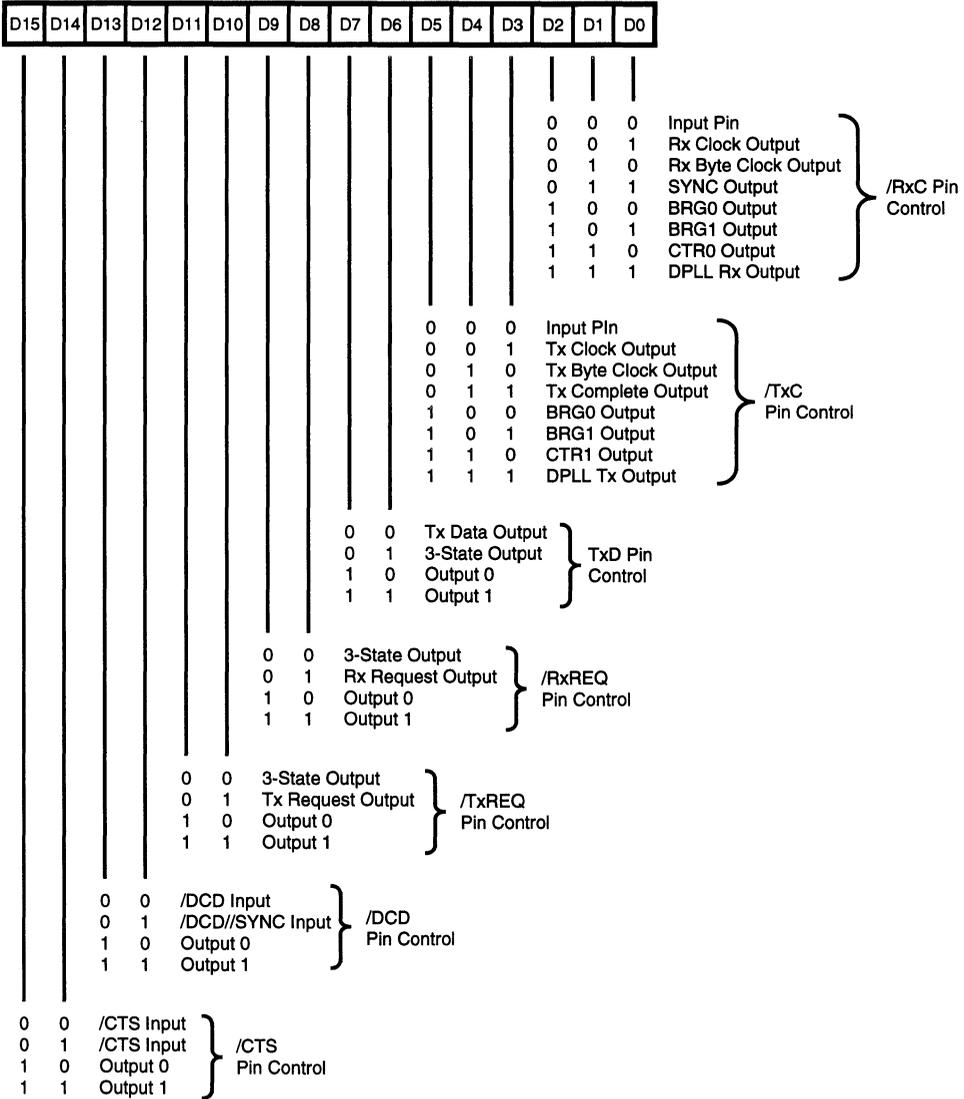
Figure 30. I/O Control Register
