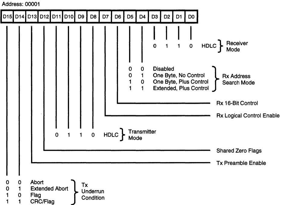
Figure 15. Channel Mode Register, HDLC Mode
