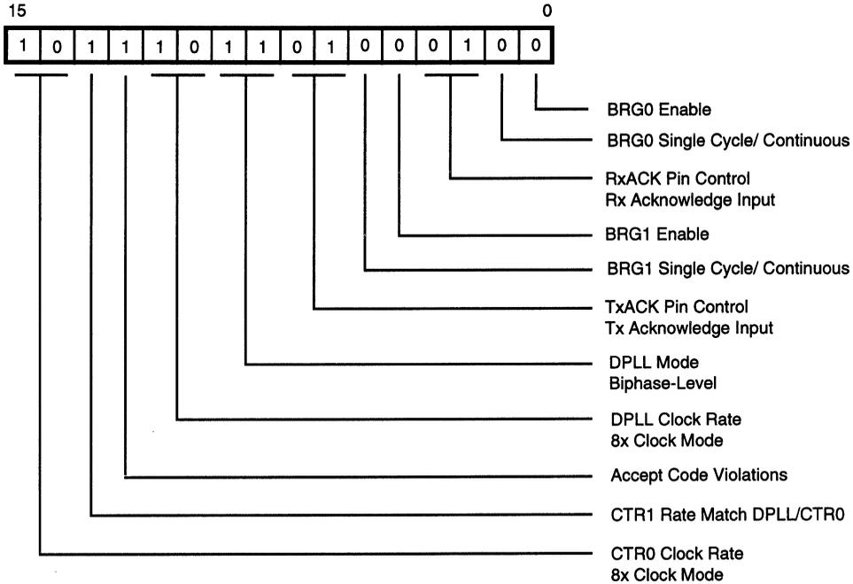
**Figure 4. Hardware Configuration Register**
