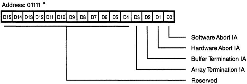
**Figure 19. Tx/Rx DMA Interrupt Arm (TDIAR)/(RDIAR)**
