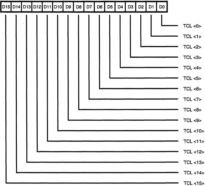
**Figure 75. Transmit Count Limit Register (TCLR)**
