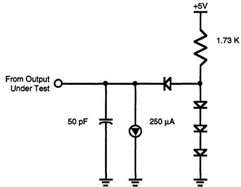
**Figure 81. Standard Test Load**
