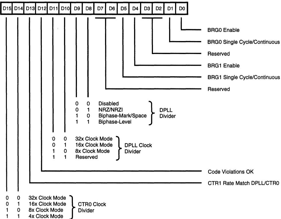
**Figure 55. Hardware Configuration Register (HCR)**
