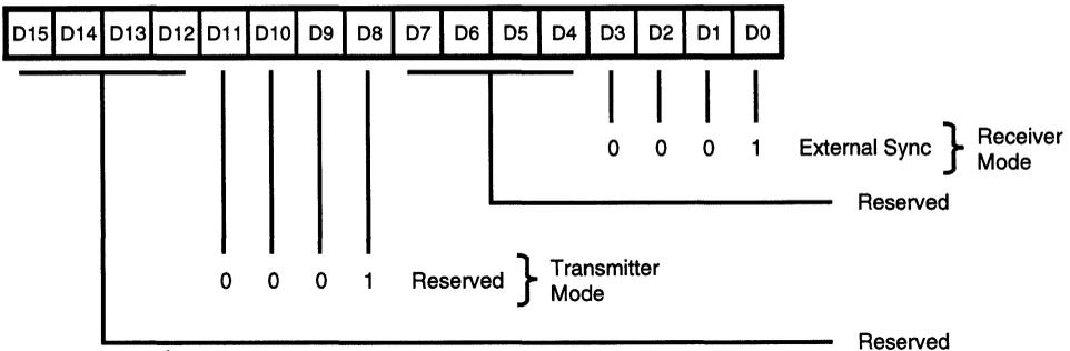
Figure 37. Channel Mode Register, External Sync Mode
