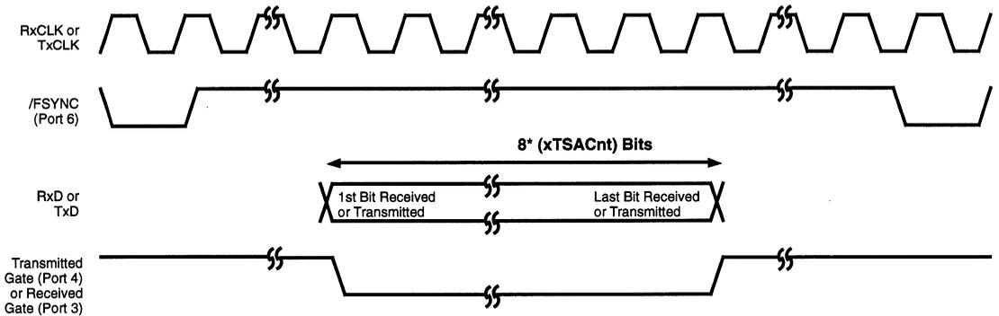
Figure 2. Length of Received or Transmitted Data in a TSA Application
