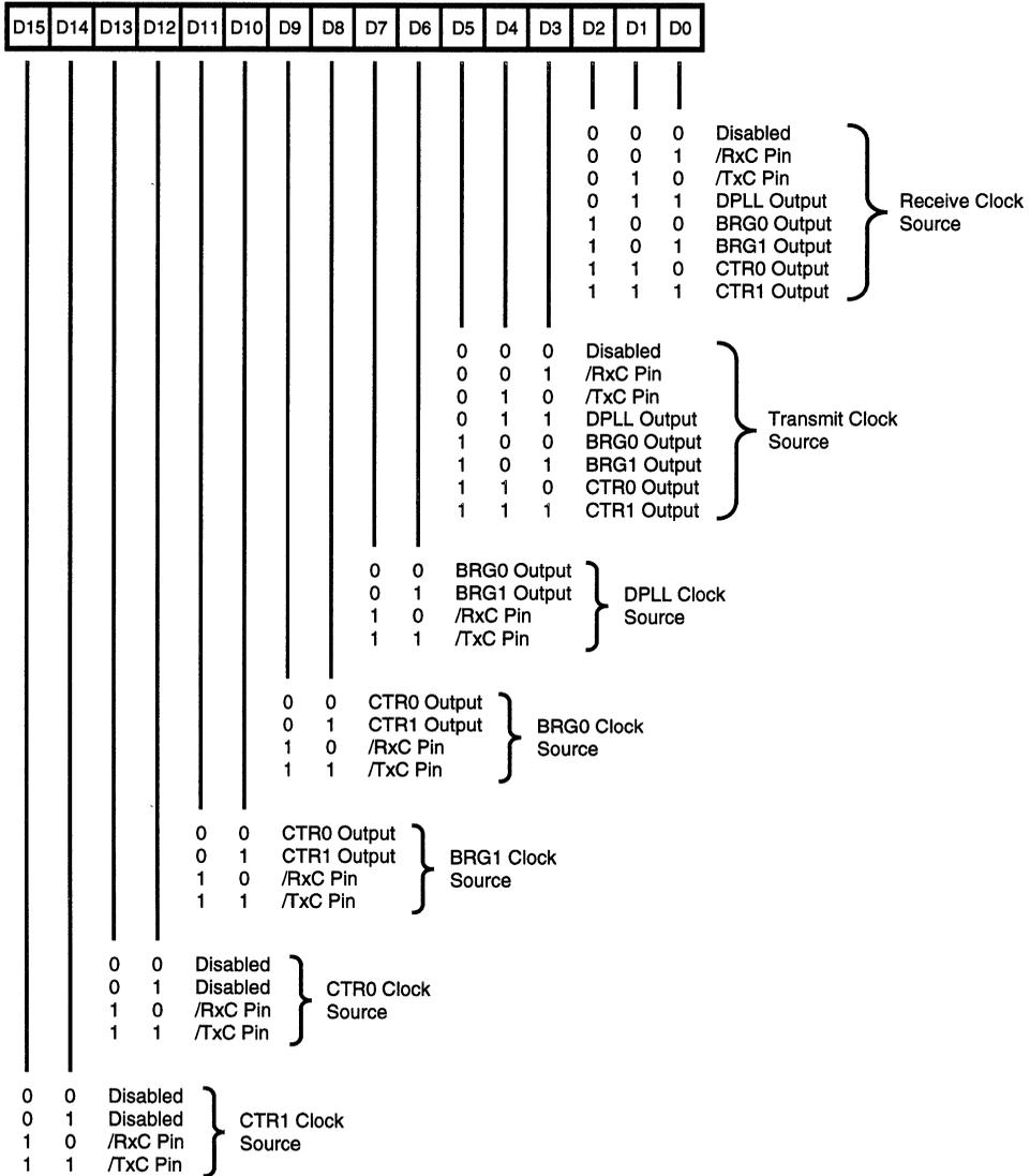
Figure 27. Clock Mode Control Register
