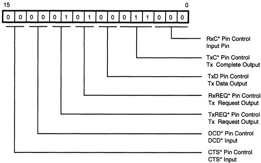
**Figure 5. I/O Control Register**
