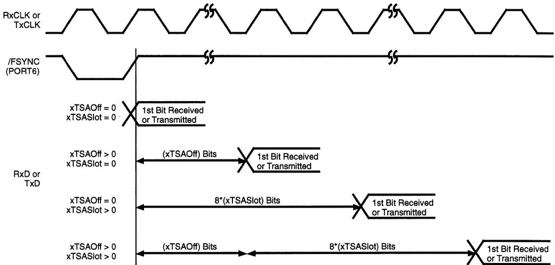
Figure 1. Start of Received or Transmitted Data in a TSA Application
