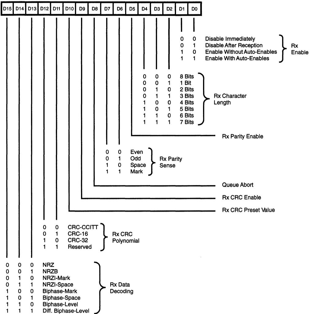
Figure 36. Receive Mode Register
