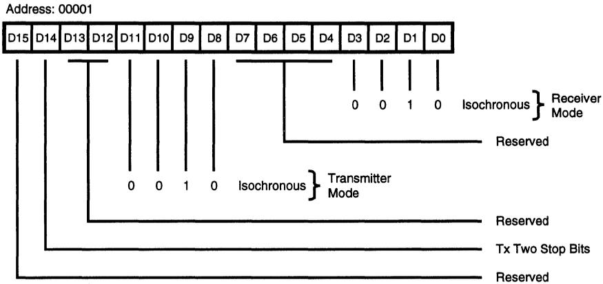
Figure 11. Channel Mode Register, Isochronous Mode
