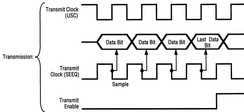
Note: /Transmit Clock Pin of USC is Programmed to be used as a Signal to Flag the End of Transmit.
