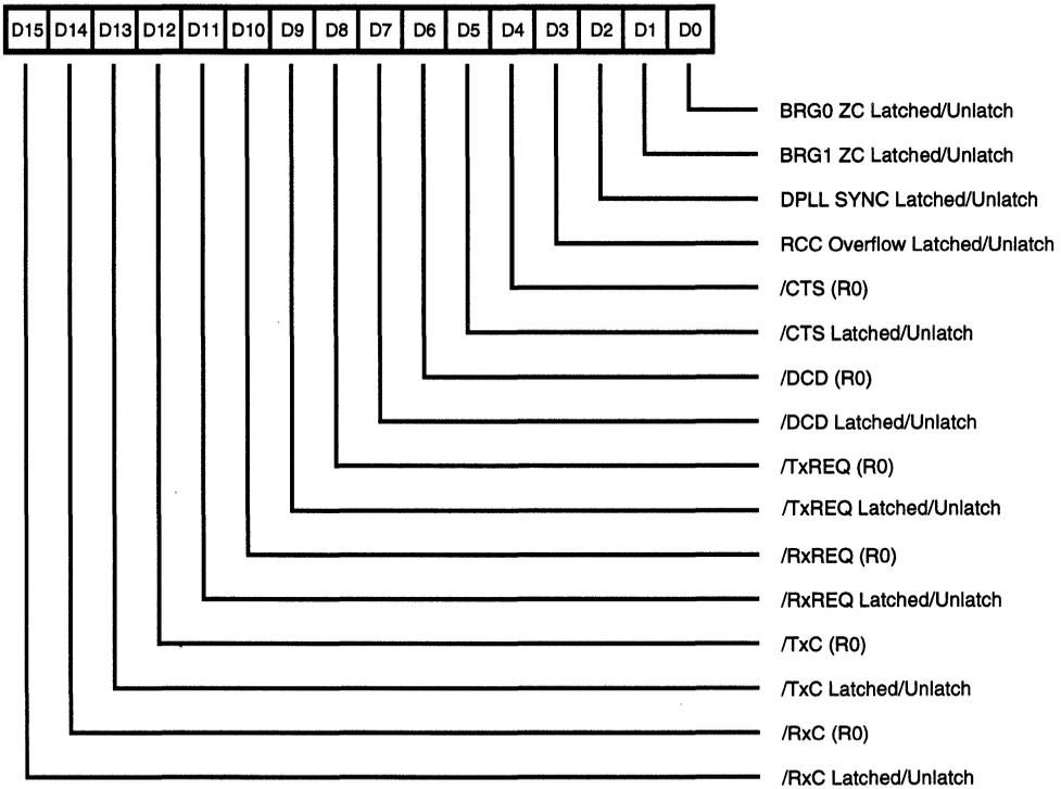
**Figure 33. Miscellaneous Interrupt Status Register**
