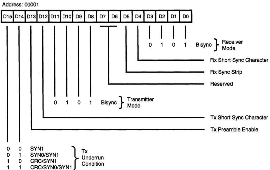
Figure 14. Channel Mode Register, Bisync Mode
