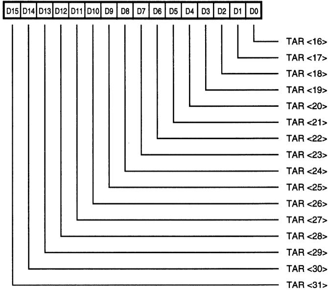
Figure 22. Tx/Rx Address Register (Upper) (TARU)/(RARU)
