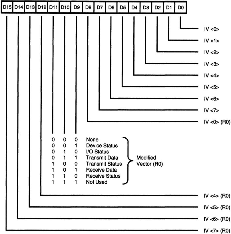
**Figure 29. Interrupt Vector Register**
