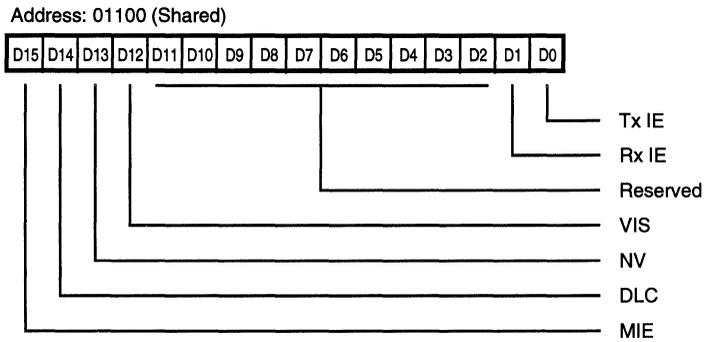
**Figure 16. DMA Interrupt Control Register (DICR)**
