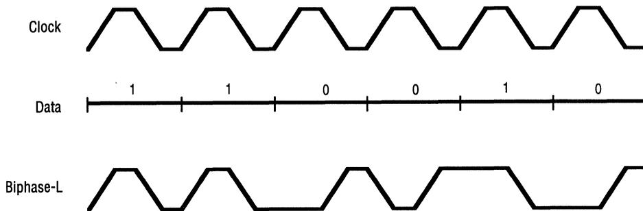
Figure 2. Manchester II (Bi-phase-Level) Data Encoding
