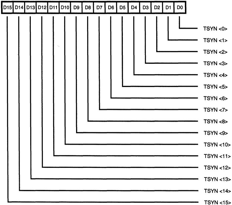
**Figure 47. Transmit Sync Register**
