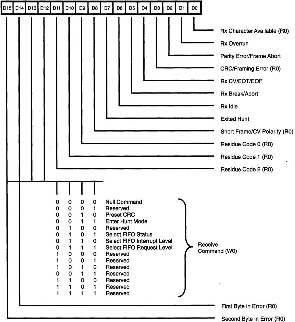
Figure 37. Receive Command Status Register
