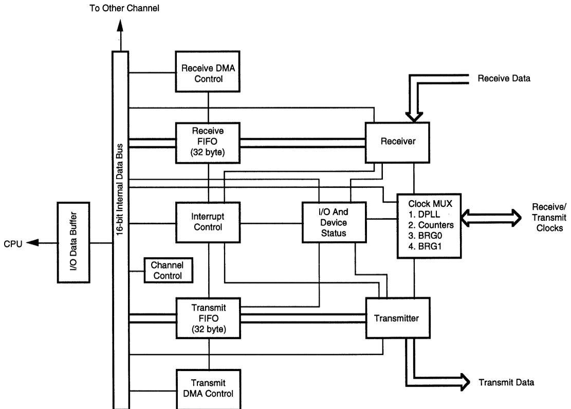
Figure 2. Z16C30 Universal Serial Controller
