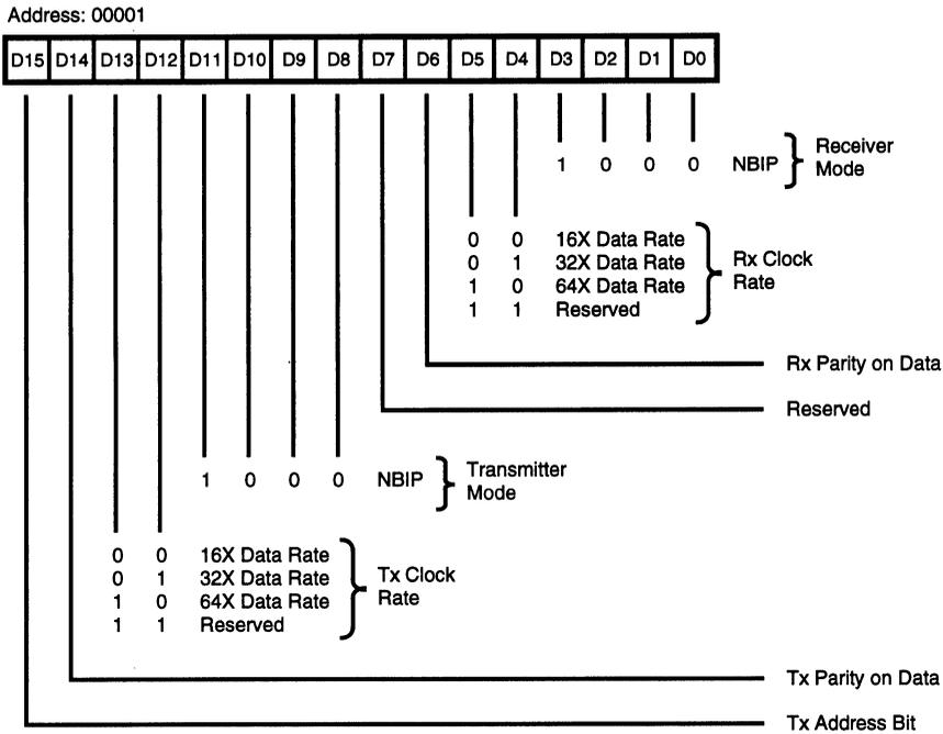
Figure 44. Channel Mode Register, NBIP Mode
