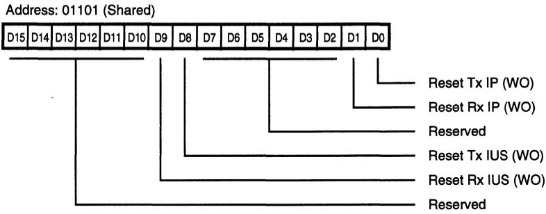
**Figure 17. Clear DMA Interrupt Register (CDIR)**
