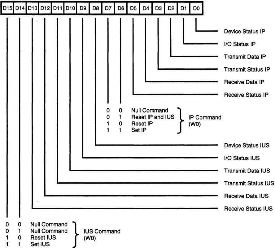
Figure 32. Daisy-Chain Control Register
