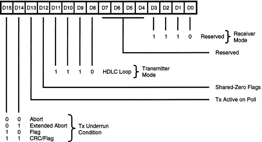
**Figure 47. Channel Mode Register, HDLC Loop Mode**
