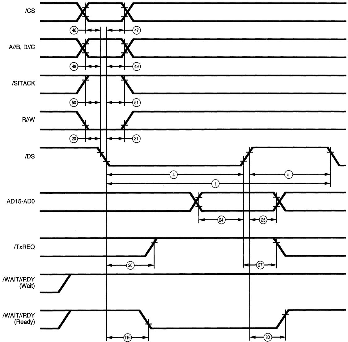
Figure 64. Non-Multiplexed /DS Write Cycle
