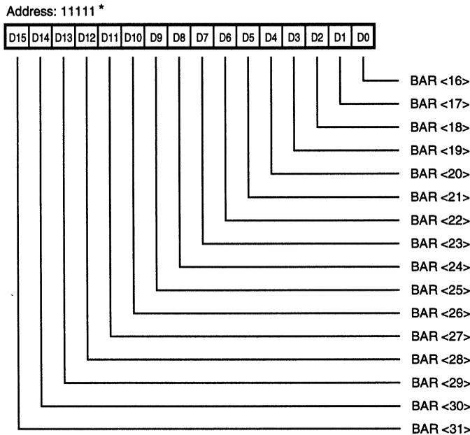
Figure 25. Next Tx/Rx Address Register (Upper) (NTARU)/(RTARU)
