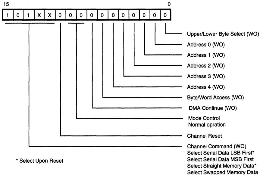
**Figure 13. Channel Command/Address Register**
