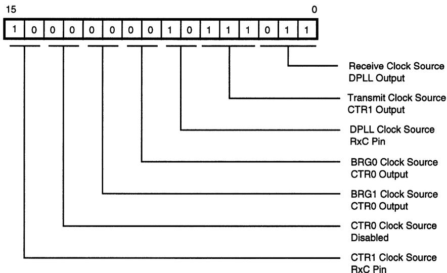
**Figure 3. Clock Mode Control Register**
