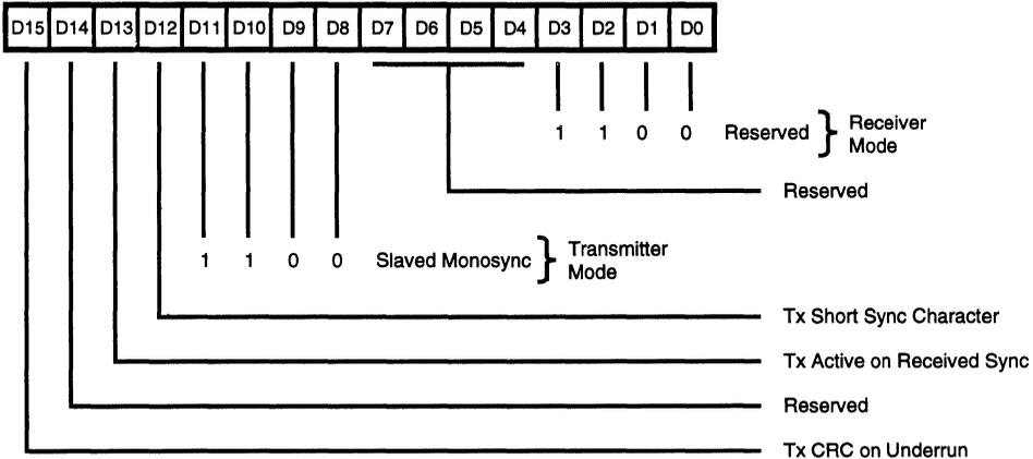
Figure 19. Channel Mode Register, Slaved Monosync Mode
