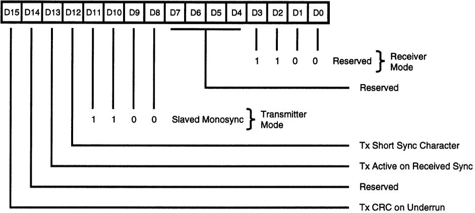
**Figure 46. Channel Mode Register, Slaved Monosync Mode**
