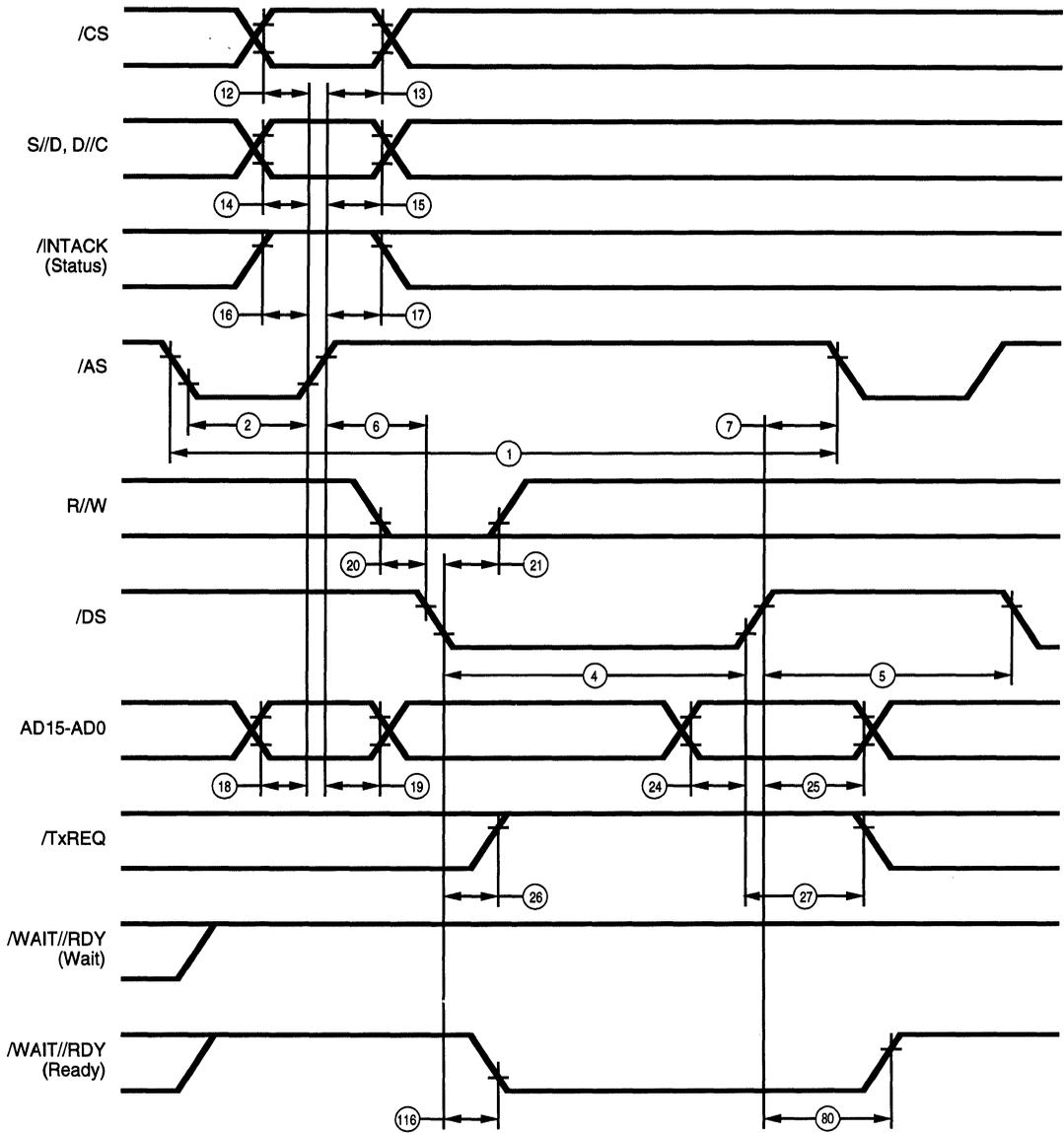
Figure 85. Multiplexed /DS Write Cycle
