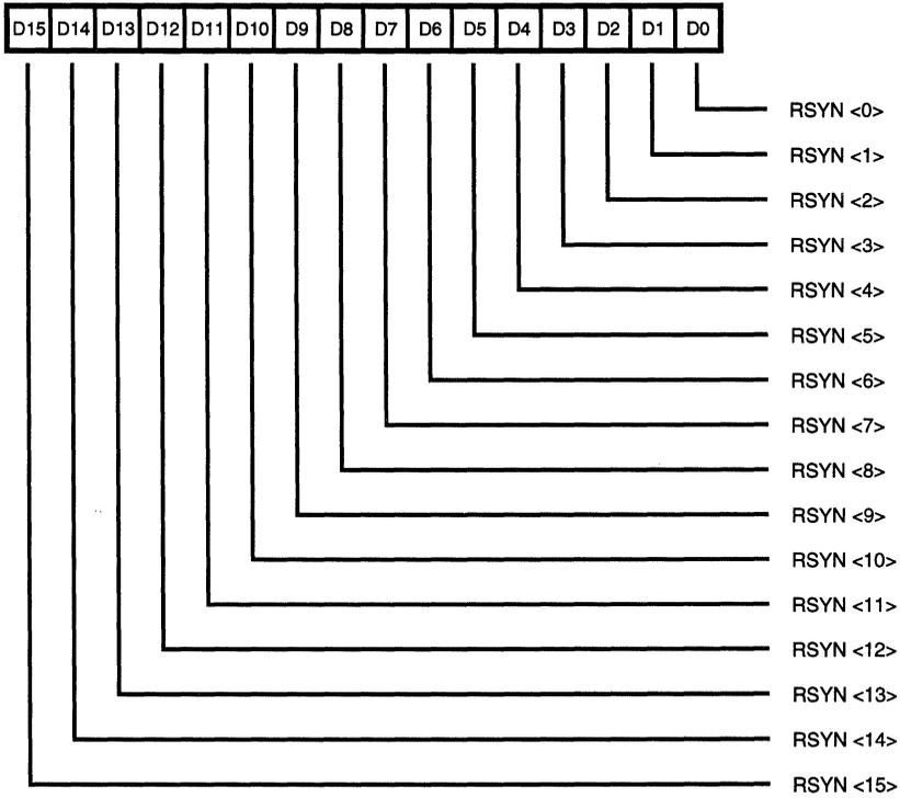
**Figure 66. Receive Sync Register (RSR)**
