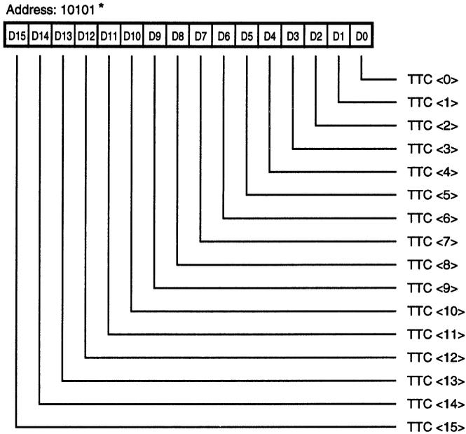
**Figure 20. Tx/Rx Byte Count Register (TBCR)/(RBCR)**
