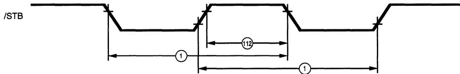
Figure 56. Bus Cycle Timing
