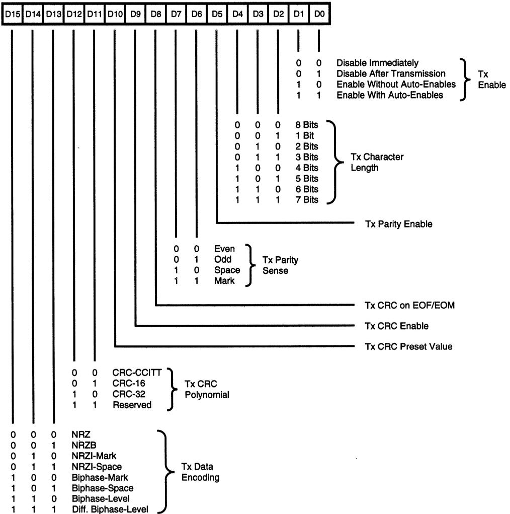
Figure 44. Transmit Mode Register
