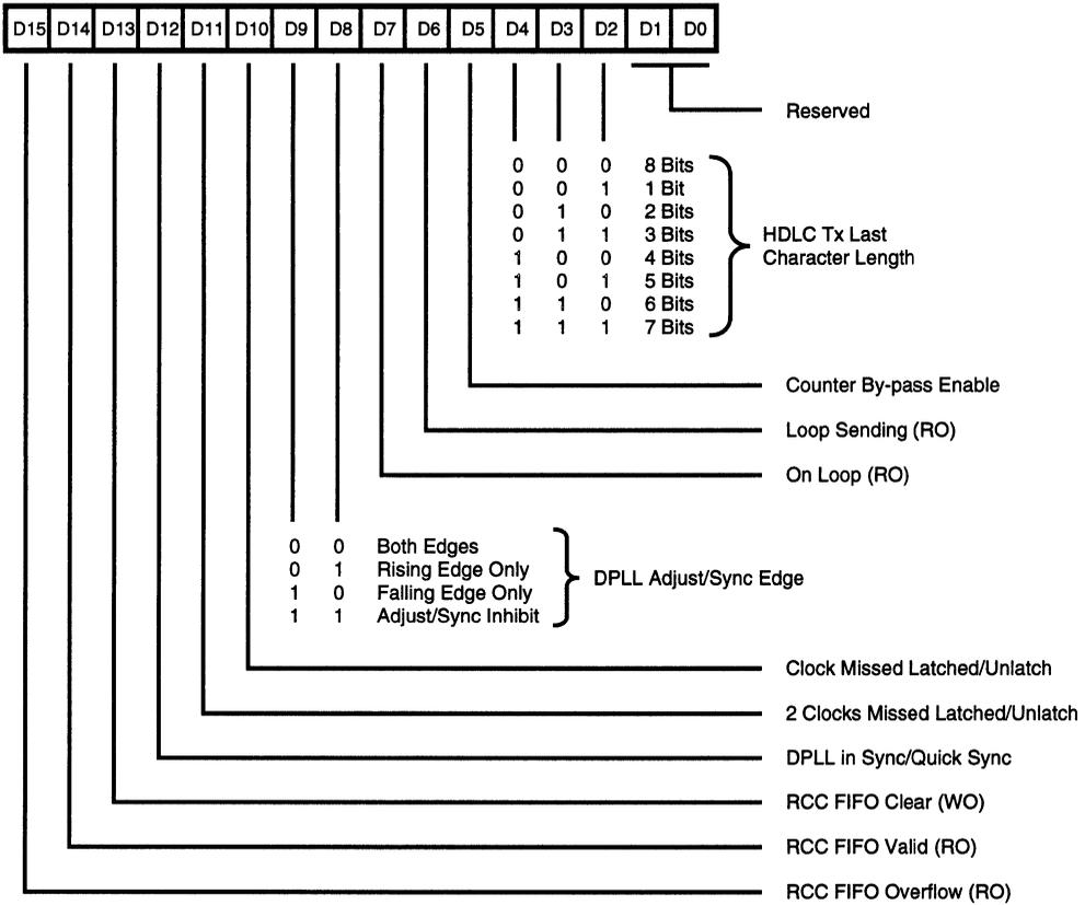
Figure 48. Channel Command/Status Register (CCSR)
