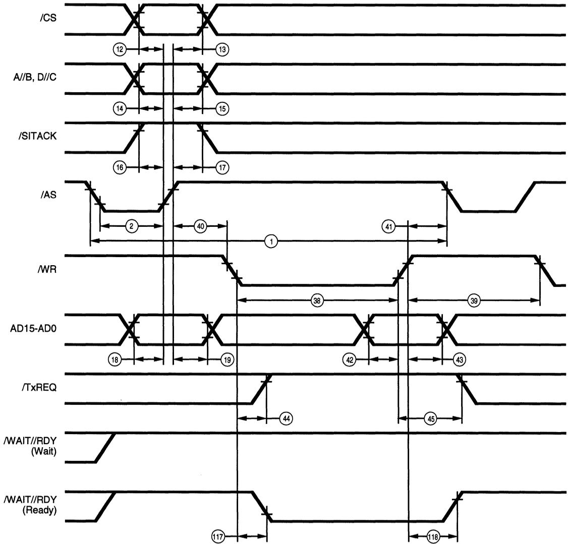
Figure 62. Multiplexed /WR Write Cycle
