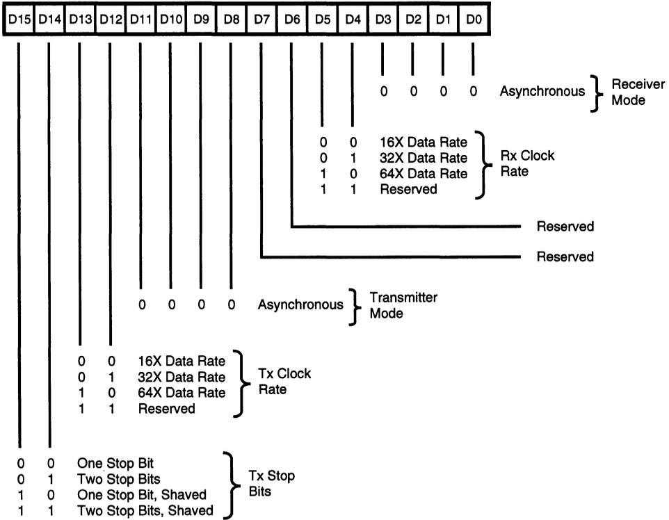
Figure 36. Channel Mode Register, Asynchronous Mode
