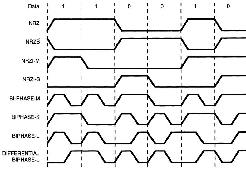
Figure 5. Data Encoding
