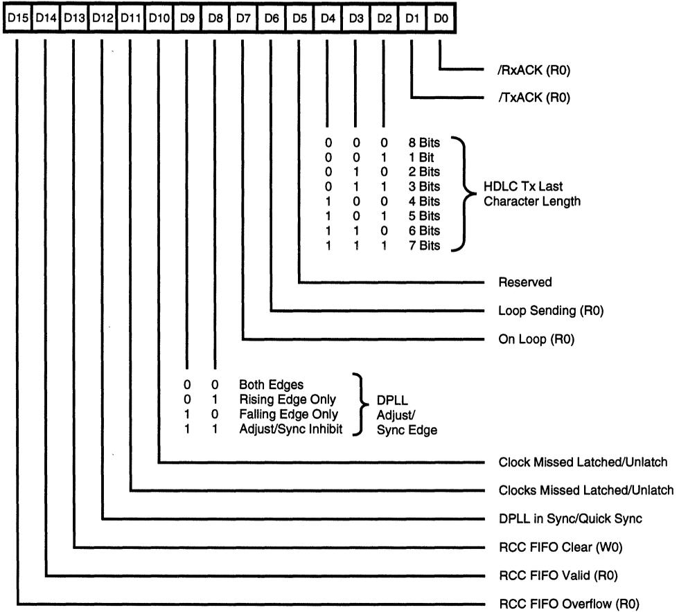
Figure 21. Channel Command/Status Register
