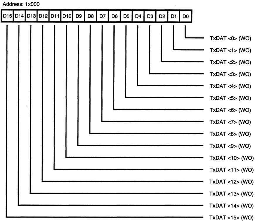
Figure 70. Transmit Data Register (TDR)
