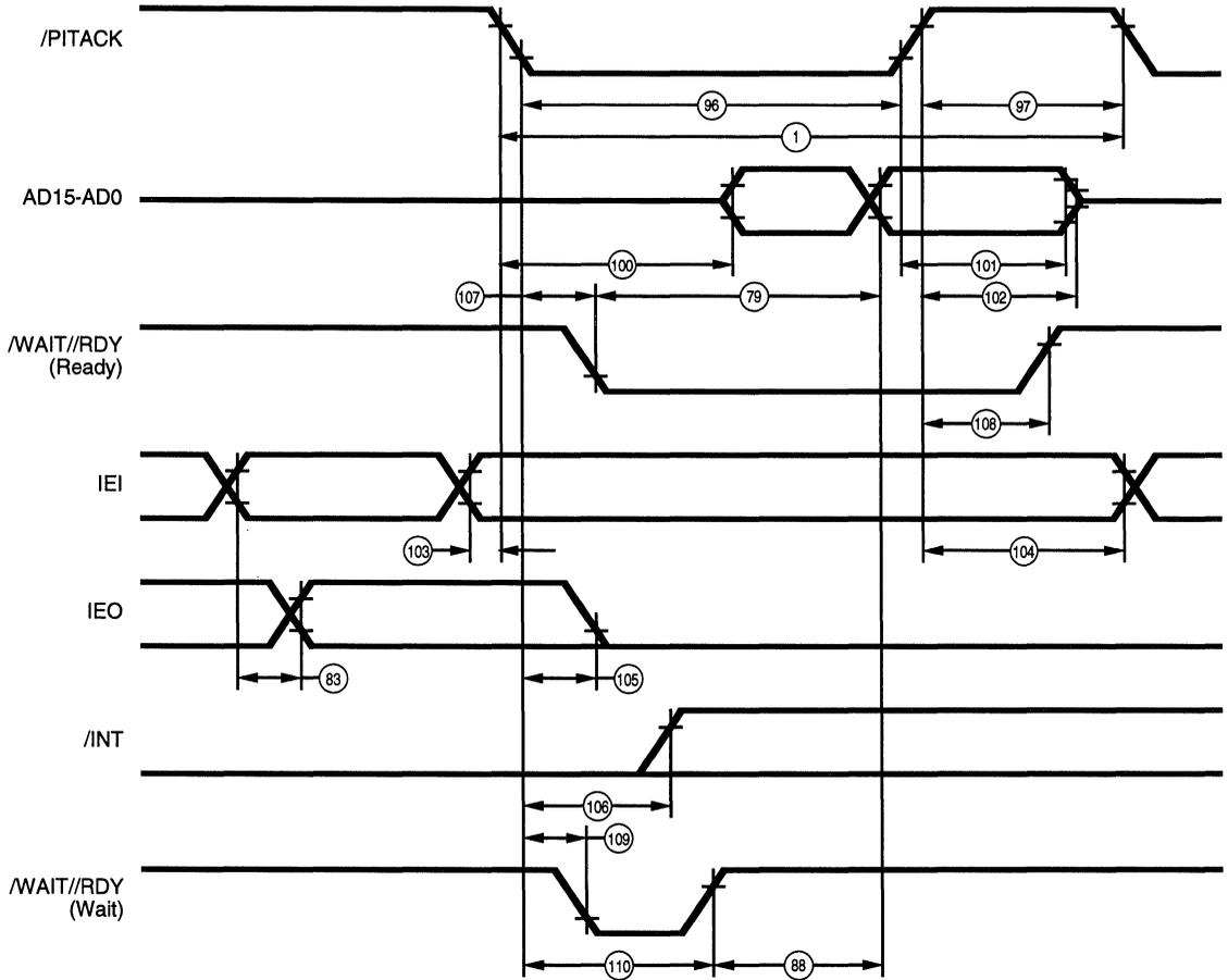
Figure 72. Non-Multiplexed Pulsed Interrupt Acknowledge Cycle
