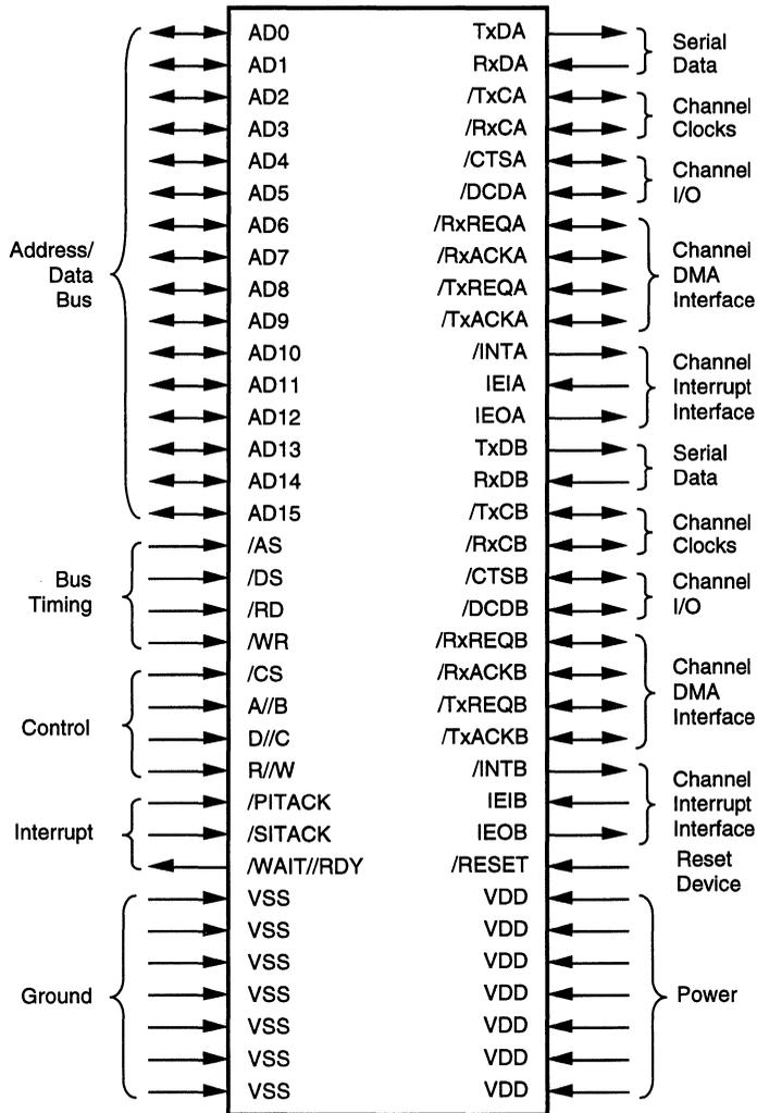
Figure 2. Pin Functions
