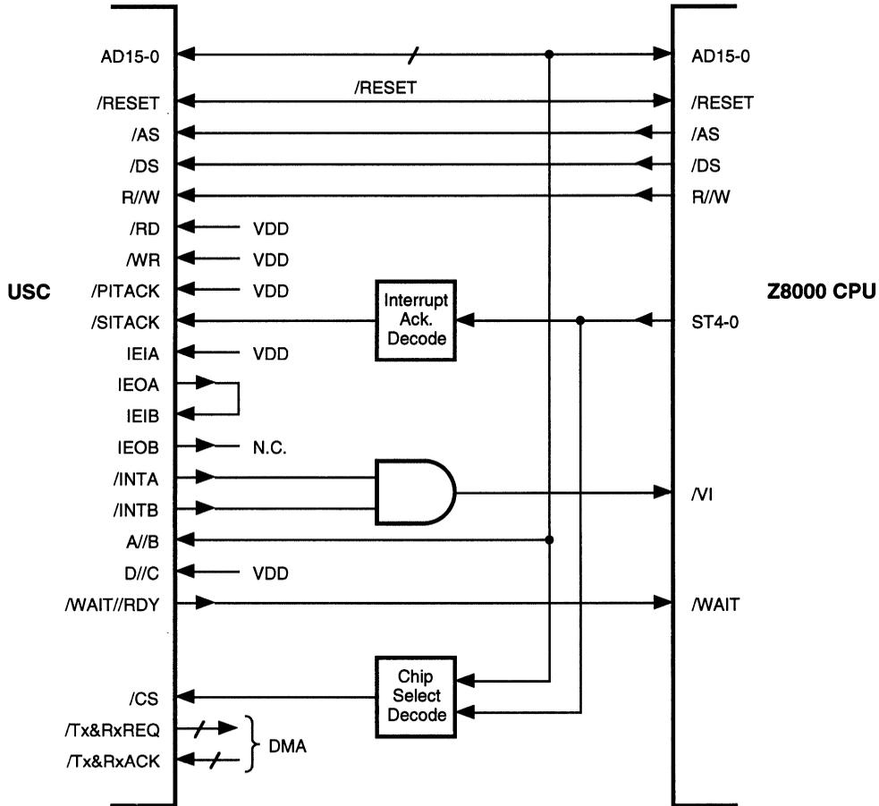
**Figure 16. USC to Z8000 CPU Connection (Example)**
