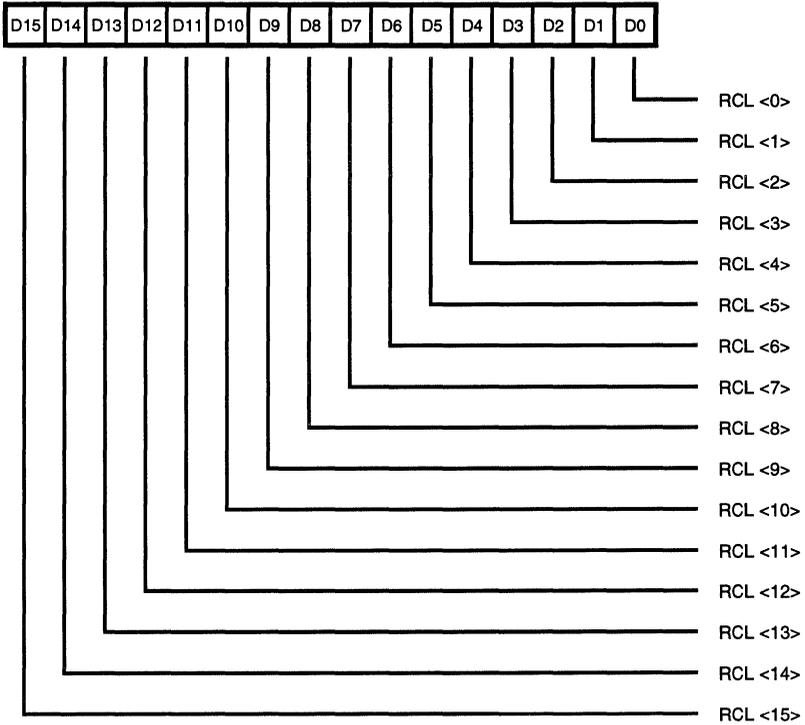
Figure 67. Receive Count Limit Register (RCLR)
