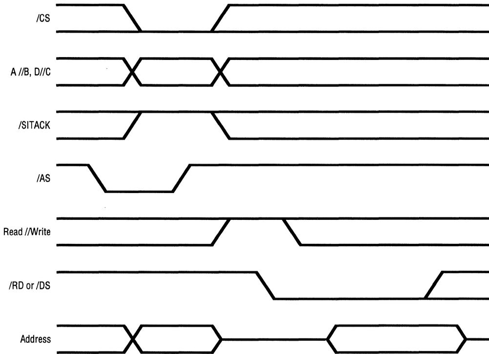
Figure 4. USC/Ethernet Interface and Two Channel Read/Write Data
