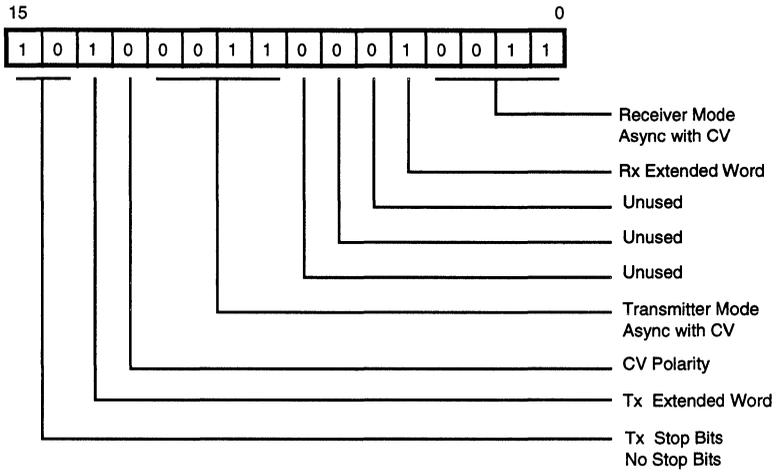
Figure 8. Channel Mode Register
