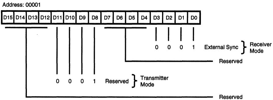
Figure 10. Channel Mode Register, External Sync Mode
