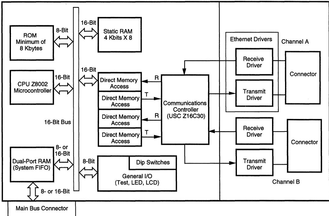
**Figure 1. IBM 80386 PC Dual-Channel Communications Board**
