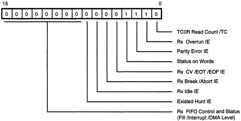
Figure 9. Receive Interrupt Control Register
