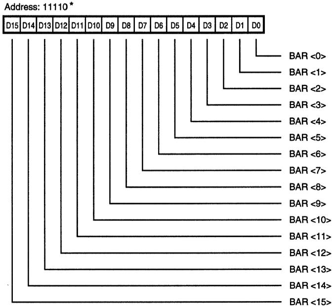
Figure 24. Next Tx/Rx Address Register (Lower) (NTARL)/(RTARL)
