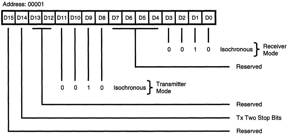
**Figure 38. Channel Mode Register, Isochronous Mode**
