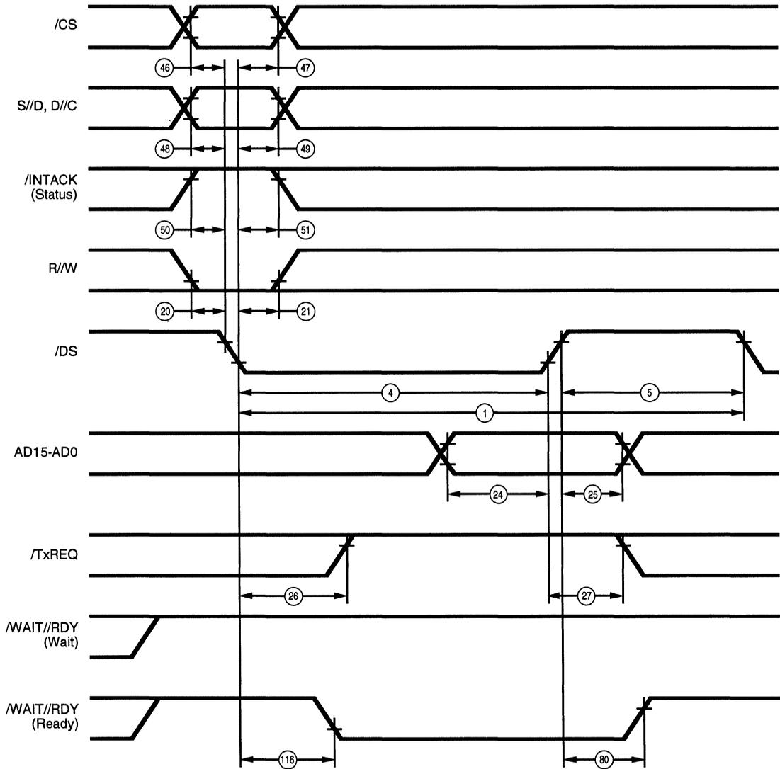
**Figure 89. Non-Multiplexed /DS Write Cycle**
