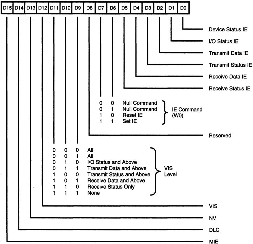
**Figure 31. Interrupt Control Register**
