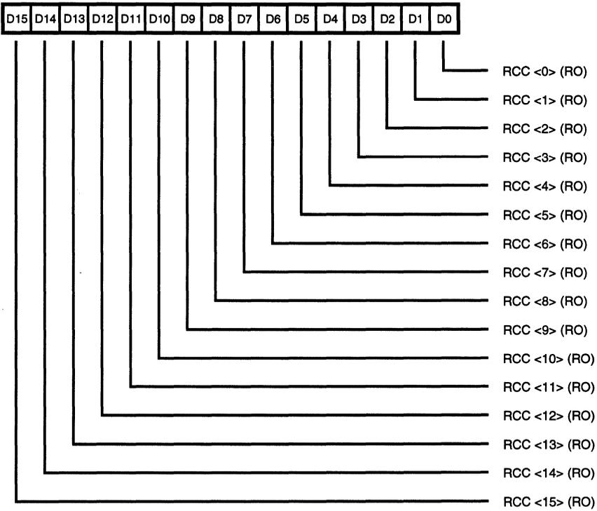
**Figure 68. Receive Character Count Register (RCCR)**
