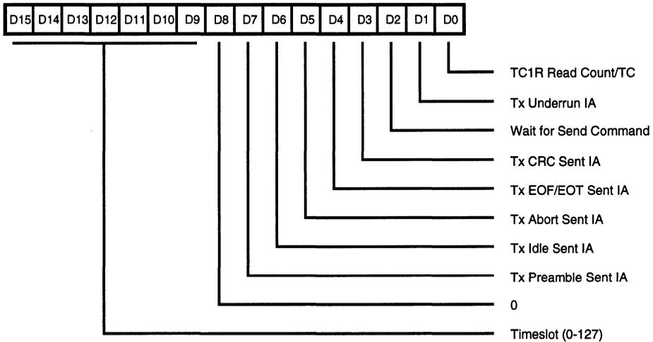
Figure 73b. Transmit Interrupt Control Register (TICR)
