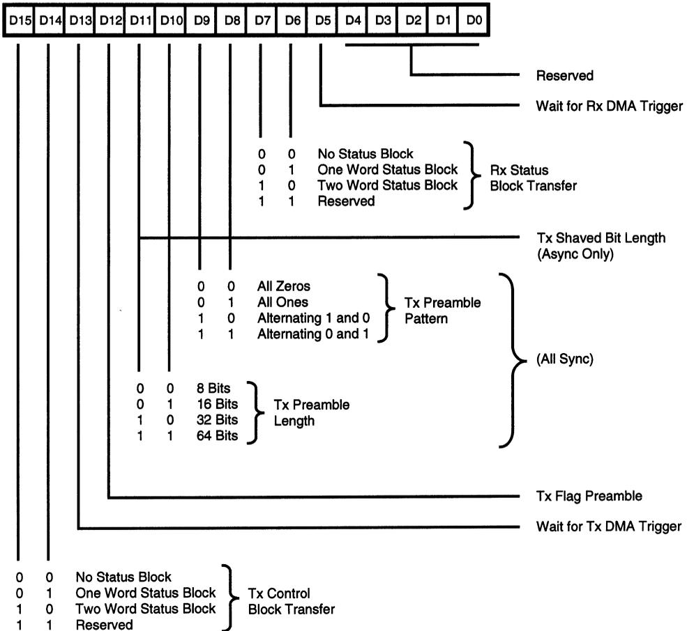
**Figure 49. Channel Control Register (CCR)**
