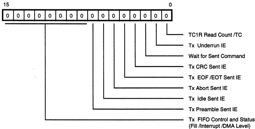
**Figure 10. Transmit Interrupt Control Register**
