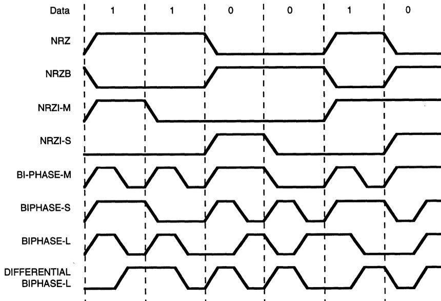
**Figure 5. Data Encoding**
