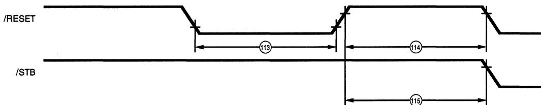
**Figure 82. Reset Timing**
