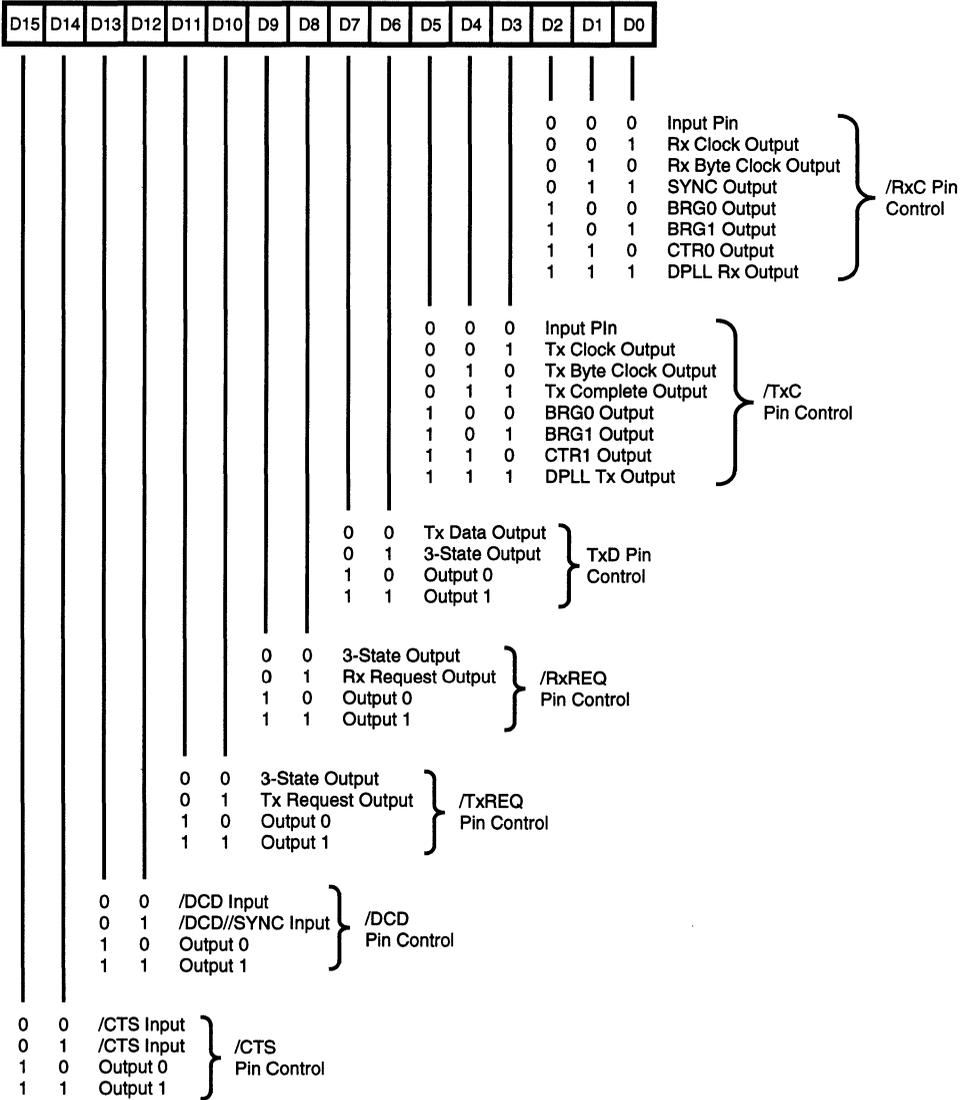
**Figure 57. I/O Control Register (IOCR)**
