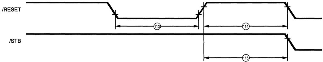
Figure 55. Reset Timing
