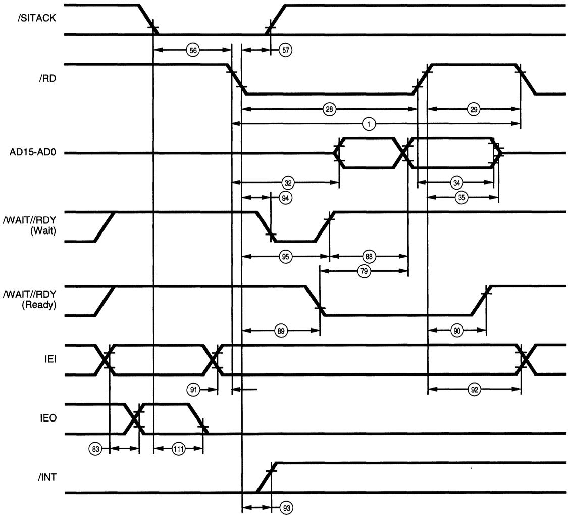
Figure 71. Non-Multiplexed /RD Interrupt Acknowledge Cycle
