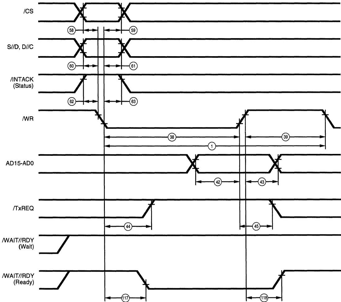
**Figure 91. Non-Multiplexed /WR Write Cycle**
