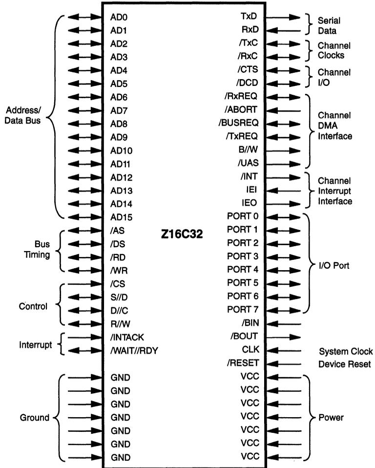
Figure 2. Pin Functions
