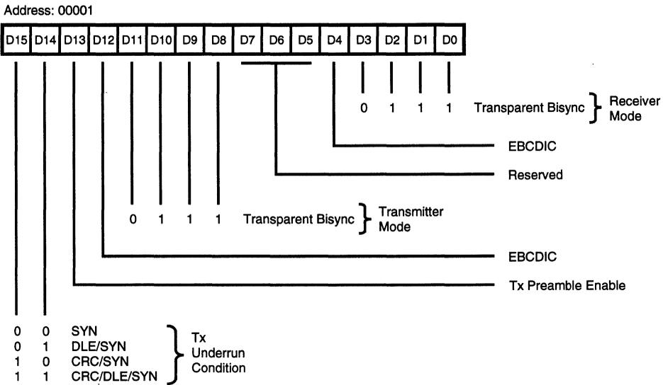
Figure 16. Channel Mode Register, Transparent Bisync Mode
