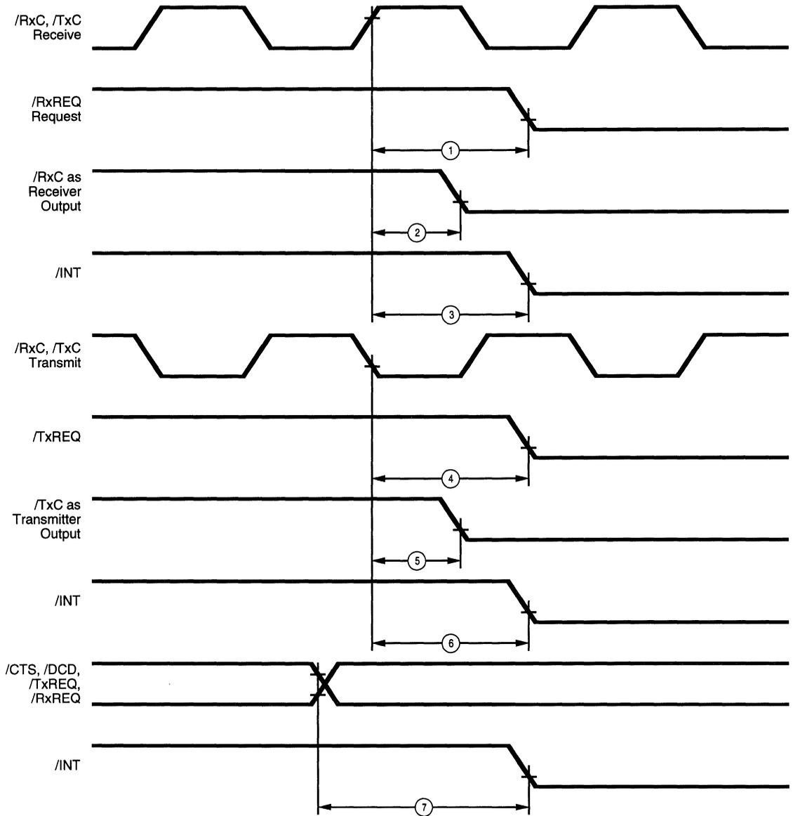
Figure 76. Z16C30 System Timing
