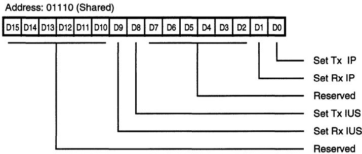
**Figure 18. Set DMA Interrupt Register (SDIR)**
