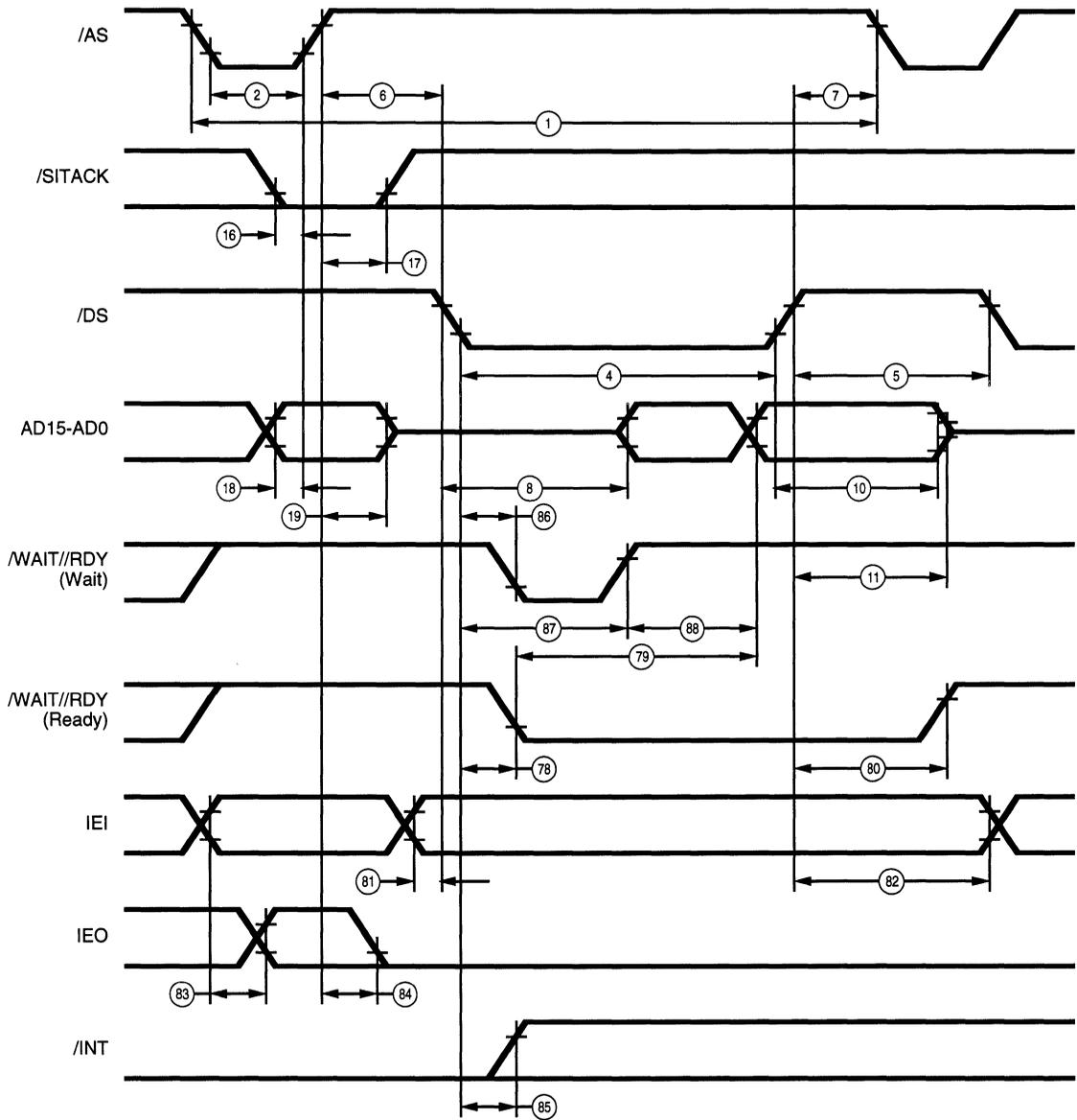
Figure 67. Multiplexed /DS Interrupt Acknowledged Cycle
