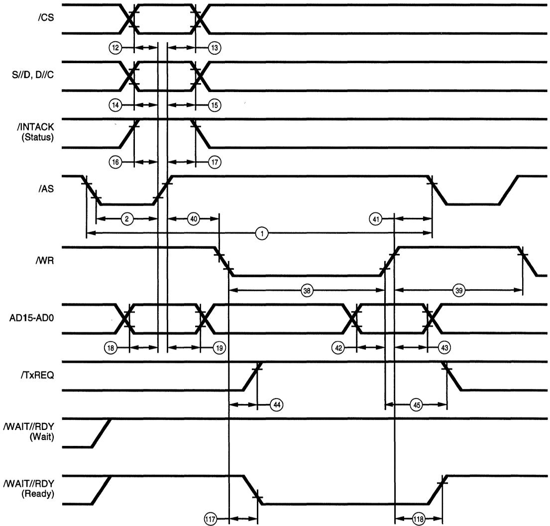
**Figure 87. Multiplexed /WR Write Cycle**
