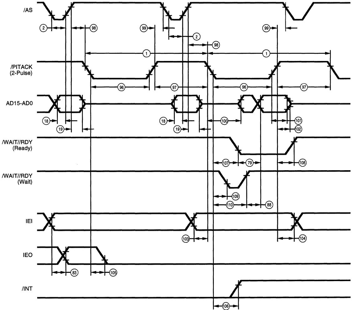
Figure 73. Multiplexed Double-Pulse Intack Cycle
