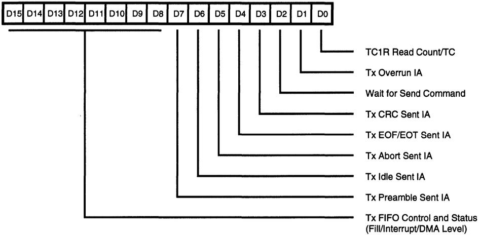
Figure 73a. Transmit Interrupt Control Register (TICR)
