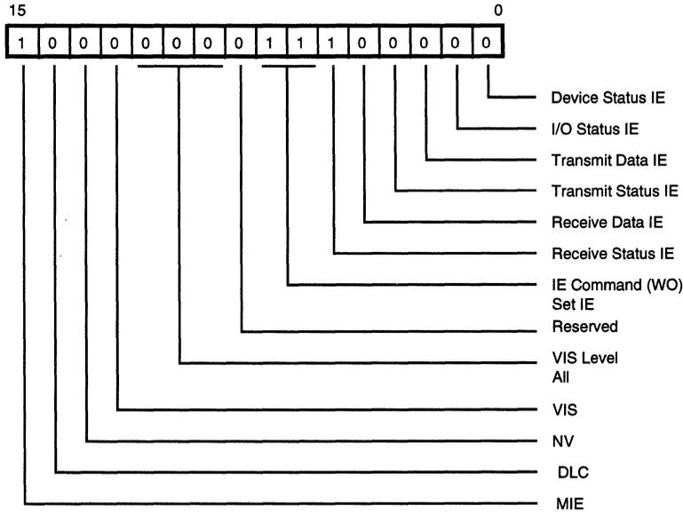
**Figure 12. Interrupt Control Register**
