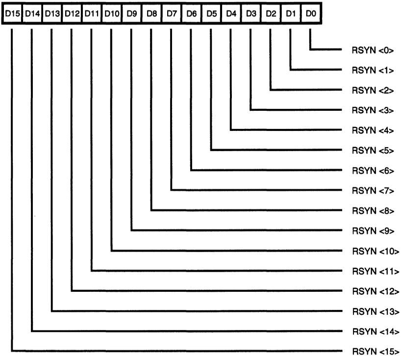
Figure 39. Receive Sync Register
