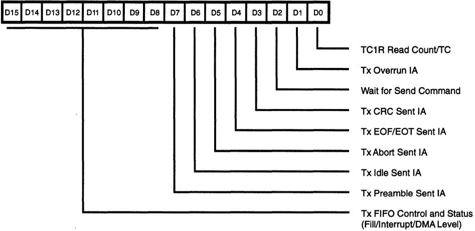
**Figure 46. Transmit Interrupt Control Register**
