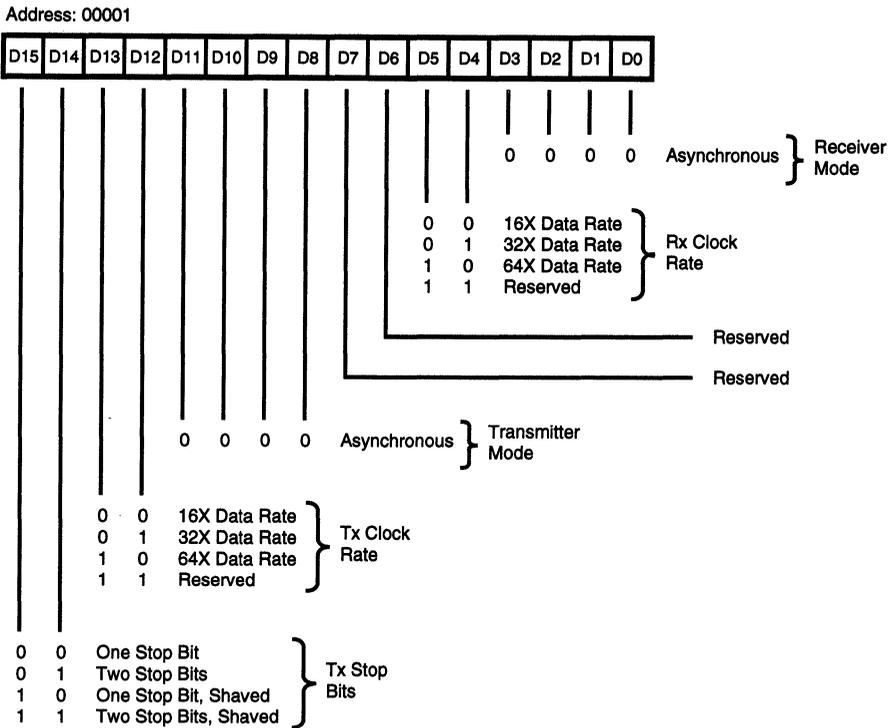
Figure 9. Channel Mode Register, Asynchronous Mode
