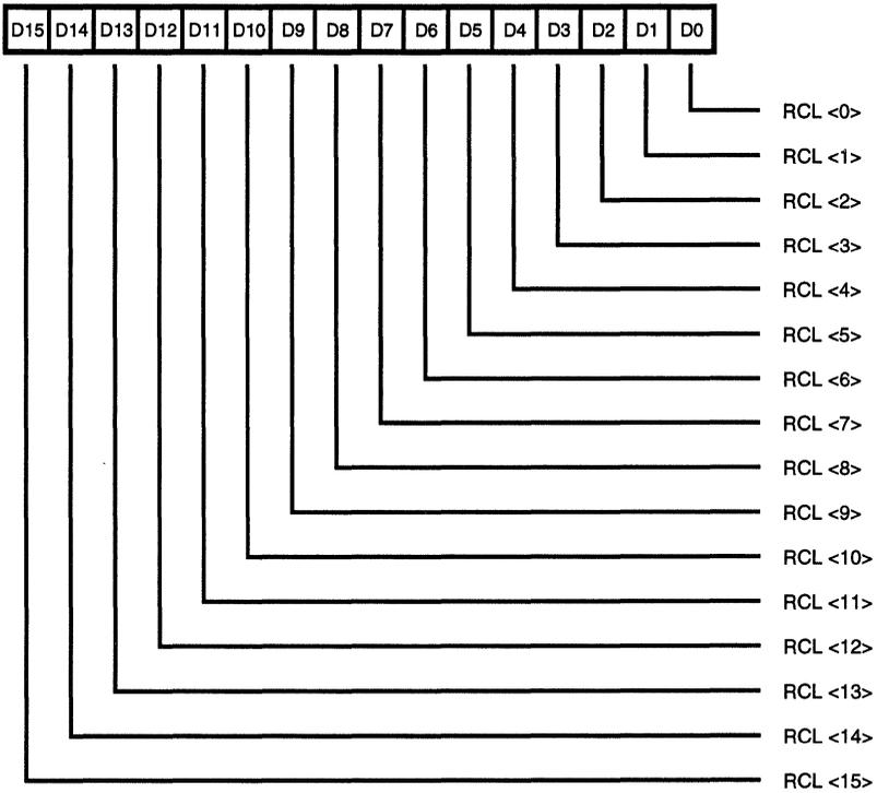
**Figure 40. Receive Count Limit Register**
