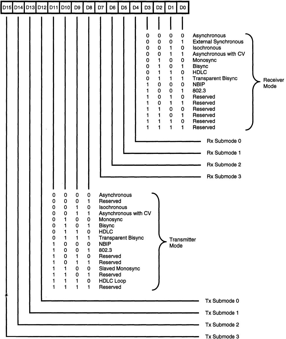
Figure 8. Channel Mode Register
