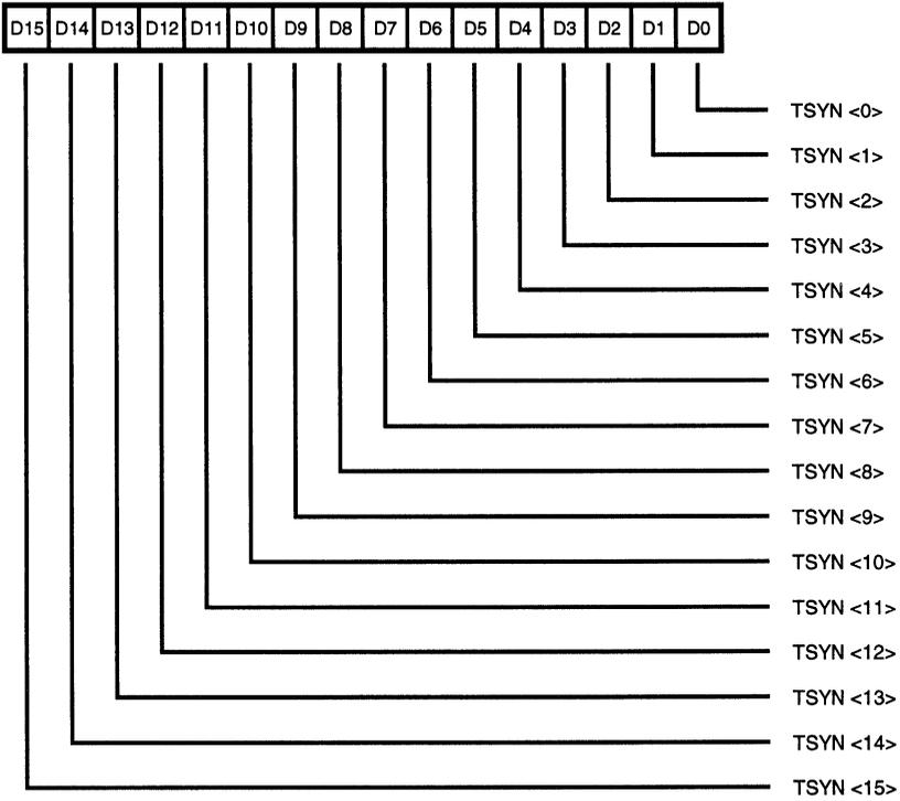
Figure 74. Transmit Sync Register (TSR)
