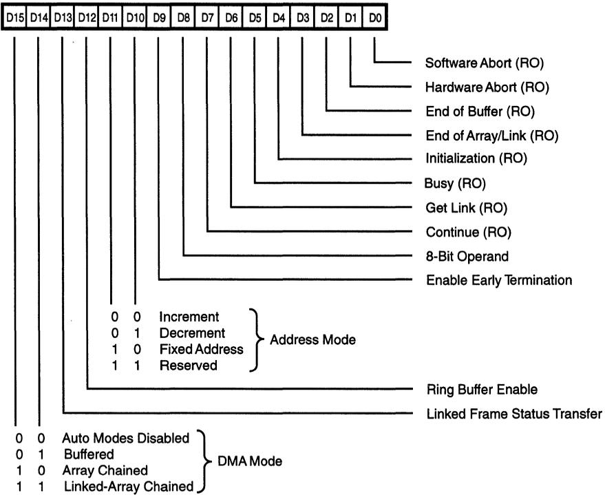
**Figure 9. Tx/Rx DMA Mode Register (TDMR) (RDMR)**
