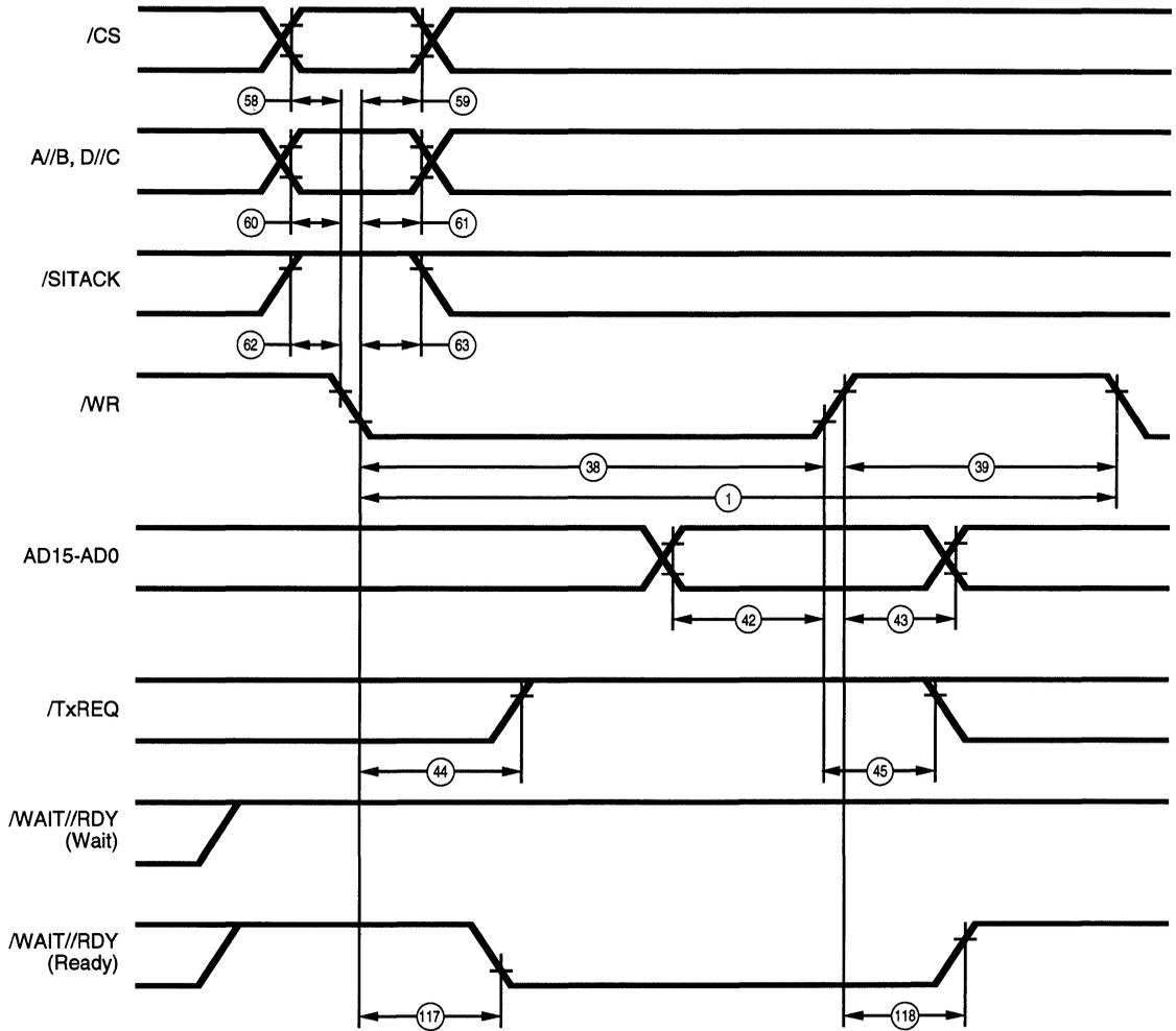
Figure 66. Non-Multiplexed /WR Write Cycle
