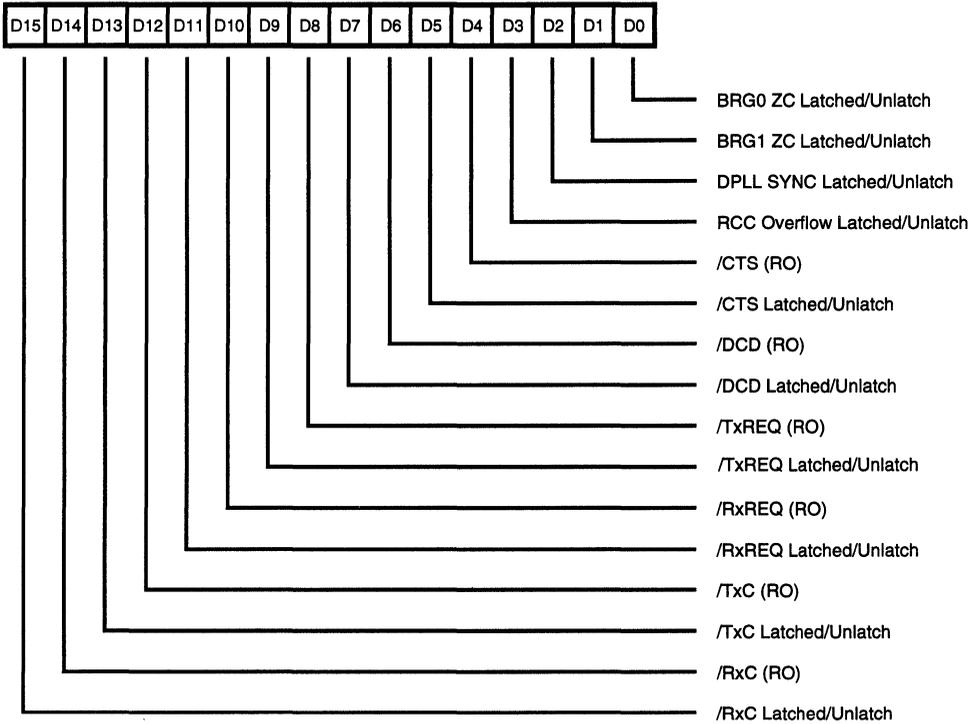
**Figure 60. Miscellaneous Interrupt Status Register (MISR)**
