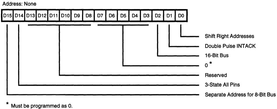
**Figure 4. Bus Configuration Register**
