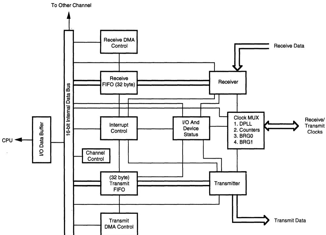
**Figure 1. USC Block Diagram**
