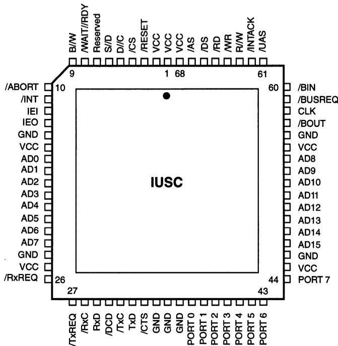
Figure 3. 68-Pin PLCC Pin Assignments
