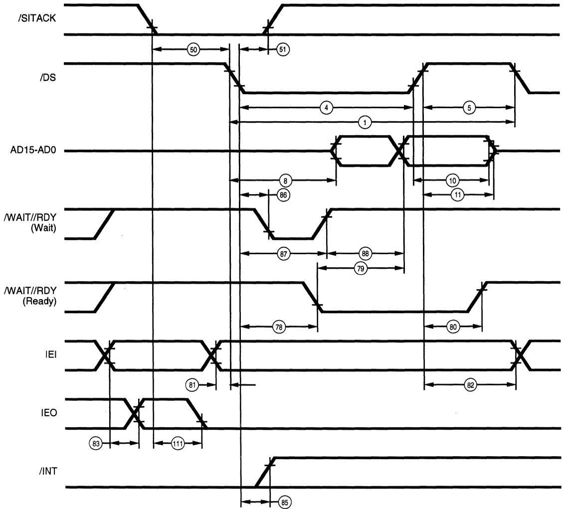
Figure 70. Non-Multiplexed /DS Interrupt Acknowledge Cycle
