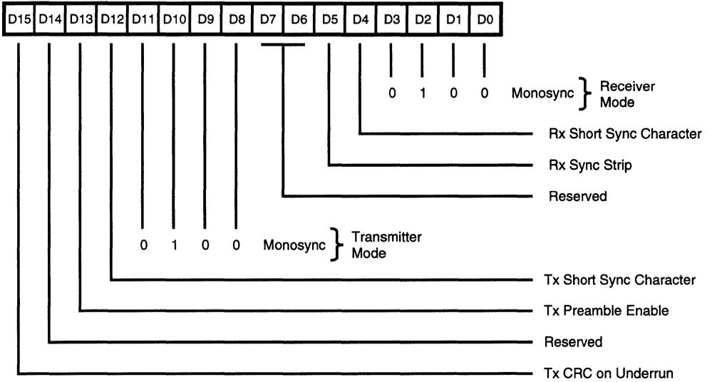
Figure 40. Channel Mode Register, Monosync Mode
