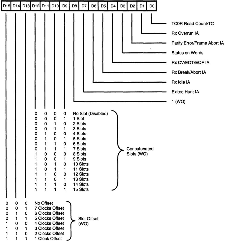
**Figure 65c. Receive Interrupt Control Register (RICR)**
