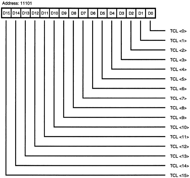
Figure 48. Transmit Count Limit Register
