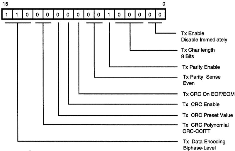
**Figure 7. Transmit Mode Register**
