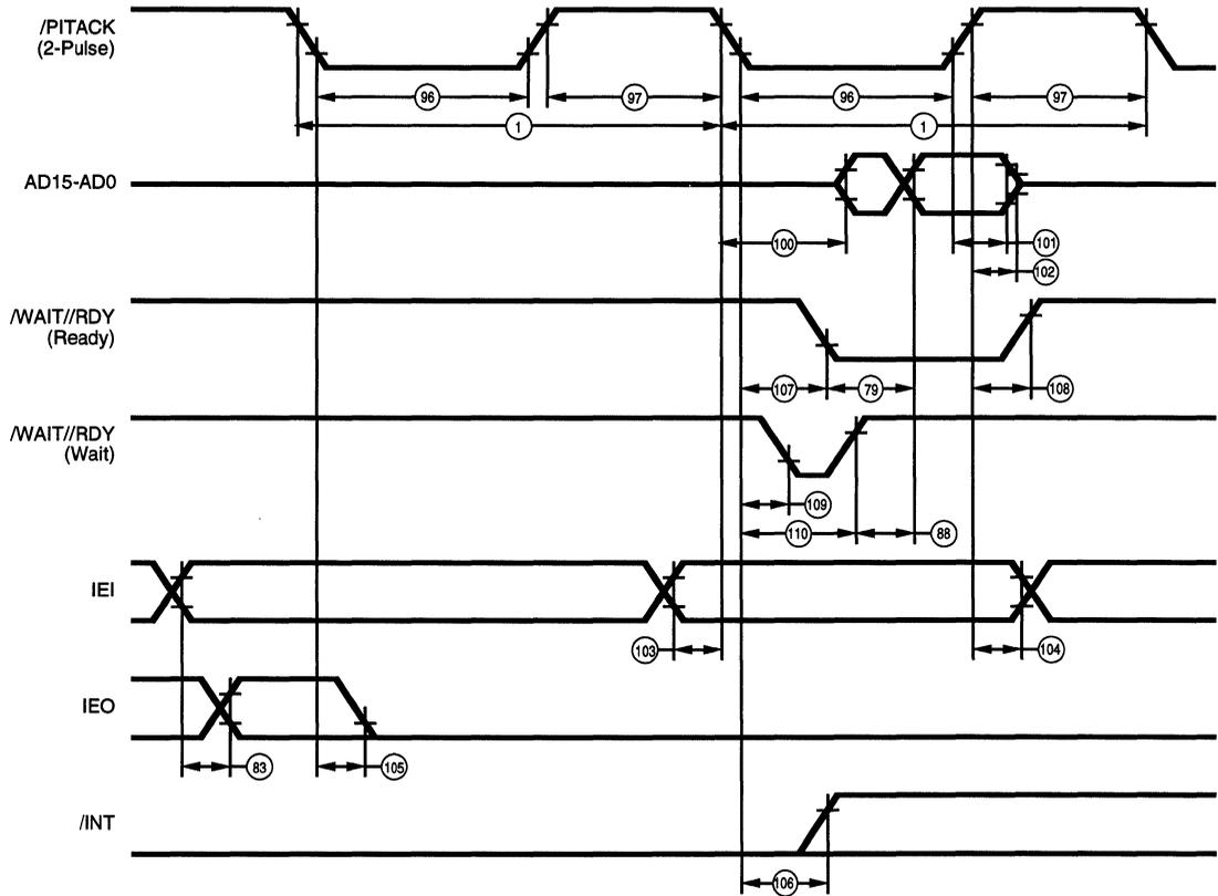
Figure 74. Non-Multiplexed Double-Pulse Intack Cycle
