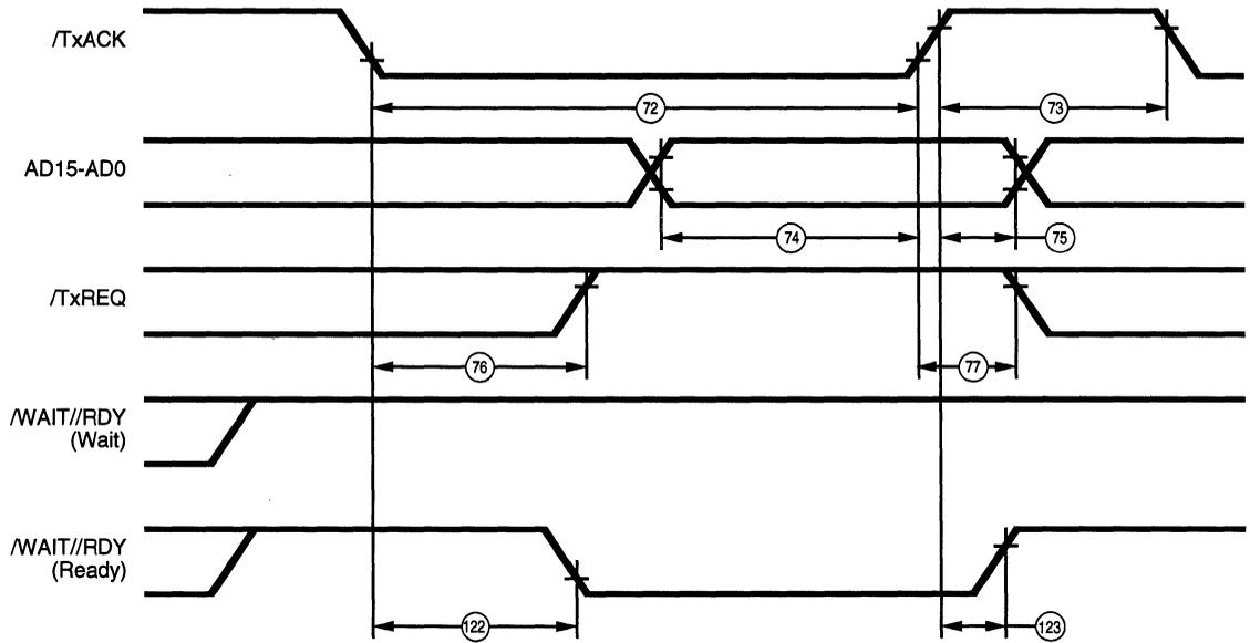
Figure 58. DMA Write Cycle
