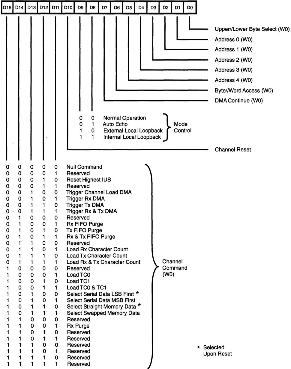
Figure 7. Channel Command/Address Register
