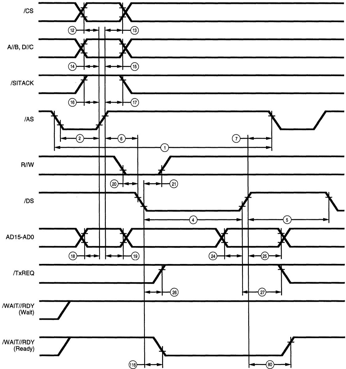
Figure 60. Multiplexed /DS Write Cycle
