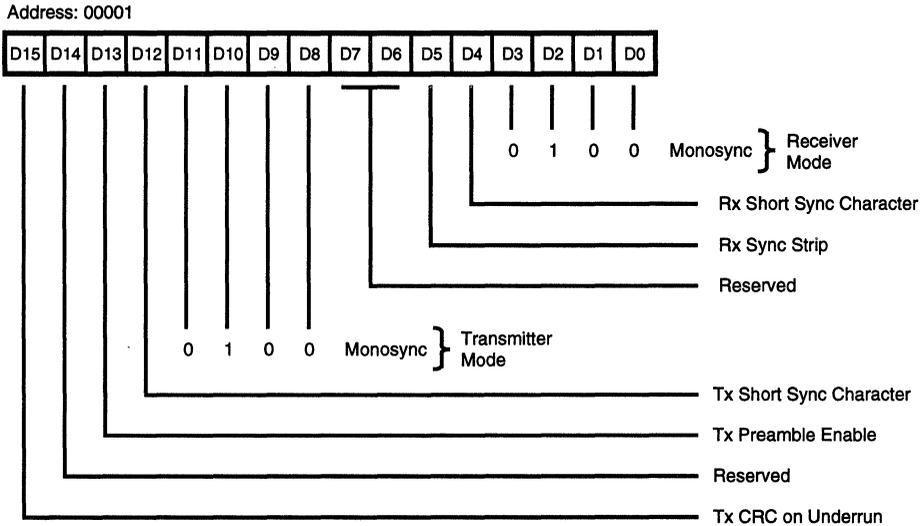
Figure 13. Channel Mode Register, Monosync Mode
