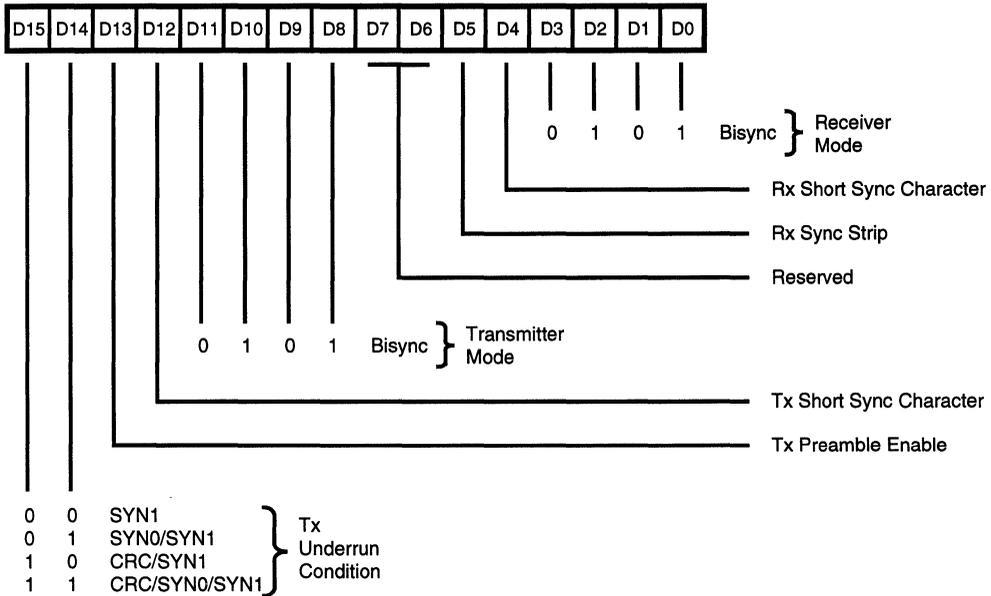
Figure 41. Channel Mode Register, Bisync Mode
