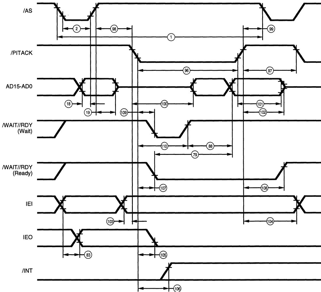
Figure 69. Multiplexed Pulsed Interrupt Acknowledge Cycle
