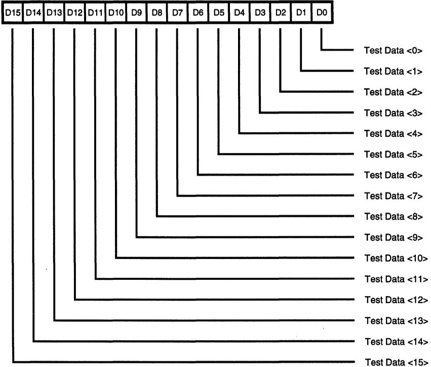
Figure 25. Test Mode Data Register
