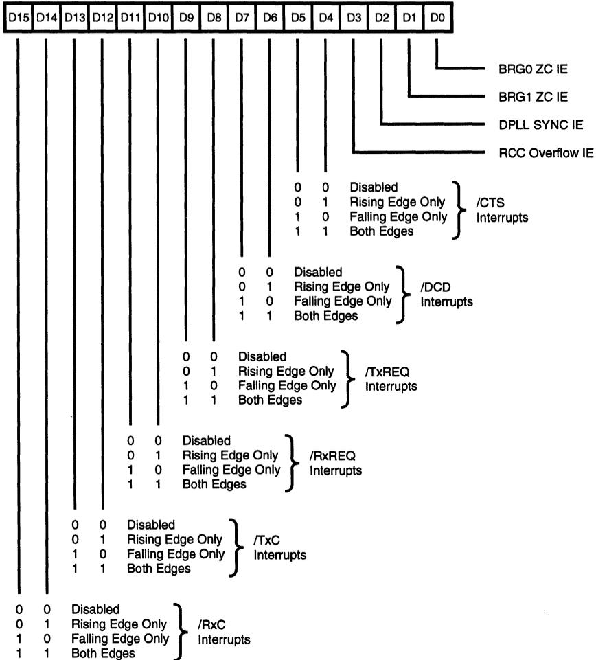
Figure 34. Status Interrupt Control Register
