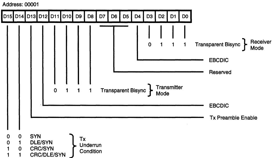
**Figure 43. Channel Mode Register, Transparent Bisync Mode**
