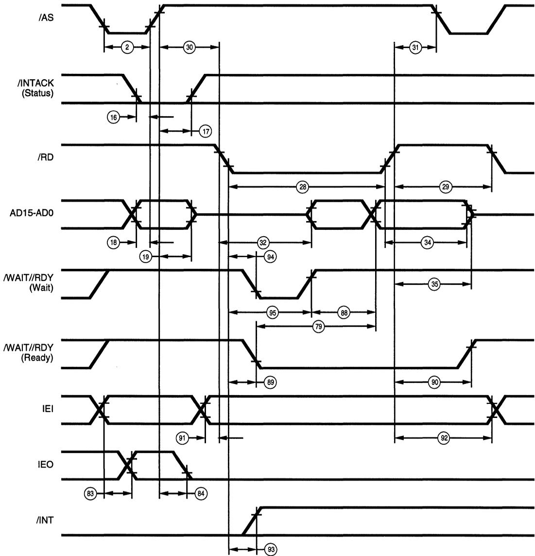
Figure 93. Multiplexed /RD Interrupt Acknowledge Cycle
