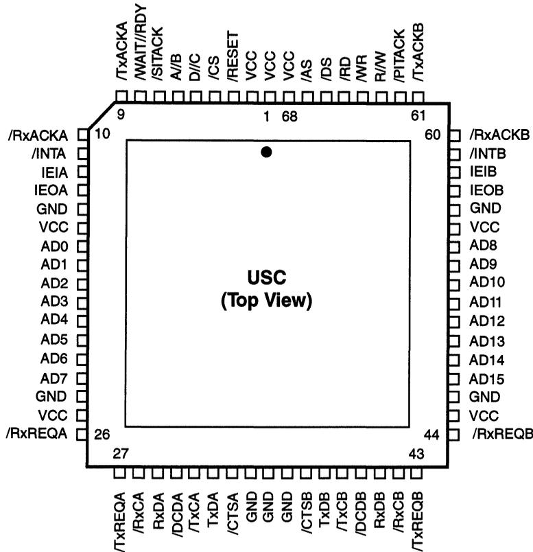
**Figure 3. Pin Assignments**
