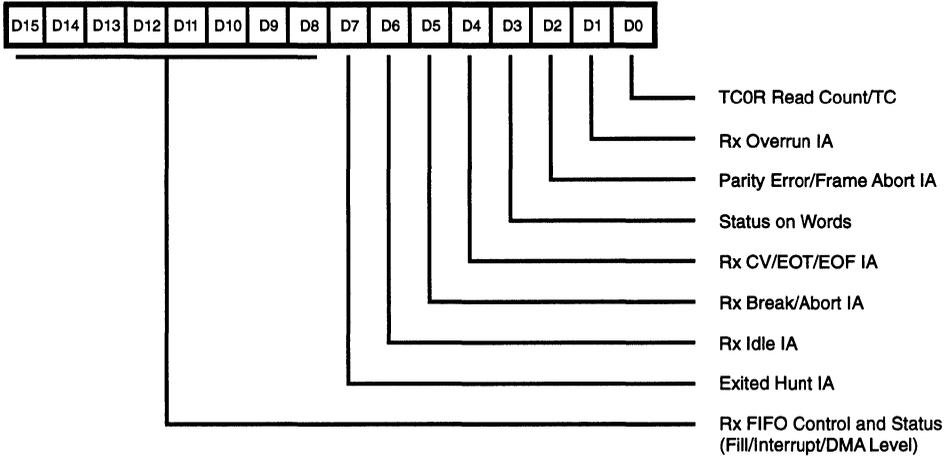
Figure 38. Receive Interrupt Control Register
