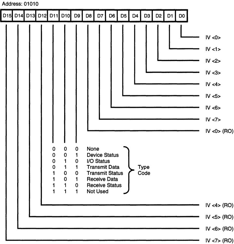
Figure 56. Interrupt Vector Register (IVR)
