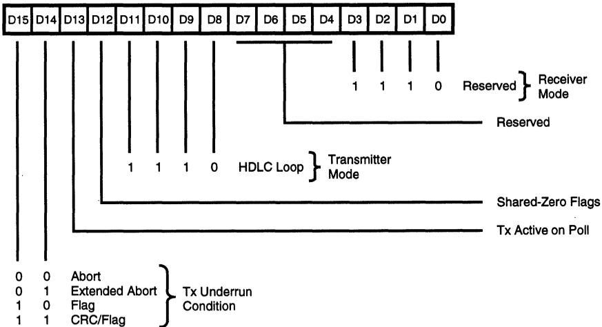
Figure 20. Channel Mode Register, HDLC Loop Mode
