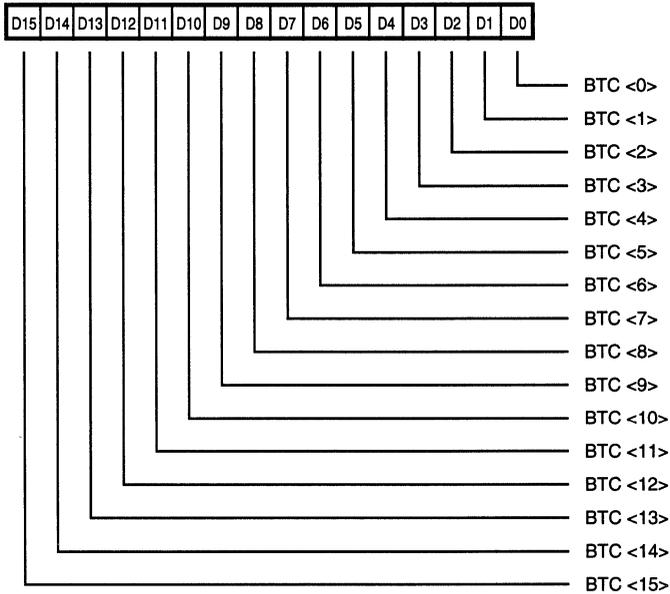
Figure 23. Next Tx/Rx Byte Counter Register (NTBCR)/(RTBCR)
