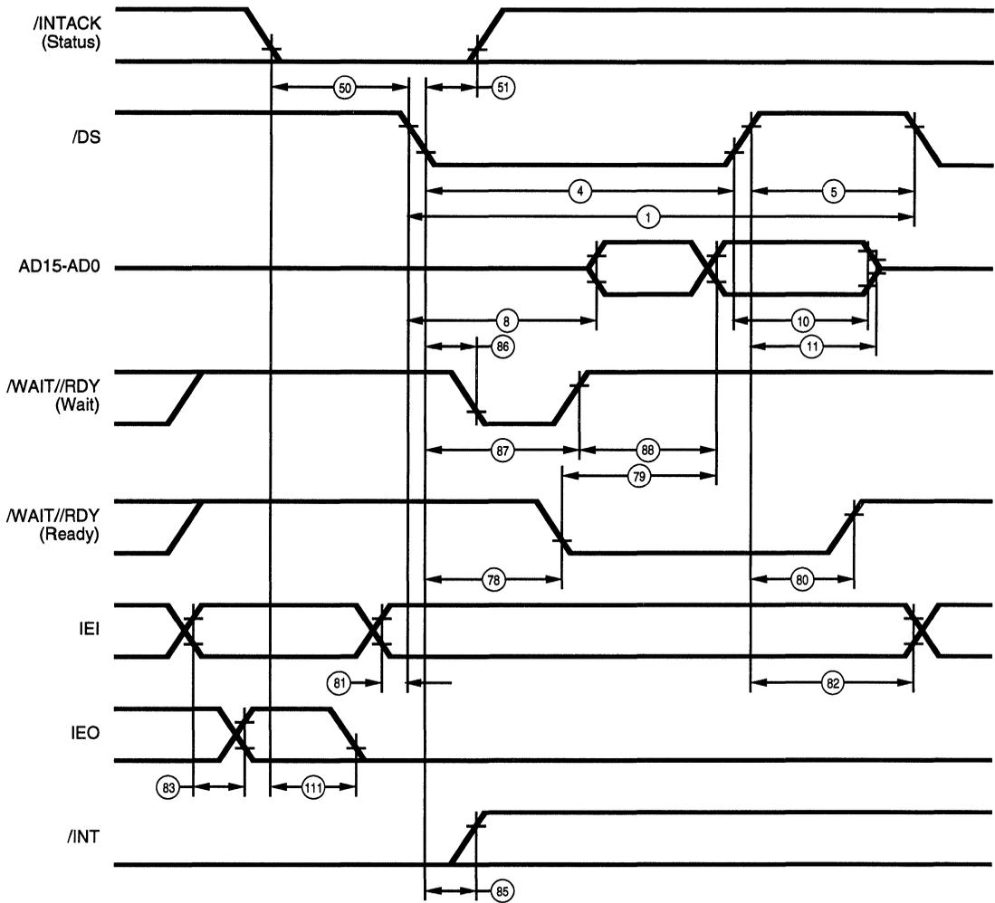
**Figure 95. Non-Multiplexed /DS Interrupt Acknowledge Cycle**
