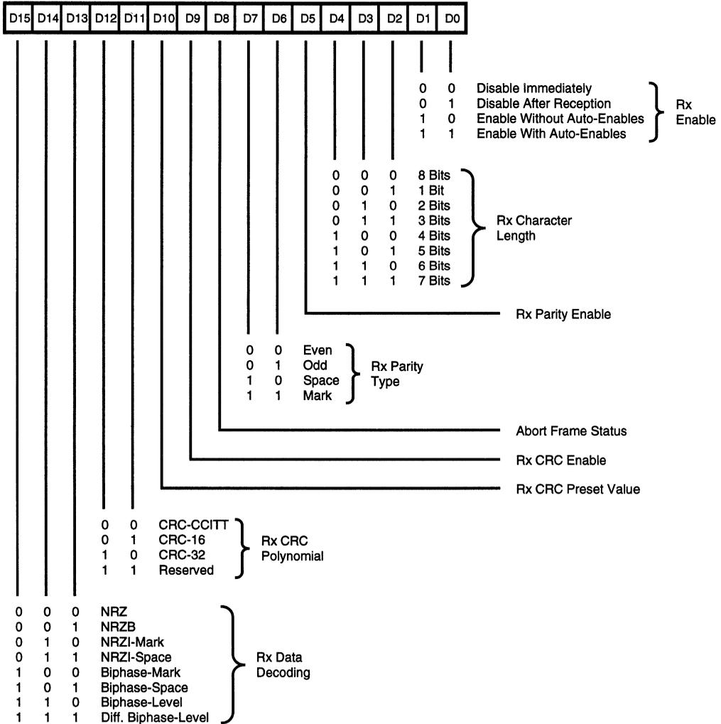
**Figure 63. Receive Mode Register (RMR)**
