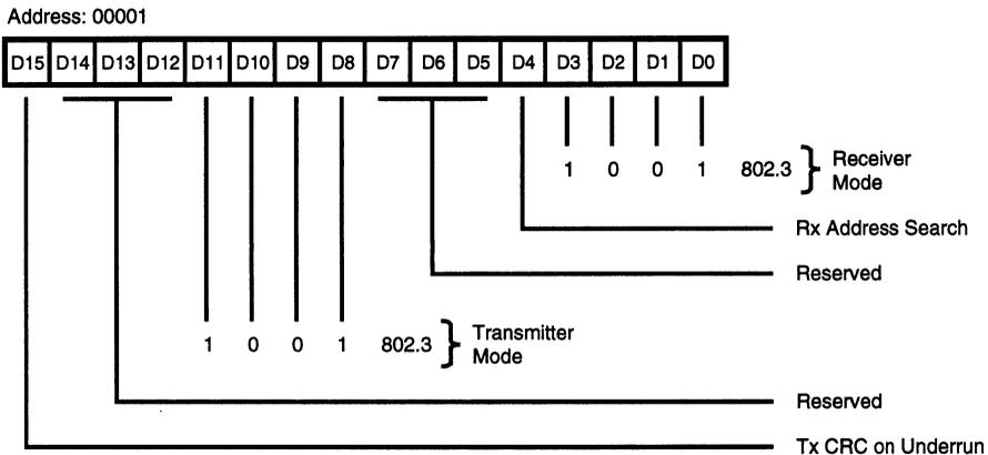
Figure 45. Channel Mode Register, 802.3 Mode
