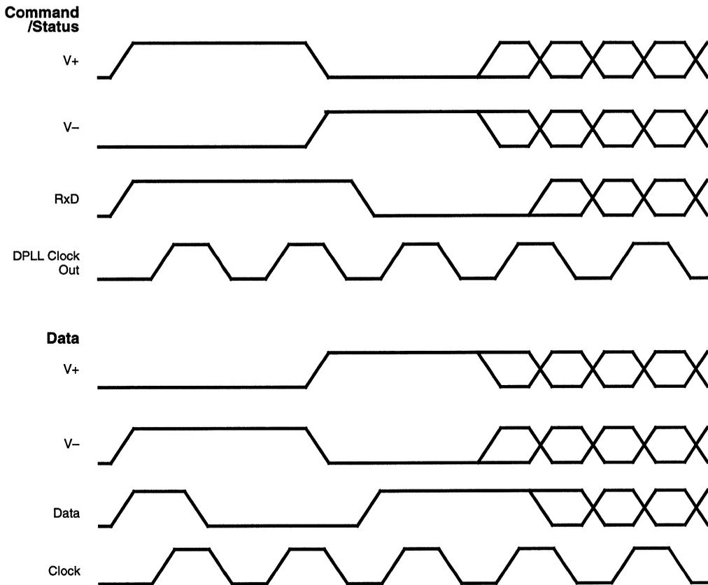
Figure 15. DPLL Idle Line Start-Up Requirements
