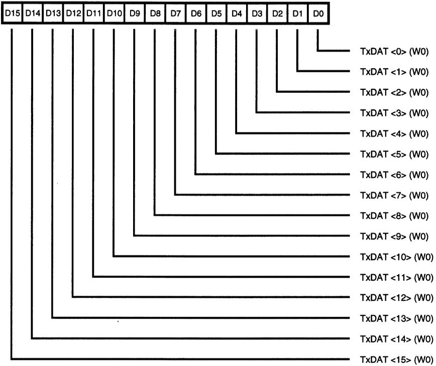
Figure 43. Transmit Data Register
