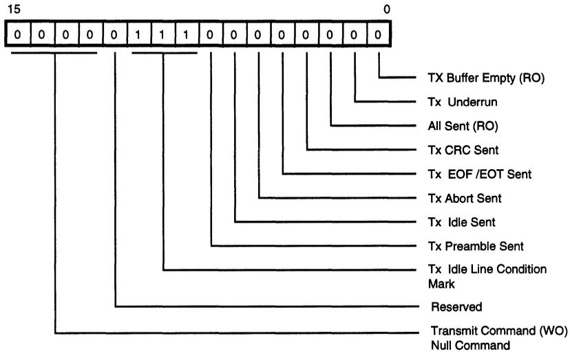
Figure 11. Transmit Command/Status Register
