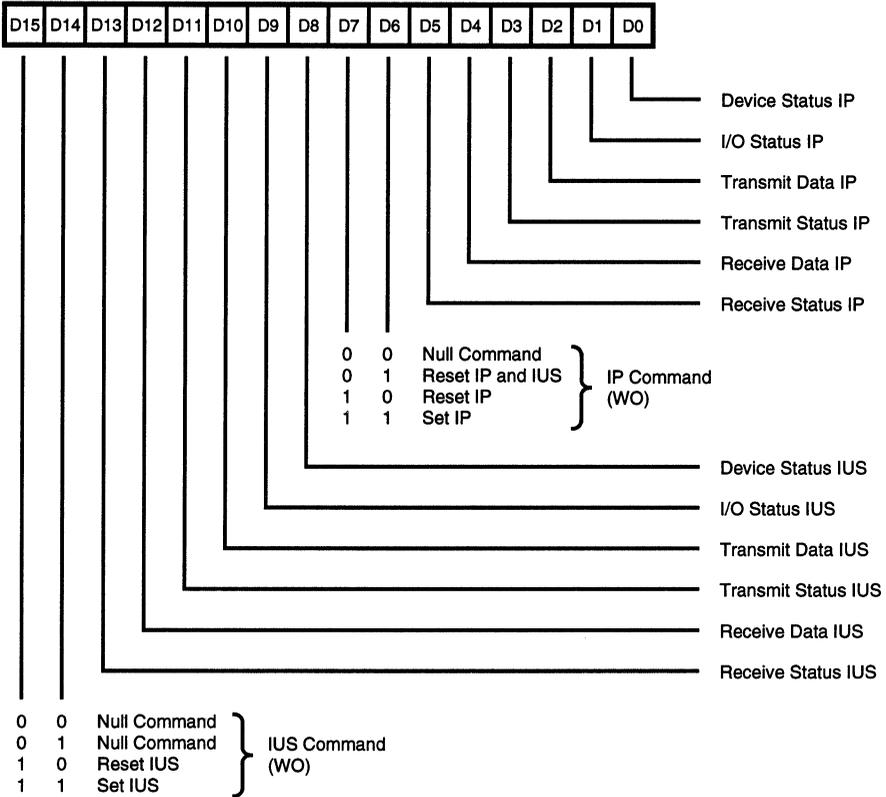
**Figure 59. Daisy-Chain Control Register (DCCR)**
