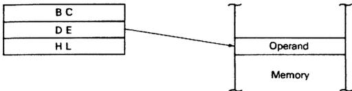
Figure 90. Register Indirect Addressing
