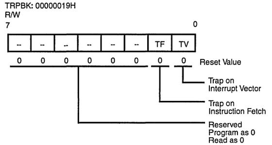
Figure 6-3. Trap and Break Register
