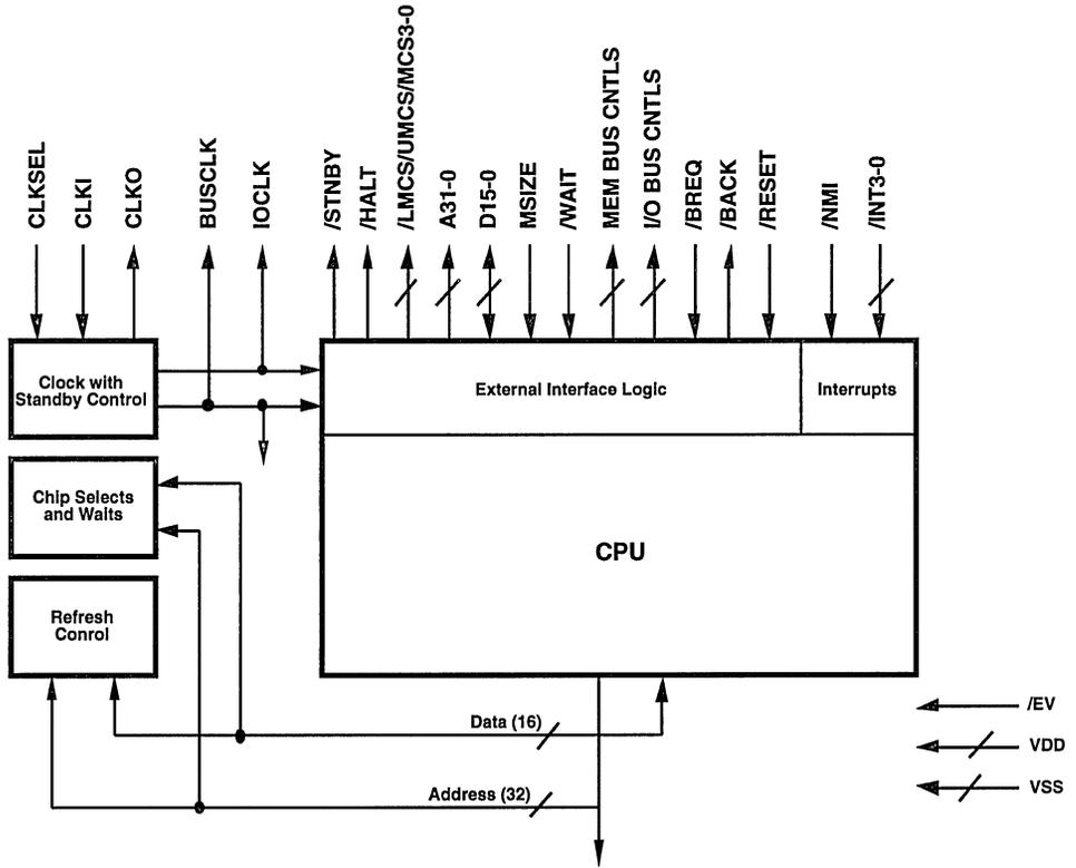
Figure 1. Z380 Functional Block Diagram
