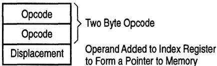
An example of an indexed instruction would be to load the contents of the memory location (Index Register + Displacement) into the accumulator. The displacement is a signed two's complement number. Indexed addressing greatly simplifies programs using tables of data since the index register can point to the start of any table. Two index registers are provided since very often operations require two or more tables. Indexed addressing also allows for relocatable code.
