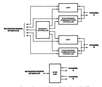
Figure 8. Conventional Devices Replaced by the Z-80 SIO
