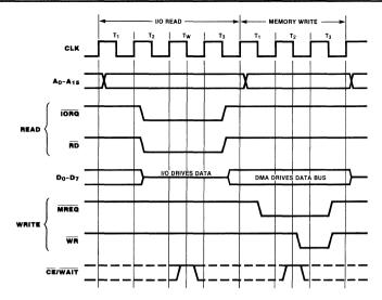
Figure 13. I/O-to-Memory Transfer
