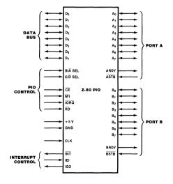
Figure 1. Pin Functions
