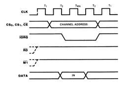
Figure 10. Write Cycle Timing
