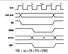
Figure 12. Write Cycle Timing
