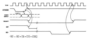
Figure 15. Mode 1 Input Timing
