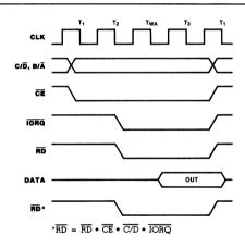
Figure 13. Read Cycle Timing
