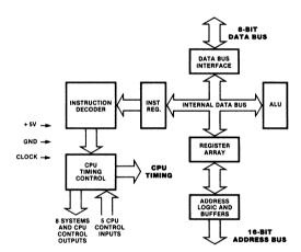
Figure 3. Z80L CPU Block Diagram
