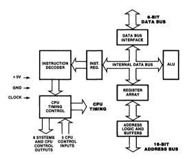
Figure 3. Z80 CPU Block Diagram
