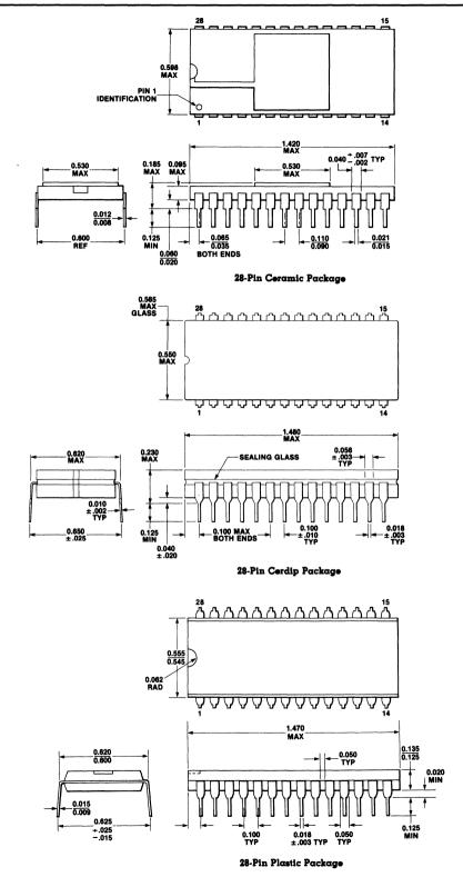
NOTE: Package dimensions are given in inches. To convert to millimeters, multiply by 25.4.
