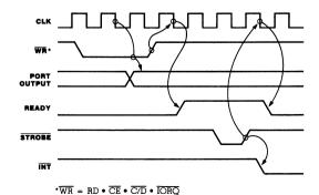
Figure 14. Mode 0 Output Timing
