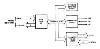
Figure 3. Functional Block Diagram
