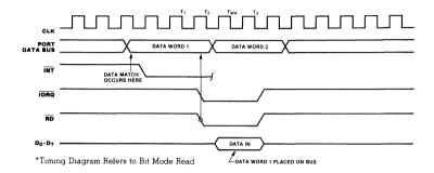
Figure 17. Mode 3 Bit Mode Timing
