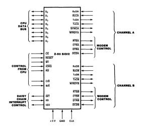
Figure 1. Z-80 SIO/2 Pin Functions
