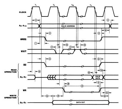
Figure 6. Memory Read or Write Cycles
