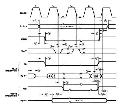
Figure 6. Memory Read or Write Cycles
