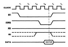
Figure 17. Interrupt Acknowledge Cycle
