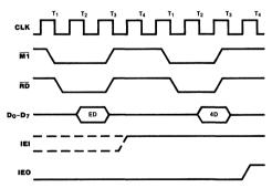
Figure 15. Return From Interrupt Timing
