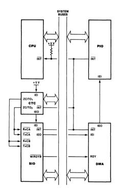
Figure 3. PIO in a Typical Z80 Family Environment
