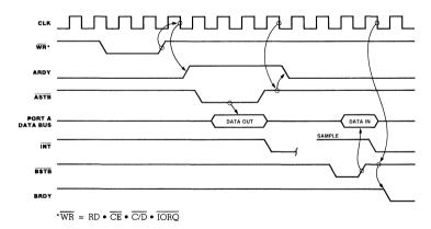
Figure 16. Mode 2 Bidirectional Timing
