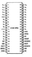
Figure 2. Pin Assignments
