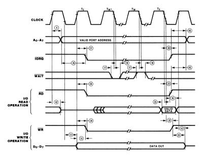
NOTE  $T_{\mathbf{W}^{\star}} = \text{One Wait cycle automatically inserted by CPU}$
