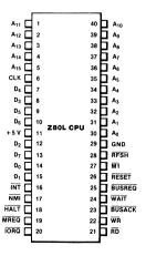
Figure 2. Pin Assignments
