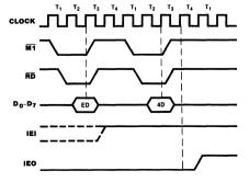
Figure 18. Return from Interrupt Cycle
