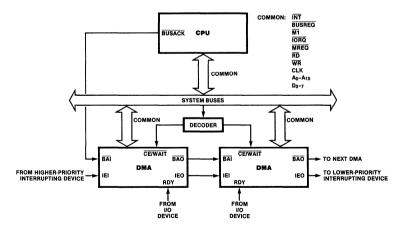
Figure 7. Multiple-DMA Interconnection to the Z-80 CPU
