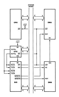
During a search-only operation, data is read from the source port and compared byte by byte with a DMA-internal register containing a programmable match byte. This match byte may optionally be masked so that only certain bits within the match byte are compared. Search rates up to 1.25M bytes per second can be obtained with the 2.5 MHz Z-80 DMA or 2M bytes per second with the 4 MHz Z-80A DMA.
