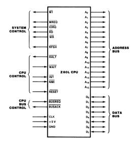
Figure 1. Pin Functions
