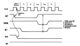
Figure 18. Interrupt Acknowledge Timing
