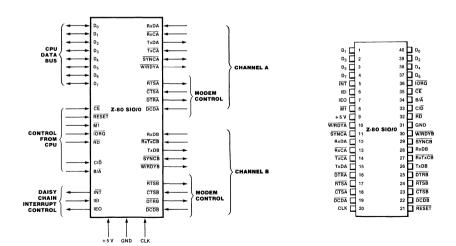
Figure 5. Z-80 SIO/0 Pin Functions
