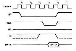
Figure 5c. Interrupt Acknowledge Cycle
