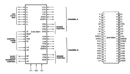
Figure 3. Z-80 SIO/1 Pin Functions
