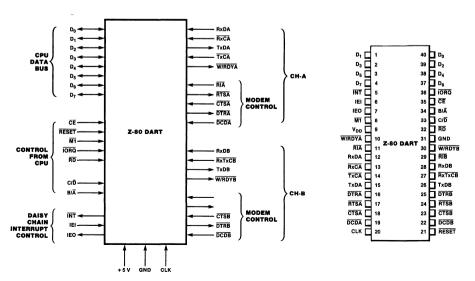
Figure 1. Z80 DART Pin Functions
