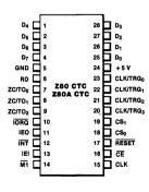
Figure 2. Pin Assignments
