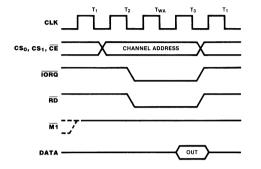
Figure 9. Read Cycle Timing
