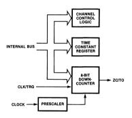
Figure 4. Counter/Timer Block Diagram
