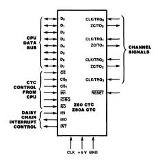
Figure 1. Pin Functions
