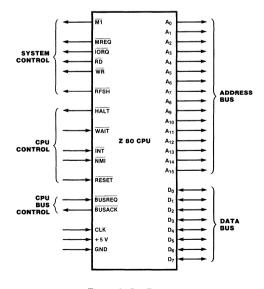
Figure 1. Pin Functions
