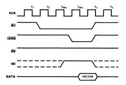
Figure 14. Interrupt Acknowledge Timing
