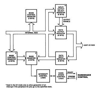
Figure 5. Typical Port I/O Block Diagram
