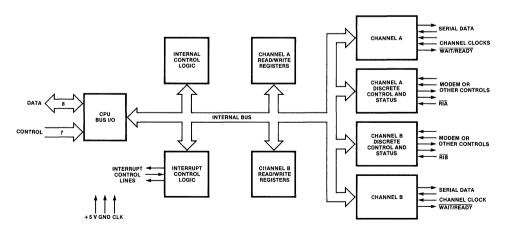
Figure 3. Block Diagram
