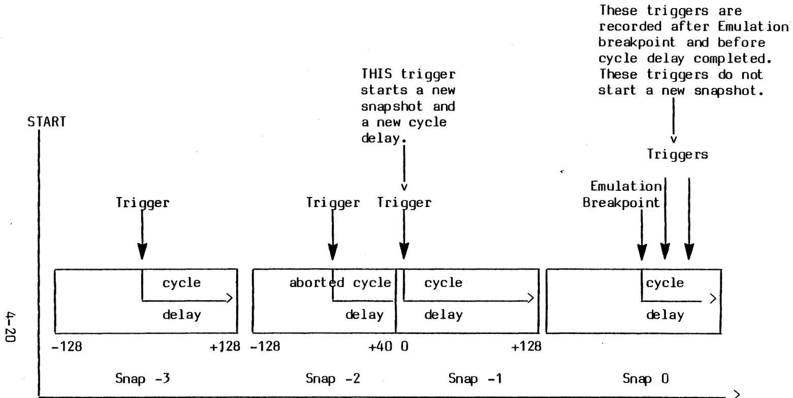
Figure 4-5. Triggers Occurring During the LAST Cycle Delay
