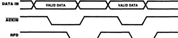
Figure 4. Two-Wire Interlocked Handshake Timing (Input)
