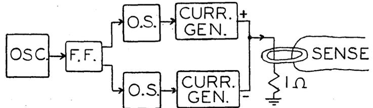
The amplitude of the current is monitored across the one-ohm resistor with an oscilloscope.
