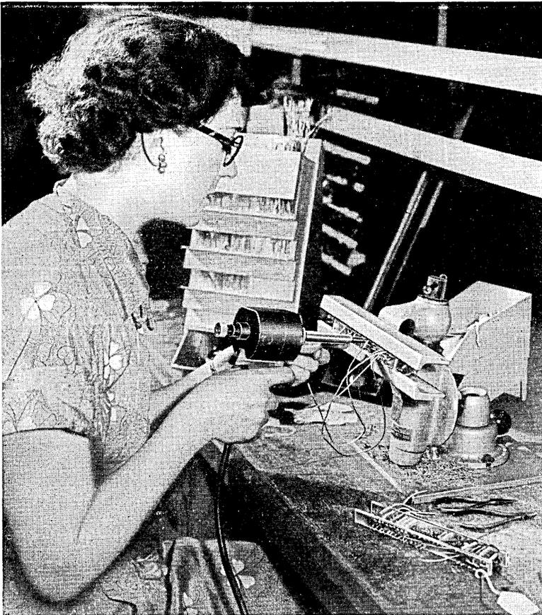
Fig. 12—Operator using electrically operated wire wrapping pistol. All wires are precut to suitable length.
