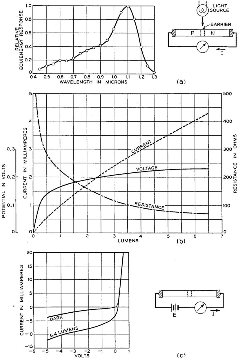
Fig. 2a—Spectral response of internal barrier in silicon.
