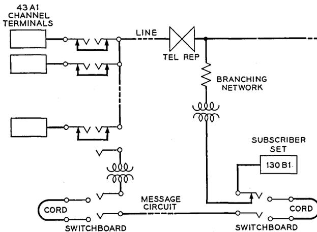
Fig. 16—Emergency circuit for intermediate branch.
