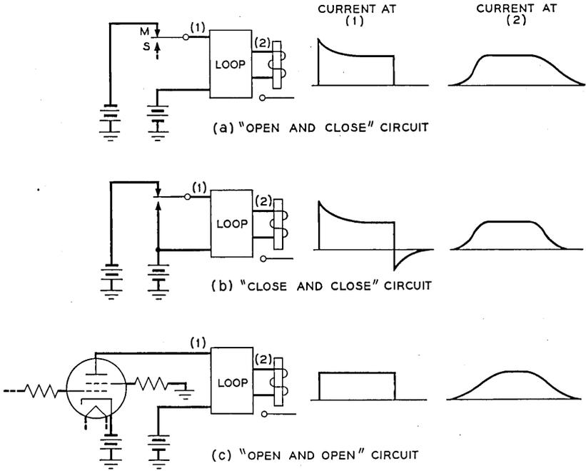
Fig. 5—Explanation of electronic loop circuit.
