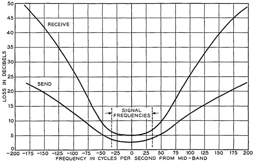
Fig. 3—Send and receive filter characteristics, VF allocation.
