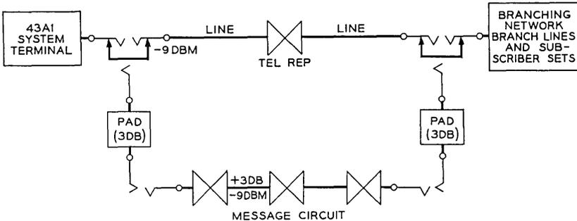
Fig. 15—Emergency circuit.
