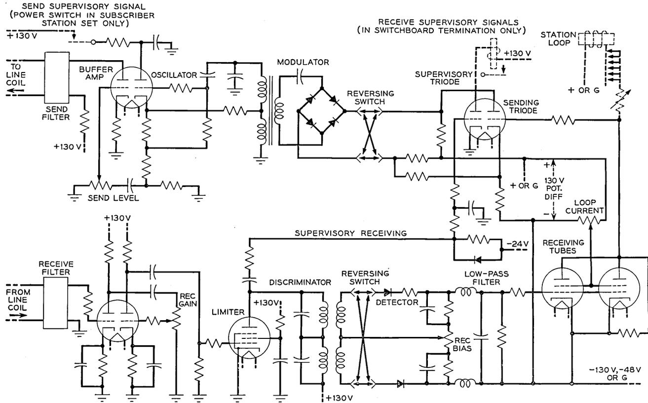
Fig. 2—Simplified diagram of channel terminal circuit, half-duplex.
