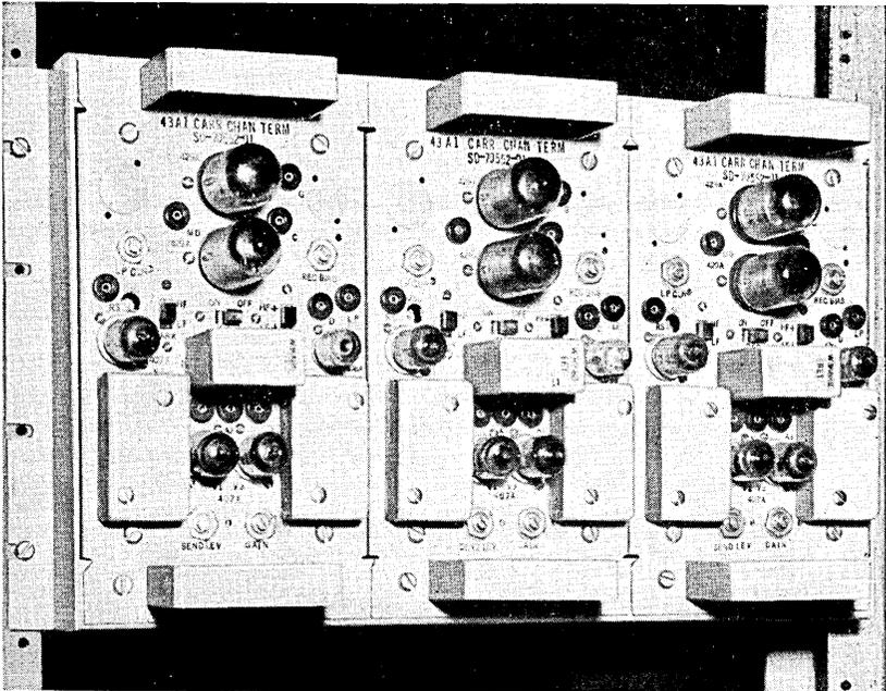
Fig. 9—Three channel terminals mounted on relay rack.
