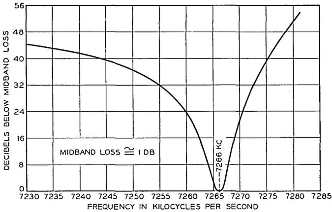
Fig. 26 — Loss characteristic of the 7266 kc crystal filter.
