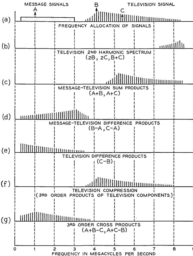
Fig. 8. — L3 coaxial system. Critical modulation products in combined message-television application.
