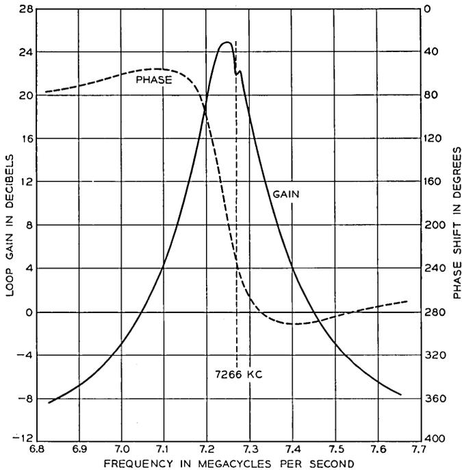
Fig. 24 — Loop gain and phase of the 7266 ke pilot amplifier.
