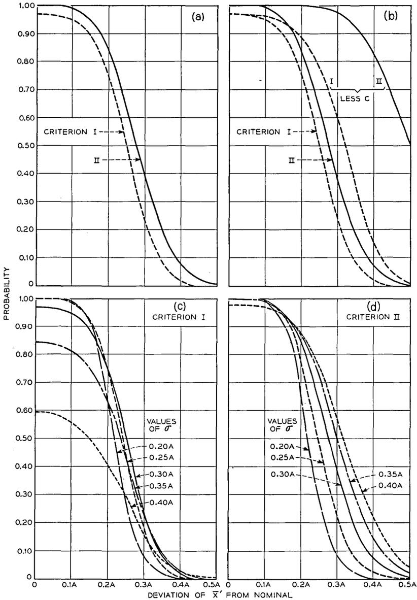
Fig. 7 — Operating characteristic curves for control chart method.
