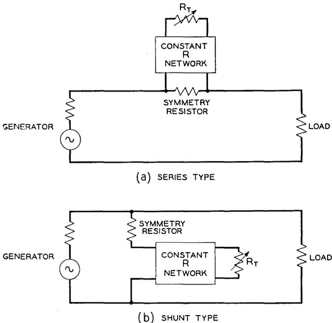
Fig. 5 — Block diagram of Bode Regulating Network.
