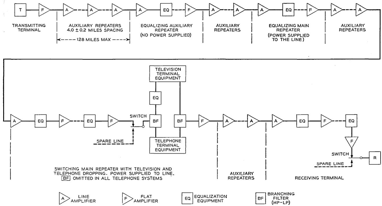
Fig. 14 — General layout of L3 repeaters.
