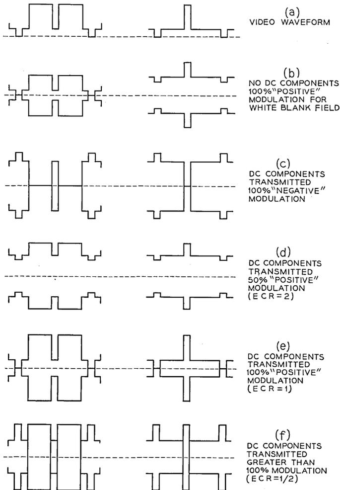
Fig. 9 — Typical television signals. Alternative carrier frequency waveforms.
