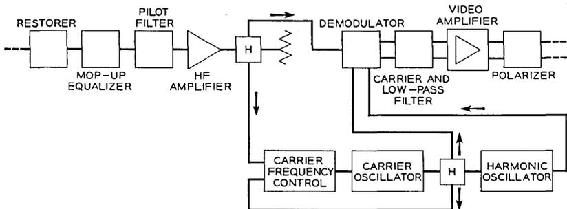
Fig. 19 — L3 receiving terminal block diagram.
