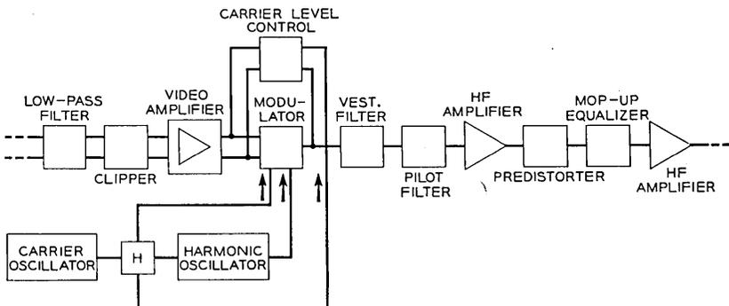
Fig. 18 — L3 transmitting terminal block diagram.
