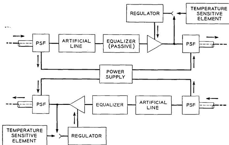
Fig. 15 — Auxiliary repeater.
