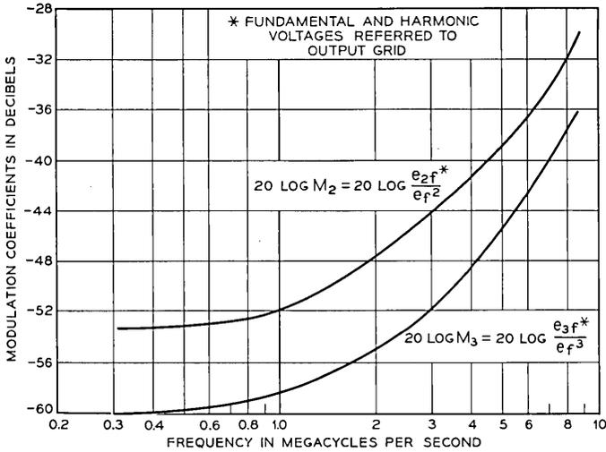
Fig. 6 —L3 amplifier modulation coefficients.
