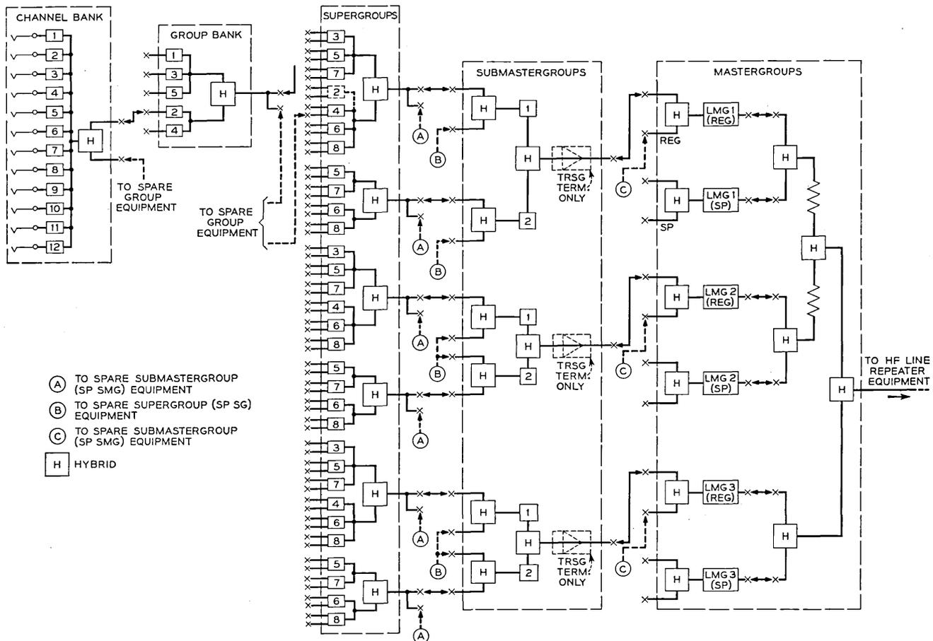
Fig. 19 — Terminal transmission equipment for an all-message system.
