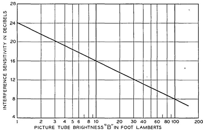
Fig. 10 — Picture tube interference sensitivity assumed for L3.
