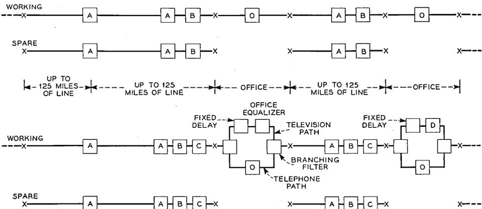
Fig. 1 — Typical equalizer locations in (a) telephone and (b) combined systems.
