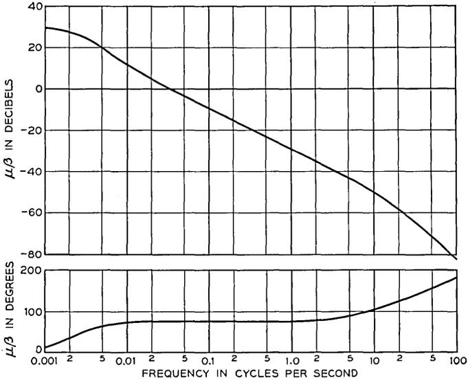
Fig. 21 — Loop gain characteristic for office regulators.
