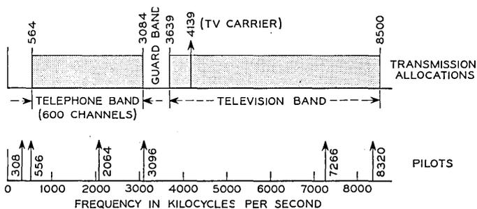
Fig. 1 — Frequency allocations for L3 combined television-telephone transmission.
