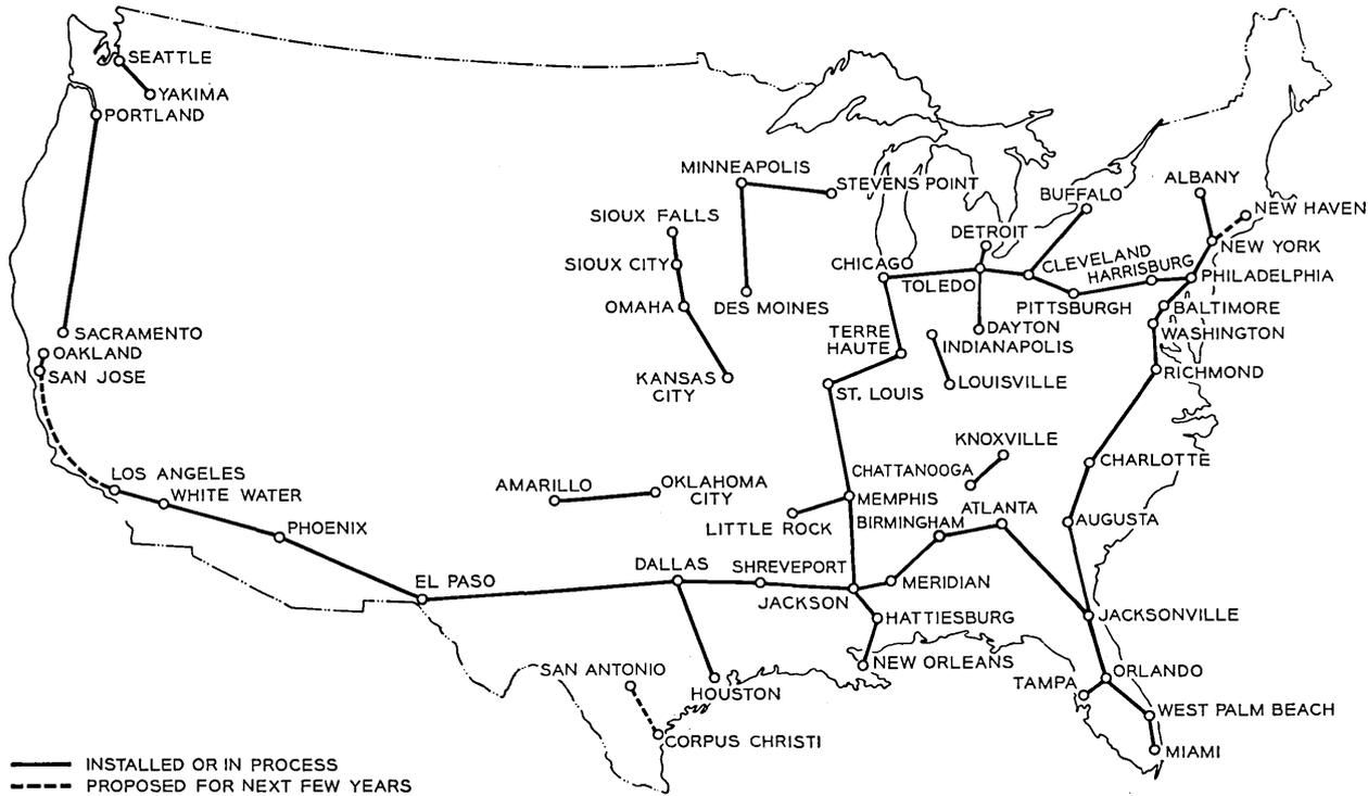
Fig. 1 — Coaxial cable routes.
