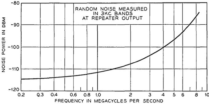
Fig. 5 — L3 Auxiliary repeater noise characteristic.
