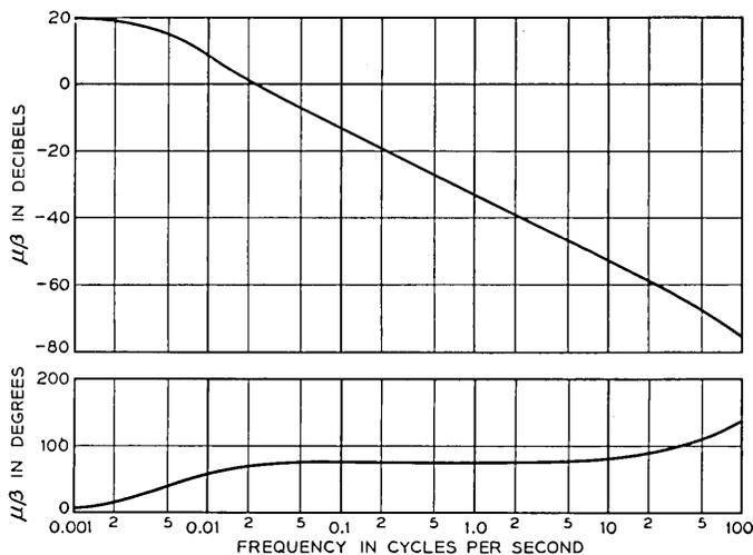
Fig. 19 — Loop gain characteristic for the line regulator.
