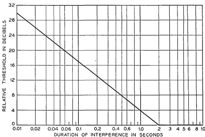
Fig. 3 — Television bar pattern threshold versus duration.
