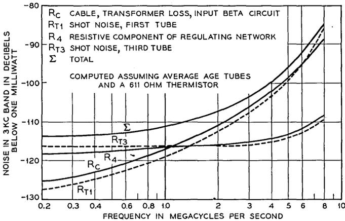
Fig. 19 — Thermal noise at line amplifier output.
