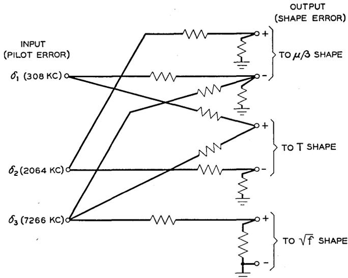
Fig. 2 — Schematic of regulation system computer.
