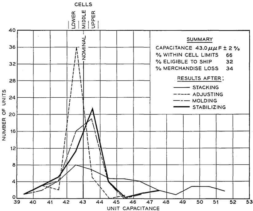
Fig. 9 — A summarized frequency distribution of a 43-mm mica condenser at various stages of manufacture.
