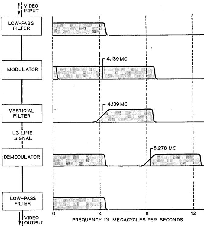
Fig. 2 — Television terminal modulation processes.
