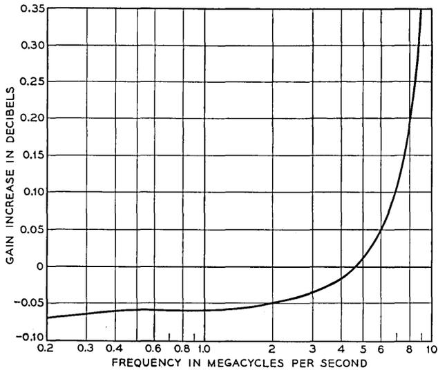
Fig. 17 — Mu beta effect, amplifier gain change for a one db decrease in each transconductance.
