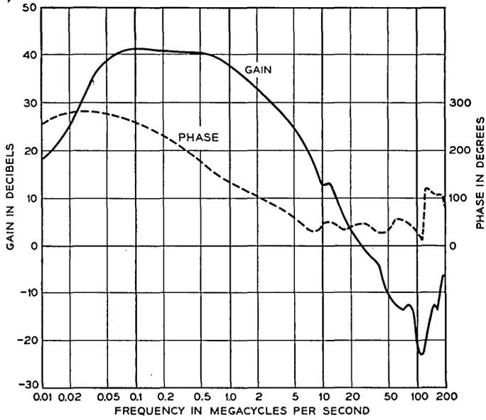
Fig. 16 — T4, return ratio of lower triode.
