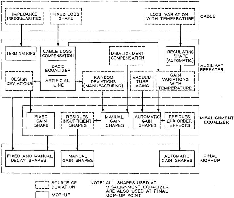
Fig. 13 — L3 coaxial system, equalization plan.
