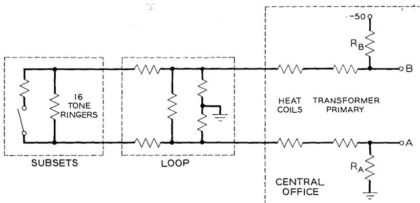
Fig. 7 — Dc circuit for a long customer loop.
