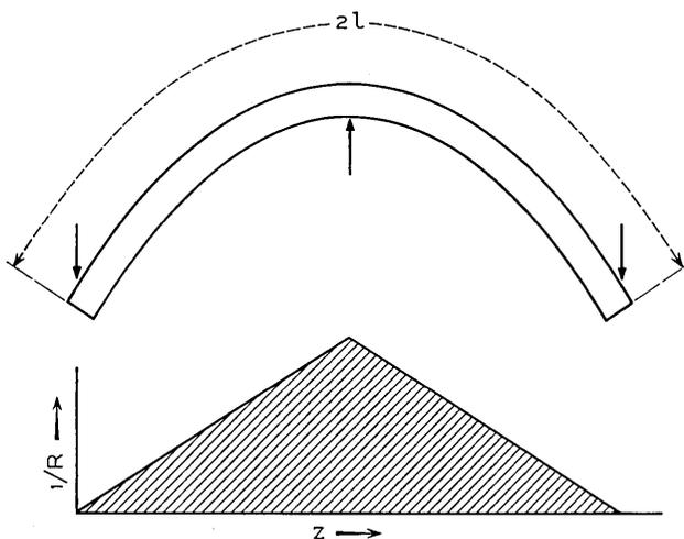
Fig. 8 — Triangular curvature distribution of an elastic deflection.
