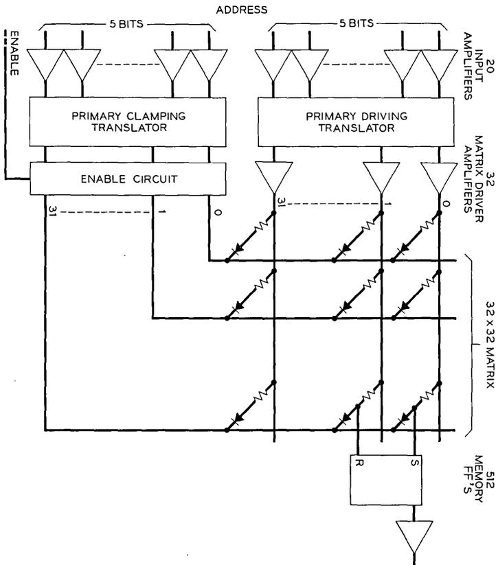
Fig. 3 — Block diagram of the signal distributor.
