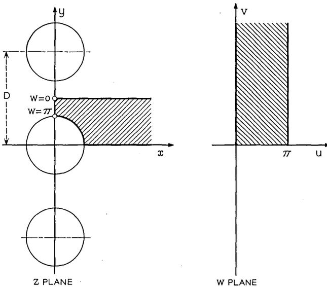
Fig. 19 — Conformal mapping of wire grating.
