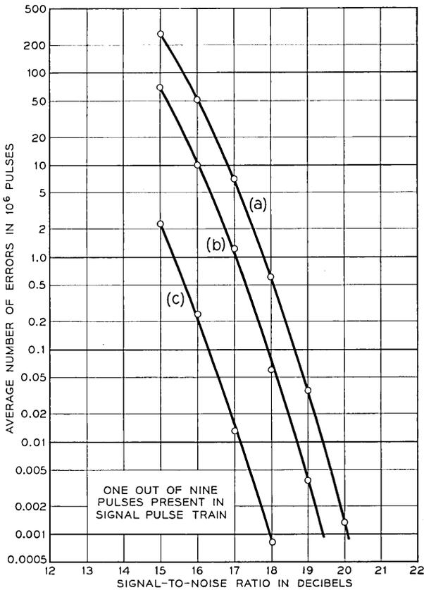
Fig. 2 — Average pulse error rate with linear timing amplifier: (a) self-timed, noise into both slicing and timing paths; (b) externally timed, noise into slicing path only; (c) self-timed, noise into timing path only.
