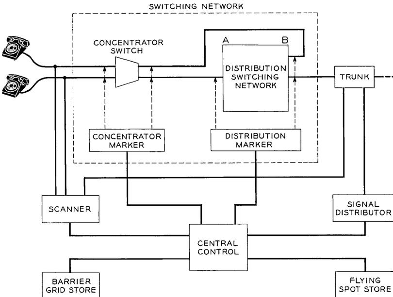
Fig. 1 — Block diagram of experimental electronic switching system.
