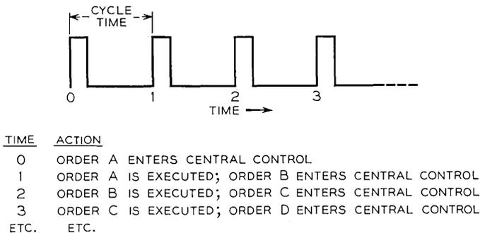
Fig. 9 — Electronic switching system clock timing.
