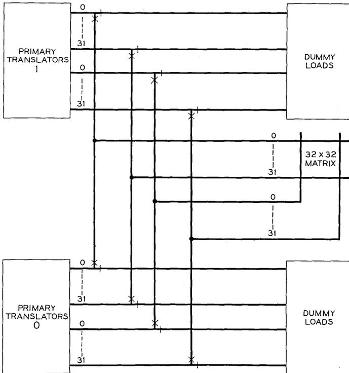
Fig. 7 — Transfer circuit.
