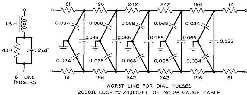
Fig. 9 — Circuits to simulate loop and tone ringers.
