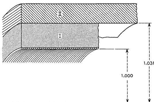
Fig. 12 — Shielded helix waveguide with low loss jacket. Helix: No. 37 copper wire with heavy Formex coat; Medium I: glass cloth laminated with epoxy resin,  $\epsilon/\epsilon_0 = 4 - j0.1$  at 55.5 kmc; Medium II: copper tubing.
