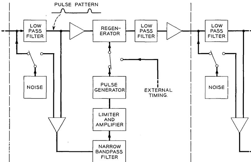
Fig. 1 — Block diagram of the baseband repeater.
