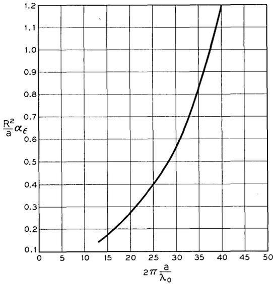
Fig. 6 — Curvature attenuation of the TE<sub>01</sub> mode, with  $\epsilon' = 3$ ,  $\epsilon'' = 0.03$ ;  $(b - a)/a = 0.025$ .
