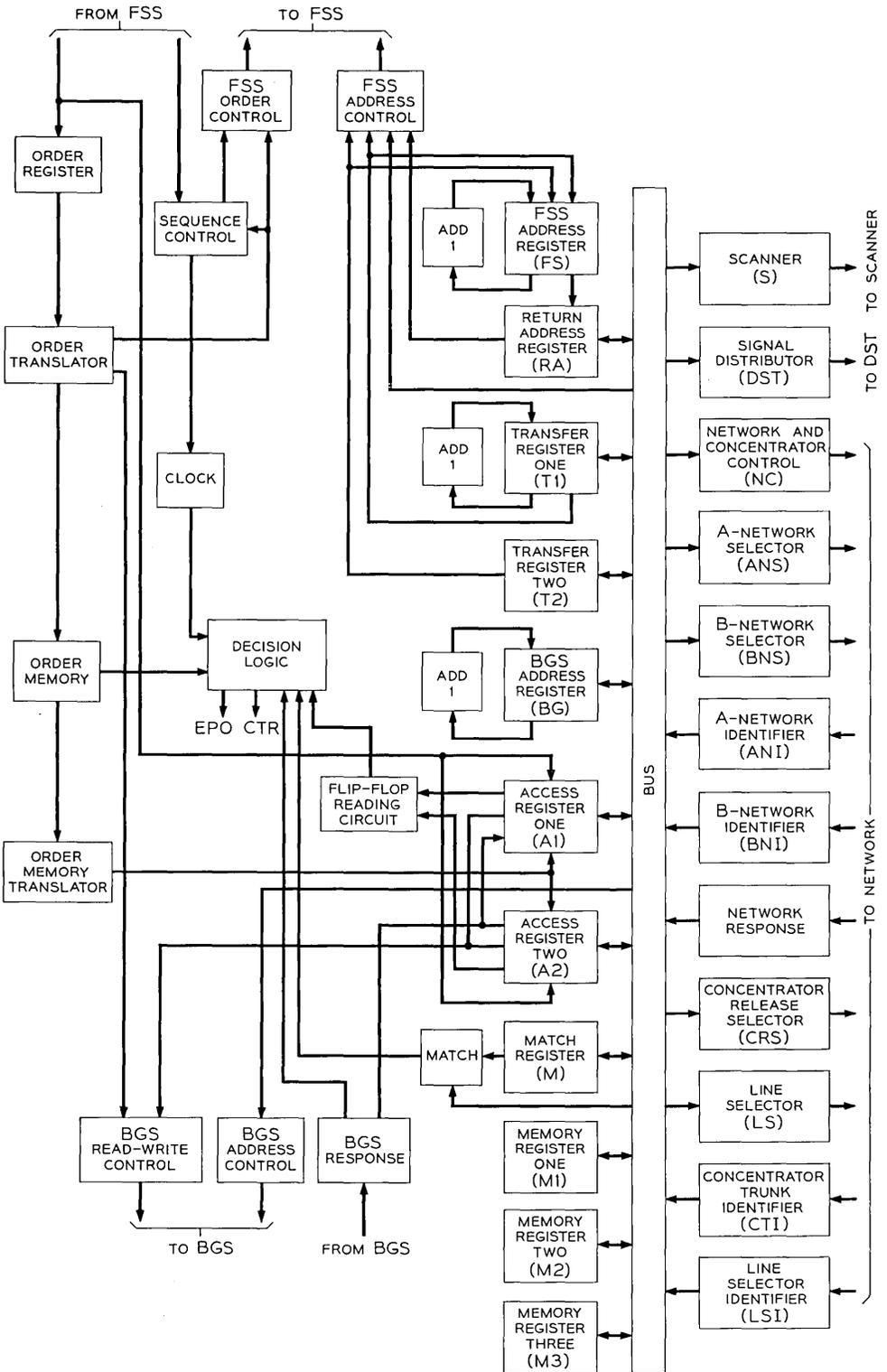
Fig. 17 — Functional block diagram of central control.
