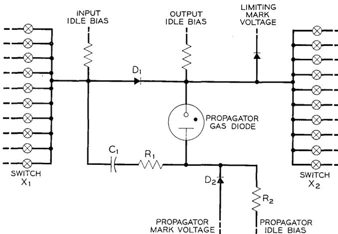
Fig. 3 — Active mark propagator circuit.
