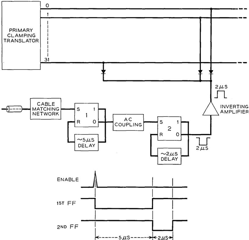
Fig. 5 — Enable circuit.
