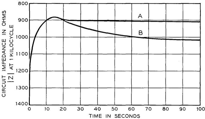
Fig. 8 — Starting circuit impedance transient due to the thermal properties of the Al624 negative-resistance characteristic: (a) air flow of 500 feet per minute across tubes; (b) tubes in stagnant air.
