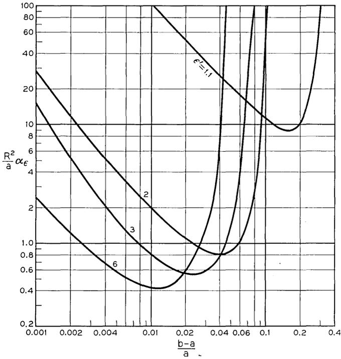
Fig. 5 — Curvature attenuation of the TE<sub>01</sub> mode, with  $\epsilon''/\epsilon' = 0.01$ .
