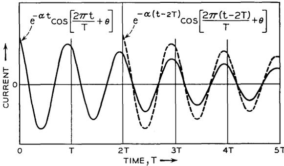
Fig. 5 — Response of tuned circuit to synchronous impulses.
