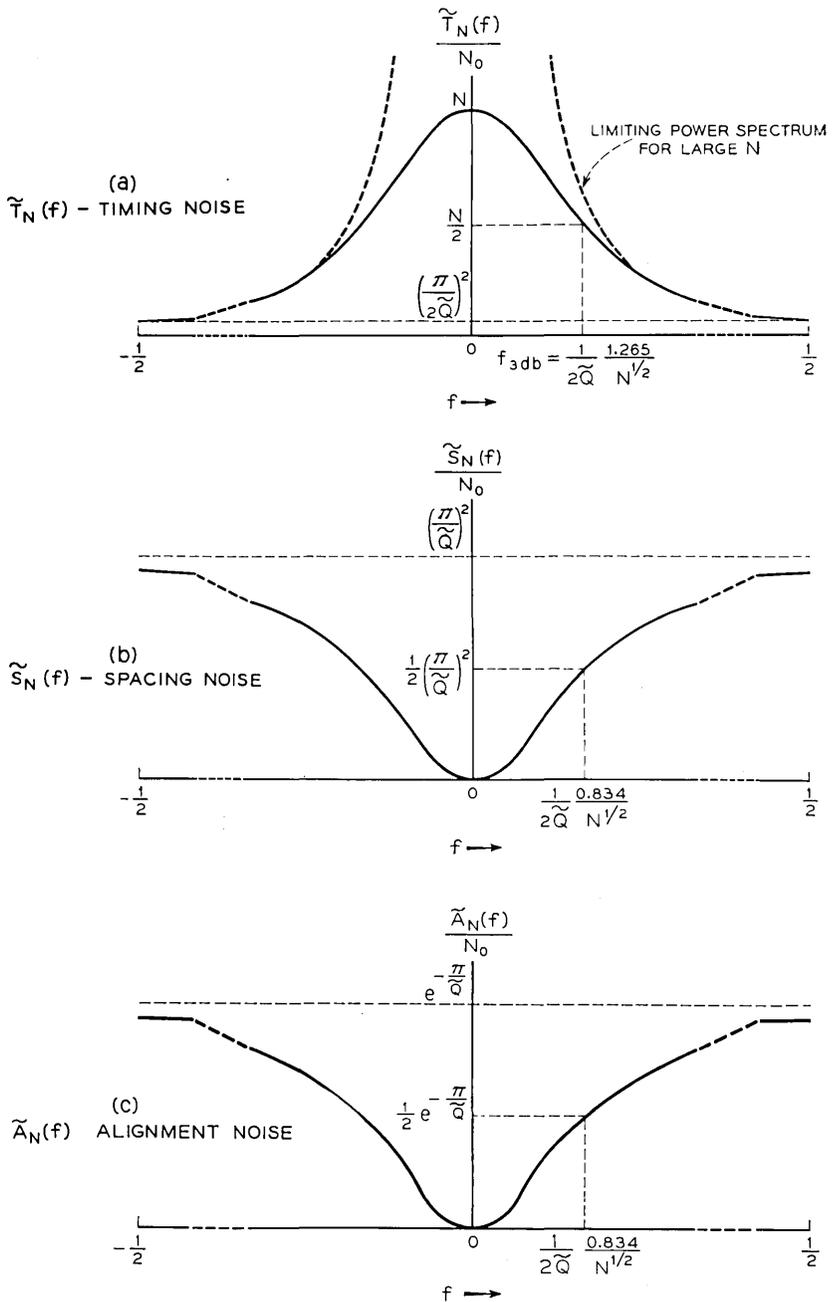
Fig. 9 — Timing (a), spacing (b) and alignment (c) noise power spectra for a chain of  $N$  repeaters with zero tuning error and complete retiming, with a white timing noise of power  $N_0$  added at the input of each repeater;  $Q \gg 1$ ,  $N \gg 1$ .
