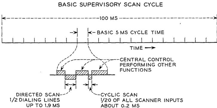
Fig. 6 — Time relations in scanner operation.
