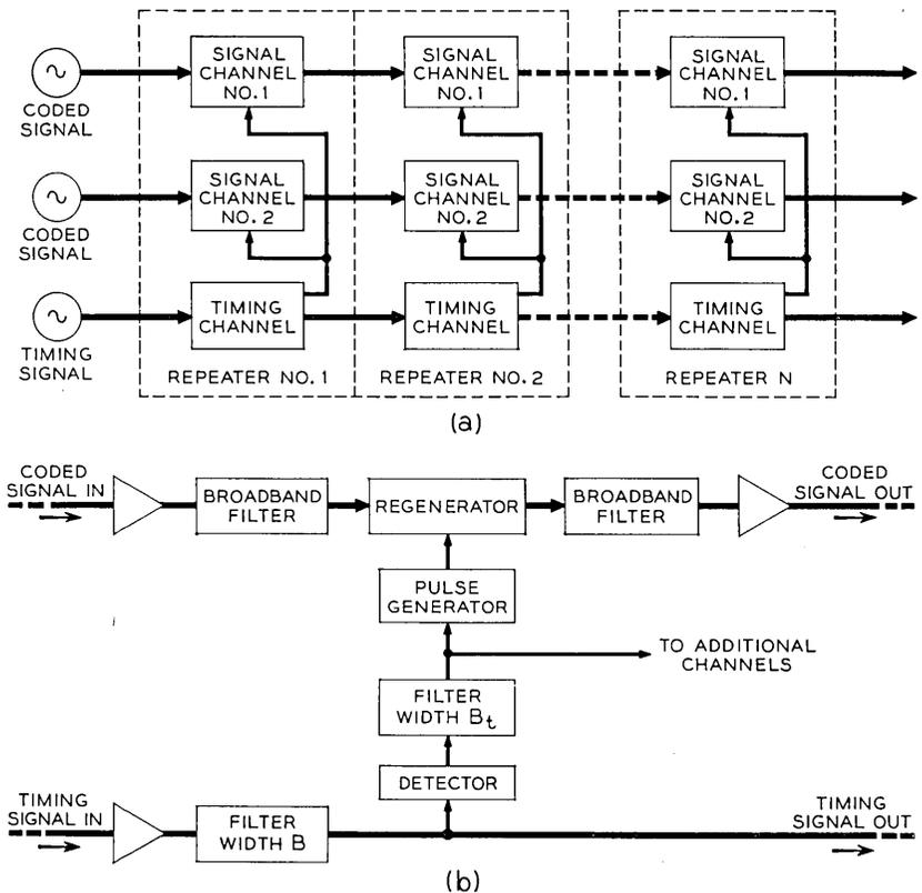
Fig. 2 — (a) Externally timed system with one timing channel supplying two signal channels; (b) single repeater—straight-through timing channel.
