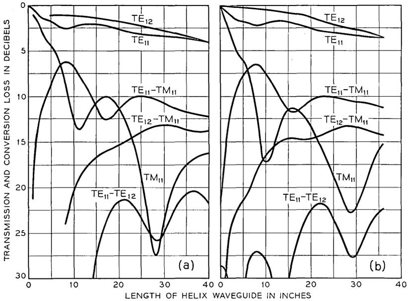
Fig. 5 — (a) Calculated transmission and conversion loss in helix waveguide:  $a/\lambda = 4.70$ , semi-infinite jacket with  $\epsilon/\epsilon_0 = 4 - j1$ ; (b) measured transmission and conversion loss in helix waveguide of Fig. 6,  $f = 55.5$  kmc.
