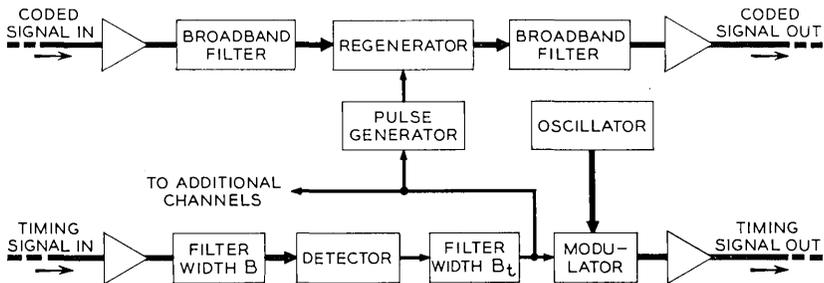
Fig. 3 — Single repeater—remodulation timing channel.
