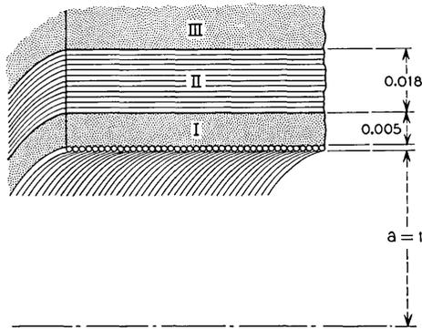
Fig. 6 — Helix waveguide structure. Helix: No. 37 copper wire with heavy Formex coat; Mediums I and III: Fibreglas laminated with epoxy resin; Medium II: six layers of tin oxide-coated glass cloth;  $\epsilon_z/\epsilon_0 = 9 - j13$ ,  $\epsilon_r/\epsilon_0 = 5 - j1$  at 55.5 kmc.
