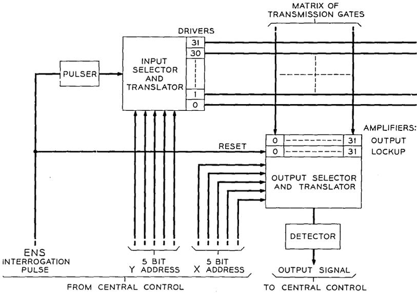
Fig. 4 — Block diagram of the scanner.
