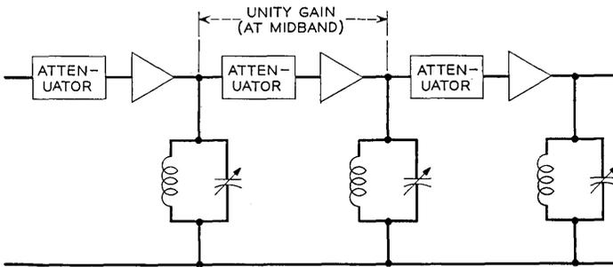
Fig. 11 — Simple tuned circuits in tandem.
