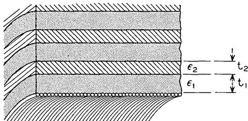
Fig. 2 — Laminated jacket of helix waveguide.
