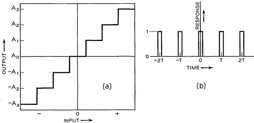
Fig. 1 — Specification of ideal regenerative repeater characteristic.
