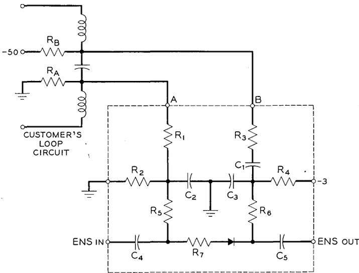
Fig. 12 — Balanced transmission gate for customer loops.
