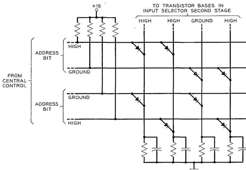
Fig. 14 — Portion of input selector translator.
