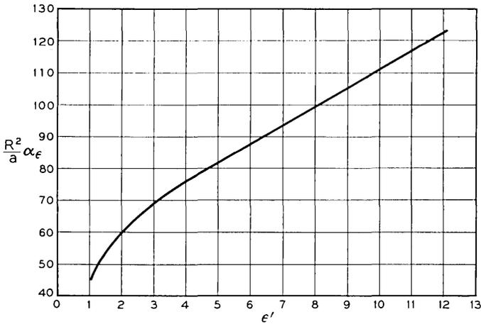
Fig. 2 — Curvature attenuation of the TE<sub>01</sub> mode, with  $\epsilon' = \epsilon''$ .
