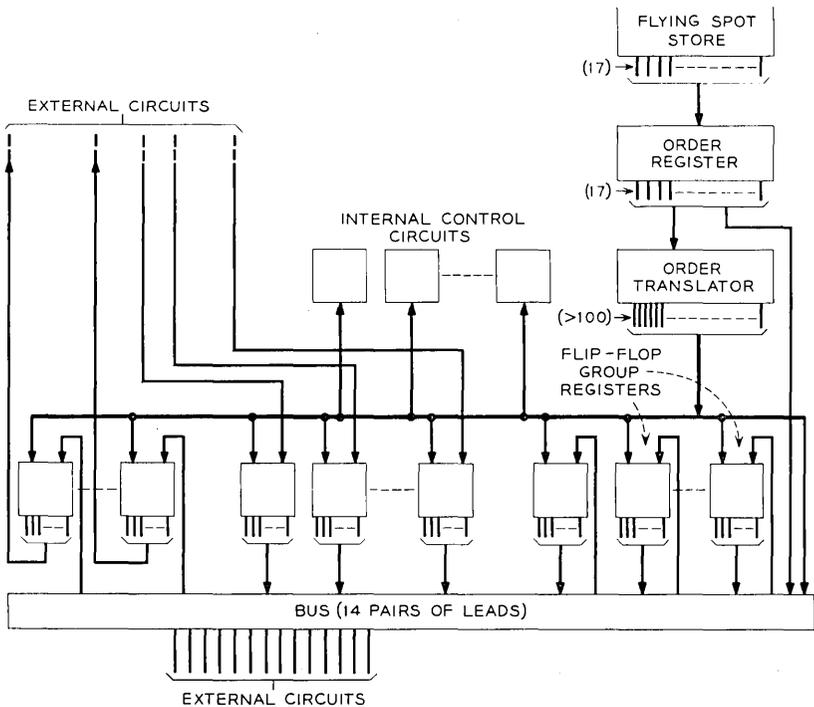
Fig. 12 — Simplified block diagram of central control.
