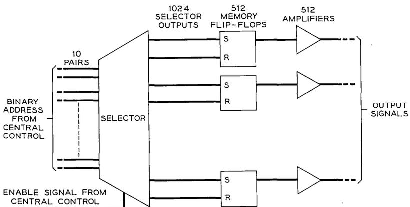
Fig. 2 — Functional diagram of the signal distributor.
