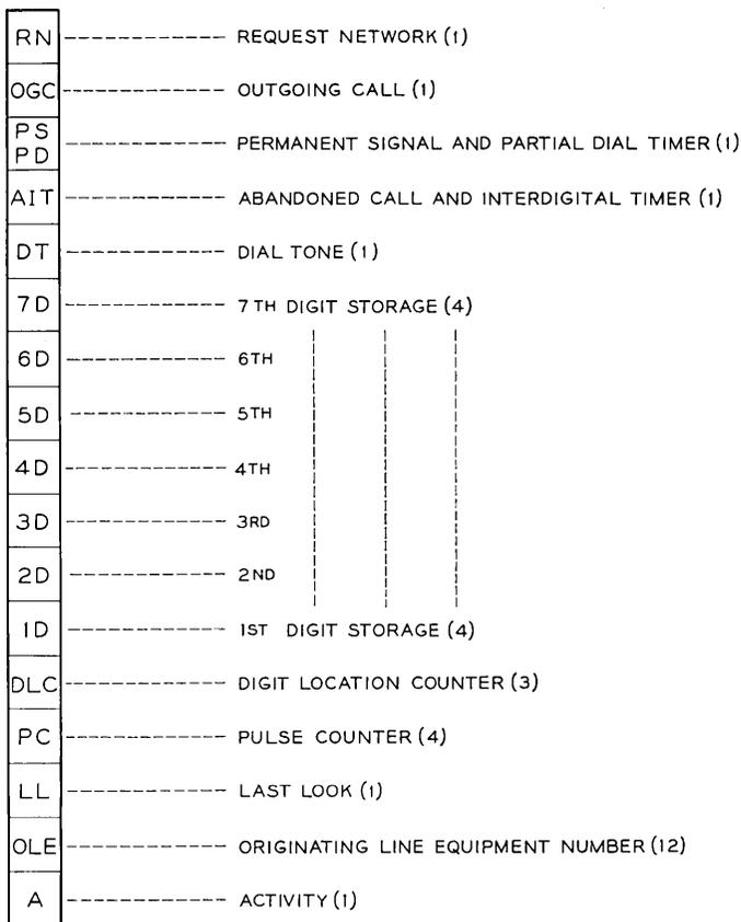
Fig. 2 — Originating register layout.
