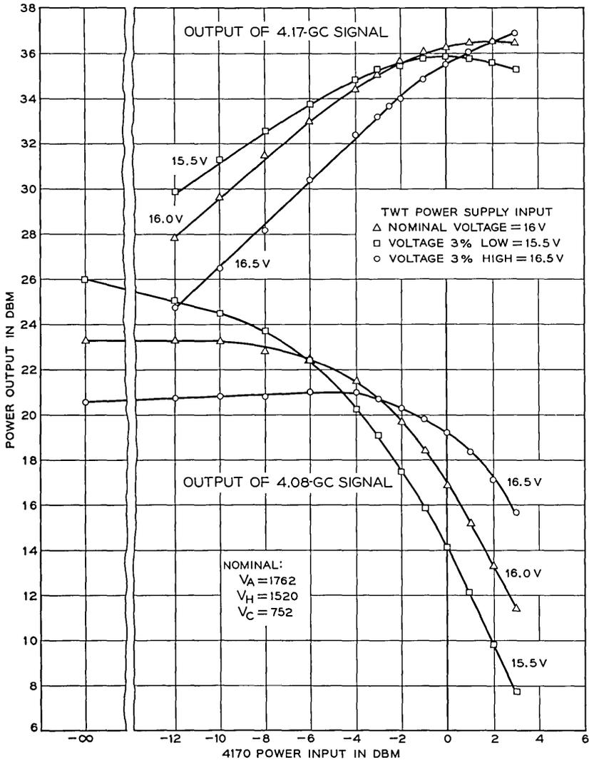
Fig. 24 — Two-signal operation of KP24 in final package. The 4.08-gc beacon input is held constant at  $-12$  dbm as the 4.17-gc signal is varied. Power output is shown for both frequencies with the input voltage to the TWT power supply as a parameter.
