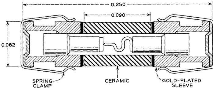
Fig. 2 — Encapsulation of sealed diode.
