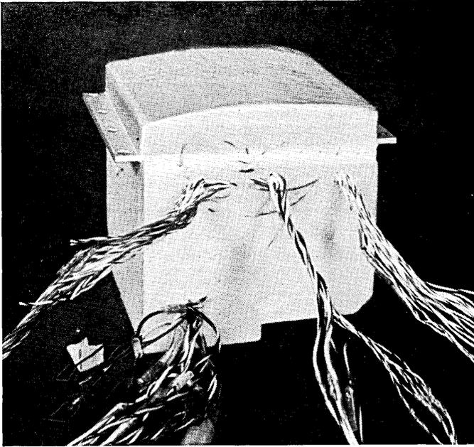
Fig. 4 — Encapsulated regulator.
