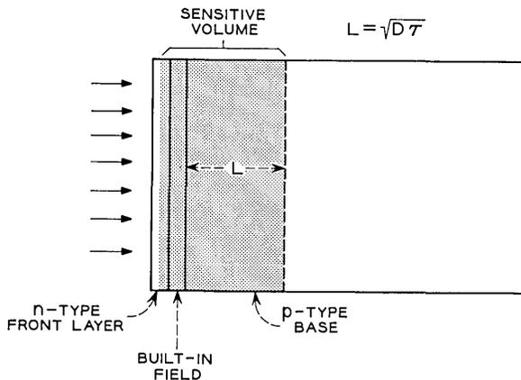
Fig. 1 — Schematic of n-on-p solar cell.
