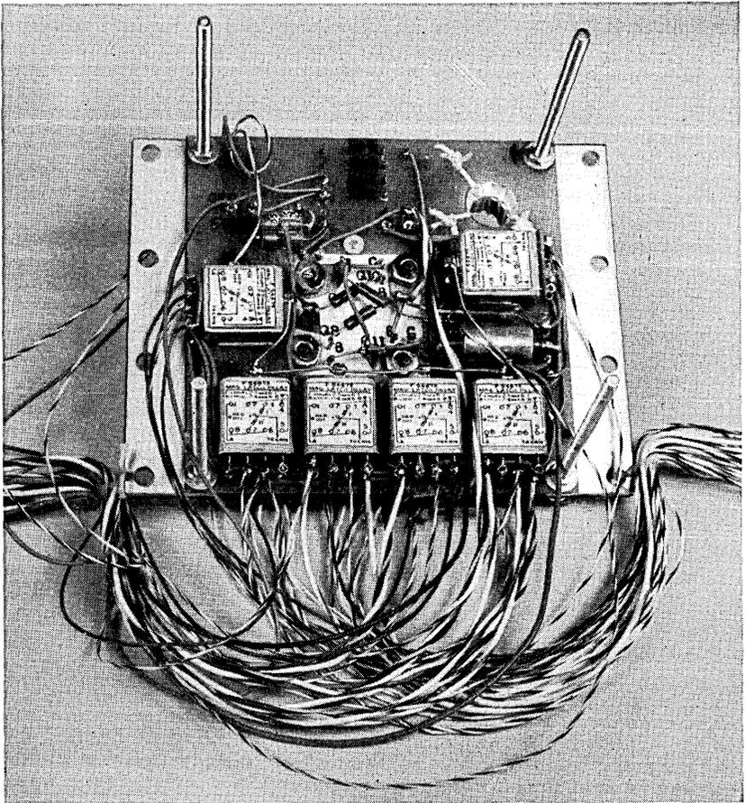
Fig. 1 — First circuit board of regulator.
