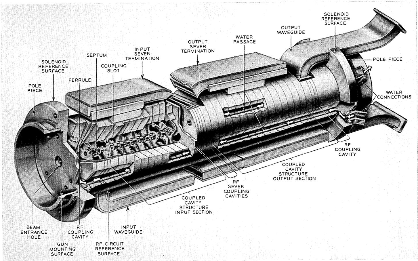
Fig. 4 — M4040 RF circuit.
