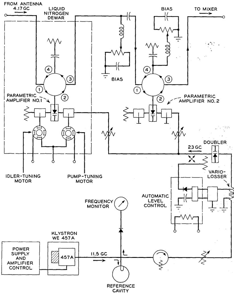
Fig. 1 — Block diagram of parametric receiver.
