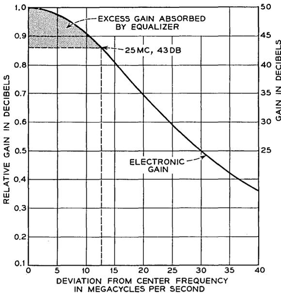
Fig. 11 — Determination of effective gain available with equalization.
