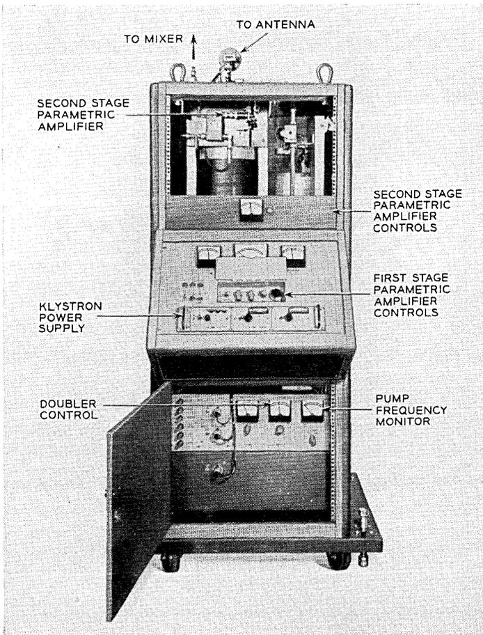
Fig. 10 — Front view of large amplifier package.
