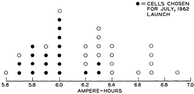
Fig. 5 — Capacity distribution, 40 nickel-cadmium cells.
