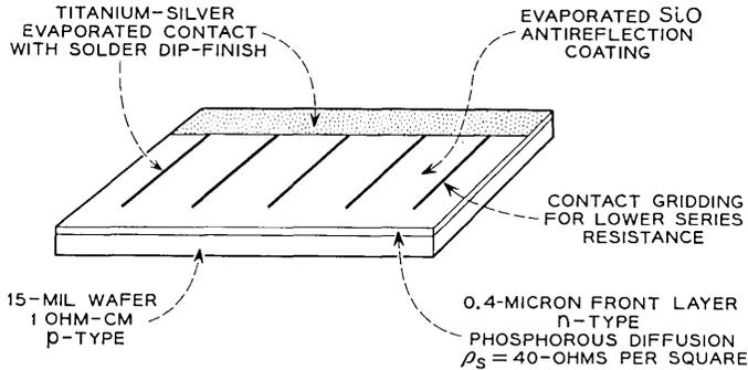
Fig. 11 — Cell structure.
