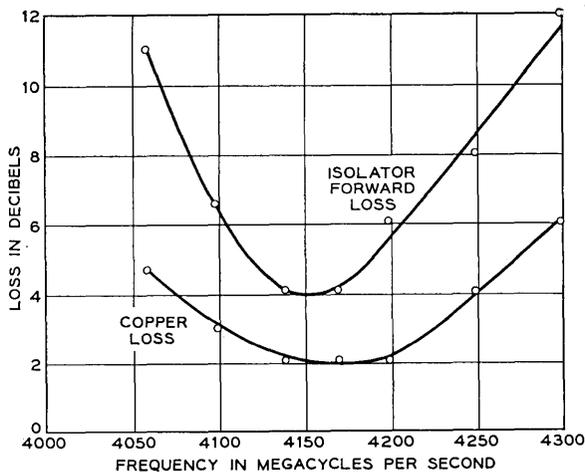
Fig. 7 — Typical losses for the structure at 4.2°K.
