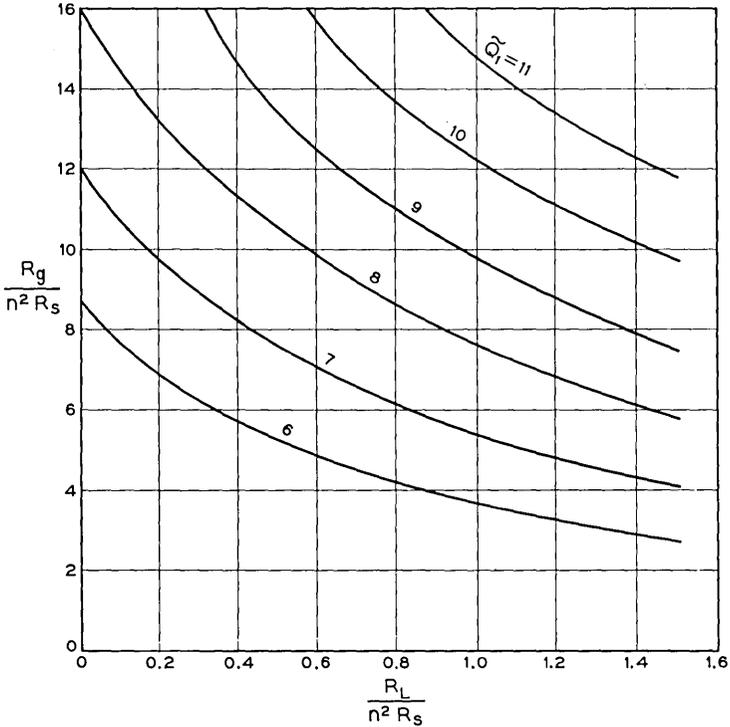
Fig. 5 — Normalized generator impedance  $R_g/R_s$  required for 20-db regenerative gain as a function of external idler loading factor  $R_L/R_s$  for given values of input circuit dynamic quality-factor  $\tilde{Q}$ .
