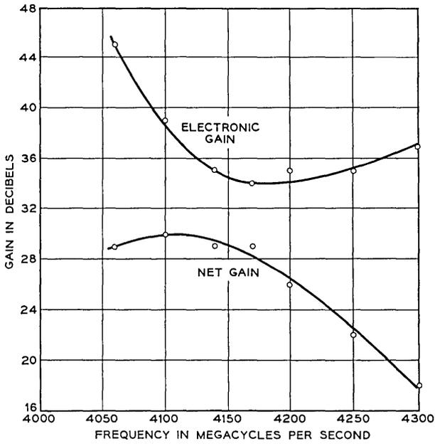
Fig. 9 — Gain of the stagger-tuned maser at 4.2°K.
