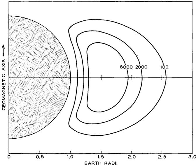
Fig. 31 — Isointensity contours of omnidirectional 24-36 Mev flux in protons/cm<sup>2</sup> per second.
