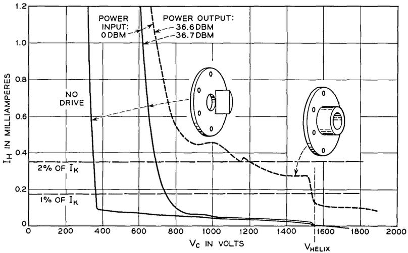
Fig. 10 — Depressed collector operation. Helix current vs collector voltage is shown for symmetrical and asymmetrical output pole-pieces. (Note the suppression of secondary and reflected electrons.)  $I_k = 17.4$  ma,  $V_{helix} = 1550$  v.
