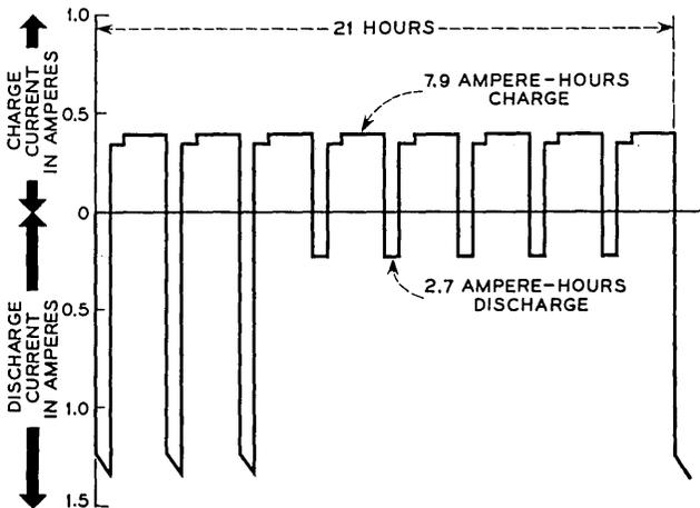
Fig. 7 — Load profile — simulated orbital cycle.
