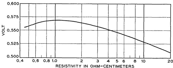
Fig. 10 — Solar cell open-circuit voltage vs resistivity.
