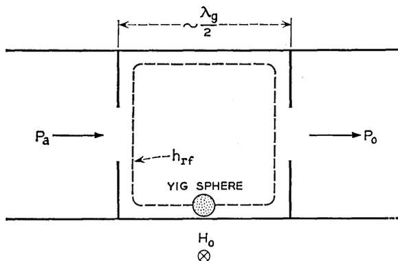
Fig. 4 — Schematic of the Telstar limiter.
