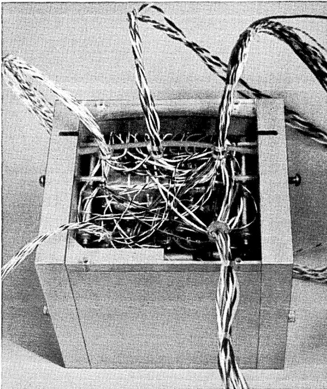
Fig. 3 — Regulator in mold ready for foam encapsulating.
