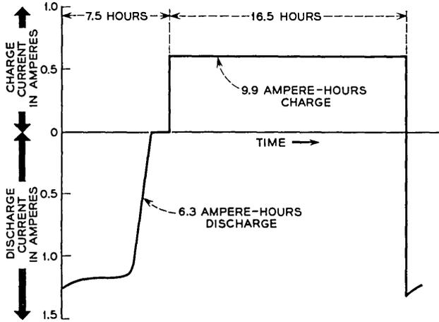
Fig. 8 — Load profile — accelerated life cycle.
