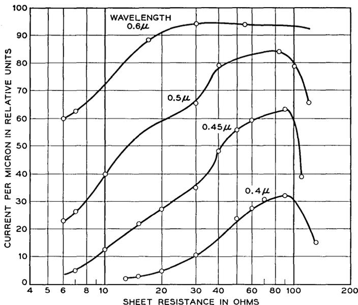
Fig. 15 — Spectral response vs sheet resistance.
