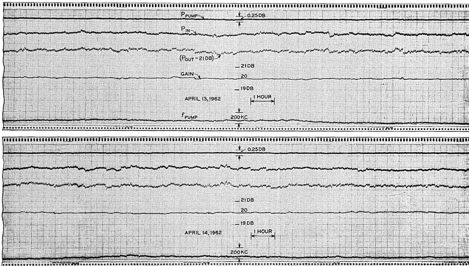
Fig. 15 — Recorded graph of amplifier stability. Pump line shows the pump power level;  $P_{in}$ , signal input;  $P_{out} - 21$  db, 21 db below amplifier output;  $f_{pump}$  the pump frequency deviation from 23 gc.
