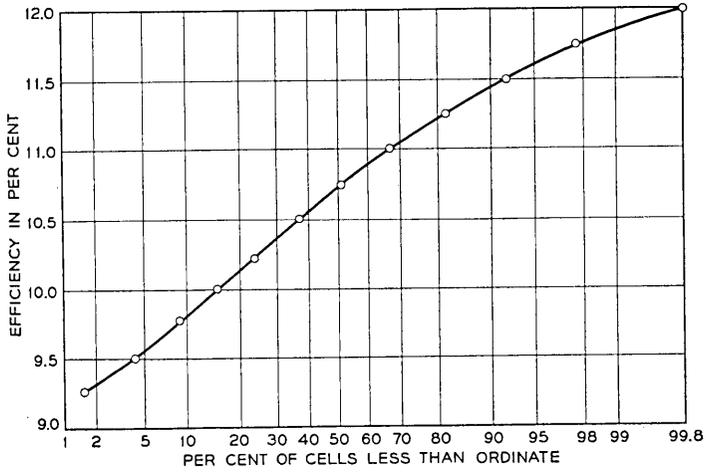
Fig. 19 — Conversion efficiency at 0.45 v.
