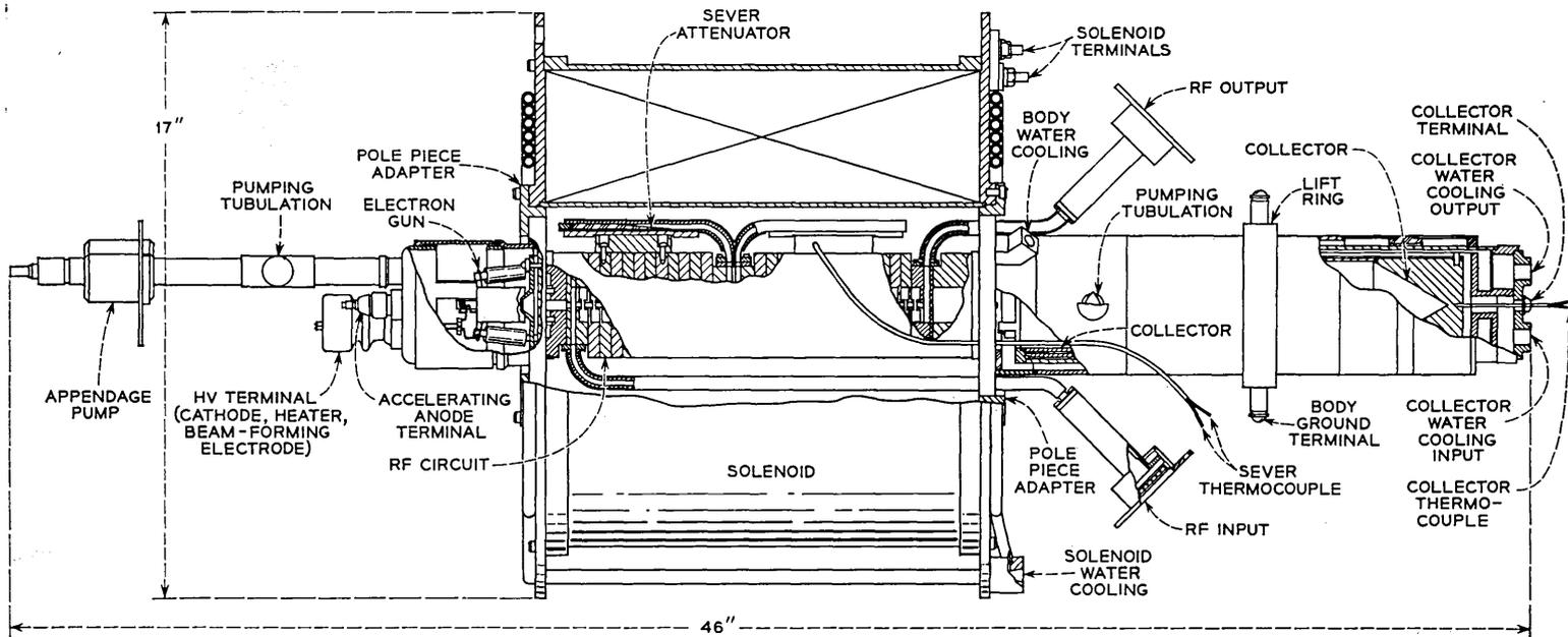
Fig. 2 — Internal structure of the M4040 tube.
