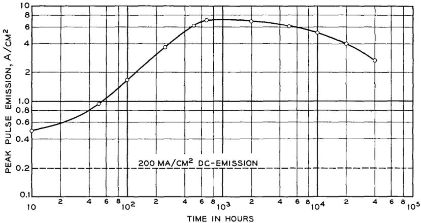
Fig. 4 — Life tests of control diodes with 0.1 per cent Zr-nickel base. Normal operating condition 200 ma/cm<sup>2</sup> dc, cathode temperature 740°C true. Activity measured by superimposing pulse directly over dc.
