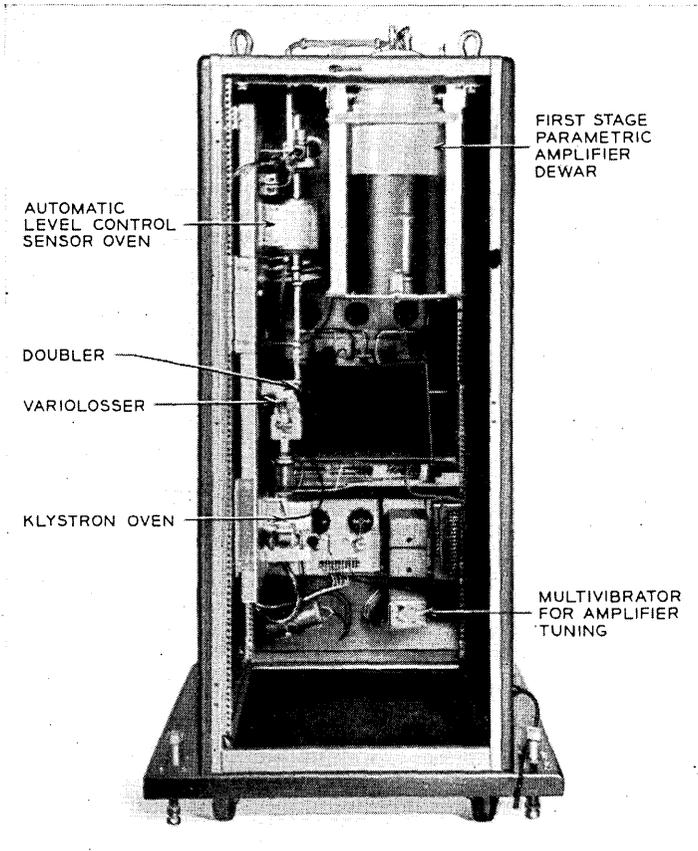
Fig. 11 — Back view of large amplifier package.
