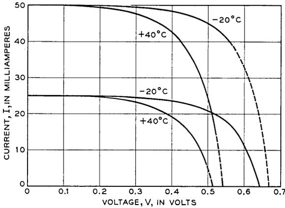
Fig. 27 — Typical solar cell output characteristic.
