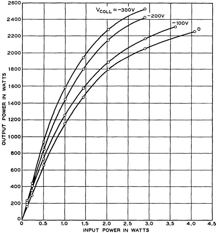
Fig. 22 — Output power vs input power [ $V_k = 17.0$  kv;  $H = 1.2$  H (Bri-louin);  $f = 6.4$  gc; parameter is collector depression].
