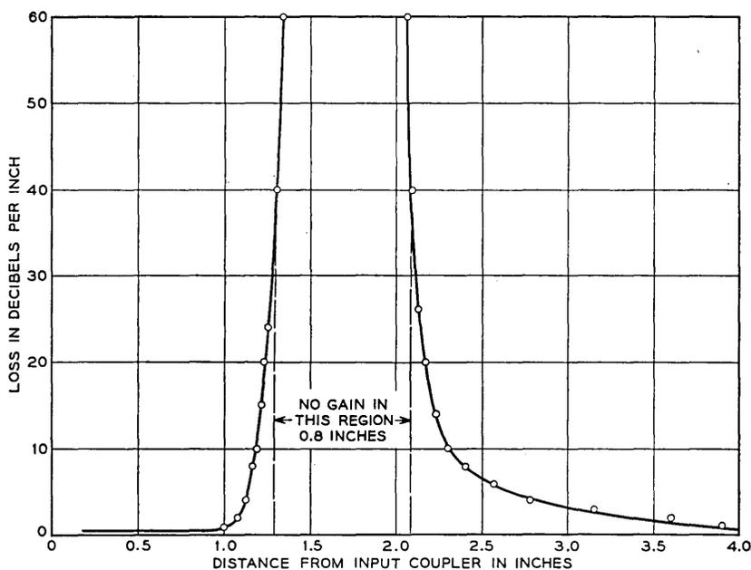
Fig. 7 — Final helix loss patterns of sprayed aquadag (intrinsic loss with Cu plating 2.78 db; total loss 83 db).
