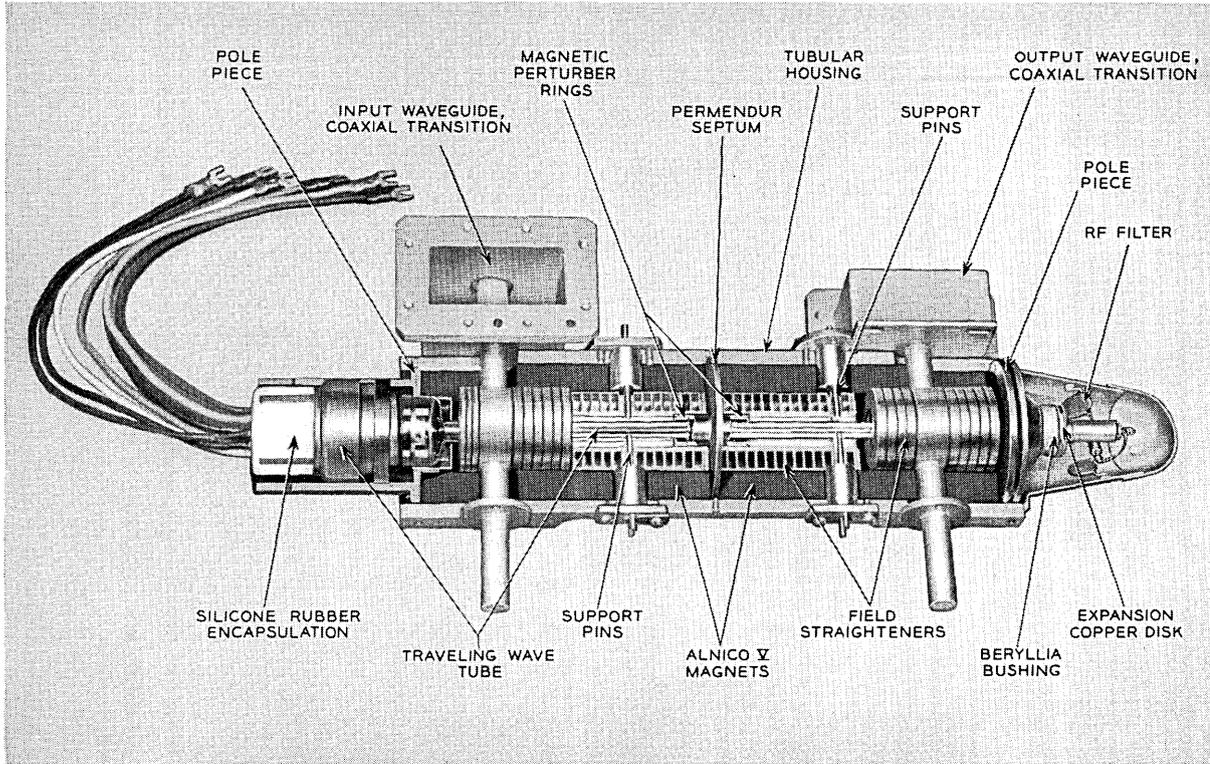
Fig. 17 — Cross-section view of completed amplifier package.
