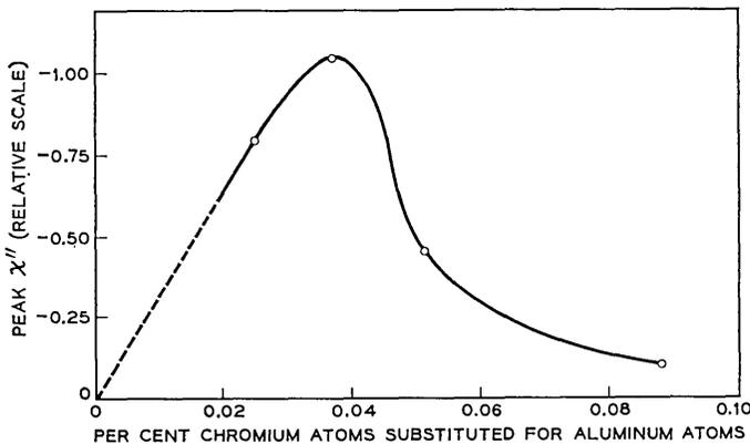
Fig. 1 — Inverted susceptibility vs concentration for ruby at 5.6 ge and  $4.2^\circ\text{K}$ .
