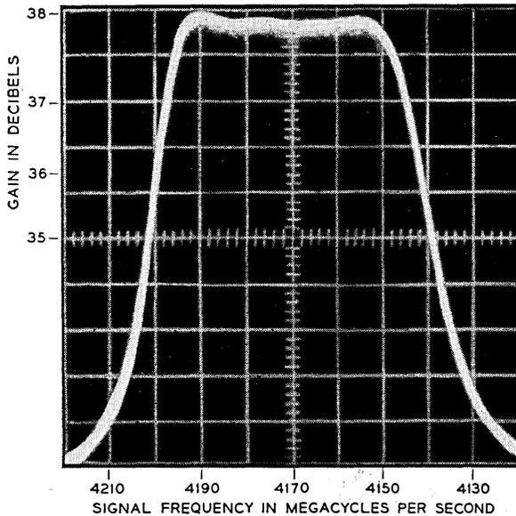
Fig. 14 — Gain-frequency band characteristic of parametric amplifier no. 2.
