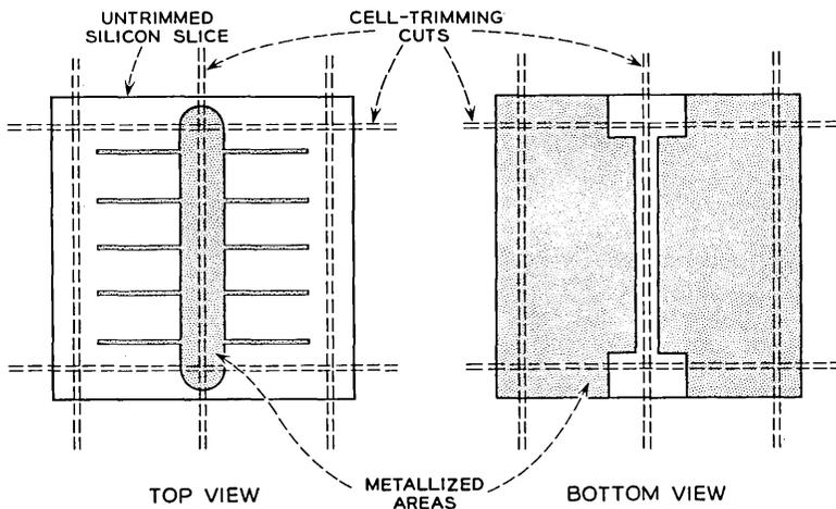
Fig. 16. — Contact configuration and cell trimming.
