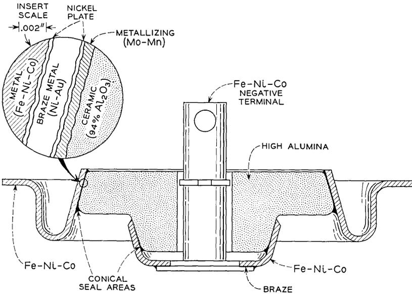
Fig. 2 — Details of ceramic seal.
