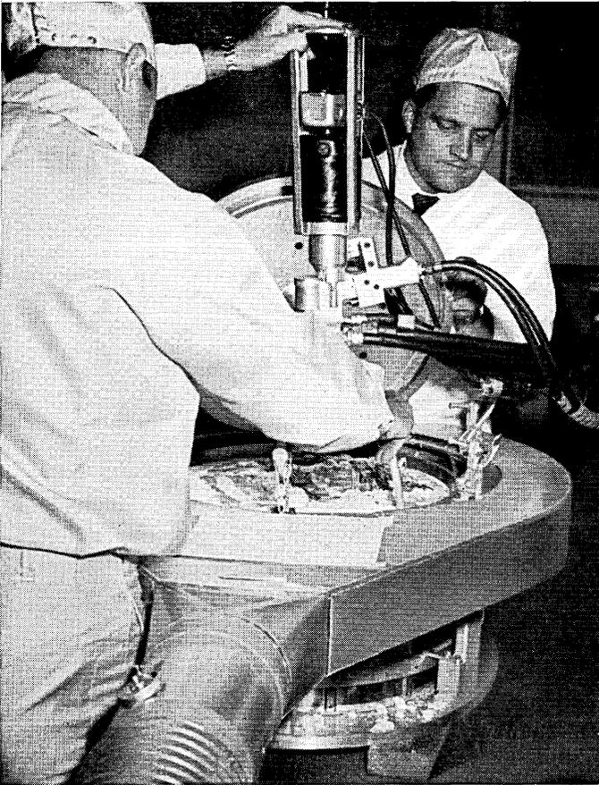
Fig. 8 — Foam encapsulation of the canister.
