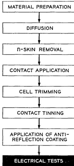
Fig. 13 — Fabrication sequence for n-on-p solar cells.
