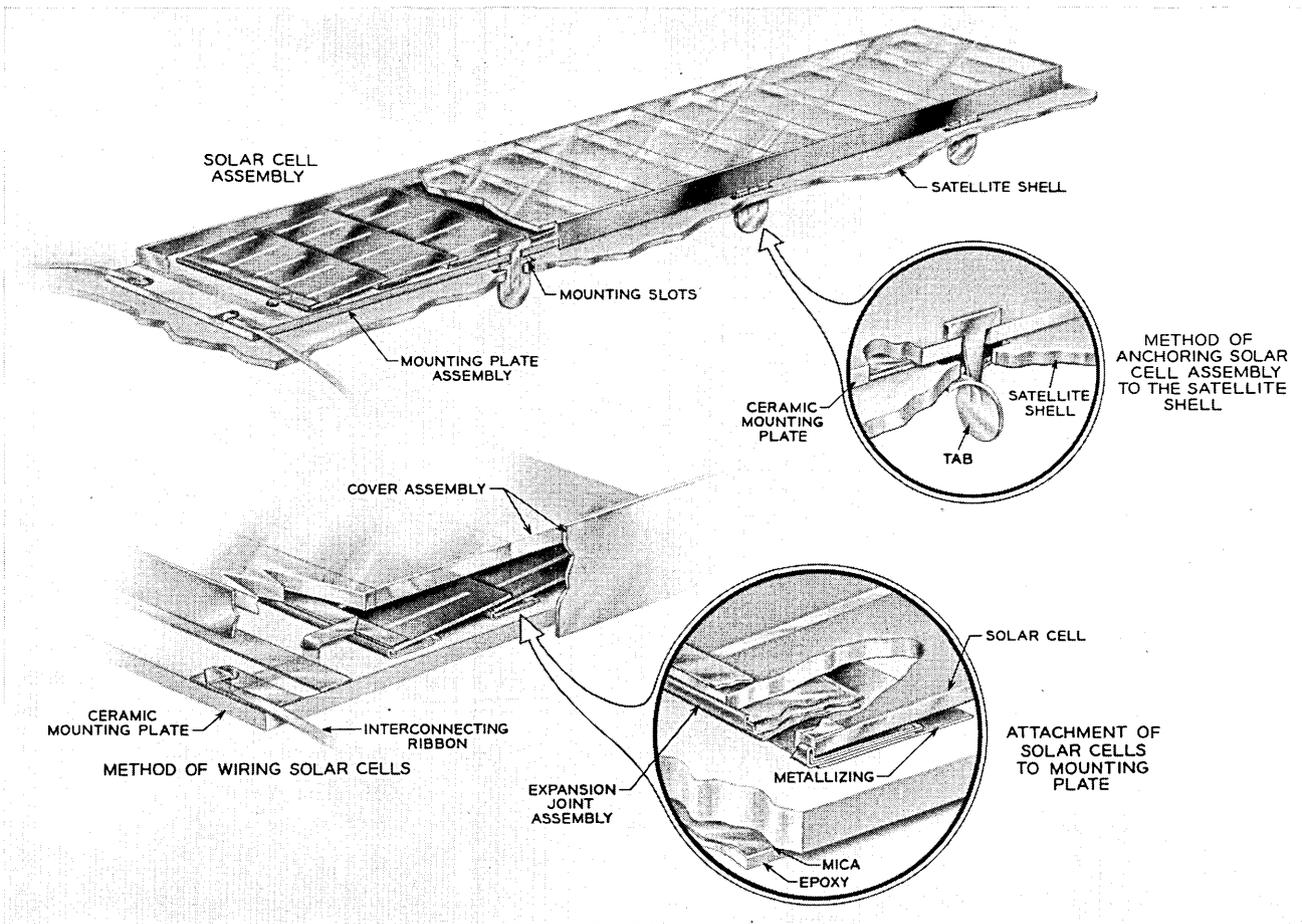
Fig. 22 — Solar cell assembly for communications satellite.
