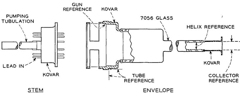
Fig. 11 — Envelope assembly with reference surfaces.
