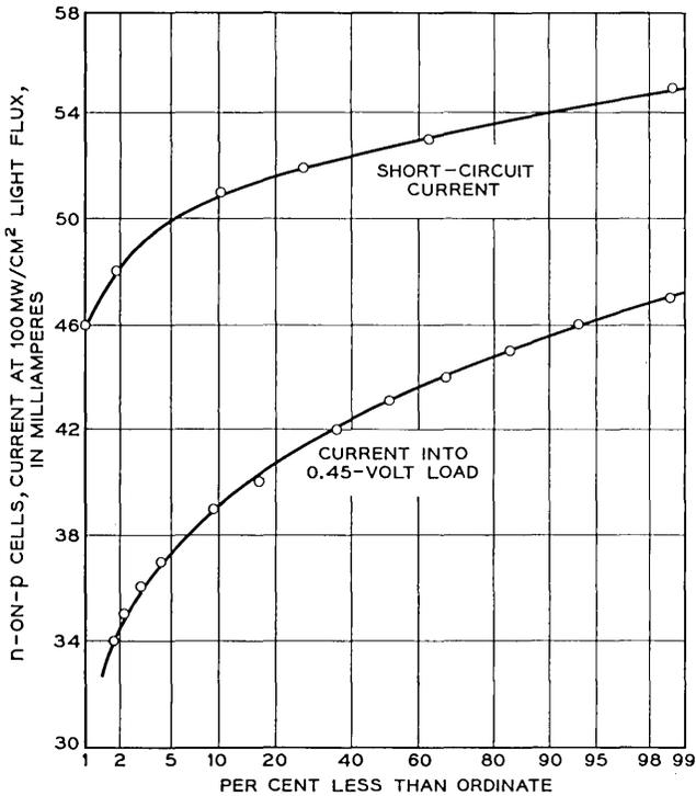
Fig. 18 — Short-circuit current and current into 0.45-v load.
