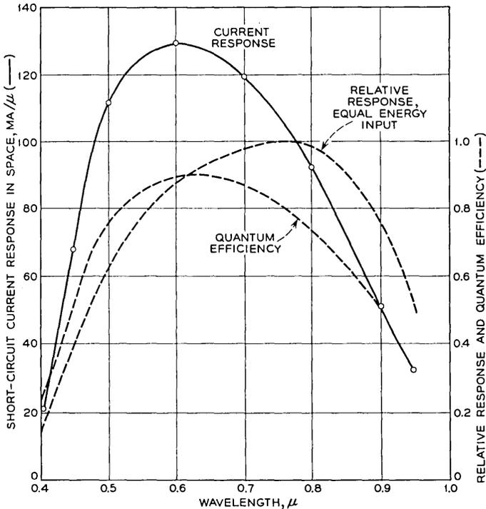
Fig. 12 — Spectral response, n-on-p solar cell.
