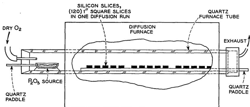
Fig. 14 — Schematic of phosphorus diffusion system.
