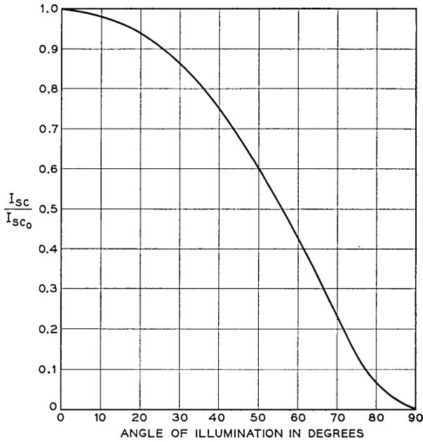
Fig. 26 — Normalized short-circuit current vs angle of illumination.
