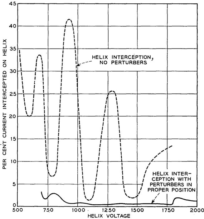
Fig. 14 — Single-reversal circuit, helix interception vs helix voltage.
