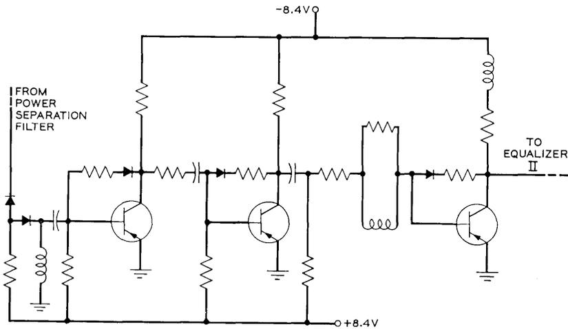
Fig. 24 — Preamplifier circuit.
