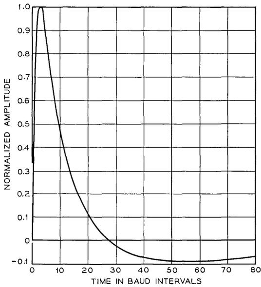
Fig. 15 — Nominal isolated pulse without equalization.
