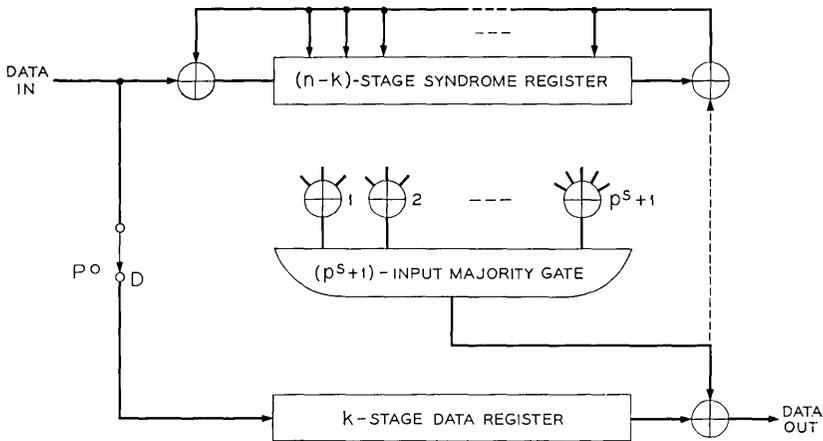
Fig. 1 — Fixed threshold majority-logic decoder for difference-set cyclic codes.
