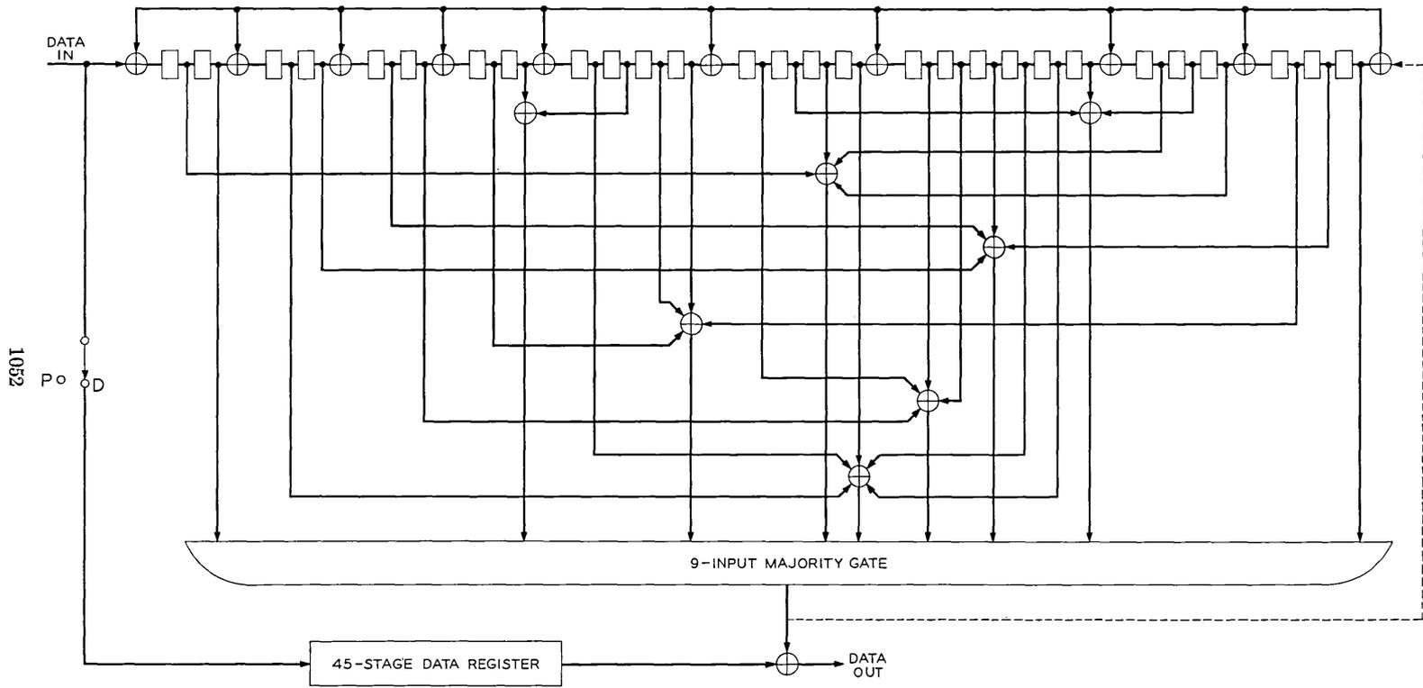
Fig. 2 — Decoder for (73, 45),  $d = 10$ , binary difference-set cyclic code.
