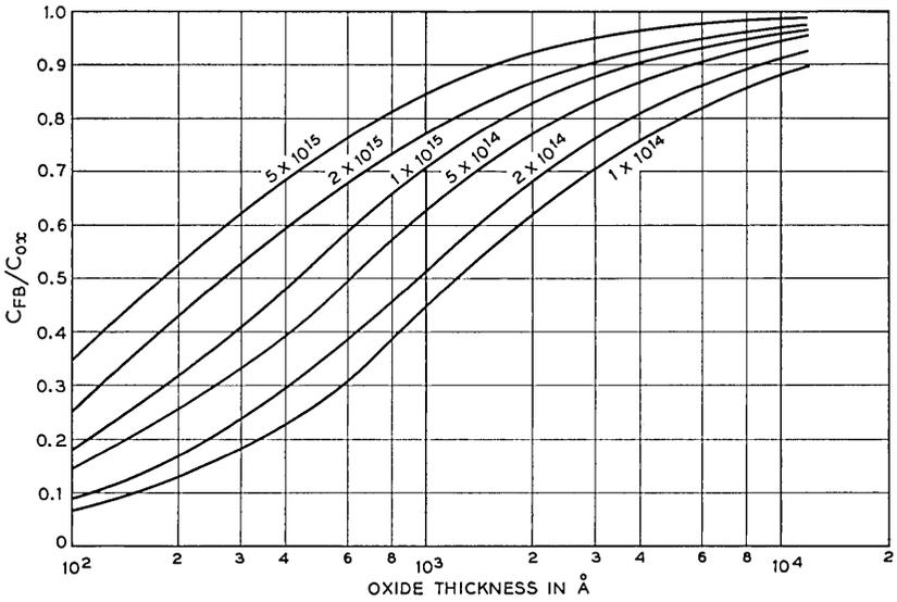
Fig. 42 — Flatband capacity vs oxide thickness II.
