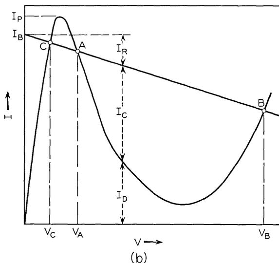
Fig. 34—Esaki diode model; (a) equivalent circuit; (b) volt-ampere characteristic of nonlinear resistance.
