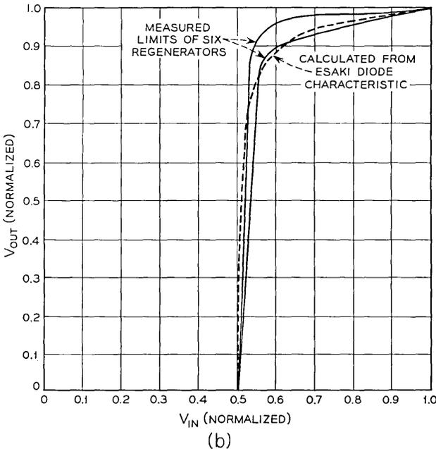
Fig. 35 — Input-output dynamic regenerator characteristic; (a) experimental setup; (b) measured and calculated characteristic.
