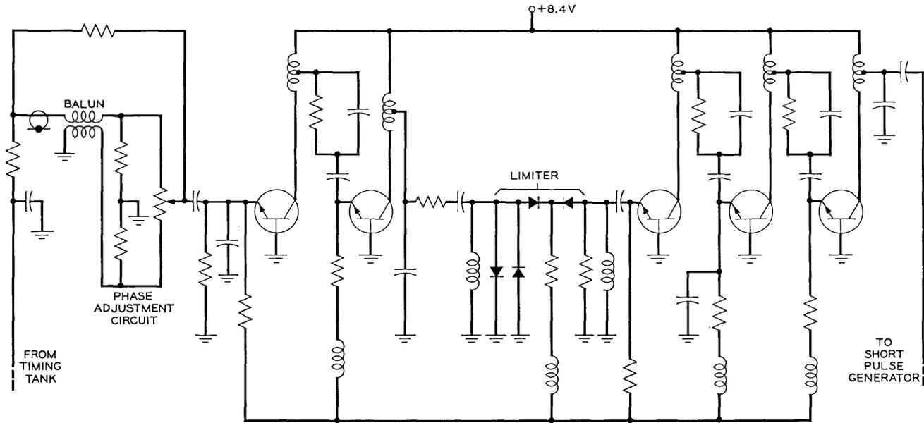
Fig. 28 — Timing amplifier circuit.
