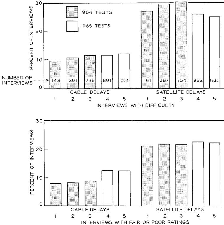
Fig. 25 — Comparison of 1964 and 1965 tests.
