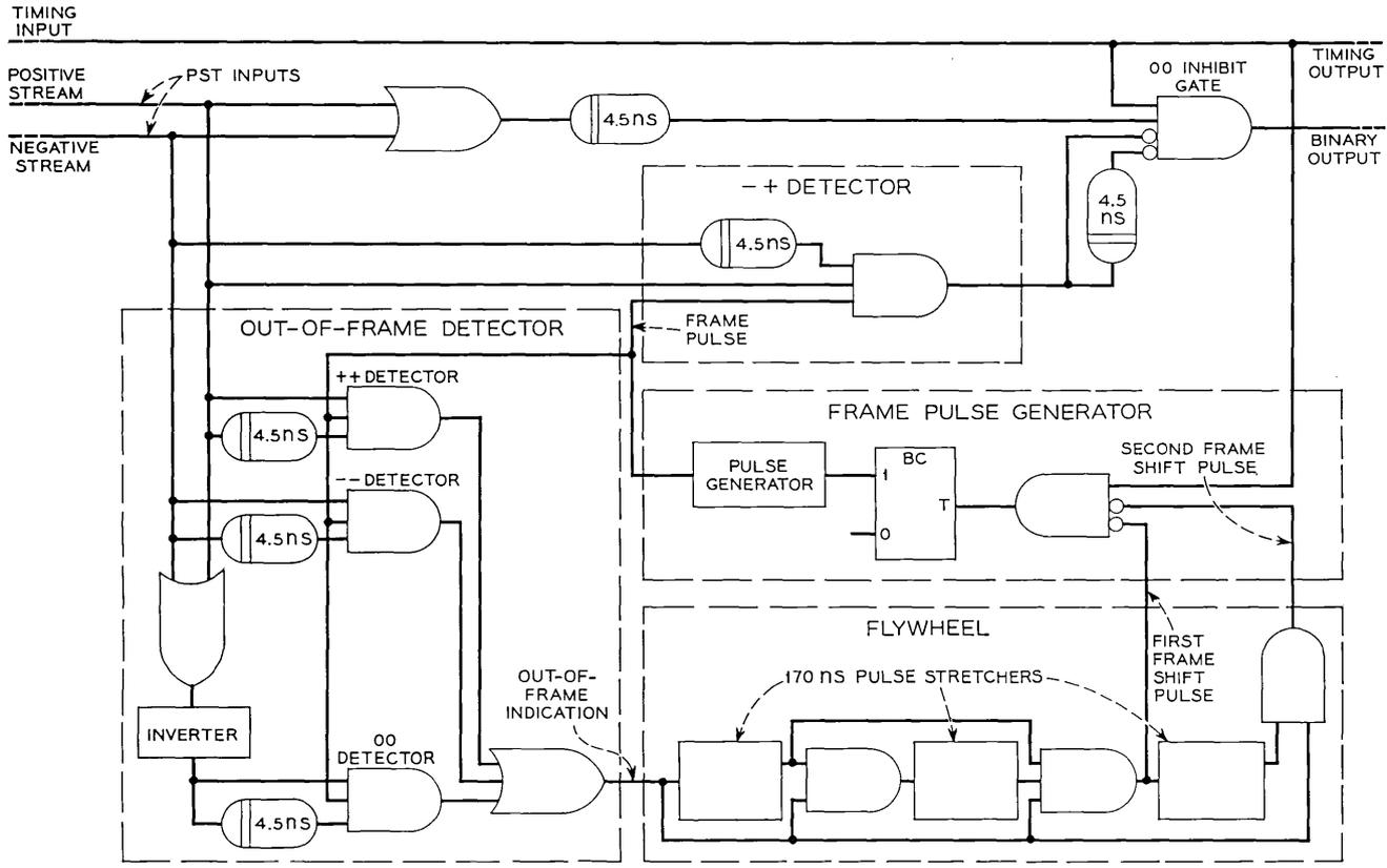
Fig. 4 — Logical diagram of the PST-to-binary translator.
