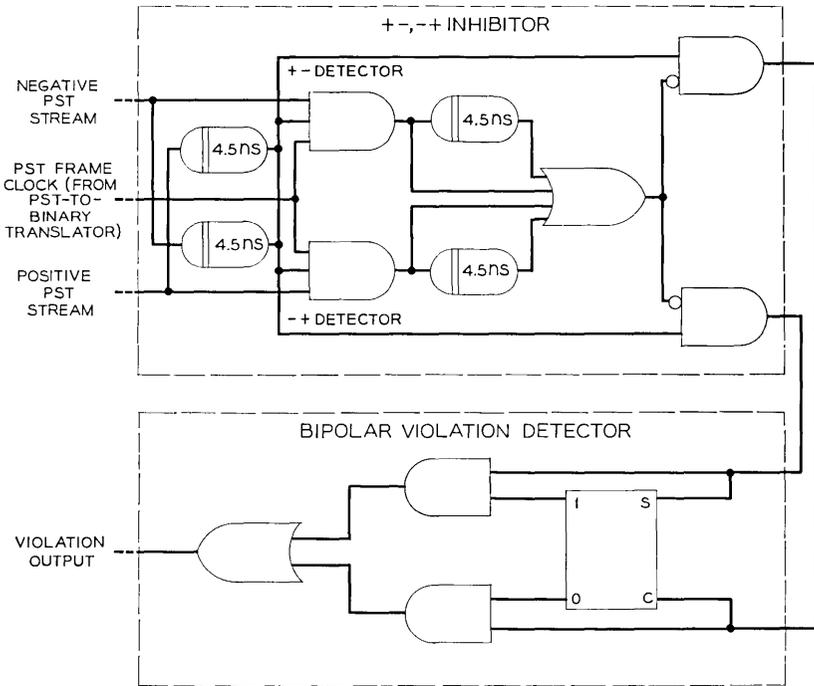
Fig. 7 — Logical diagram of the PST violation monitor.
