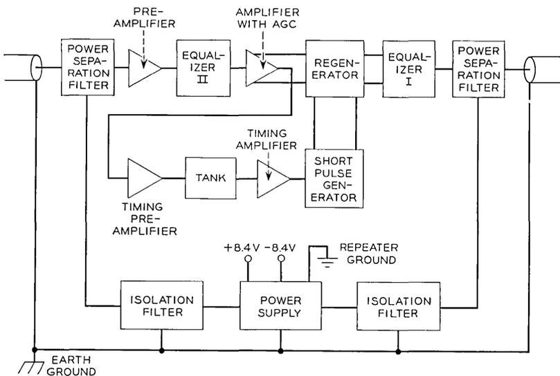
Fig. 21 — Functional block diagram of the repeater.
