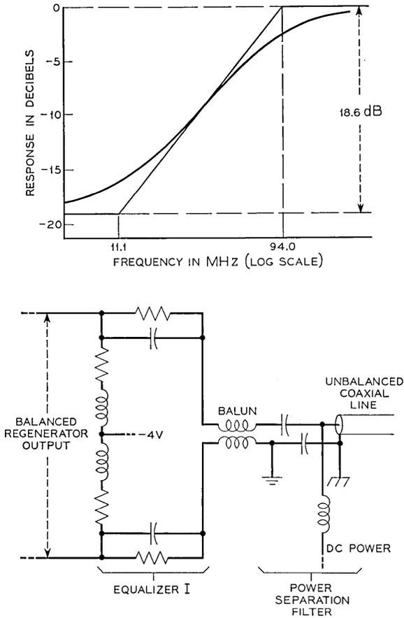
Fig. 22 — Equalizer I—attenuation characteristic and circuit configuration.
