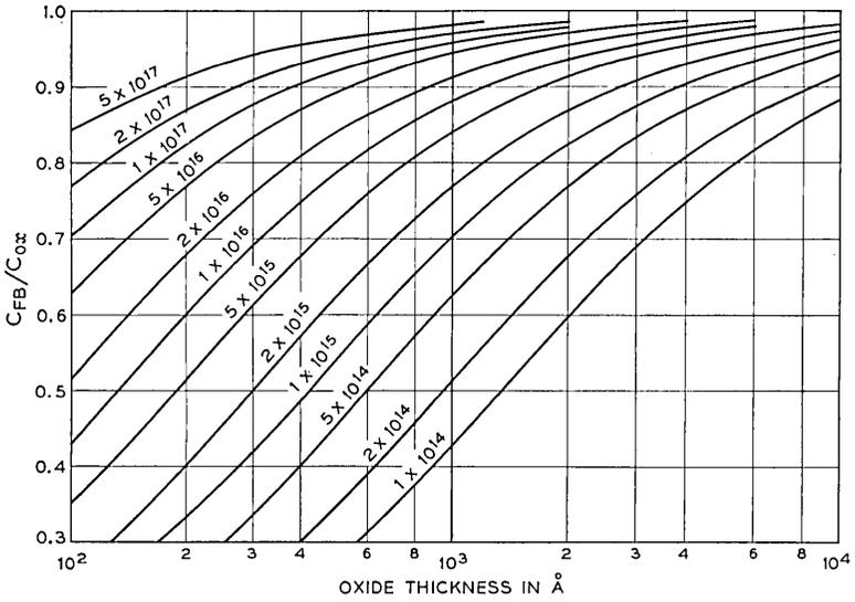
Fig. 41 — Flatband capacity vs oxide thickness I.
