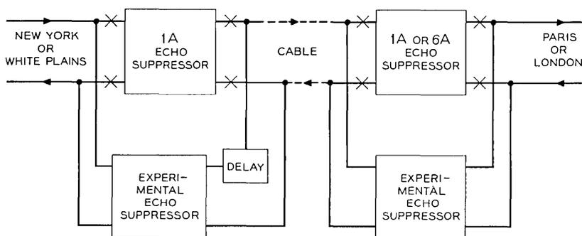
Fig. 1 — Placement of echo suppressors and delay.
