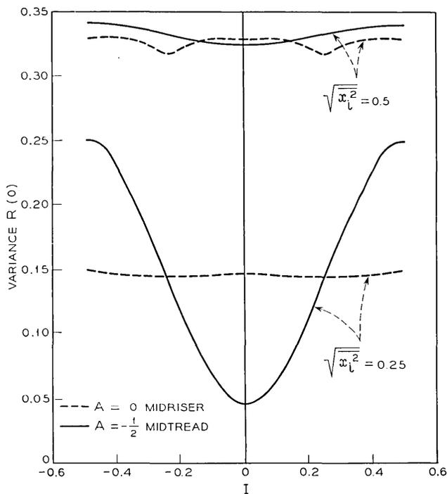
Fig. 12 — Idle channel noise in DPCM system.
