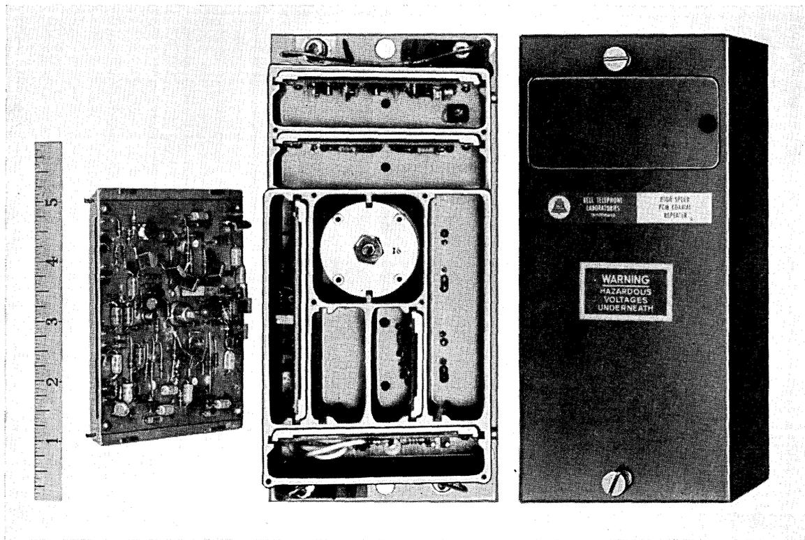
Fig. 37—Photograph of repeater with the amplifier printed circuit board removed. Shielding covers have been removed and are not shown.
