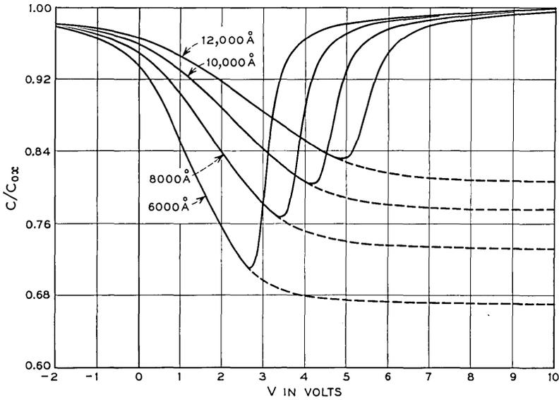
Fig. 23 — MOS capacity vs voltage. Oxide thickness 6000-12,000 Å. ( $N_A = 1.0 \times 10^{15} \text{ cm}^{-3}$ )
