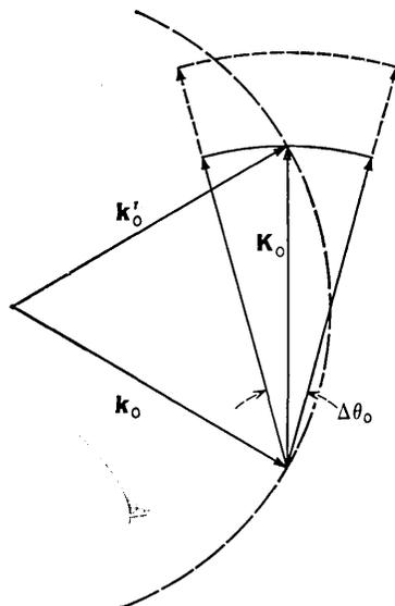
Fig. 5—A  $k$ -vector diagram of the Bragg diffraction process in which the acoustic diffraction angle is large compared with the optical diffraction angle.
