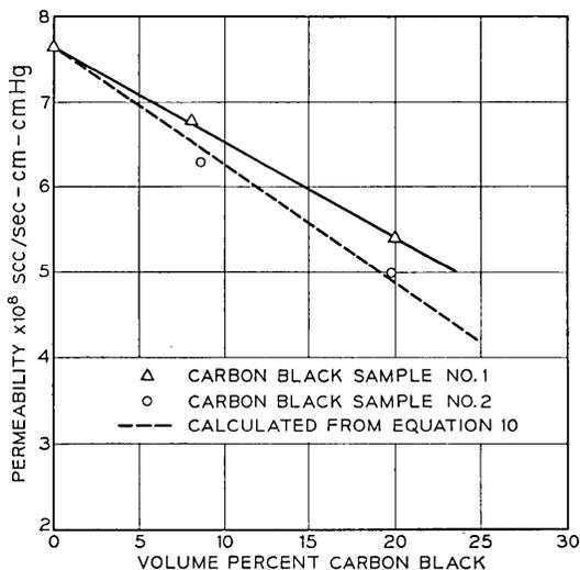
Fig. 15—Effect of carbon black on permeability of poly (ethylene ethyl acrylate) copolymer.
