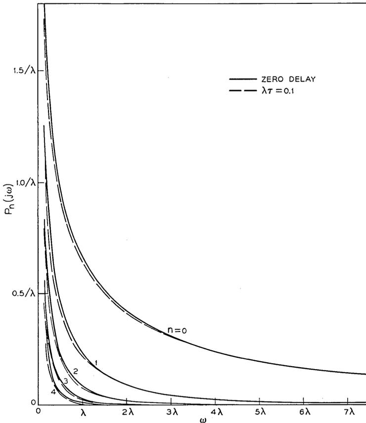
Fig. 12—Frequency response of an infinite bilateral ring.
