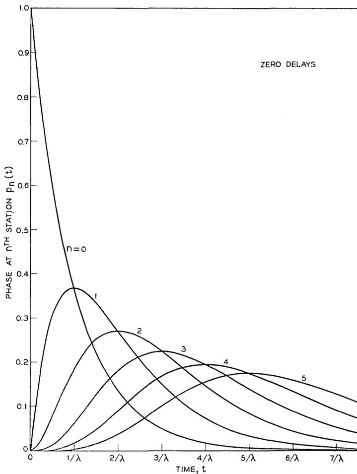
Fig. 8—Impulse response of an infinite unilateral ring.
