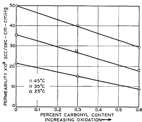
Fig. 10 — Increasing oxidation decreases permeability of polyethylene.
