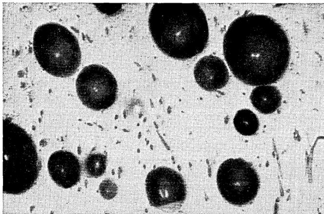
Fig. 12 — Photomicrograph ( $50\times$ ) showing pores in polyurethane.
