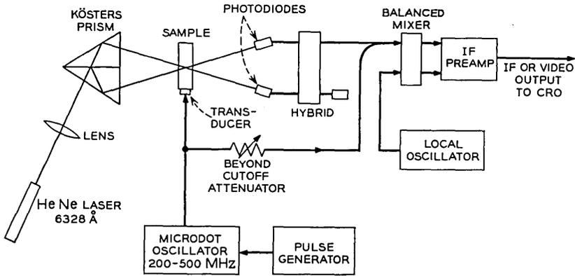
Fig. 3 — Schematic diagram of experimental apparatus.
