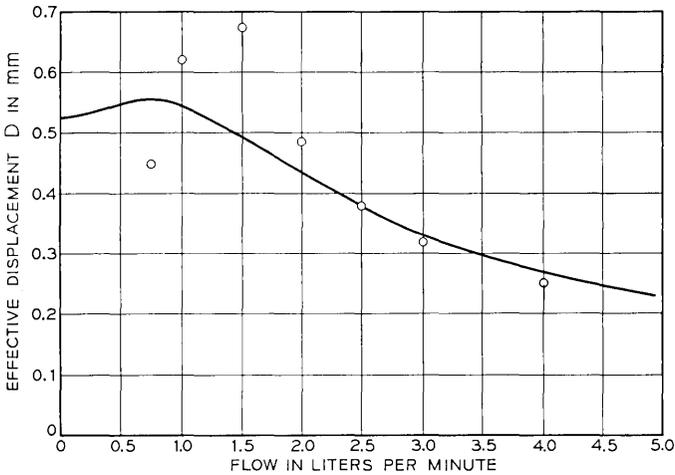
Fig. 5—Displacement of the optical center of a tubular gas lens using  $\text{CO}_2$  and a tube of 7 inches long and  $\frac{1}{4}$ -inch diameter. Measured data by Steier.<sup>3</sup>
