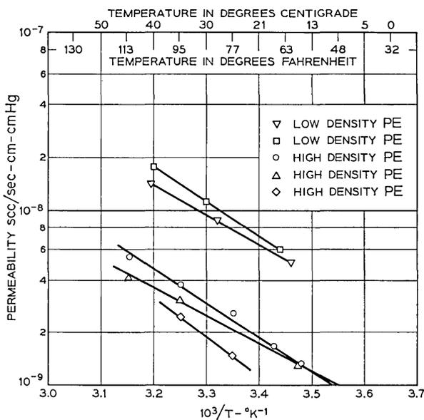
Fig. 6 — Comparison of high-density with low-density polyethylene.
