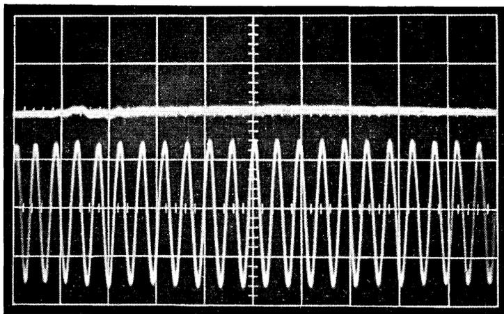
Fig. 10 — Oscilloscope trace showing 80 percent modulation depth at 20 MHz obtained using optical heterodyne detection. The relative diffracted intensity was about 20 percent.
