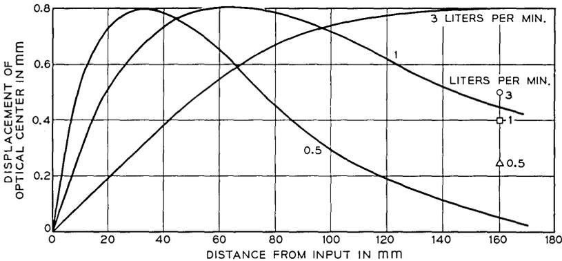
Fig. 3 — Displacement of the profile center in a tubular gas lens of  $\frac{3}{8}$ -inch i. d. for flow rates of 0.5, 1, and 3 liters per minute using air. ( $\alpha = 0.22 \text{ cm}^2/\text{s}$ ). Measured data by DeGano.<sup>3</sup>
