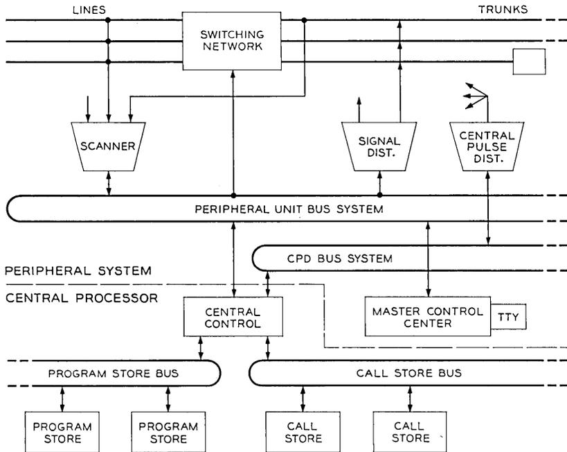
Fig. 6 — No. 1 ESS block diagram.
