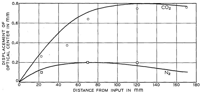
Fig. 4—Displacement of the profile center in a tubular gas lens of  $\frac{1}{4}$ -inch i. d. for a flow rate of 1 liter per minute using  $\text{CO}_2$  ( $\alpha = 0.1 \text{ cm}^2/\text{s}$ ) or  $\text{N}_2$  ( $\alpha = 0.2 \text{ cm}^2/\text{s}$ ). Measured data by Steier.<sup>3</sup>
