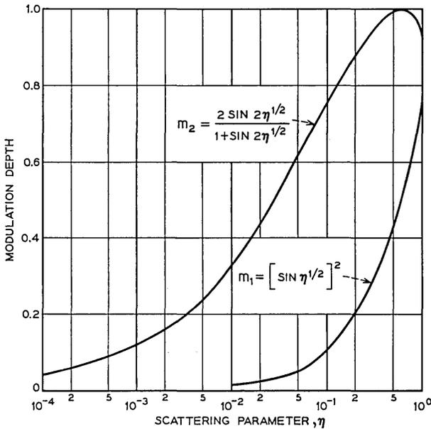
Fig. 9—Theoretical curves, valid for plane waves, of the ordinary optical modulation depth  $m_1$  and the optical heterodyne modulation depth  $m_2$  both plotted vs acoustic scattering parameter  $\eta$ .
