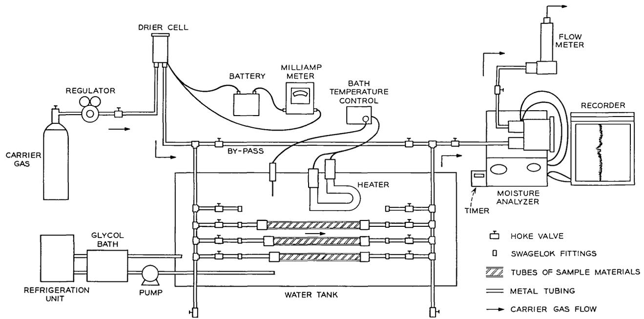
Fig. 1 — Moisture permeability apparatus for tubular samples.
