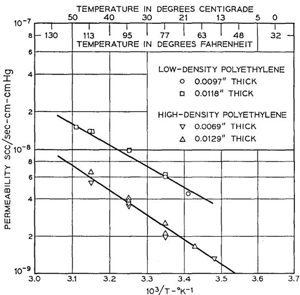
Fig. 4 — Measured permeability is not a function of film thickness.
