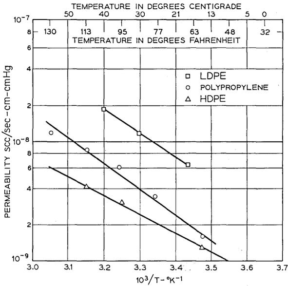
Fig. 8—Comparison of polypropylene with typical high- and low-density polyethylenes.
