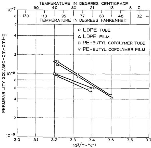
Fig. 5—Permeabilities of films are slightly lower than tubes.
