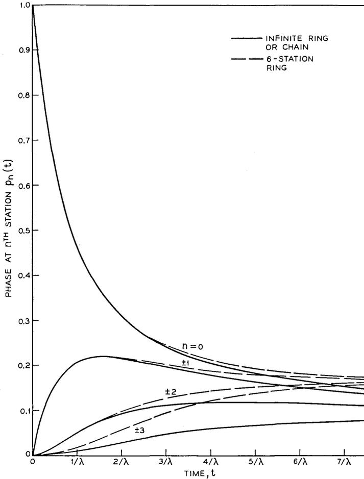
Fig. 4—Impulse response of bilateral rings with zero delays.
