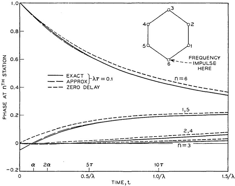
Fig. 6—Impulse response of a 6-station bilateral ring.
