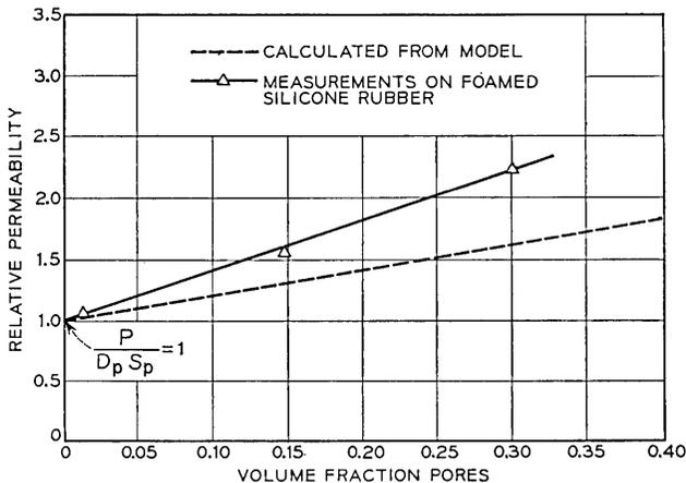
Fig. 13 — Measured foam WVP is higher than calculated.
