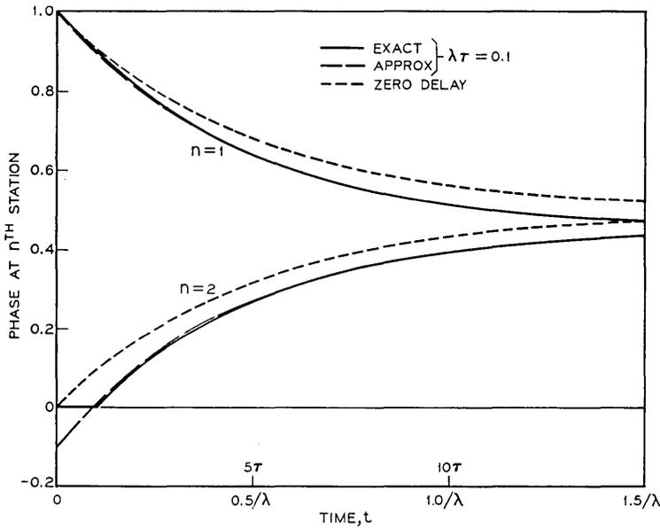
Fig. 2— Impulse response of a two-station system.
