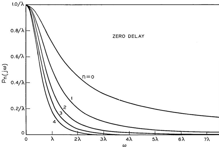
Fig. 13—Frequency response of an infinite unilateral ring.
