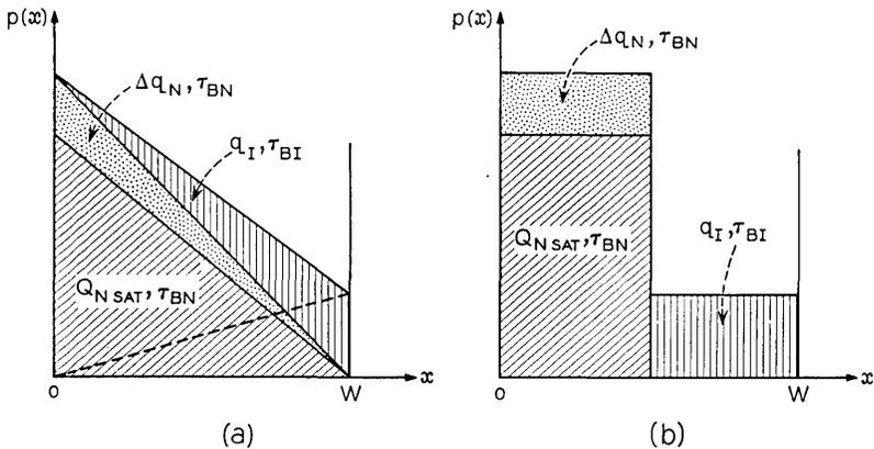
Fig. 22—The transistor in saturation. (a) Actual distribution of excess minority carriers. (b) Lumped approximation. The  $\pi$  and  $T$  models use  $q_N$  and  $q_I$  with lifetimes  $\tau_{BN}$  and  $\tau_{BI}$ ; the Beaufoy-Sparkes model uses  $Q_{N\text{ SAT}}$  and  $q_{BS} = \Delta q_N + q_I$  with lifetimes  $\tau_{BN}$  and  $\tau_S$ , where  $\tau_S$  is as defined in (88).
