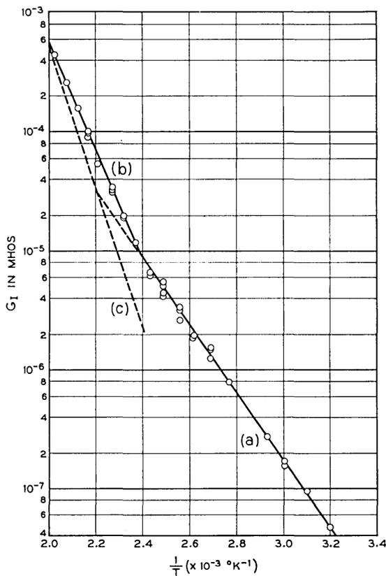
Fig. 6—Equivalent parallel conductance measured at 6 kHz and a bias of  $-15$  volts as a function of reciprocal degrees Kelvin. The experimental points indicated by the circles were obtained from Fig. 3. Multiple circles at a given temperature represent several runs. The solid lines are the best fit to the experimental points. Curve (c) is obtained by subtracting the values of  $G_T$  in curve (b) from the extrapolation of curve (a) at each temperature.
