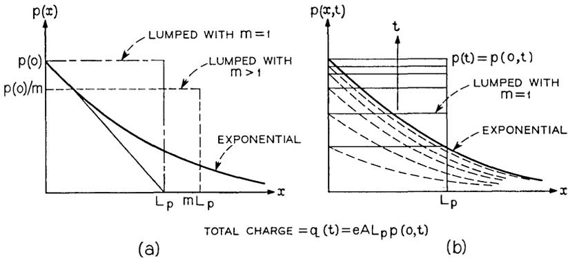
Fig. 8—Exponential and corresponding lumped distribution of excess minority carriers in the bulk material of a diode. (a) Illustration of the choice of lumping length. (b) Time variation for  $m = 1$ ;  $m = 1$  is generally preferred in the Linvill model, and is irrelevant in charge models or circuit applications of the Linvill model.
