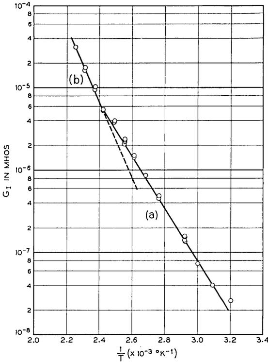
Fig. 7—Equivalent parallel conductance measured at 100 kHz and a bias of  $-15$  volts as a function of reciprocal degrees Kelvin. The experimental points indicated by the circles were obtained from Fig. 5. Multiple circles at a given temperature represent several runs. The solid lines are the best fit to these points.
