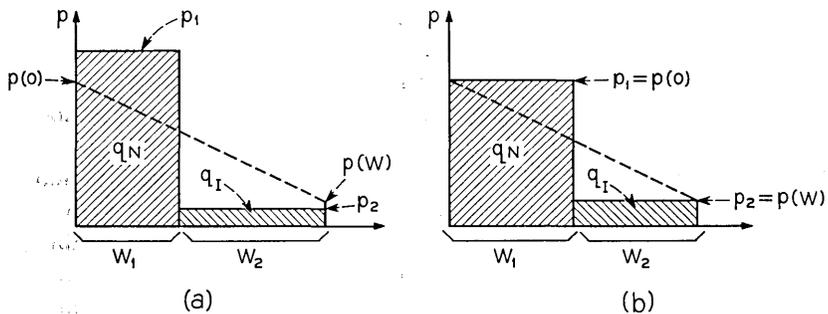
Fig. 18—Excess carrier distribution in the transistor base as used or implied in all first-order transistor models. (a) General case  $p_1 \neq p(0)$ ,  $p_2 \neq p(W)$ . (b) Commonly used choice  $p_1 = p(0)$ ,  $p_2 = p(W)$ .
