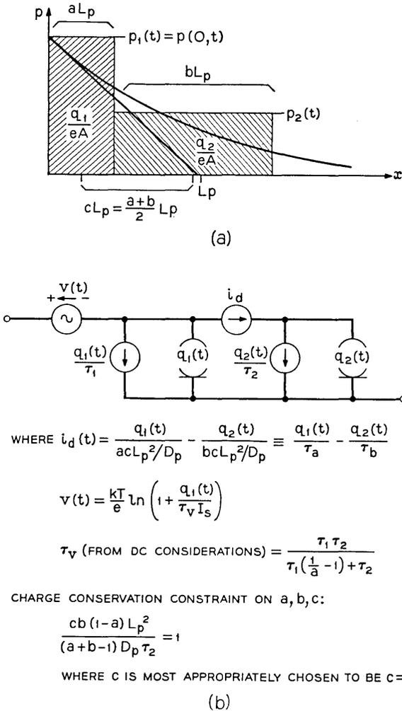
Fig. 12—Higher-order,  $\pi$ -Approximation of diode charge-control model. (a) Charge approximation. (b) Corresponding model.
