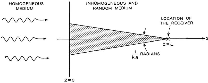
Fig. 12—Physical configuration for calculation of amplitude fluctuations.
