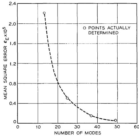
Fig. 7—Mean square error  $\epsilon_E$ , as function of the number of modes used, for H-plane discontinuity.
