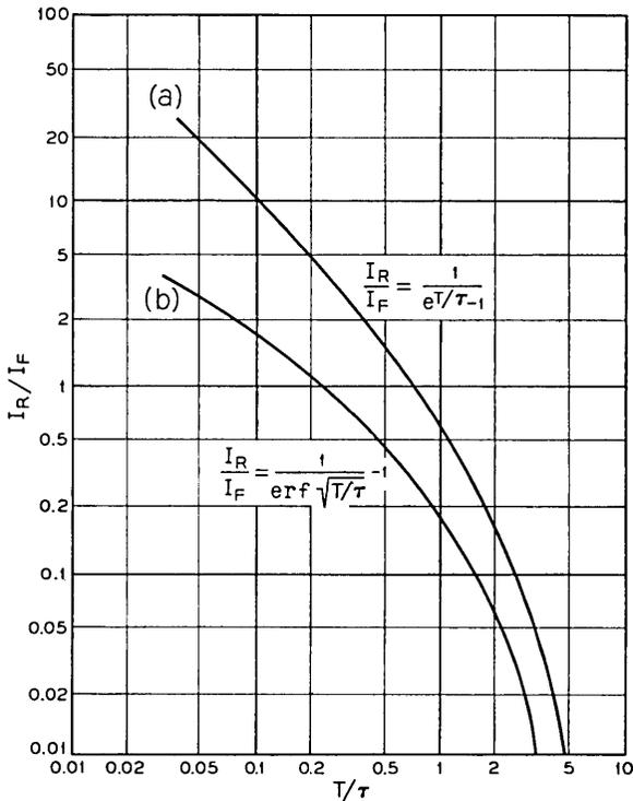
Fig. 11—Comparison of diode storage times as functions of the driving ratios. (a) Single lump model;  $T$  = time when charge is fully depleted. (b) Differential model;  $T$  = time when excess carrier density at  $x = 0$  reaches zero.
