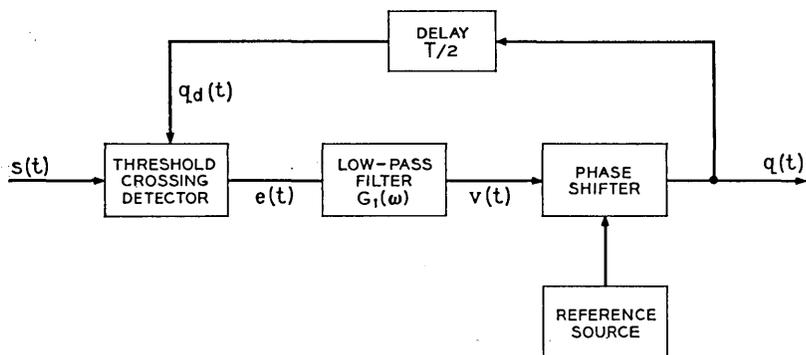
Fig. 1—Threshold crossing timing recovery system.
