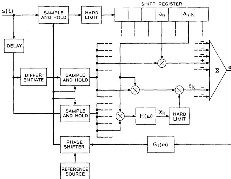
Fig. 5—Improved timing recovery system.
