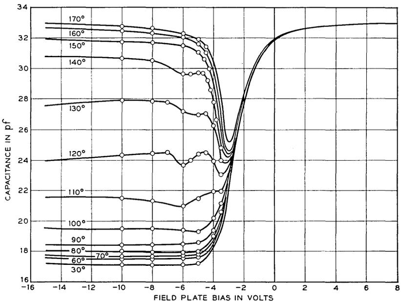
Fig. 2—Capacitance vs field plate bias measured at 6 kHz with temperature in  $^\circ\text{C}$  as parameter. Sample is *n*-type silicon oriented in the [100] direction. Field plate diameter is  $370\ \mu$ , donor density is  $1.17 \times 10^{16}\ \text{cm}^{-3}$ , and oxide layer capacitance is  $2.84 \times 10^{-7}$  farads/cm $^2$ .
