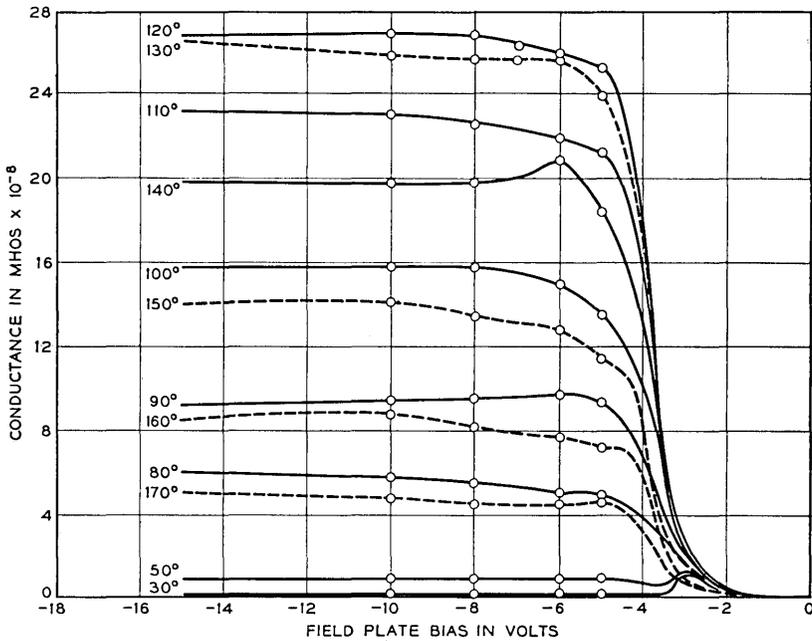
Fig. 3 — Equivalent parallel conductance vs field plate bias measured at 6 kHz with temperature in  $^{\circ}\text{C}$  as parameter. Sample is the same as in Fig. 2. Conductance is peaked at  $120^{\circ}\text{C}$ . Dotted lines are on high and solid lines on low-temperature side of peak.
