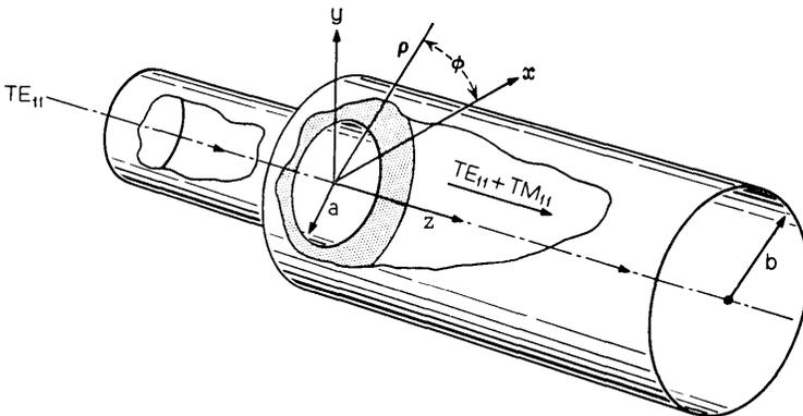
Fig. 9—TE<sub>11</sub> → TM<sub>11</sub> mode conversion at a discontinuity in a circular waveguide.
