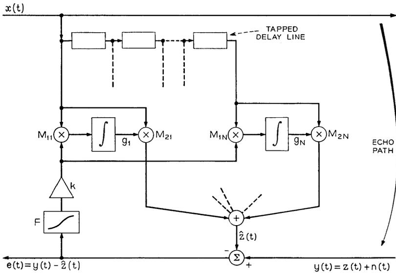
Fig. 2 — Schematic of the echo canceller using a transversal filter.
