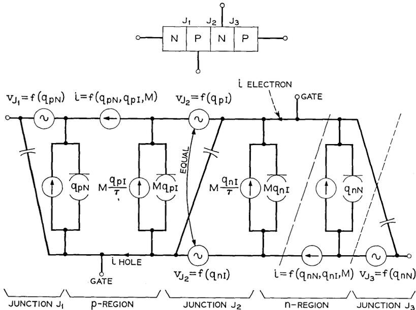
Fig. 25 — Charge-control model for npn device. The model for an npn-transistor with storage in the collector can be obtained from this model by omitting the part to the right of the dashed or the dotted line.
