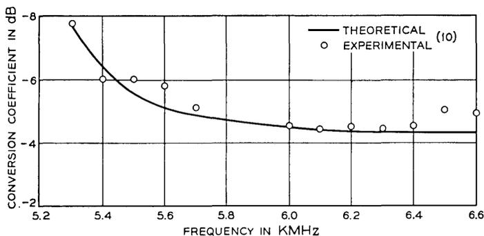
Fig. 10— $TE_{11} \rightarrow TM_{11}$  conversion coefficient of a step discontinuity in a circular waveguide.  $a = 1.05''$ ,  $b = 1.4''$ .
