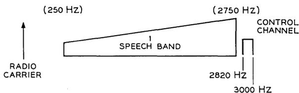
Fig. 4 — One-channel operation.
