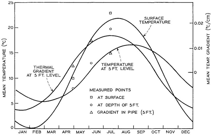
Fig. 3 — Mean annual change of the temperature at the surface and at a depth of 5 ft and the corresponding thermal gradient in an iron pipe at a depth of 5 ft as expected from data given in Ref. 7. The dots show values measured at Bell Telephone Laboratories, Holmdel, N. J. in 1966.
