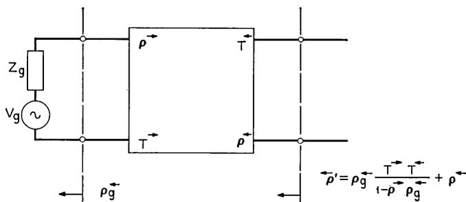
Fig. 2 — Effect of  $\rho_g^-$  on the output reflection of a stage.
