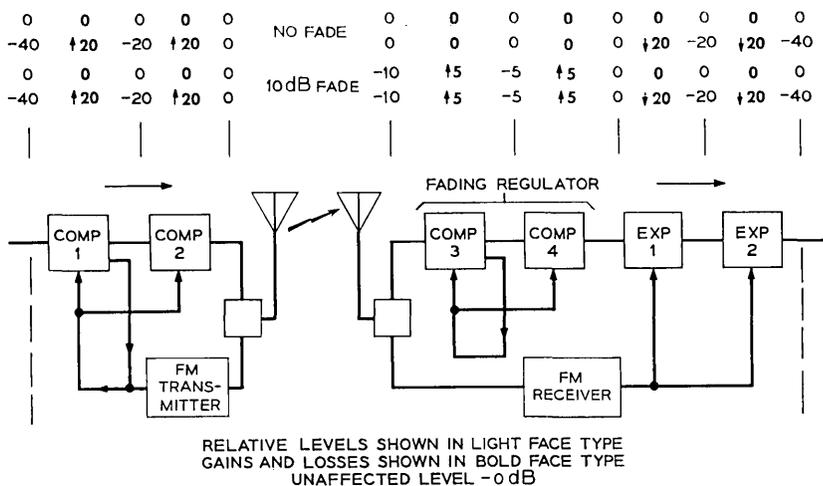
Fig. 23 — Example of CNL system gains and losses.
