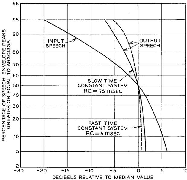
Fig. 16 — Input and output speech envelope peak distribution.
