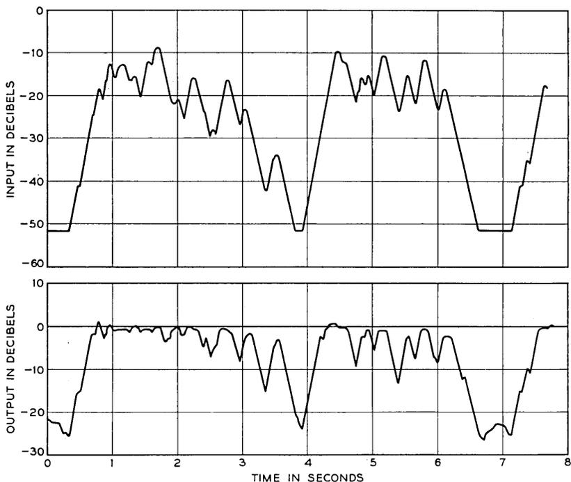
Fig. 17 — Chart record of compressor input and output— $RC = 20$  milliseconds; recorder integrating time—approximately 100 milliseconds.
