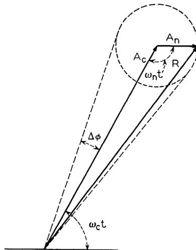
Fig. 25 — Phasor diagram, carrier and noise.
