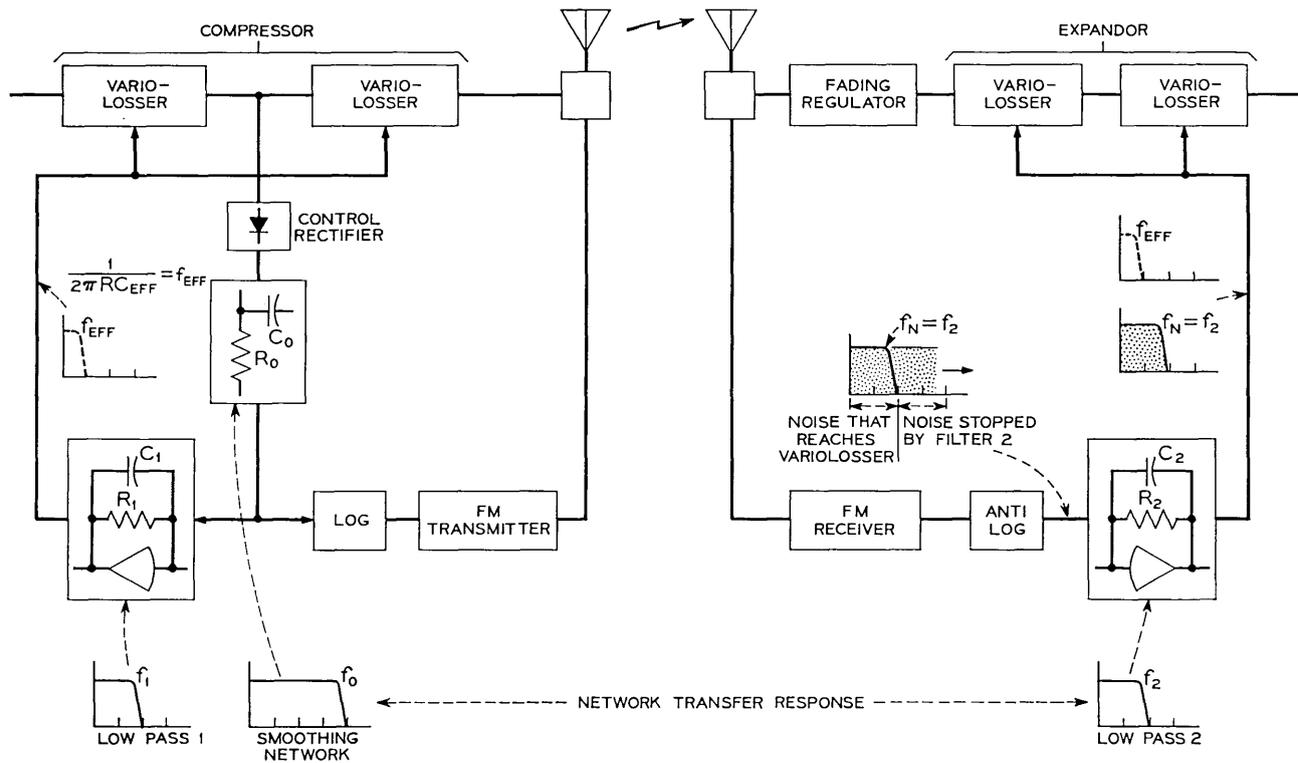
Fig. 7—Time constant determining elements of CNL system.
