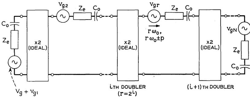
Fig. 4—Chain of doublers equivalent to the multiplier of order  $N = 2^r$  shown in Fig. 5.
