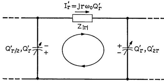
Fig. 21 — *S*th loop ( $r = 2^s$ ) of the chain of Fig. 20.
