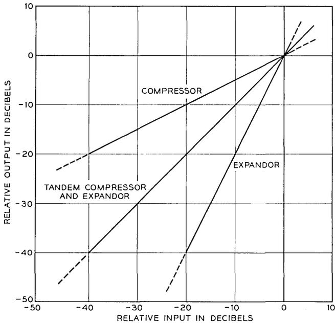
Fig. 22 — Input/output characteristic of 2:1 compandor.
