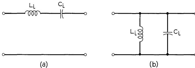
Fig. 8—Single-tuned resonant circuits.
