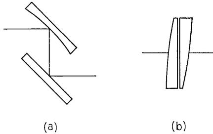
Fig. 6—Possible redirecting devices in a lens waveguide. (a) Mirror arrangement as proposed by Kompfner.<sup>2</sup> (b) Rotatable split lens which contains a variable prism.
