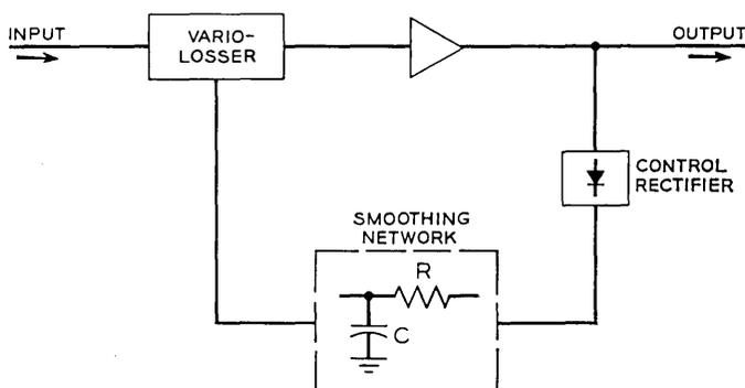
Fig. 10 — Simple model of 2:1 compressor.
