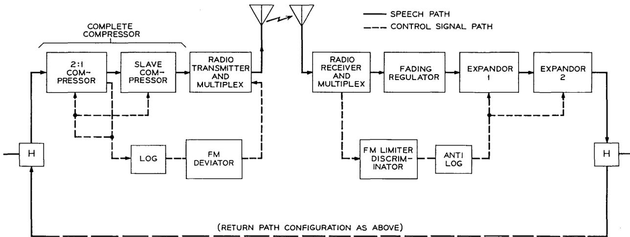
Fig. 3 — Constant net loss radiotelephone system (simplified).
