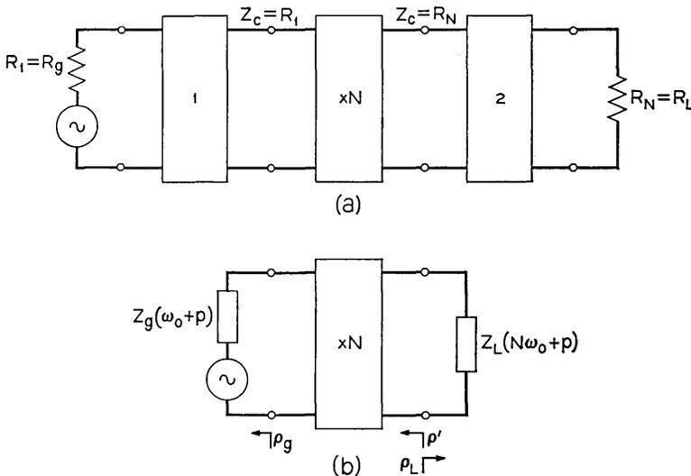
Fig. 3 — Multiplier connected between two stages.
