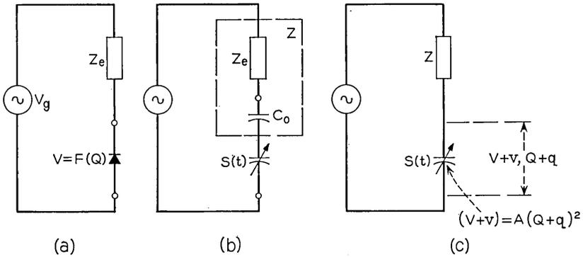
Fig. 7 — Equivalent circuit of the frequency multiplier.
