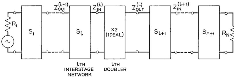
Fig. 7—Schematic representation of the chain of doublers equivalent to the multiplier of order  $N = 2^n$ .
