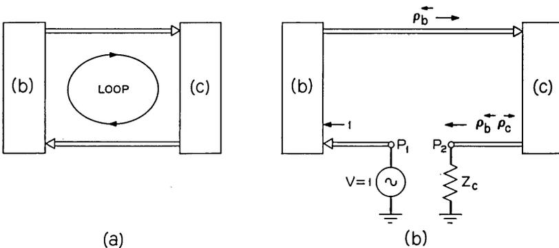
Fig. 1 — "Loop transmission" at the interconnection between two stages.
