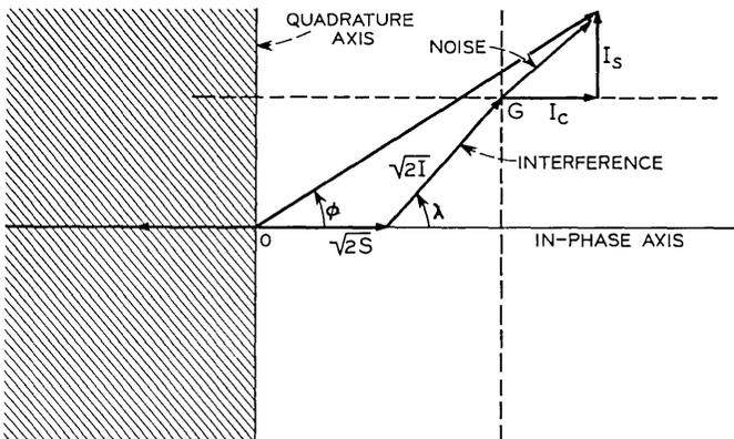
Fig. 3—Phasor representation of CPSK signals for  $m = 2$ .  $I_c$  and  $I_s$  are the in-phase and quadrature components of gaussian noise corrupting the desired received signal.
