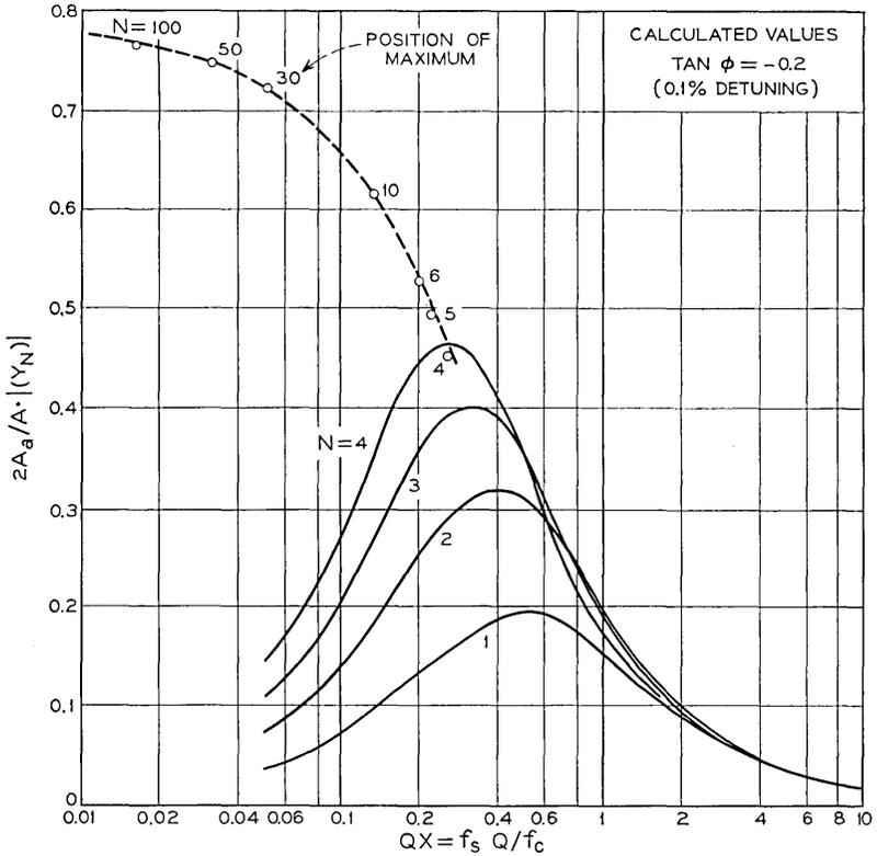
Fig. 14 — Calculated spectra of timing noise caused by tank circuit detuning.
