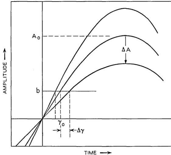
Fig. 7— Amplitude-to-phase conversion in trigger with offset bias.
