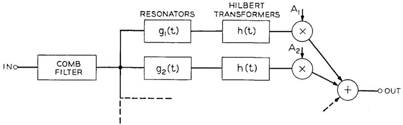
Fig. 4—Frequency sampling filter with separate Hilbert transformers.
