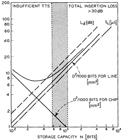
Fig. 4—For a delay line consisting of sodium-potassium niobate transducers attached to a Bausch & Lomb T-40 glass delay medium and  $f_o = 100$  MHz: the loss in the delay medium  $L_d$ , the latency time  $t_L$ , the combined endface area of the delay line, silicon chip area both per 1000 bits, and their sum. Outside the shaded region either the loss is too high or the triple travel suppression too low.
