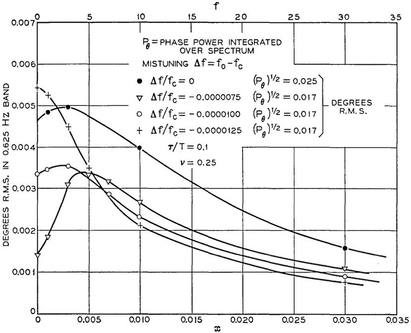
Fig. 22 — Spectrum of phase noise for rectangular pulse.
