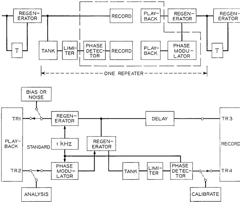
Fig. 24 — Block diagram of simulation of chain of regenerative repeaters. Part within dashed section at top is redrawn at bottom.
