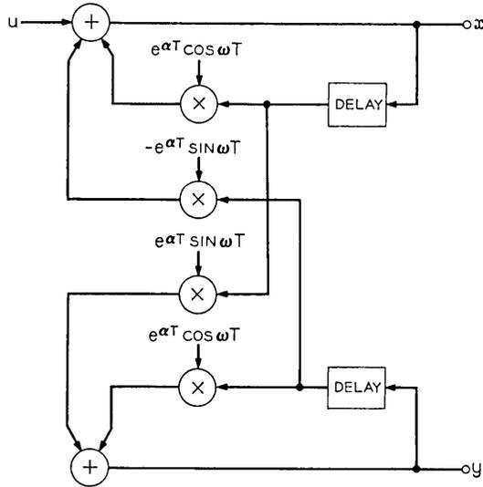
Fig. 7—Expanded flow chart for complex number resonator.
