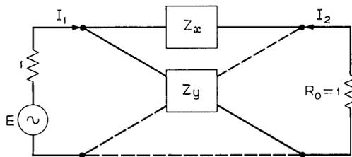
Fig. 1 — General constant resistance lattice network.
