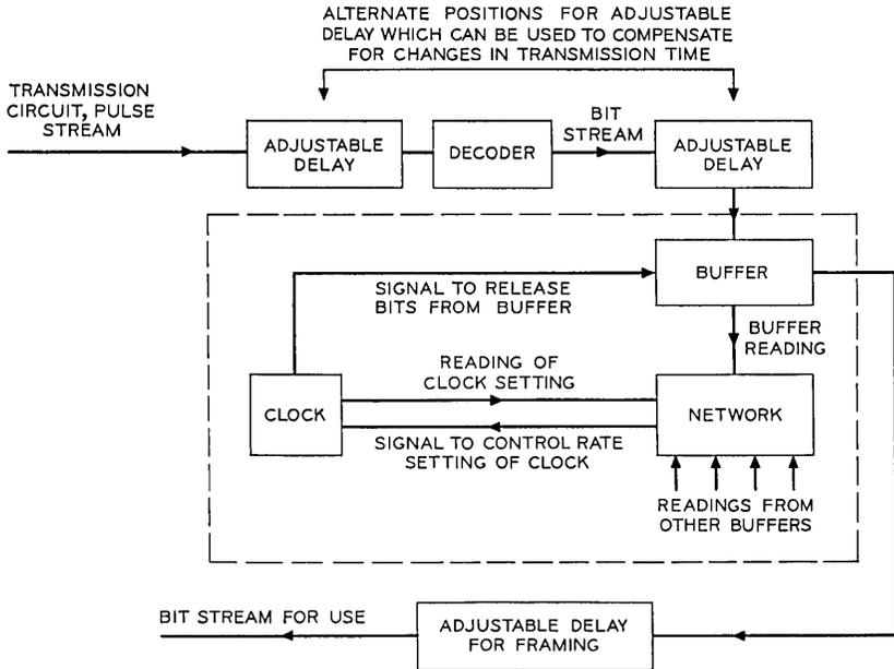
Fig. 2 — Block diagram showing components used in synchronization.
