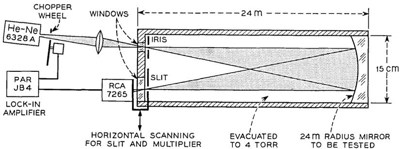
Fig. 1 — Setup to measure the scattering under vacuum.
