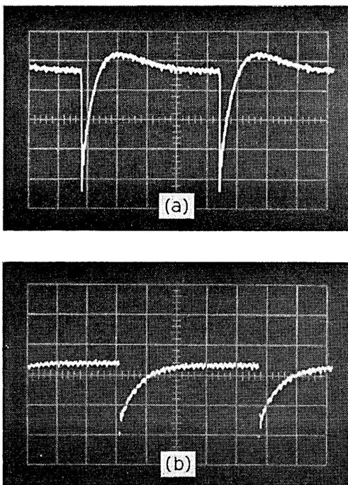
Fig. 39—Photographs of oscilloscope traces—Phase deviation of recovered fundamental pulse rate for pattern of 239 pulses, 1 space, with (a) tank circuit mistuning, (b) amplitude to phase conversion by means of trigger offset.
