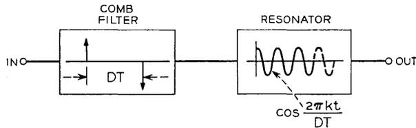
Fig. 2 — Comb filter followed by cosine resonator.
