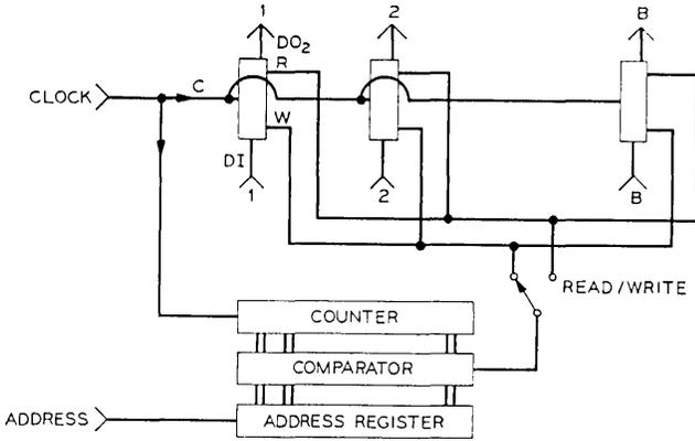
Fig. 6 — Bit-parallel, word-serial organization of B storage loops.
