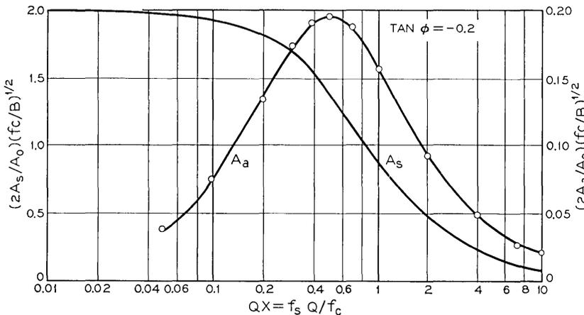
Fig. 8—Amplitude spectra of symmetrical ( $A_s/A$ ) and antisymmetrical ( $A_a/A$ ) side frequencies caused by tank mistuning (calculated).
