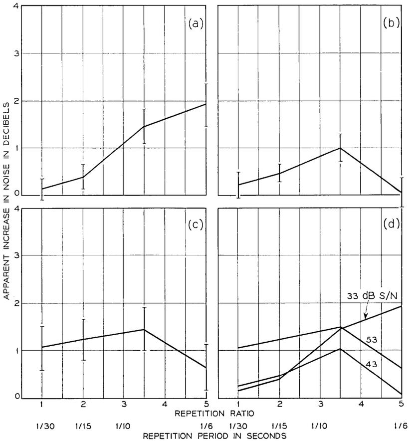
Fig. 3 — Interlaced scanning: (a) 33 dB signal-to-noise ratio; (b) 43 dB signal-to-noise ratio; (c) 53 dB signal-to-noise ratio; (d) combined results.
