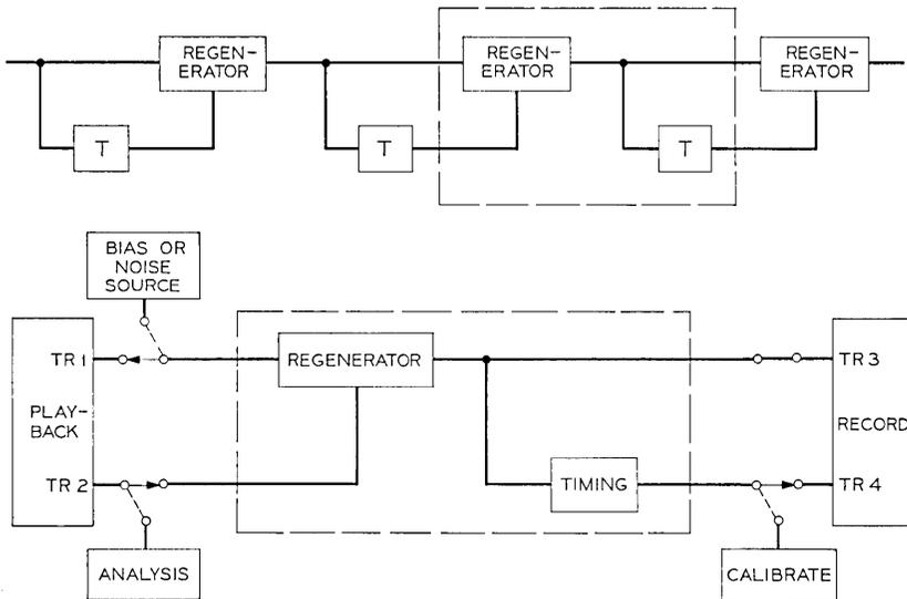
Fig. 1—Simulation of regenerative repeater chain.
