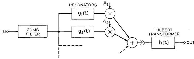
Fig. 3 — Frequency sampling filter, followed by Hilbert transformer.
