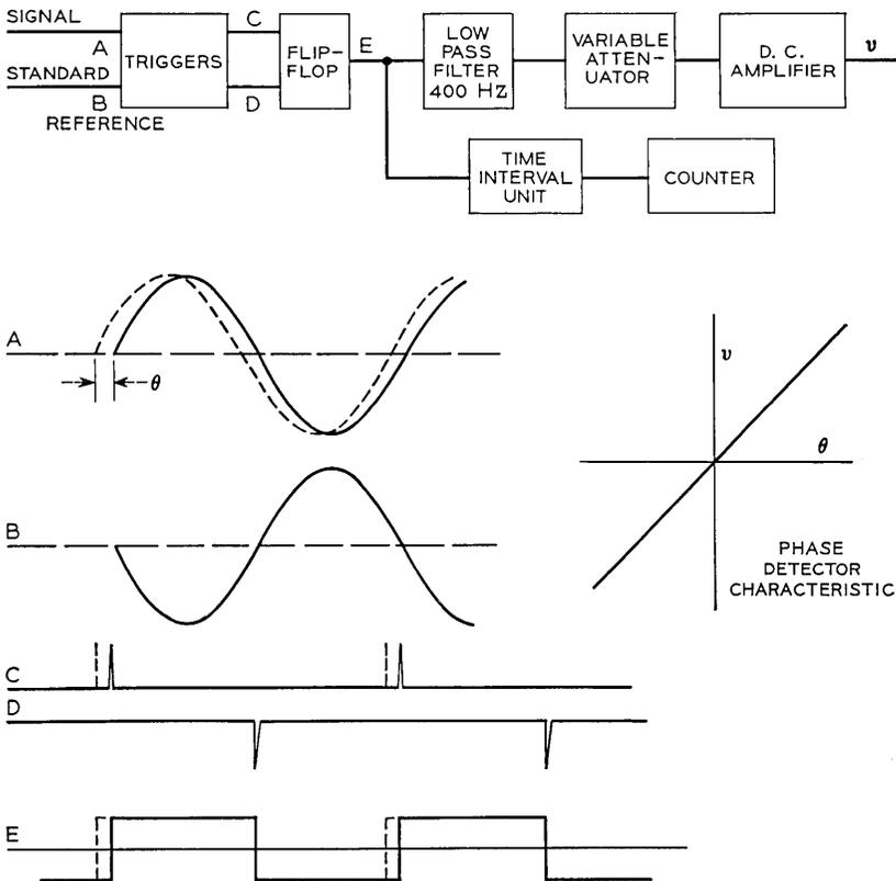
Fig. 26 — Block diagram and operation of phase detector.
