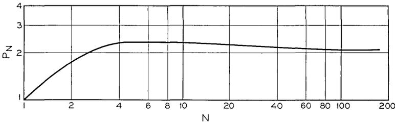
Fig. 15—Calculated total timing noise caused by tank circuit mistuning as a function of the number  $N$  of like repeaters in a chain.
