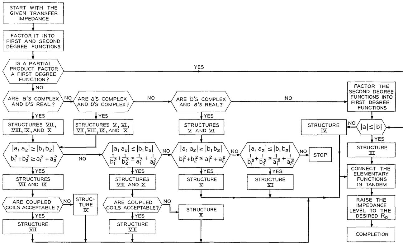
Fig. 8—Flow chart for synthesizing transfer impedance functions with constant resistance lattice networks.
