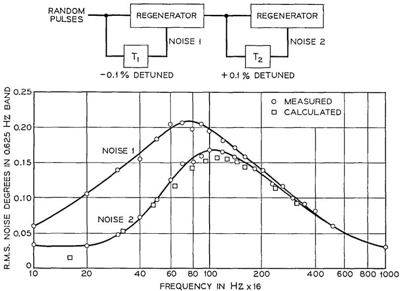
Fig. 30—Spectra of timing noise at two successive regenerative repeaters with oppositely detuned timing tanks.
