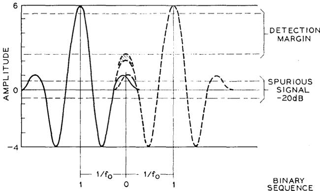
Fig. 3—Output signal from a delay line when rectangular pulses of duration  $1/2f_0$  are applied to its input. The worst case for detection is obtained when such pulses are entered at the rate  $f_0/2$  representing a binary 1-0-1 sequence as shown; since the outermost sidelobes of the nearest neighbors will fill in the “zero” slot between “one” pulses, this creates intersymbol interference. A spurious signal at a -20 dB level further reduces the detection margin to the one shown.
