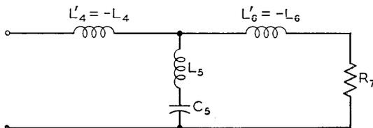
Fig. 6—Cross arm  $z_v$  for structure VIII of Fig. 2. ( $L$ 's,  $C_s$  and  $R_7$  are same as for Fig. 4.)
