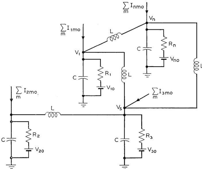
Fig. 5 — Interconnected nodes of electric analog.
