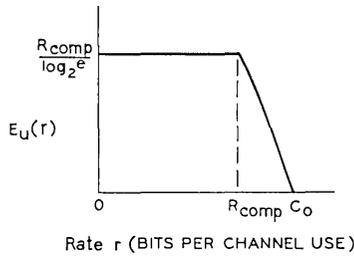
Fig. 6 — Sequential code error exponent  $E_u(r)$  for a typical DMC.
