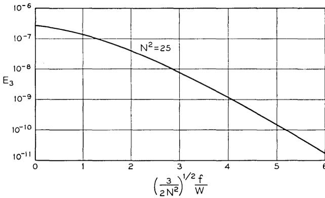
Fig. 14 — Parameter  $E_3$  as a function of  $(\frac{3}{2N^2})^{1/2} \frac{f}{W}$ , with  $N^2 = 25$ .
