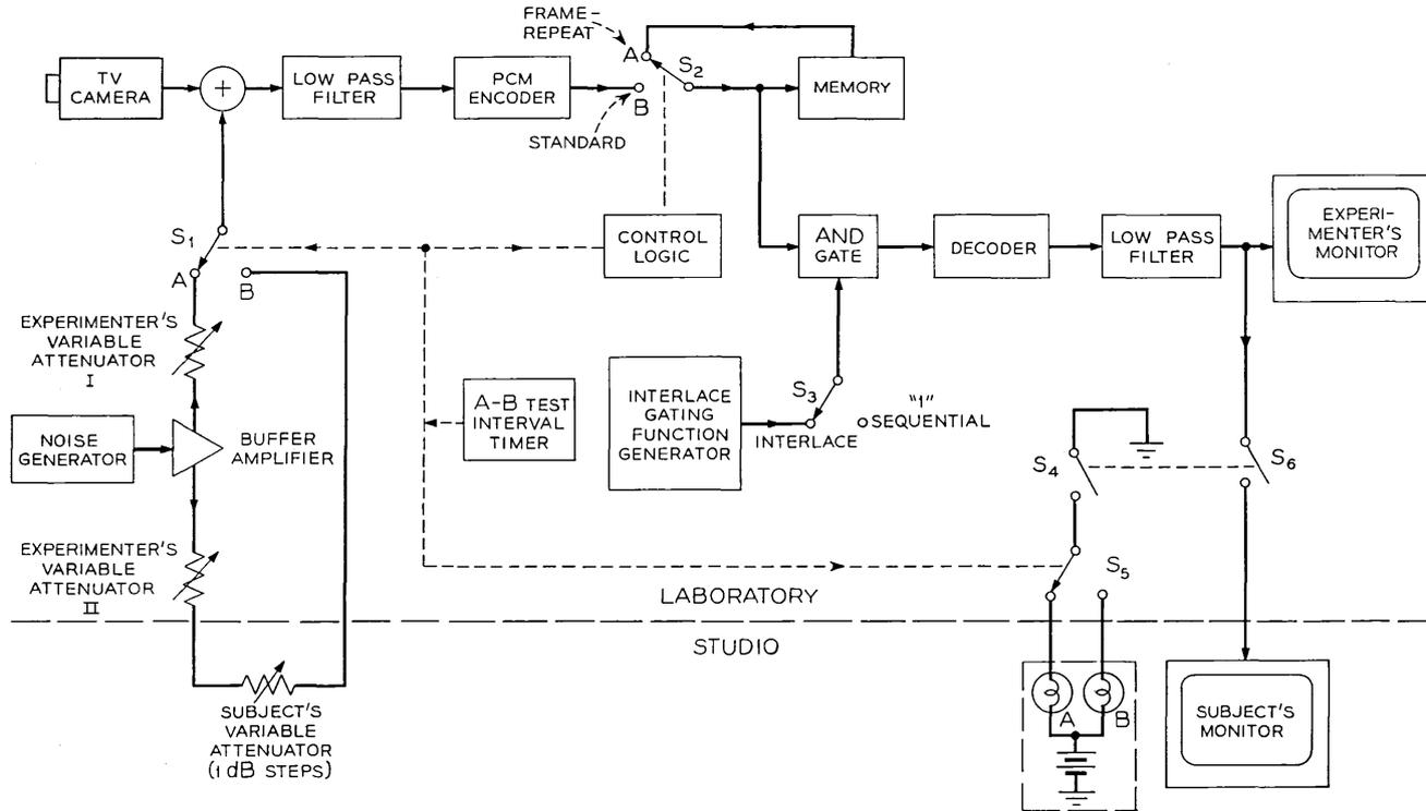
Fig. 4 — Block diagram of the experimental equipment.
