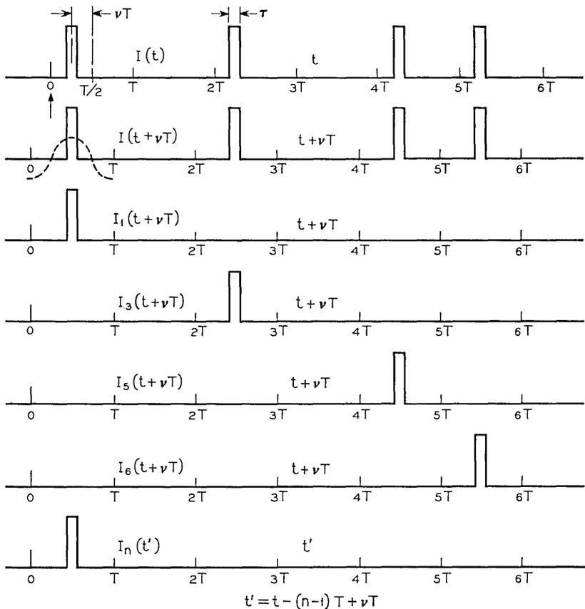
Fig. 19—Representation of pulse train for Fourier analysis.
