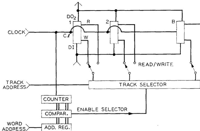
Fig. 5 — Bit-serial, word-serial organization of B storage loops as in Fig. 1.
