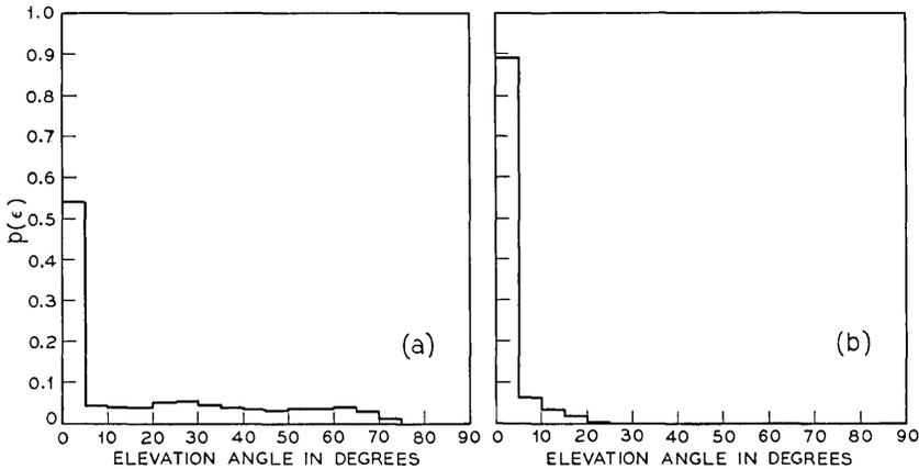
Fig. 12—Interference density vs. elevation angle into CCIR reference system centered at (a) 20° latitude and (b) 70° latitude. Satellite spacing = 6°.
