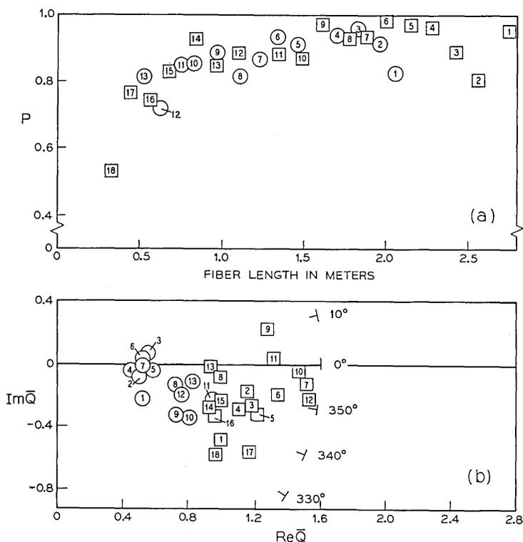
Fig. 9—Analyses of the states of polarization along two different  $13\mu\text{m}$  unclad fibers ( $\Delta = 2.44\%$ ): (a)  $p$  vs fiber length, and (b)  $\bar{Q}$  is plotted in the complex plane with fiber length as the parameter. The points are numbered sequentially to correspond to the points of (a) and Figure 8a, b reading from right to left.
