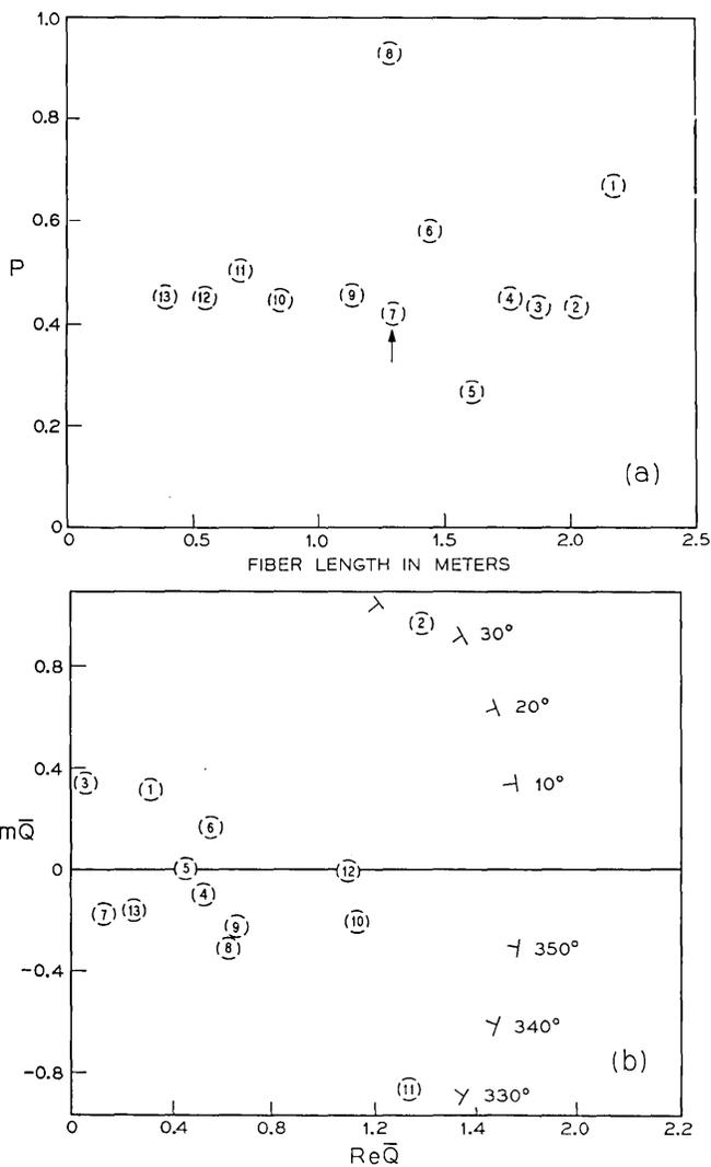
Fig. 10—Analyses of the states of polarization along a 3 μm clad fiber ( $\Delta = 0.824\%$ ): (a)  $p$  vs fiber length. The notation  $\uparrow$  refers to a bright spot indicative of a gross defect within the core or at the core cladding interface. (b)  $\bar{Q}$  is plotted in the complex plane with fiber length as the parameter. The points are numbered sequentially to correspond to the points of (a) and Figure 8c reading from right to left.
