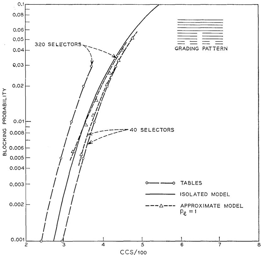
Fig. 7—Load-loss relations for a 19-trunk graded multiple.
