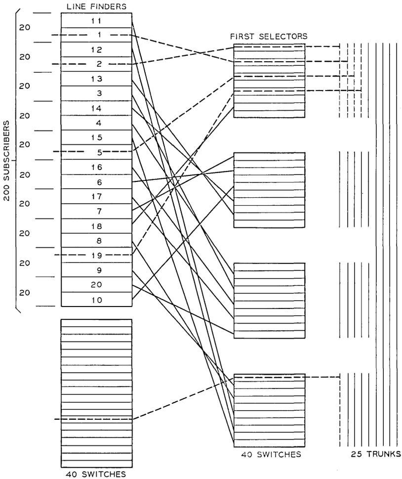
Fig. 1—Inherent load-balancing.
