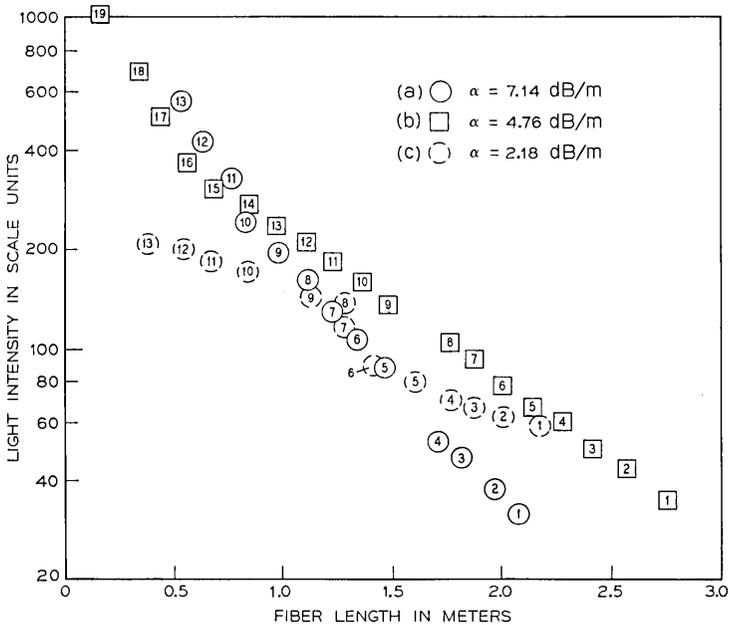
Fig. 8—(a, b) Transmission loss measurements along two different  $13 \mu\text{m}$  unclad fibers immersed in oil ( $\Delta = 2.44\%$ ). (c) Transmission loss measurements along a  $3 \mu\text{m}$  clad fiber.
