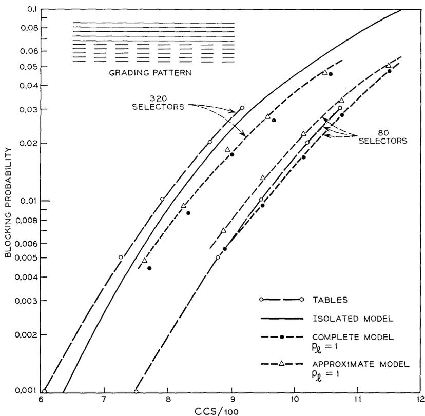
Fig. 4—Load-loss relations for a 45-trunk graded multiple.
