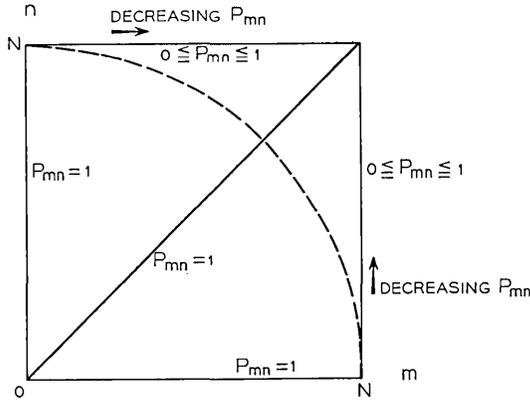
Fig. 11—Values of  $p_{mn}$  are shown projected onto the  $m - n$  plane. If  $N \rightarrow \infty$  then the  $N \times N$  square domain of definition for  $p_{mn}$  may be replaced by the dashed circle of radius  $N$ .
