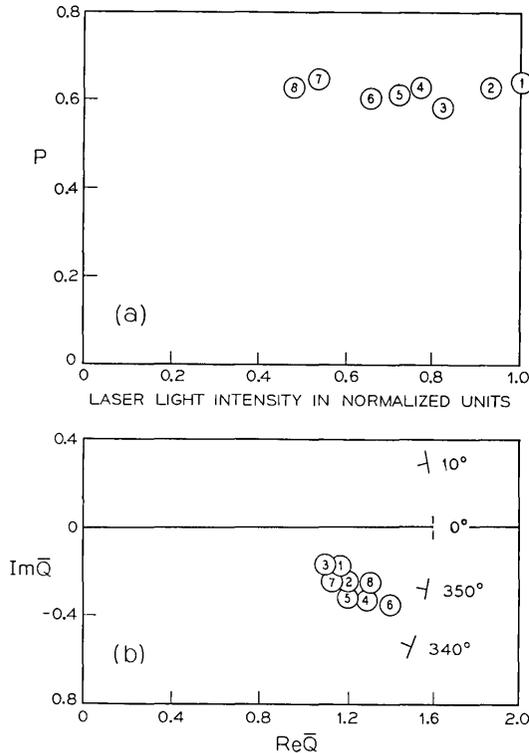
Fig. 7—The state of polarization of a  $28\mu\text{m}$  unclad fiber ( $L = 30 \text{ cm}$ ,  $\Delta = 2.44\%$ ) analysed as a function of input power: (a)  $p$  vs normalized laser light power, (b)  $\bar{Q}$  is plotted in the complex plane with light power as the parameter. The points are numbered sequentially to correspond to the points of (a) reading from right to left.
