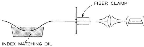
Fig. 2—Arrangement used to determine the refractive index of the unclad fiber core.
