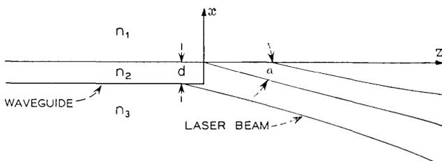
Fig. 3—Thin-film waveguide geometry used for the calculation.
