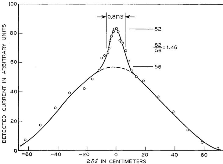
Fig. 6—Experimental results for a mode-locked He-Ne laser.
