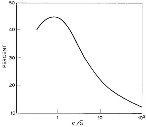
Fig. 7—Percent by which upper bound exceeds lower bound vs  $\sigma/\bar{G}$  for unilateral gain diode. Percent =  $((\Delta_U - \Delta_L)/\Delta_L) \times 100$ .
