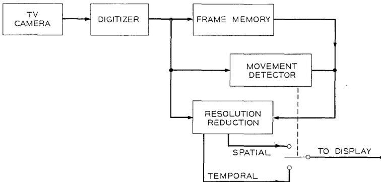
Fig. 1—System for resolution exchange.
