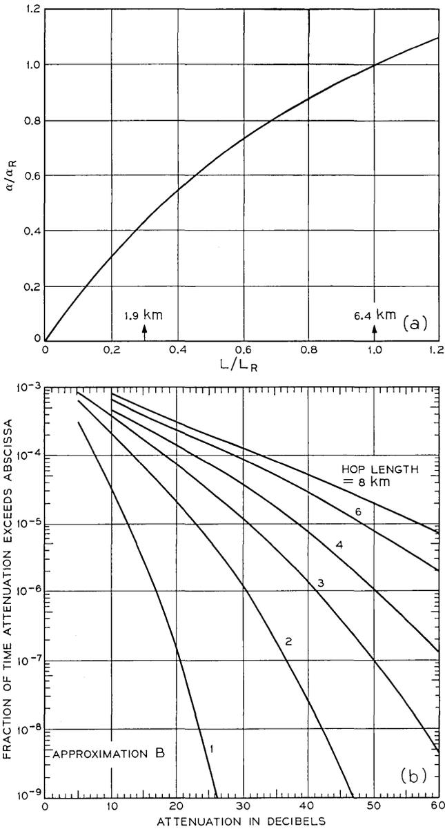
Fig. 3—(a) Attenuation as a function of hop length at constant probability using equation (2) with  $\rho = 0.543$ . (b) Probability distributions of rain attenuation with hop length as a parameter using approximating function B and equation (2) with  $\rho = 0.543$ .
