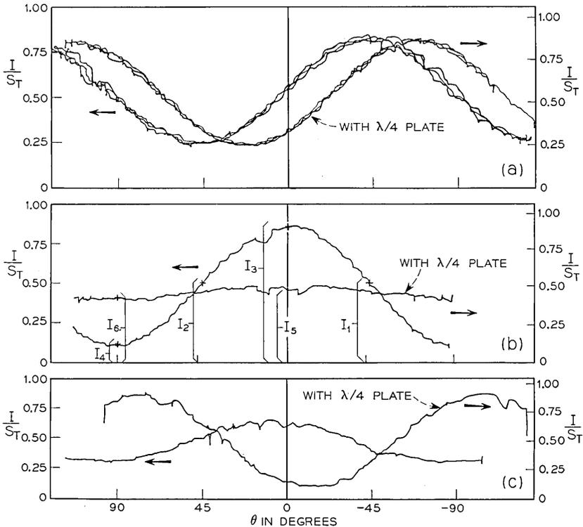
Fig. 6—Sample profiles of  $I/S_T$  vs  $\theta$  for partially polarized light leaving: (a) 19  $\mu\text{m}$  clad fiber ( $L = 301$  cm,  $\Delta = 0.824\%$ ), (b) 28  $\mu\text{m}$  unclad fiber ( $L = 238$  cm,  $\Delta = 2.44\%$ ), and (c) 28  $\mu\text{m}$  unclad fiber ( $L = 197$  cm,  $\Delta = 0.56\%$ ).
