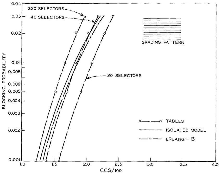
Fig. 5—Load-loss relations for the 11-trunk graded multiple.
