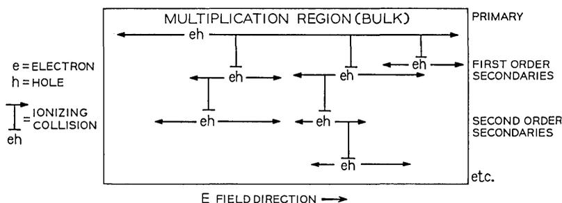
Fig. 1—Model of equal ionization device.
