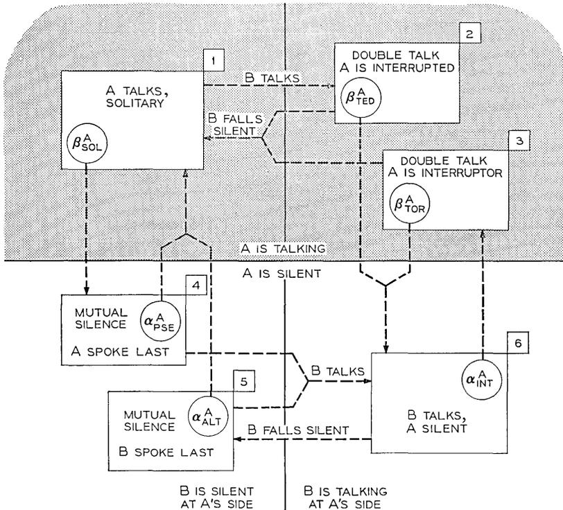
Fig. 2—The six-state model used in this study. Vertical transitions are due to Poisson processes at *A*'s side. Horizontal transitions, due to *B*, are in *A*'s external environment and are not generated by *A*'s model.
