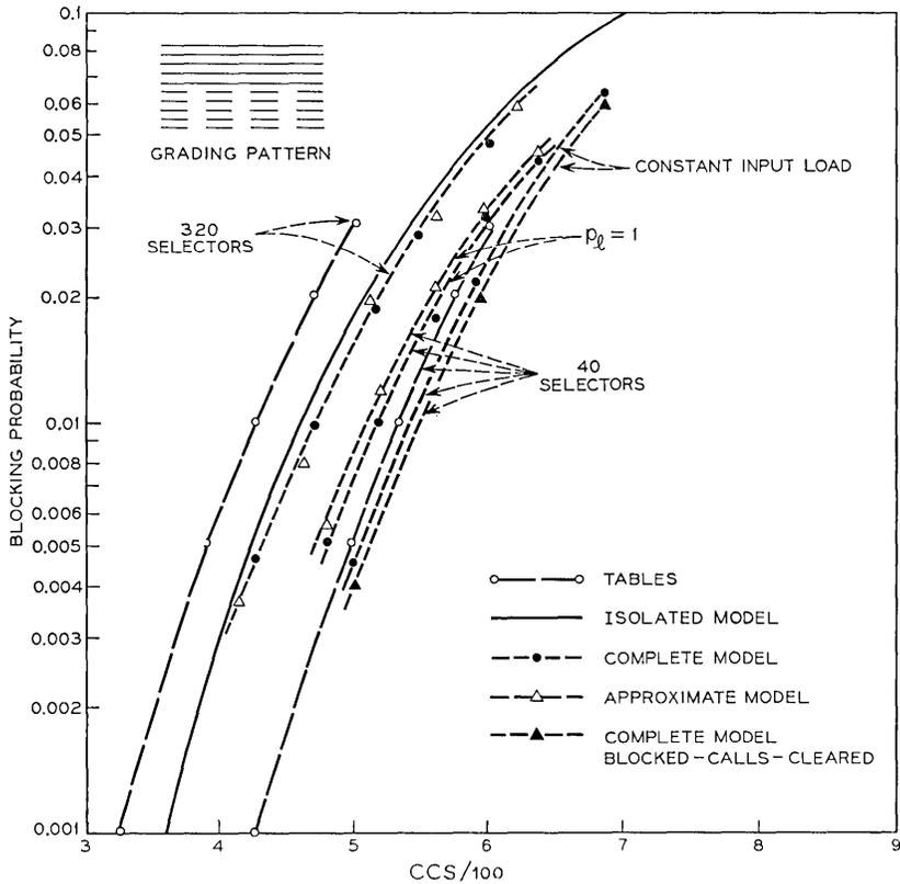
Fig. 3—Load-loss relations for a 25-trunk graded multiple.
