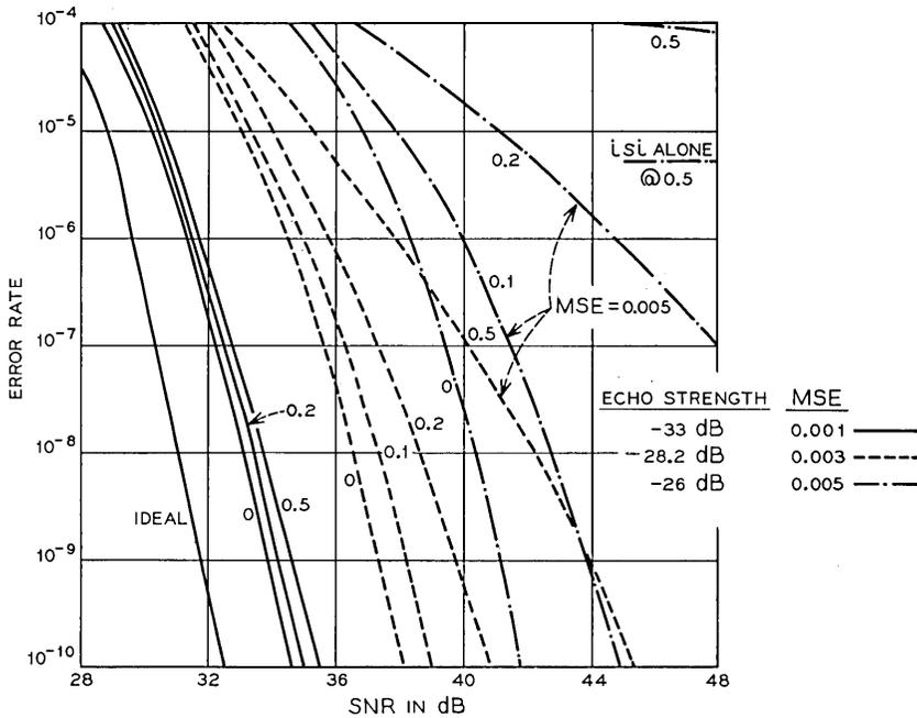
Fig. 7—Error rate vs SNR for single echo.
