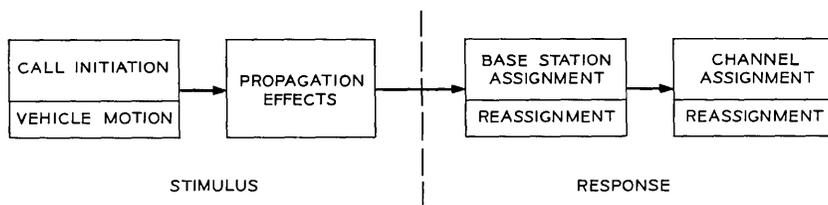
Fig. 3—Functions of a high-capacity mobile radio system.
