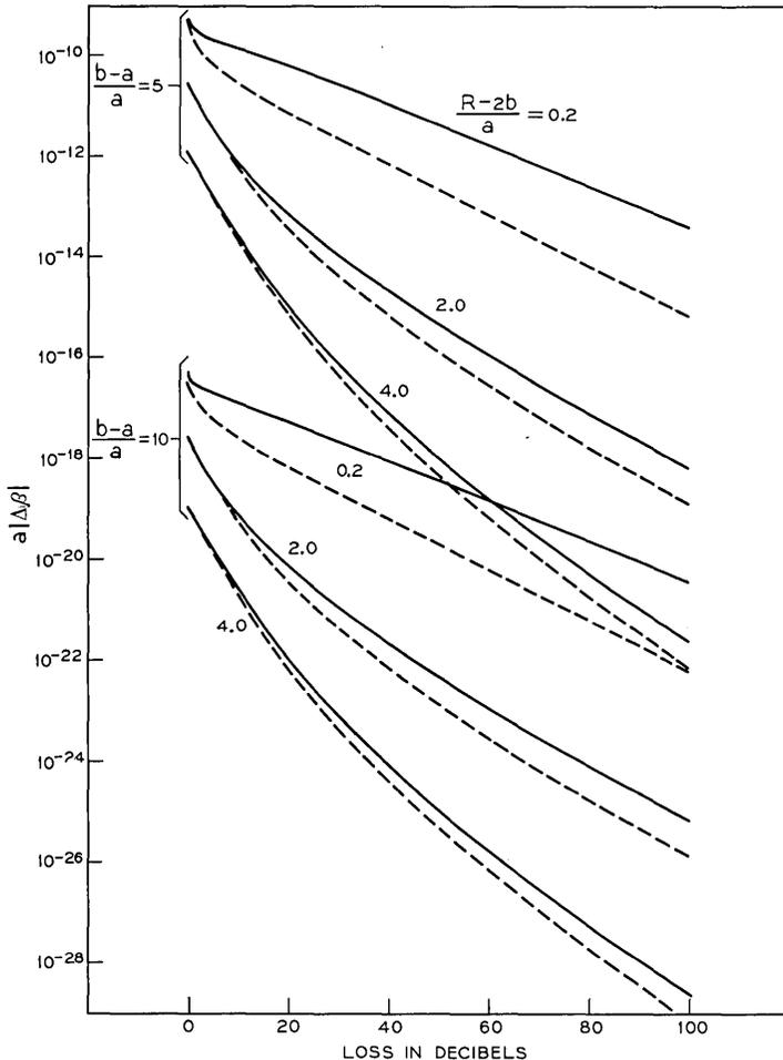
Fig. 4—Coupling of round fibers.  $a|\Delta\beta|$  is the coupling parameter of equations (60) and (61), the abscissa indicates the loss (in db) that a plane wave would experience in going from the boundary of one fiber to the boundary of the other fiber. The solid lines hold for horizontal polarization, equation (60), while the dotted lines apply to the case of vertical polarization, equation (61).  $n_m k a = 16$ ,  $\gamma a = 1.594$ ,  $n_c/n_m = 1.01$ ,  $\text{Re}(n_s) = n_m$ .
