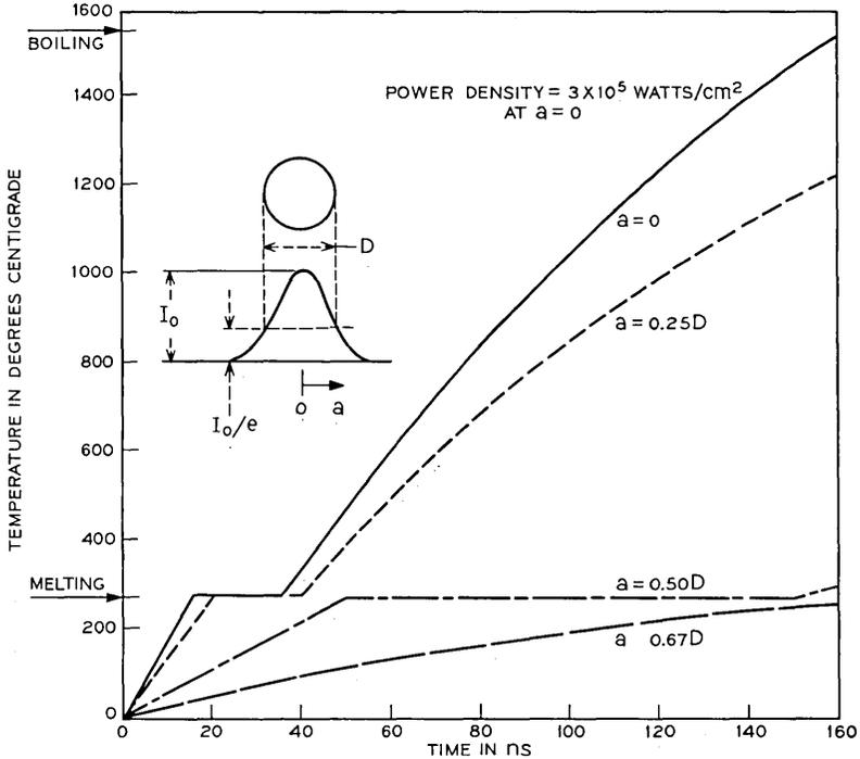
Fig. 6—Temperature distribution across the machine spot diameter.
