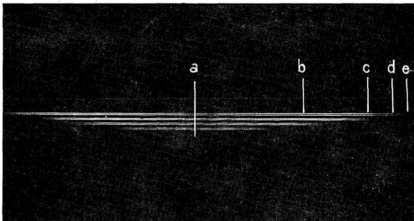
Fig. 8—Four sets of lines machined with different intensities.
