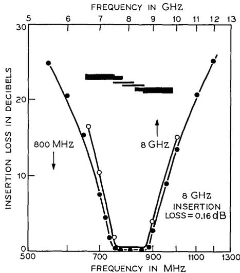
Fig. 8—Microstrip band-pass filter (results of scaling from 800 MHz to 8 GHz).
