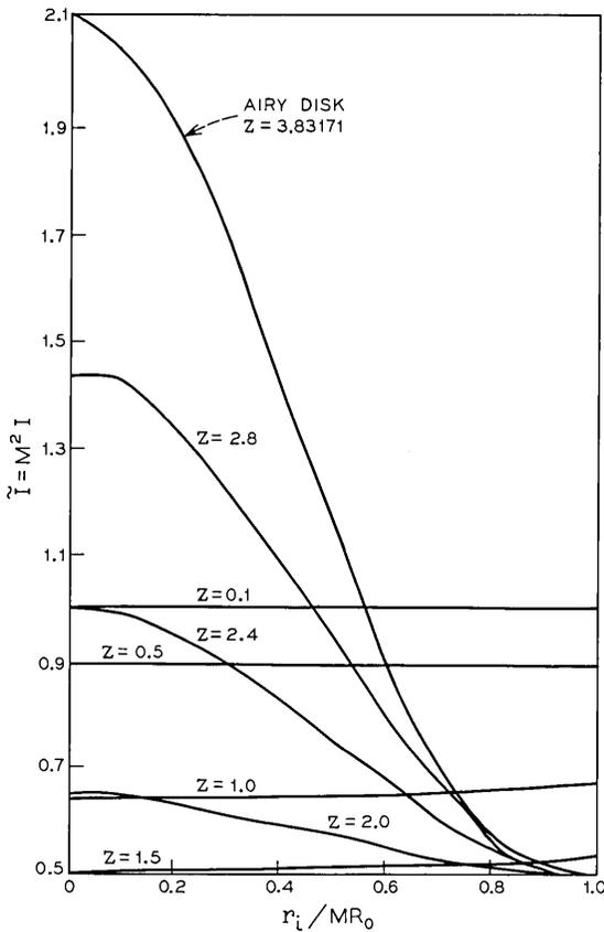
Fig. 2—Background intensity distributions for spot sizes less than or equal to the Airy disk ( $a = 1, \alpha = \pi/2$ ).
