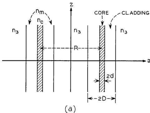
Fig. 2a—Sketch of two coupled cladded slab waveguides.
