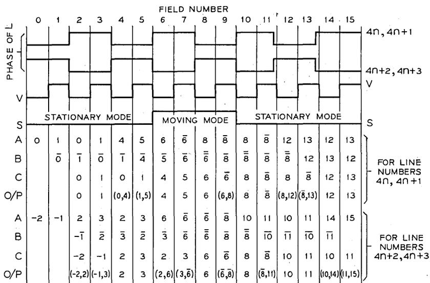
Fig. 3b—Waveforms *L*, *V*, and *S* and fields present at points *A*, *B*, *C* (Fig. 3a) and at the output for both sets of lines. In real time, waveform *L* switches at the line rate but is shown here as two waveforms, one for each set of lines switching at the frame rate.
