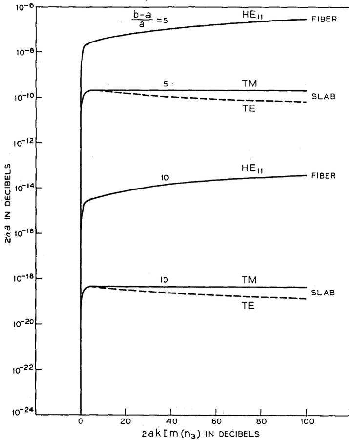
Fig. 7—Additional mode loss caused by the lossy surrounding medium. The abscissa indicates the loss (in db) that a plane wave would suffer by traveling a distance equal to the core radius in the surrounding medium.  $n_m k a = 16$ ,  $n_c/n_m = 1.01$ .
