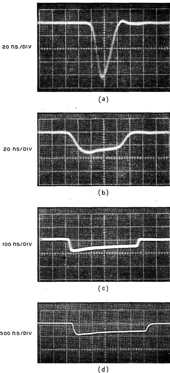
Fig. 13—Different light pulse durations obtained by the modulation system.
