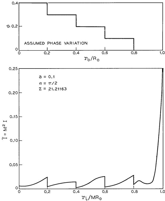
Fig. 14—Response to phase rings ( $\alpha = 0.1$ ,  $z = 21.21163$ ).
