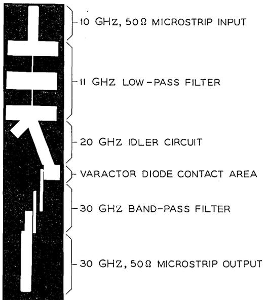
Fig. 1—Conductor pattern of hybrid integrated multiplier on silica substrate.
