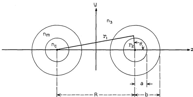
Fig. 3—Cross section of two coupled cladded fibers.
