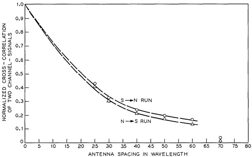
Fig. 4—The correlation coefficient of two base-station antennas broadside with the incoming wave vs antenna spacing for runs on Broadway, Keyport, N. J.
