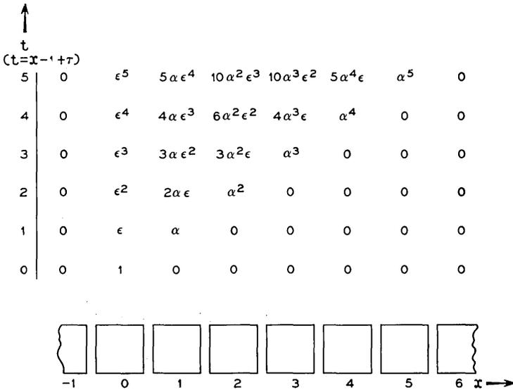
Fig. 2—Evolution of a unit charge initially in station  $x = 0$  at  $t = 0$ . A fraction  $\alpha$  of the charge is advanced per step and a fraction  $\epsilon$  remains behind.
