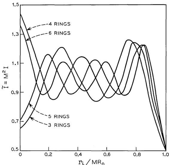
Fig. 3—Background intensity distributions for spot sizes larger than the Airy disk ( $a = 1, \alpha = \pi/2$ ).
