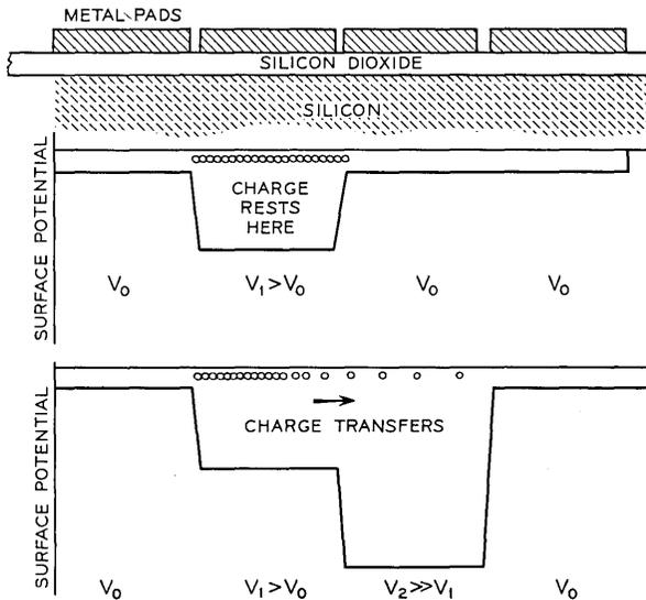
Fig. 1—A diagram of a CCD cross section and surface potential diagrams illustrating charge storage and charge transfer in CCD's.
