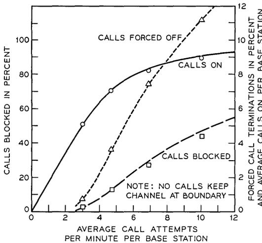
Fig. 14—Performance of a fixed-channel assignment system (flat loading).
