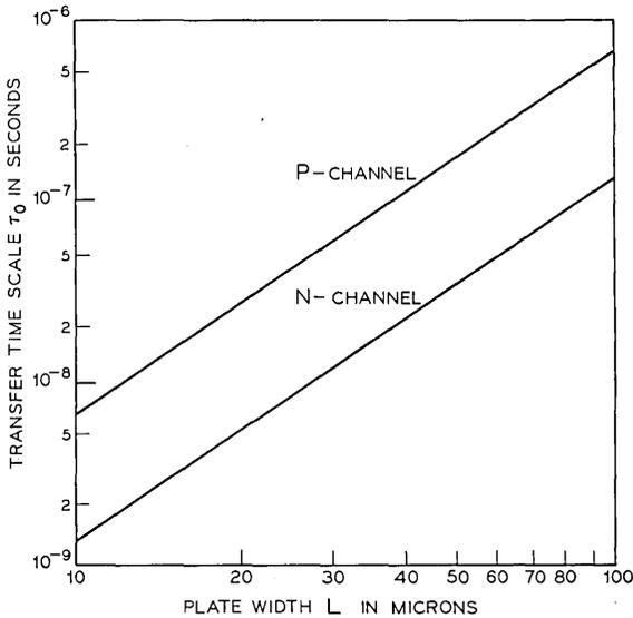
Fig. 8—A plot of the time scale factor  $\tau_0$  as a function of the CCD plate length  $L$ .
