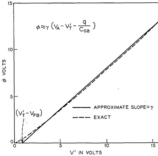
Fig. 2—The exact variation of deep depletion surface potential in an MOS with 1000Å of SiO<sub>2</sub> over a substrate with  $5 \times 10^{14}$  ionized impurities per cm<sup>3</sup>, and the linear approximation  $\Phi \propto \gamma V'$ .
