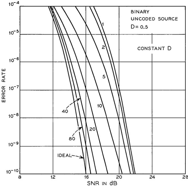
Fig. 8—Error rate for equal error samples.
