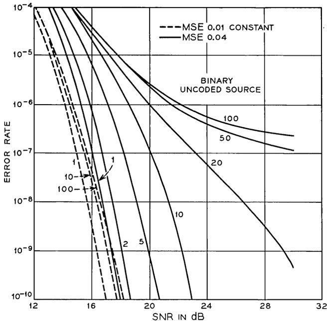
Fig. 9—Error rate for equal error samples.
