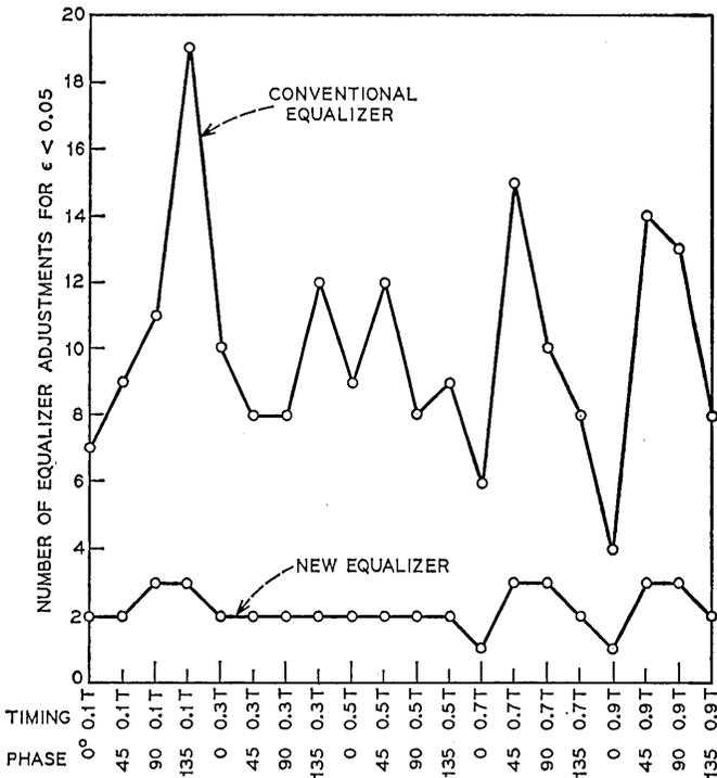
Fig. 7—Number of equalizer adjustments required to reduce the mean-square error to less than 0.05 for different timing and carrier-phase settings.
