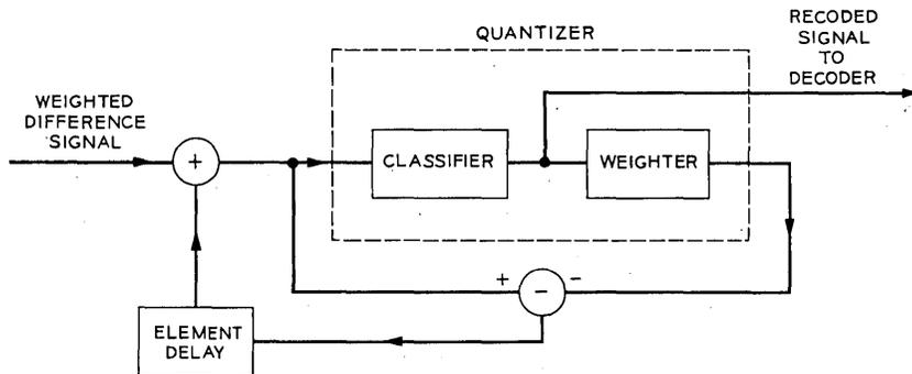
Fig. 4—Recoder to convert averaged weights to standard weights.
