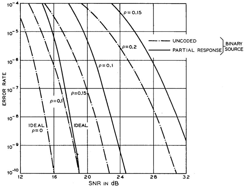
Fig. 5—Error rate vs SNR for timing error.
