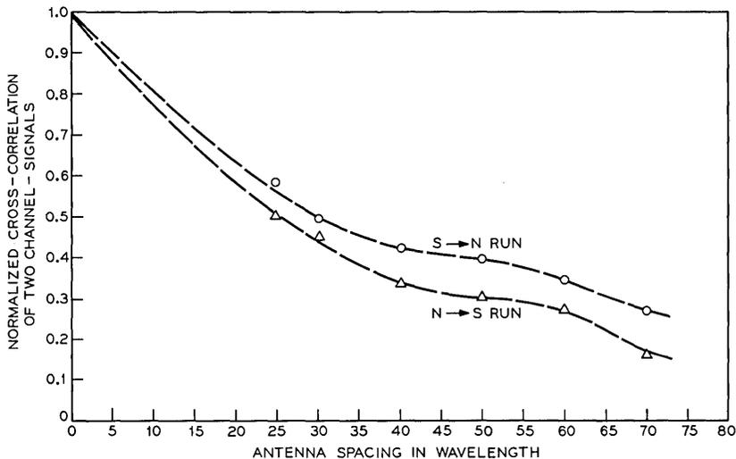
Fig. 2—The correlation coefficient of two base-station antennas broadside with the incoming wave vs antenna spacing for runs on Main St., Keyport, N. J.
