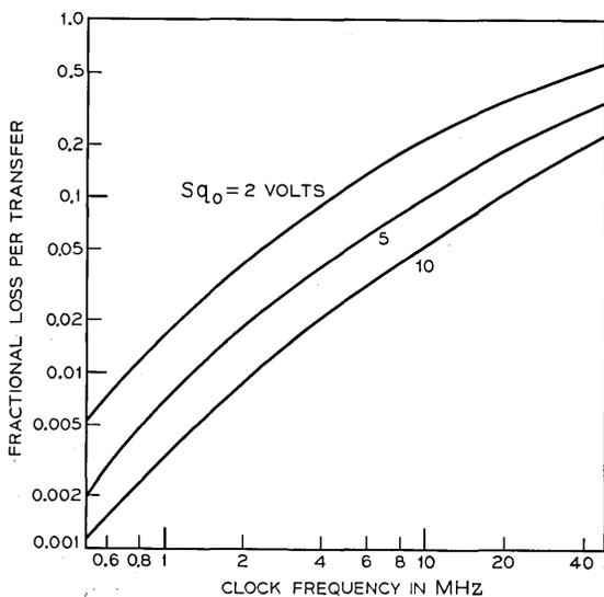
Fig. 9—The fractional loss per transfer of a P-channel 2-phase CCD, with a field-free length  $L$  of  $25 \mu\text{m}$ , plotted against clock frequency with the initial one signal as a parameter. The ZERO's have no charge.
