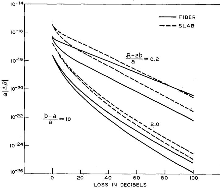
Fig. 6—Comparison between the coupling of round fibers and slab waveguides ( $a = d, b = D$ ). The parameter value  $\gamma a = 1.594$  is correct for the round fibers. It has also been used for the slab waveguides to enable a realistic comparison.  $n_m k a = 16, n_c/n_m = 1.01$ .
