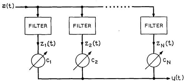
Fig. 3—Generalized equalizer structure.
