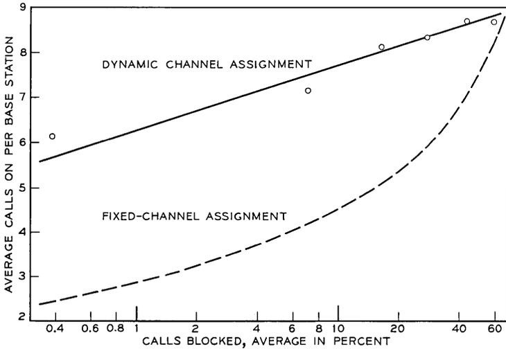
Fig. 19—Channel usage (peaked loading).
