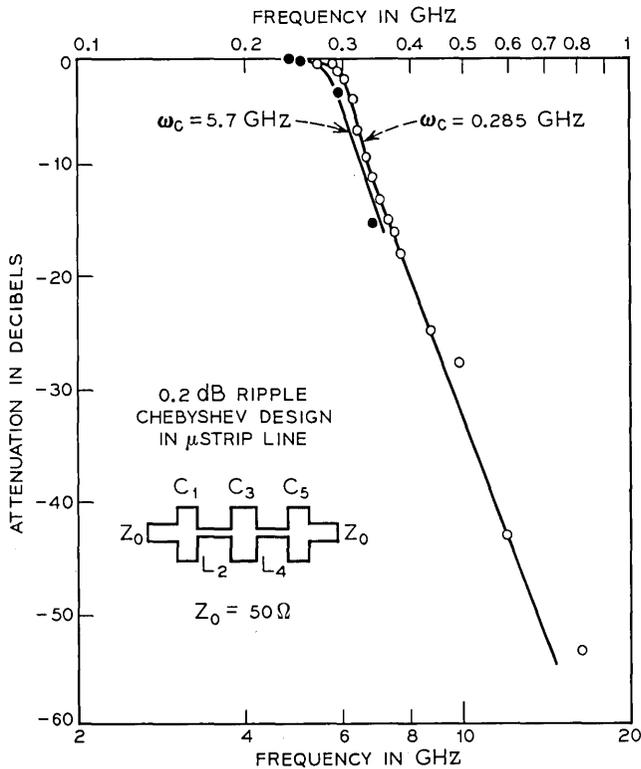
Fig. 5—5-element low-pass filter (results of scaling from 285 MHz to 5.7 GHz).
