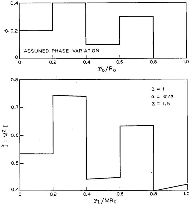
Fig. 13—Response to phase rings with alternating phase.
