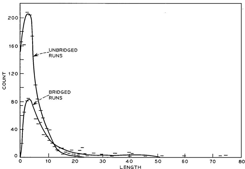
Fig. 10—The effect of raising the threshold from  $4/256$  to  $7/256$  on the runs and bridged-runs given in Figs. 7 and 9. Changes that equal or exceed the threshold are counted.
