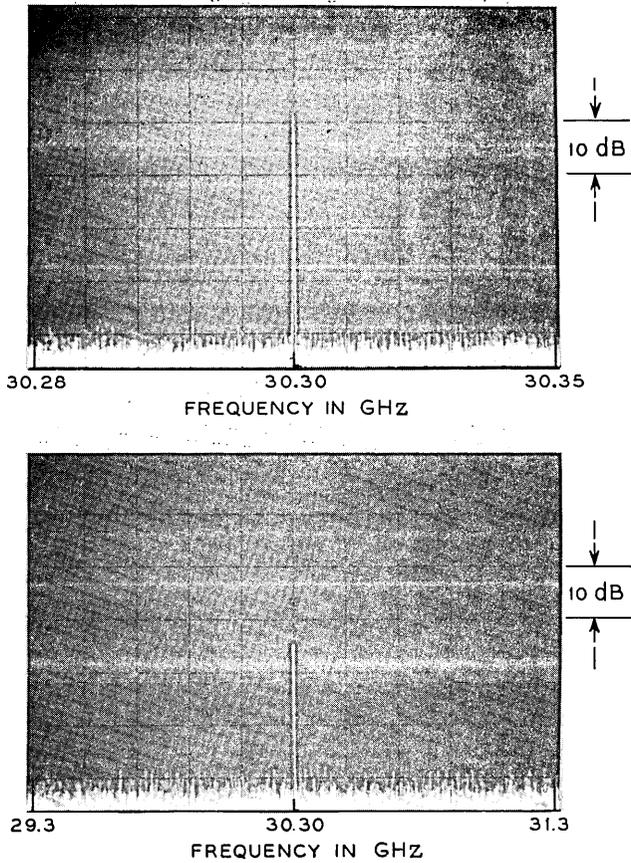
Fig. 5—Output spectrum of multiplier from 29.3 to 31.3 GHz.
