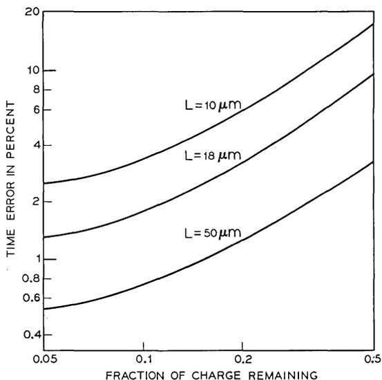
Fig. 15—An illustration of the effect of limiting the carrier velocity at  $x = L$  to  $10^7$  cm/s, expressed as an error between the time predicted in the idealized case and the time in the velocity-limited case.
