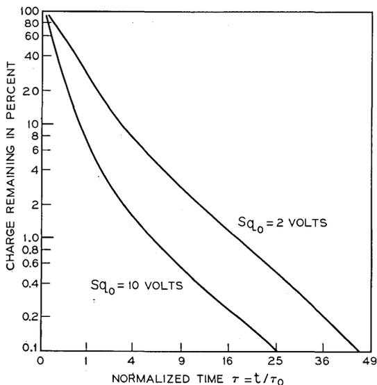
Fig. 6—The fraction of the charge remaining under the first plate as a function of the normalized time  $\tau = t/\tau_0$ . The abscissa is plotted as  $\tau^{1/2}$ , which spreads the region where  $\tau < 1$ , and leads to straight lines over the transition portion of the characteristic.
