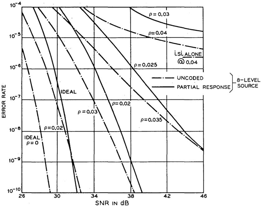
Fig. 6—Error rate vs SNR for timing error.
