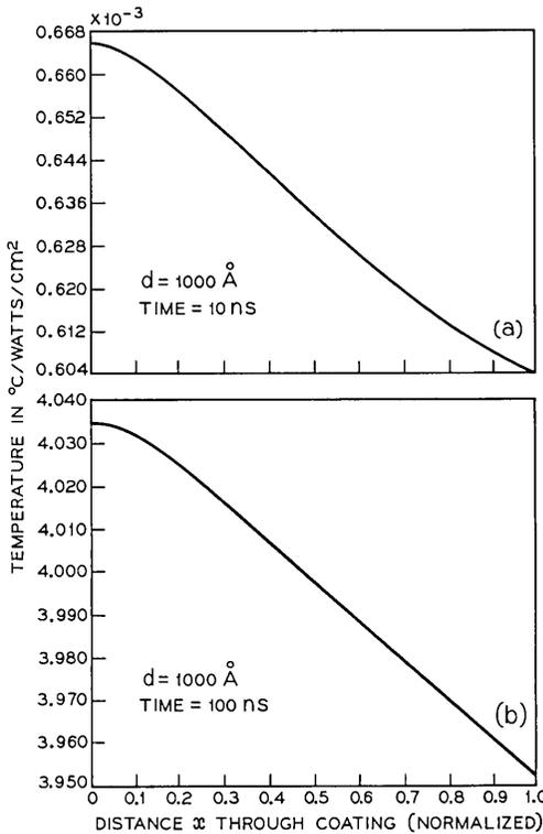
Fig. 4—Temperature distribution across 1000 Å of a bismuth film on mylar: (a) after 10 ns of front illumination; (b) after 100 ns of front illumination.
