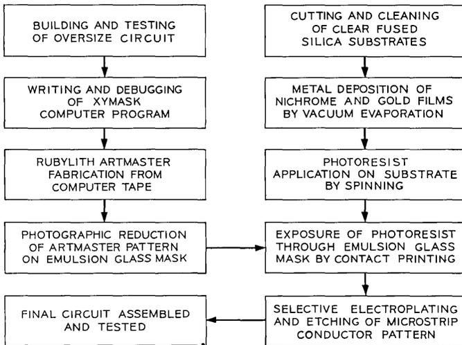
Fig. 2—MIC flow chart (detailed).
