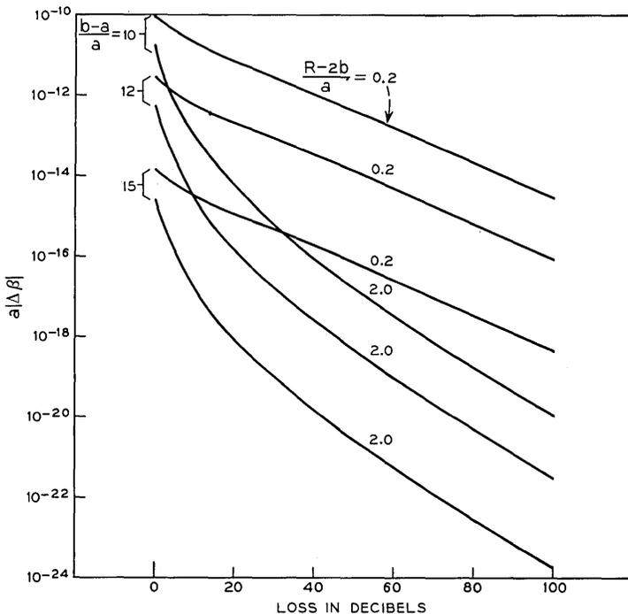
Fig. 8—Coupling of round fibers. Only the case of horizontal polarization is shown.  $n_m k a = 21$ ,  $\gamma a = 0.857$ ,  $n_c/n_m = 1.003$ .
