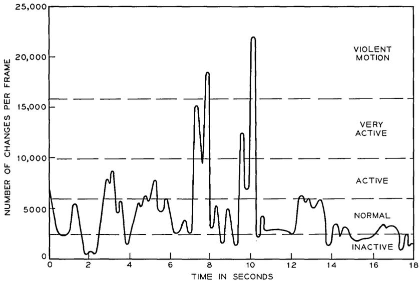
Fig. 2—The number of elements in a frame that change by more than  $3/256$  of maximum amplitude, plotted over a period of 18 seconds when there was a variety of motion. Each frame contains 67,000 elements of which 53,000 are visible.
