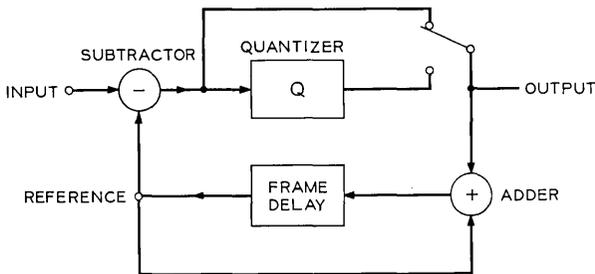
Fig. 13—The circuit used for measuring frame-to-frame difference.
