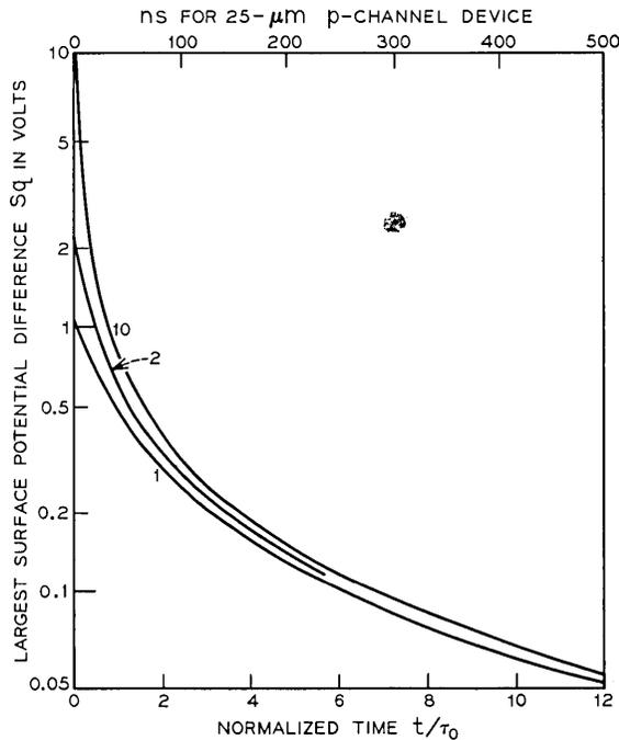
Fig. 13—The amplitude of the largest surface potential difference  $Sq(0)$  as a function of time. Two time-axes have been provided, the generalized  $\tau$ , and  $t$  for a 25- $\mu$ m p-channel device.
