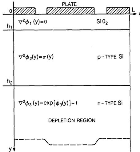
Fig. 1—A schematic diagram of a buried channel CCD.
