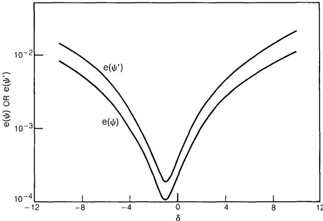
Fig. 3—Plots of  $e(\psi)$  and  $e(\psi')$  for a buried channel device with  $h_1 = 0.24$ ,  $h_2 = 12.24$ ,  $\bar{\sigma} = 20$ ,  $Q_{ss} = 0$ ,  $\eta = \frac{1}{3}$ , and  $V_0 = 0$  as functions of  $\delta$  for  $-10 \leq \delta \leq 10$ .
