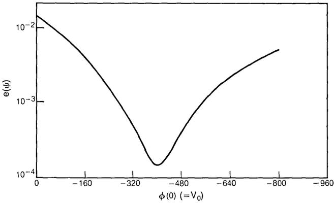
Fig. 9—Plot of  $e(\psi)$  for a buried channel device with  $h_1 = 0.24$ ,  $h_2 = 12.24$ ,  $c_s = 46$ ,  $Q_{ss} = 0$ ,  $\eta = \frac{1}{3}$  and  $\hat{R} = 39.66$  as a function of  $V_0$  for  $-800 \leq V_0 \leq 0$ .
