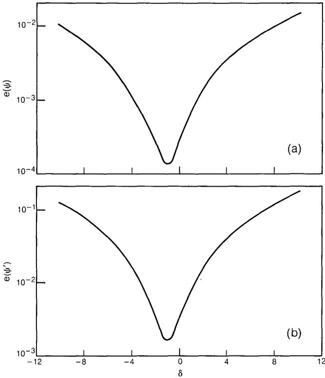
Fig. 5(a) and 5(b)—Plots of  $e(\psi)$  and  $e(\psi')$ , respectively, for a surface device with  $h_1 = h_2 = 0.24$ ,  $\sigma = 0$ ,  $Q_{ss} = 0$ ,  $\eta = \frac{1}{3}$  and  $V_0 = -160$  as functions of  $\sigma$  for  $-10 \leq \delta \leq 10$ .
