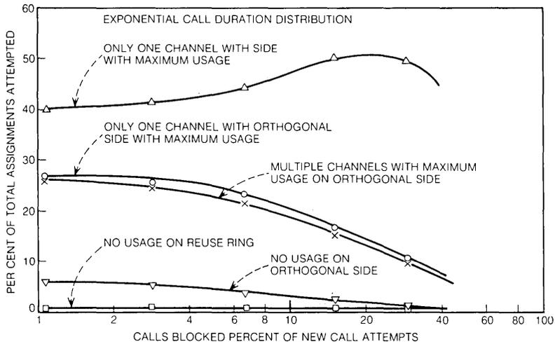
Fig. 9—Performance characteristics of two-dimensional NN channel assignment.
