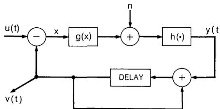
Fig. 10b—Model of a Differential Quantizer.
