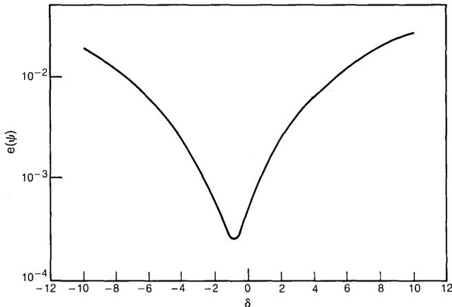
Fig. 4—Plot of  $e(\psi)$  for a buried channel device with  $h_1 = 0.24$ ,  $h_2 = 12.24$ ,  $c_s = 46$ ,  $Q_{ss} = 0$ ,  $\eta = \frac{1}{3}$ , and  $V_0 = 0$  as a function of  $\delta$  for  $-10 \leq \delta \leq 10$ .
