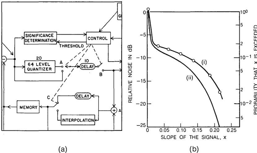
Fig. 5a, b—Picture of graphics: (i) The relative white noise plotted against threshold. (ii) The probability that the threshold is exceeded.
