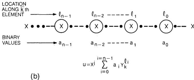
Fig. 4—(a) Representation of a single bubble. See text for explanation of  $j$ ,  $k$ , and  $l$ . (b) Representation of a bubble stream  $j$  clock cycles after a prechosen origin of time.
