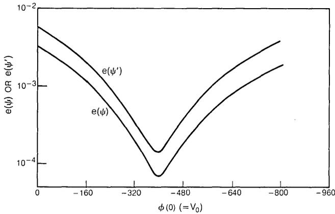
Fig. 7—Plots of  $e(\psi)$  and  $e(\psi')$  for a buried channel device with  $h_1 = 0.24$ ,  $h_2 = 12.24$ ,  $\bar{\sigma} = 20$ ,  $Q_{ss} = 0$ ,  $\eta = \frac{1}{3}$  and  $\hat{R} = 50.98$  as functions of  $V_0$  for  $-800 \leq V_0 \leq 0$ .
