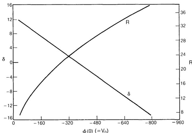
Fig. 12—Plots of  $\delta$  and "true"  $R$  for a surface device with  $h_1 = h_2 = 0.24$ ,  $\sigma = 0$ ,  $Q_{ss} = 0$ ,  $\eta = \frac{1}{3}$  and  $\hat{R} = 26.55$  as functions of  $V_0$  for  $-800 \leq V_0 \leq -40$ .
