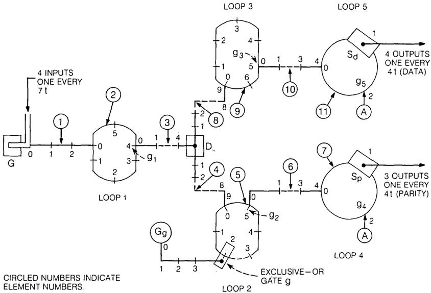
Fig. 2—(7, 4) Hamming encoder with magnetic domains and T-bars.
