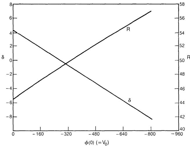
Fig. 8—Plots of  $\delta$  and “true”  $R$  for a buried channel device with  $h_1 = 0.24$ ,  $h_2 = 12.24$ ,  $\bar{\sigma} = 20$ ,  $Q_{ss} = 0$ ,  $\eta = \frac{1}{3}$  and  $\hat{R} = 50.98$  as functions of  $V_0$  for  $-800 \leq V_0 \leq 0$ .
