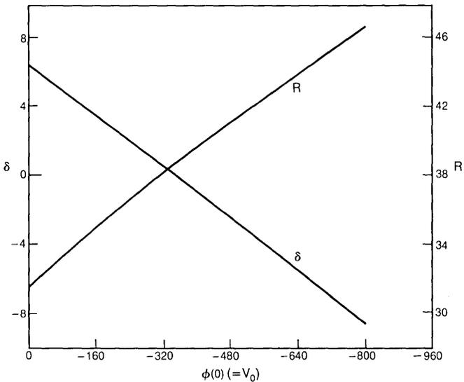
Fig. 10—Plots of  $\delta$  and "true"  $R$  for a buried channel device with  $h_1 = 0.24$ ,  $h_2 = 12.24$ ,  $c_s = 46$ ,  $Q_{ss} = 0$ ,  $\eta = \frac{1}{3}$  and  $\hat{R} = 39.66$  as functions of  $V_0$  for  $-800 \leq V_0 \leq 0$ .
