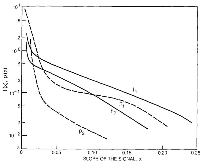
Fig. 9b—A comparison of the function  $f(x)$  with the probability density of slopes  $p(x)$ , for two scenes.
