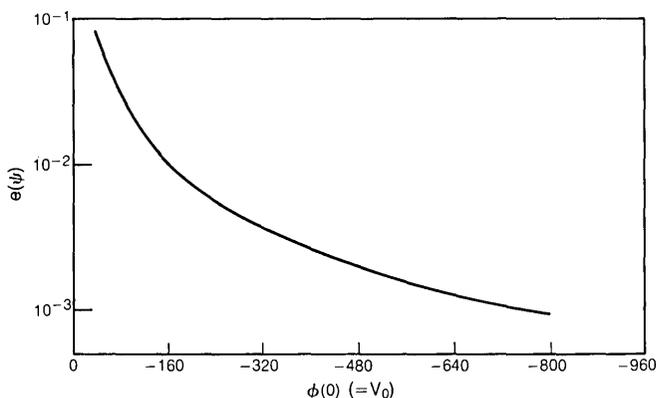
Fig. 6—A plot of  $e(\psi)$  for a surface device with  $h_1 = h_2 = 0.24$ ,  $\sigma = 0$ ,  $Q_{ss} = 0$ ,  $\eta = \frac{1}{3}$  and  $\delta = -10$  as a function of  $V_0$  for  $-800 \leq V_0 \leq -40$ .
