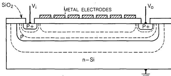
Fig. 1—Cross-sectional view of buried channel CCD.
