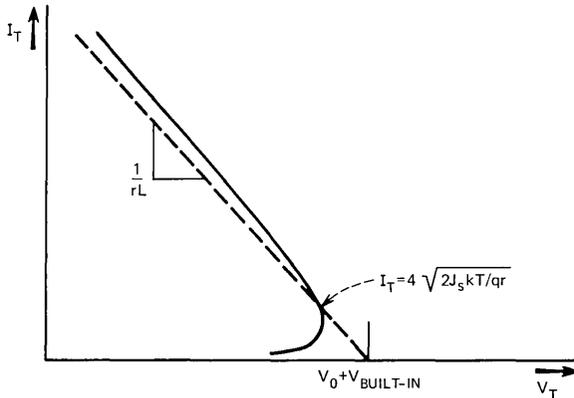
Fig. 6—Form of terminal  $I_T - V_T$  characteristic based on fully regenerative solution.
