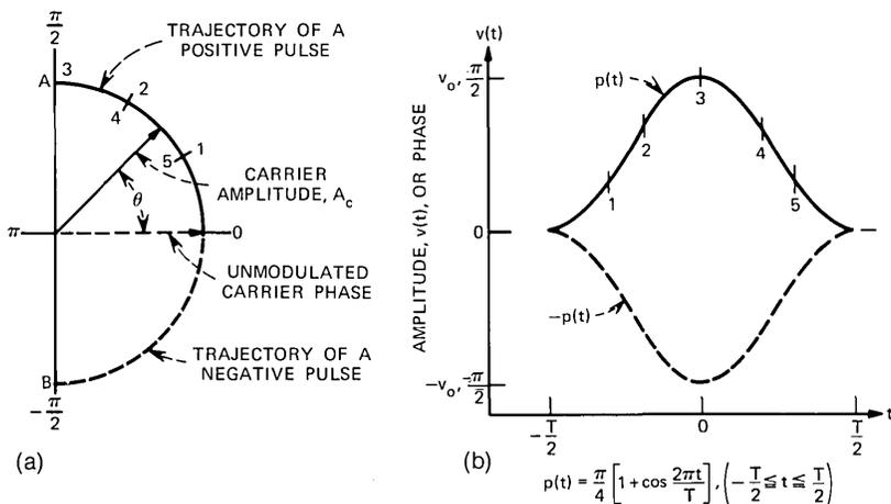
Fig. 3—Phase plane representation of a binary signal.
