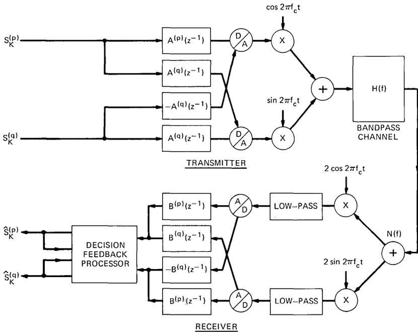
Fig. 2—QAM data system with decision feedback equalization.
