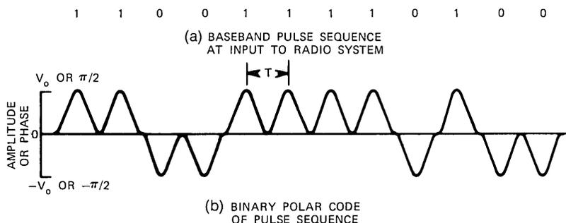
Fig. 2—Binary polar code of pulse sequence.
