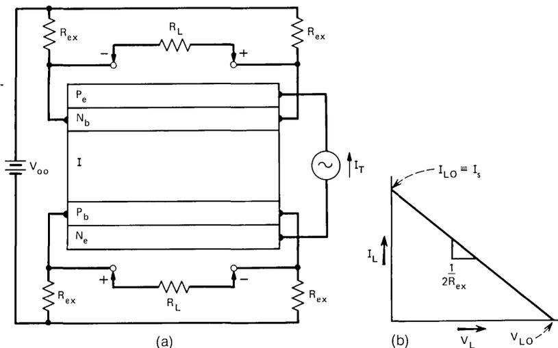
Fig. 8—(a) Magnetic field detector circuit with provision for load  $R_L$ . (b) Load line for (a).
