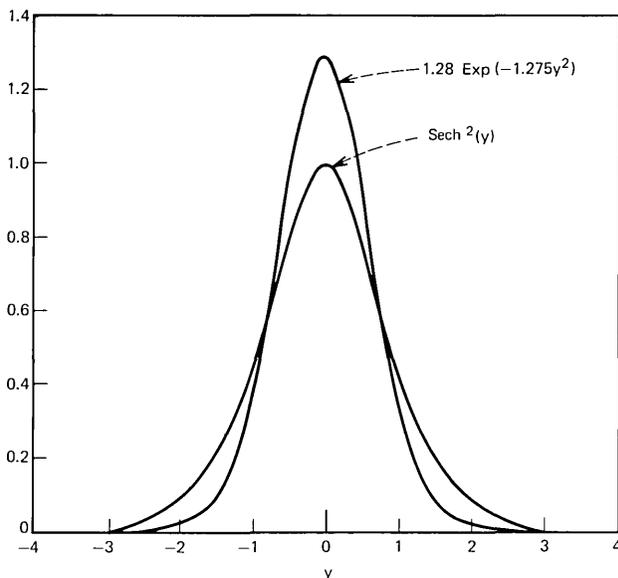
Fig. 7—Comparison of Gaussian approximation in the diffusionless case with fully regenerative solution at one value of  $I_T$ .
