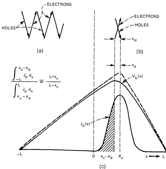
Fig. 3—(a) Representation of multipass displacement in the absence of a restoring force. (b) Representation as in (a) with restoring force. (c) Illustration of relation between hole current profile  $J_p(x)$  and base voltage  $V_b(x)$  for a displaced filament.
