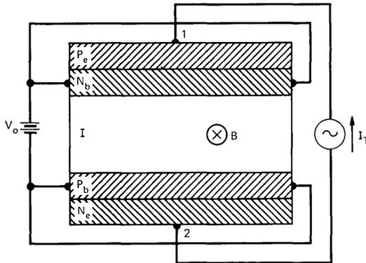
Fig. 2—Filament forming structure with multiterminal circuit connection.
