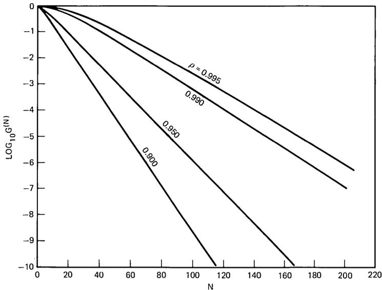
Fig. 3—Probability of overflow in a burst vs level ( $\theta_1 = 0.2$ ,  $\theta_2 = 0.1$ ,  $k = 5$ ).
