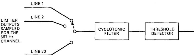
Fig. 3—System amenable to serial multiplexing.
