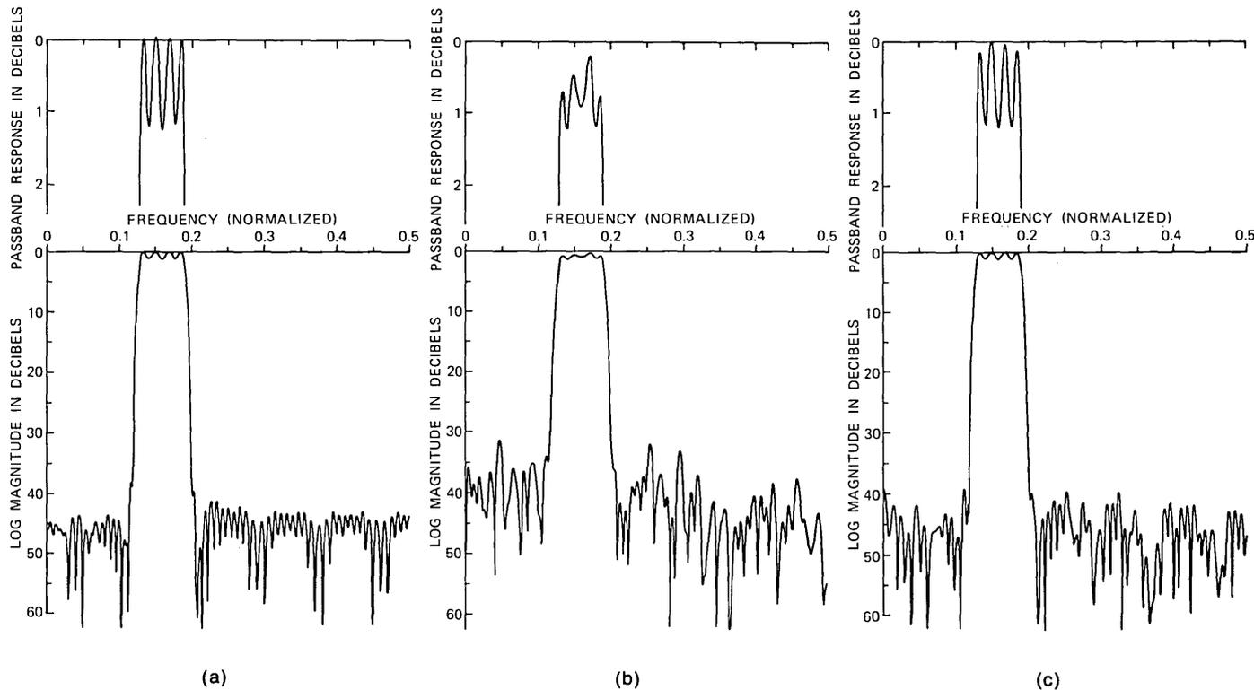
Fig. 4—Frequency response measurement using (a) an  $N = 7$  all-pass test signal in a 16-bit system, (b) an impulse test signal in an equivalent 12-bit system, and (c) an  $N = 7$  all-pass test signal in the 12-bit system.
