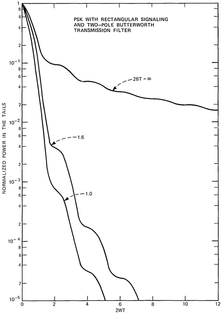
Fig. 3—Normalized power contained outside the band  $[-W, W]$  for  $M$ -ary PSK ( $M = 2^N, N \geq 1$ ) with rectangular signaling and a two-pole Butterworth transmission filter. The squared amplitude characteristic of the equivalent low-pass filter is assumed to be given by  $|H_T(f)|^2 = 1/[1 + (f/A)^4]$ , where  $2B = 2A(\pi/4)/\sin \pi/4$  is the noise bandwidth of the filter.
