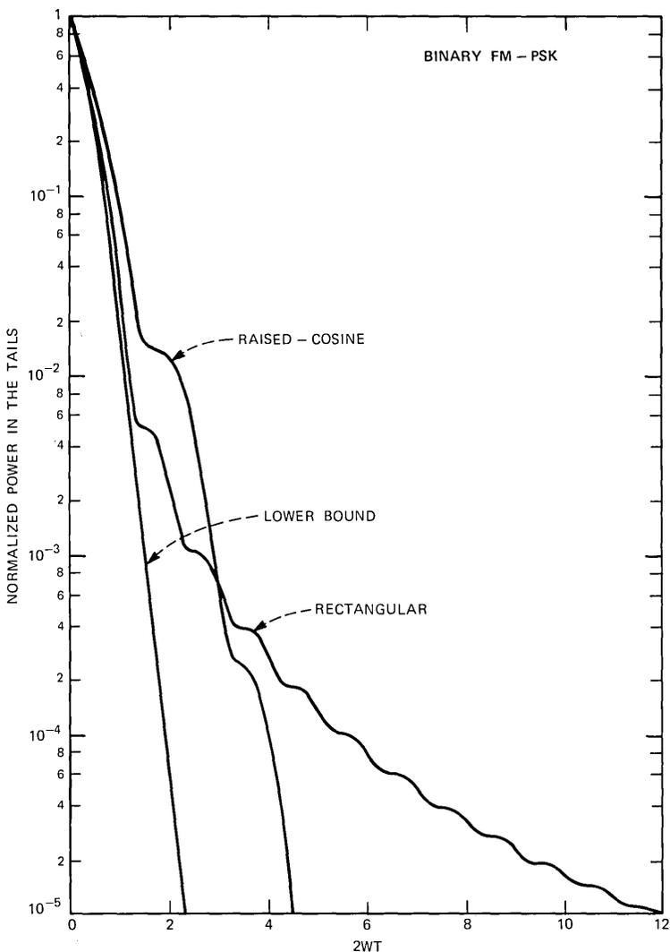
Fig. 8—Normalized power  $\Delta^2$  contained outside the band  $[-W, W]$  for binary FM-PSK with different baseband signaling waveforms and also the lower bound on  $\Delta^2$  for any baseband signaling waveform.
