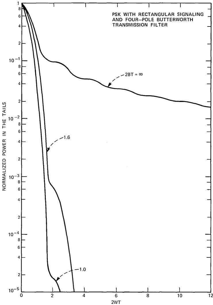
Fig. 4—Normalized power contained outside the band  $[-W, W]$  for  $M$ -ary psk ( $M = 2^N$ ,  $N \geq 1$ ) with rectangular signaling and a four-pole Butterworth transmission filter. The squared amplitude characteristic of the equivalent low-pass filter is assumed to be given by  $|H_T(f)|^2 = 1/[1 + (f/A)^2]$ , where  $2B = 2A(\pi/8)/\sin \pi/8$  is the noise bandwidth of the filter.
