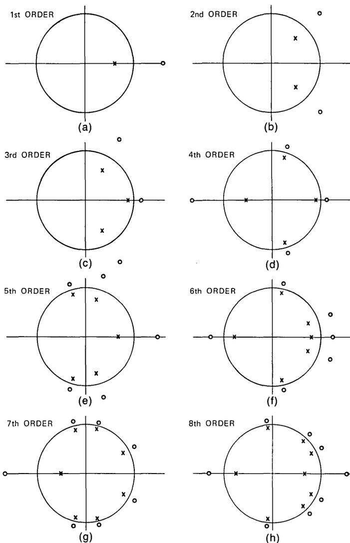
Fig. 1—Positions of the poles and zeros of the optimized all-pass signals of order 1 to 8.
