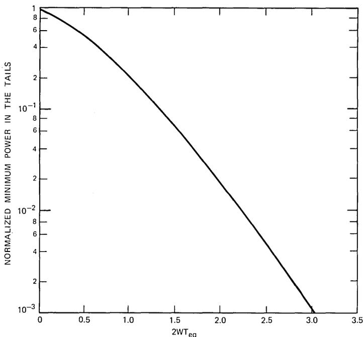
Fig. 9—Lower bound on the fractional energy contained outside the band  $[-W, W]$  when the pulse  $f(t)$  is of duration  $T_{\text{eq}}$ .
