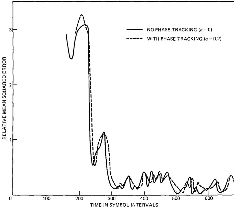
Fig. 3b—Convergence with and without phase tracking (ideal reference; all equalizer top coefficients start at zero).
