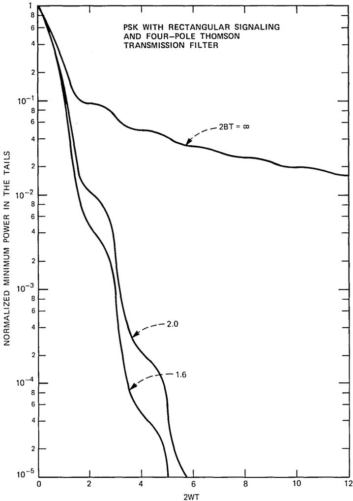
Fig. 5—Normalized power contained outside the band  $[-W, W]$  for  $M$ -ary PSK ( $M = 2^N, N \geq 1$ ) with rectangular signaling and a four-pole Thomson transmission filter. The squared amplitude characteristic of the equivalent low-pass filter is assumed to be given by  $|H_T(f)|^2 = 11025/(z^8 + 10z^6 + 135z^4 + 1575z^2 + 11025)$ ,  $z = f/A$  and  $2B = 4.4238A$  is the noise bandwidth of the filter.
