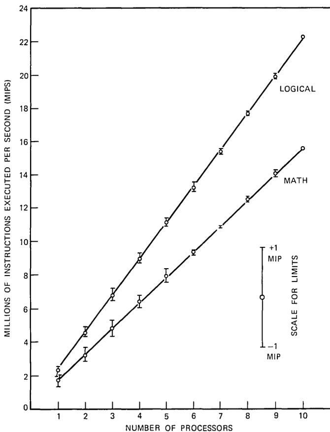
Fig. 9— $N$  processors executing from  $N$  program stores.
