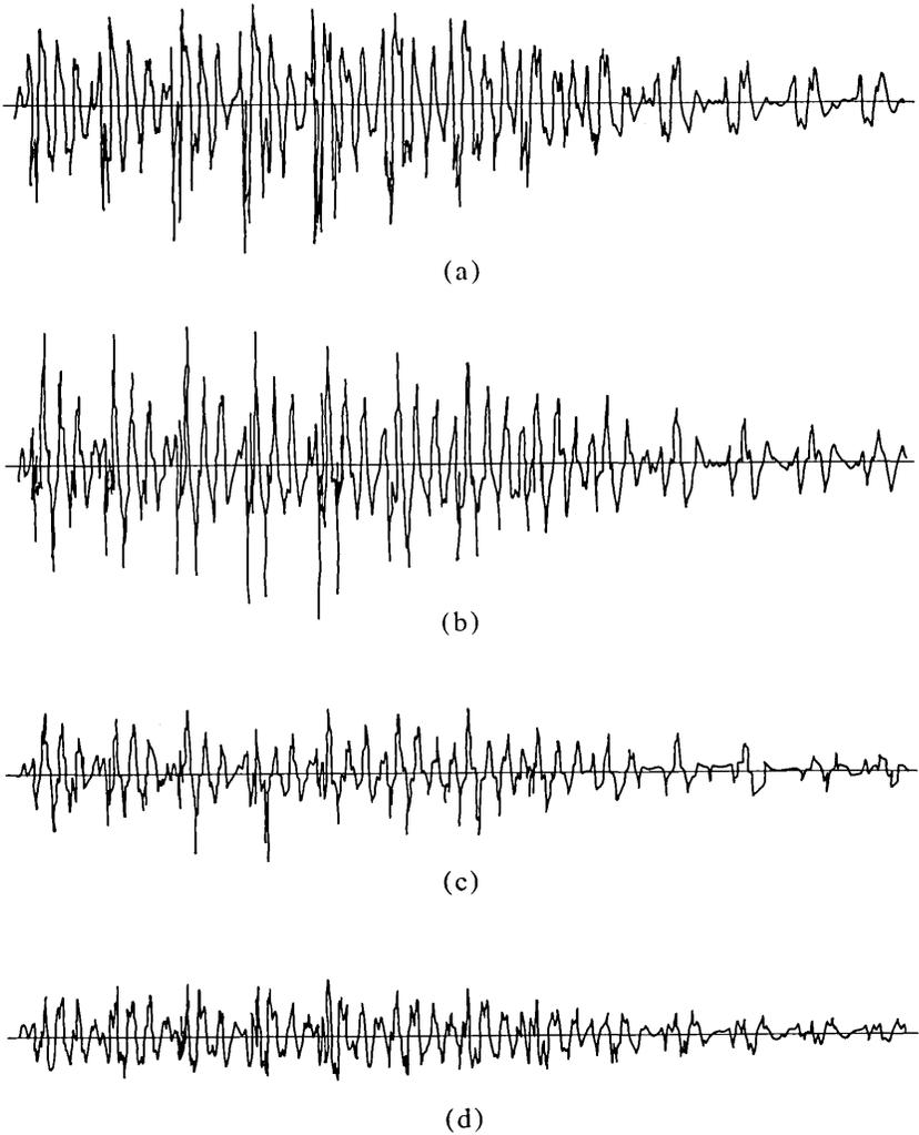
Fig. 6—Speech waveforms for the wideband system. (a) Waveform after 10:16 sampling rate conversion. (b) Waveform after first BPF (input to CVSD). (c) CVSD output waveform ( $G = 0.158$ ). (d) CVSD output waveform after BP filtering (output of wideband system).
