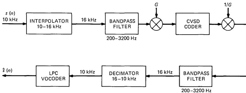
Fig. 1—Block diagram of signal processing operations in tandem link of a CVSD coder and an LPC vocoder.
