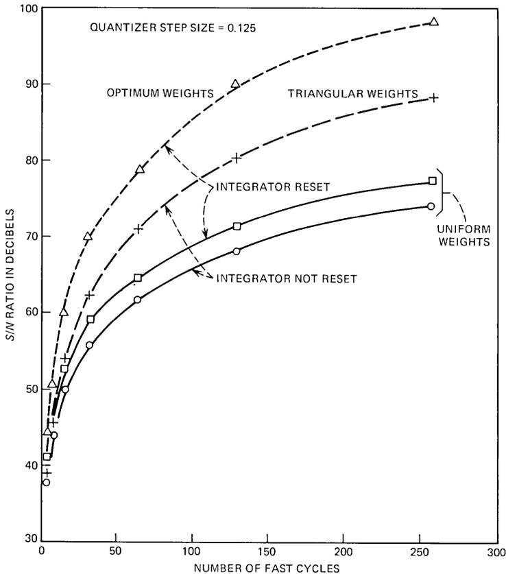
Fig. 2—Performance of an interpolative A/D converter with various digital filter weights.
