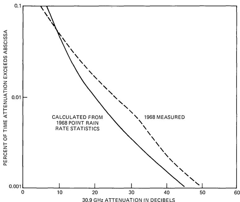
Fig. 1—Rain attenuation measured on a 1.9-km path in New Jersey compared with calculation based upon rain rate measured at a point on the path.
