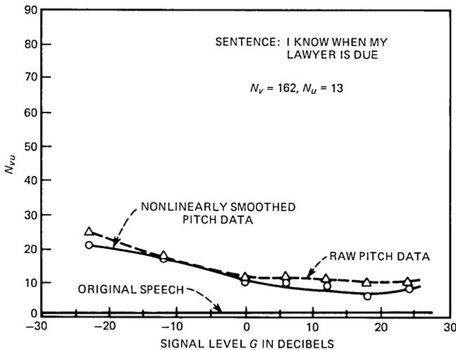
Fig. 7—Plot of number of voiced-to-unvoiced errors versus CVSD signal level for utterance “I know when my lawyer is due.”
