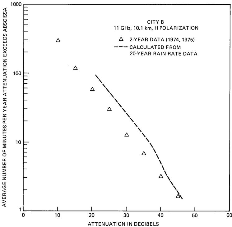
Fig. 16—Comparison of calculated (dashed line) versus measured 11-GHz rain attenuation distribution on a 10.1-km path at City B. The calculation is based on 20-year distribution of 5-minute point rain rate at City B.
