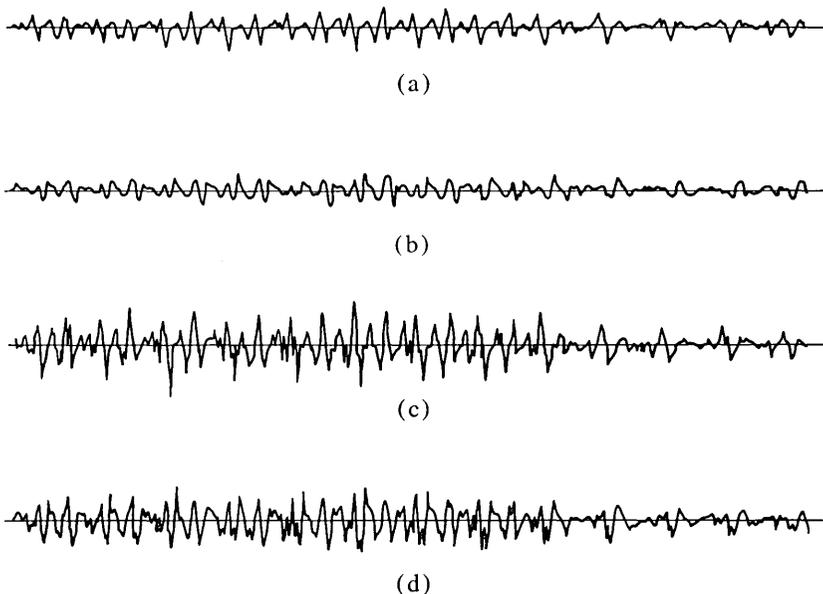
Fig. 8—Output waveforms of the CVSD coder in the slope overload region. (a) Coder output for  $G = 2.528$  and (b) the output after BP filtering. (c) Coder output for  $G = 0.632$  and (d) BP filtered output.
