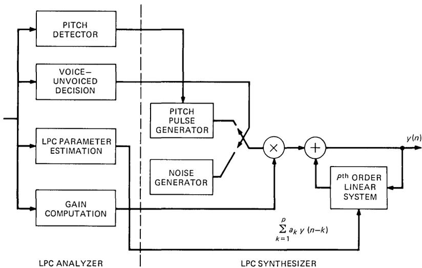
Fig. 2—Block diagram of LPC analyzer and synthesizer.
