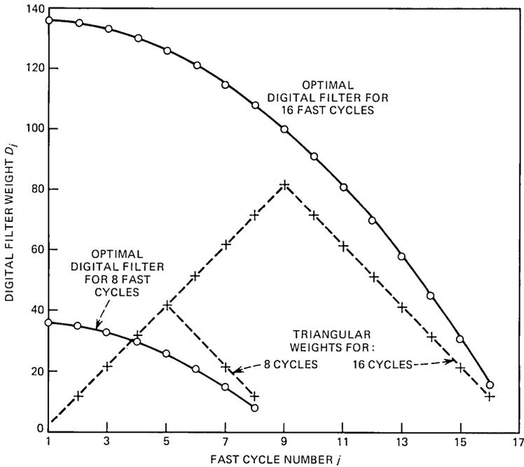
Fig. 5—Weights of optimum- and triangular-weight digital filters.
