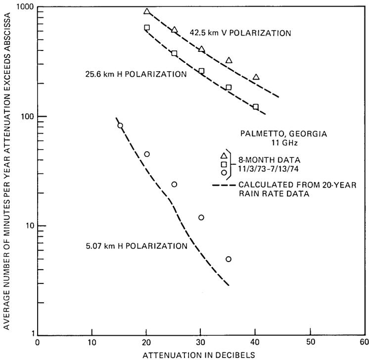
Fig. 14—Comparison of calculated (dashed lines) versus measured 11-GHz rain attenuation distributions on 5.07, 25.6, and 42.5 km paths at Palmetto, Georgia. The calculations are based on 20-year distribution of 5-minute point rain rates at Atlanta, Georgia.
