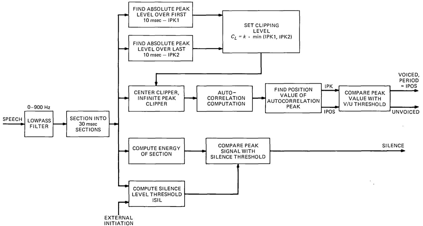
Fig. 3—Block diagram of modified autocorrelation pitch detector.
