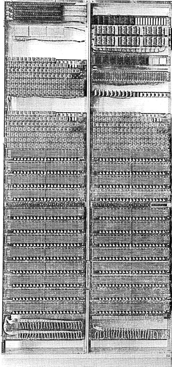
Fig. 27—Outpulser link frame.
