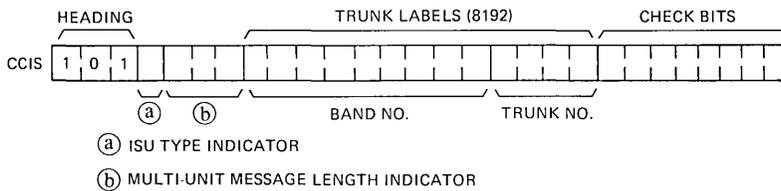
Fig. 8—Initial Signal Unit (ISU) format.
