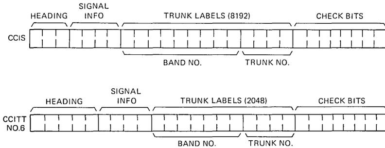
Fig. 7—Lone Signal Unit (LSU) format.
