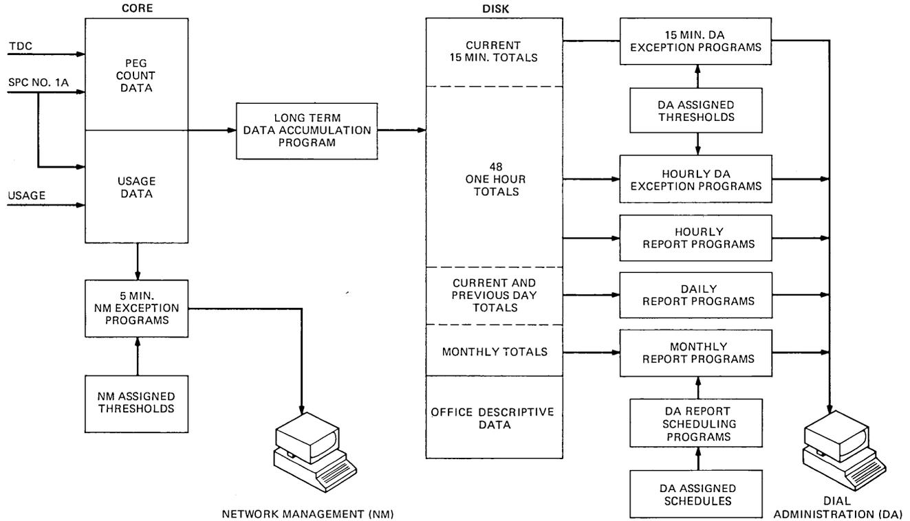
Fig. 6—PBC data accumulation.
