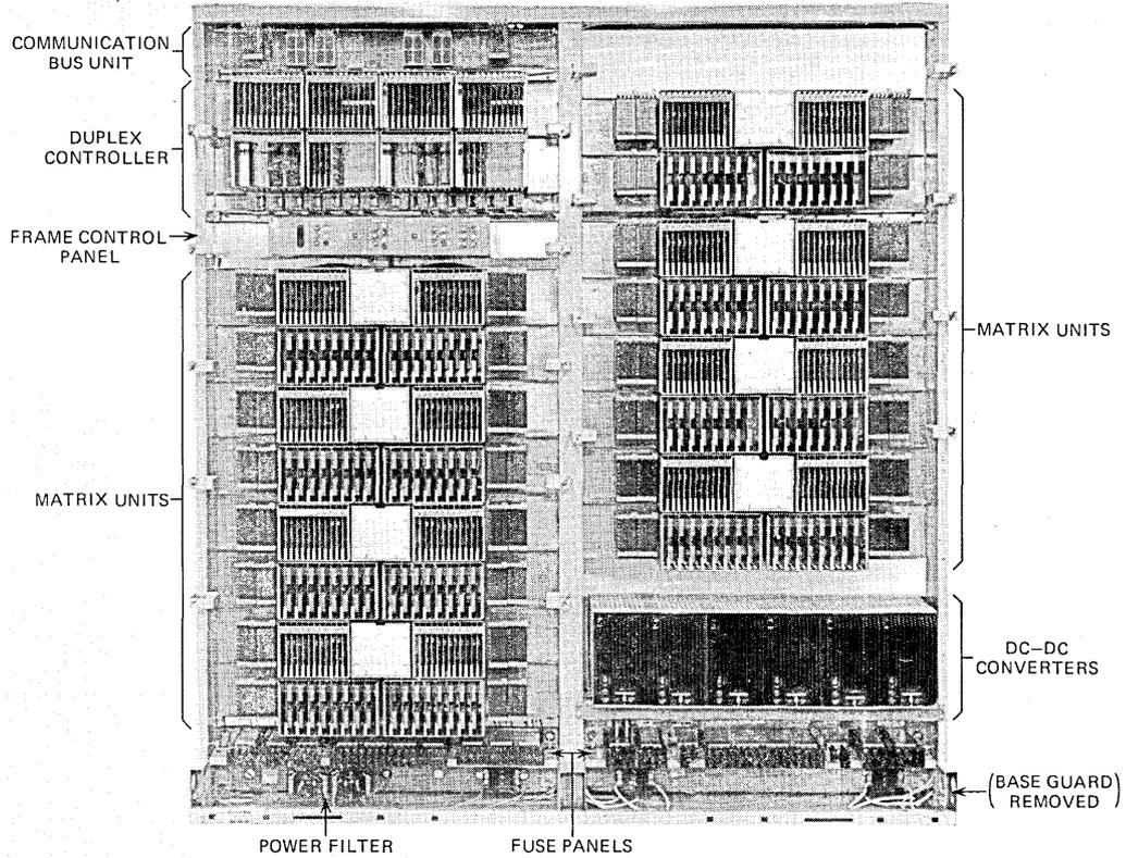
Fig. 21—Distributor and scanner frame.
