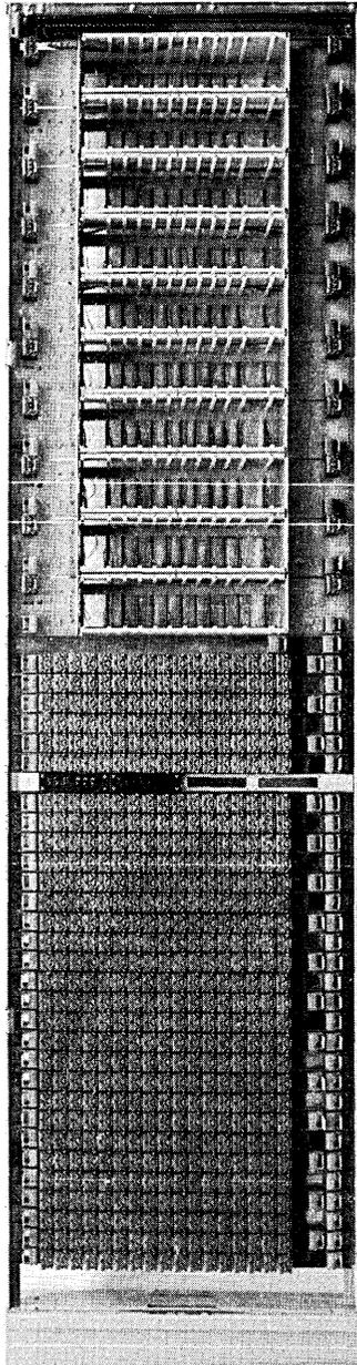
Fig. 30—Transceiver and connector frame.
