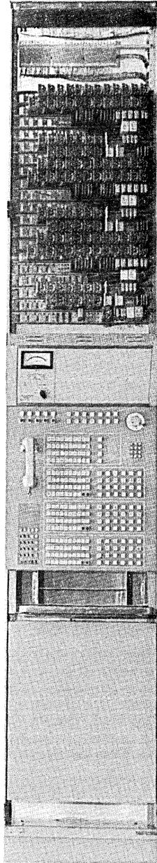
Fig. 33—CCIS intra-office trunk test frame.
