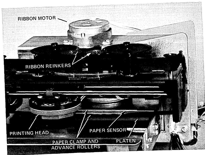
Fig. 4—Printing mechanism.
