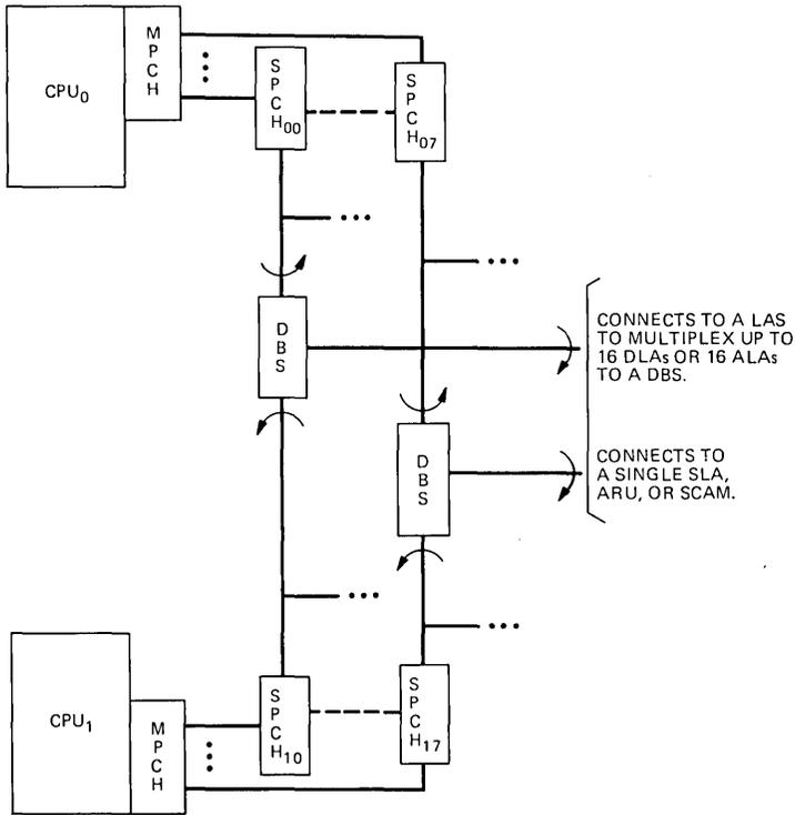
Fig. 1—Switch configuration.
