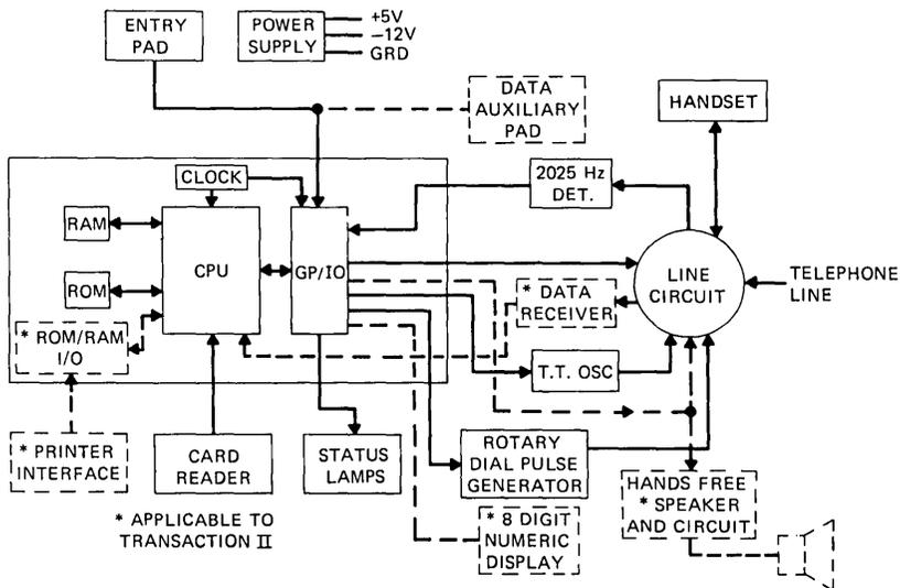
Fig. 3—Transaction telephone.
