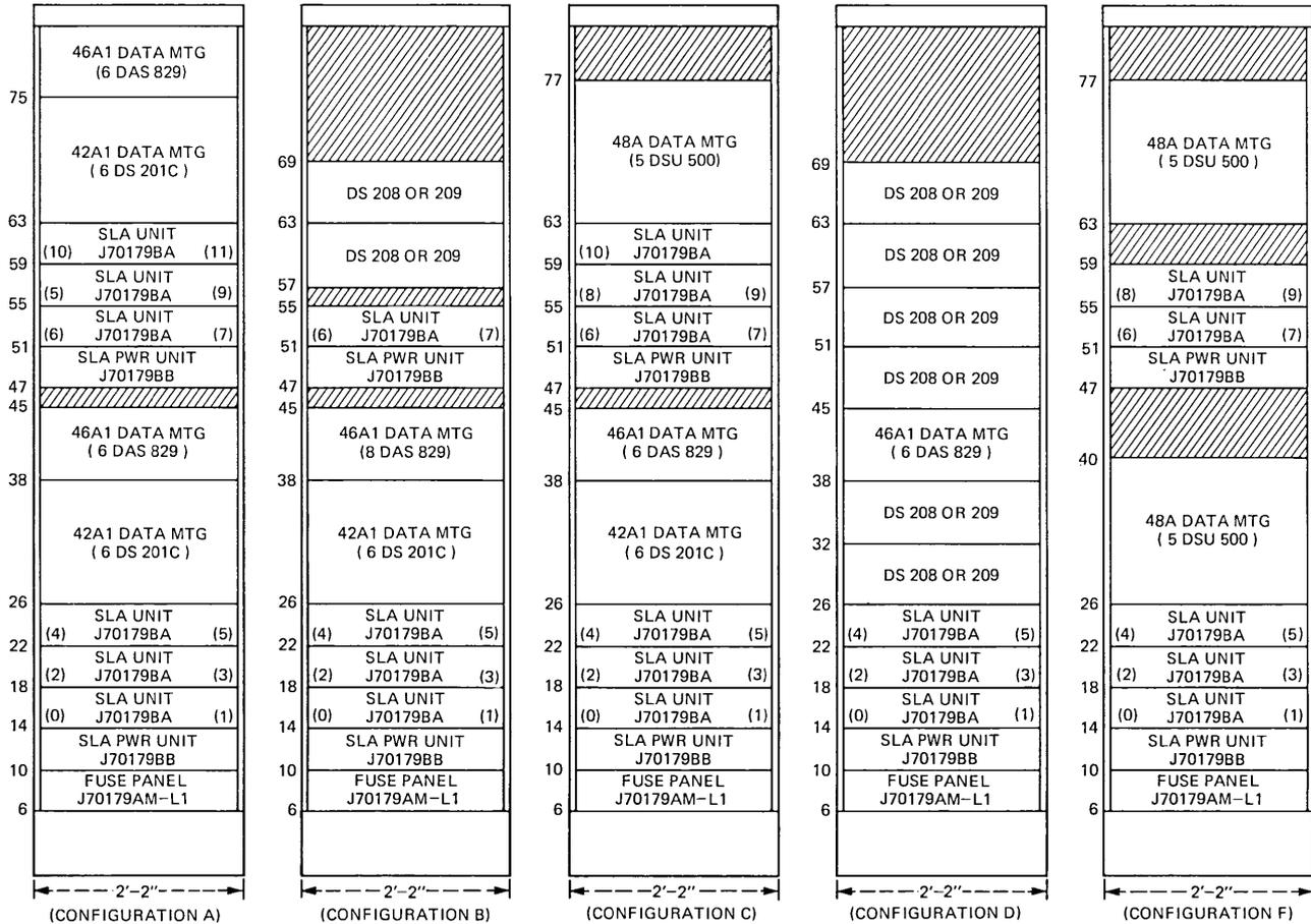
Fig. 7—Synchronous line adapter frame.
