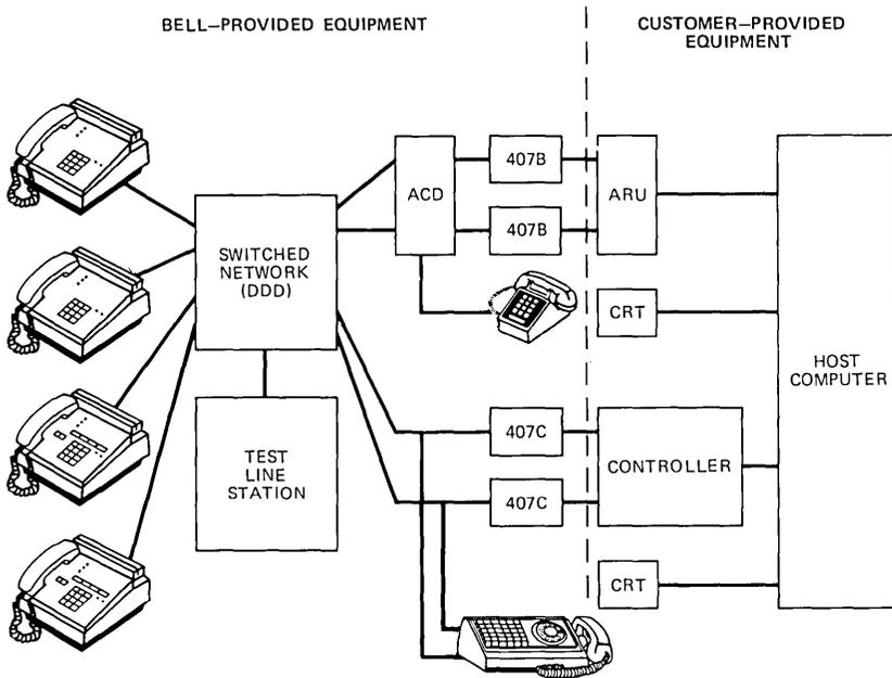
Fig. 2—Switched Network Transaction Telephone System, second phase.
