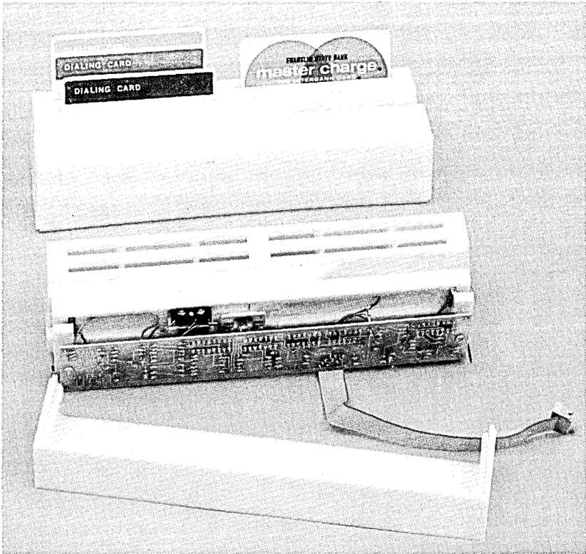
Fig. 8—Transaction III card reader.
