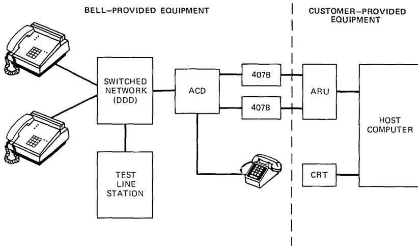
Fig. 1—Switched Network Transaction Telephone System, first phase.
