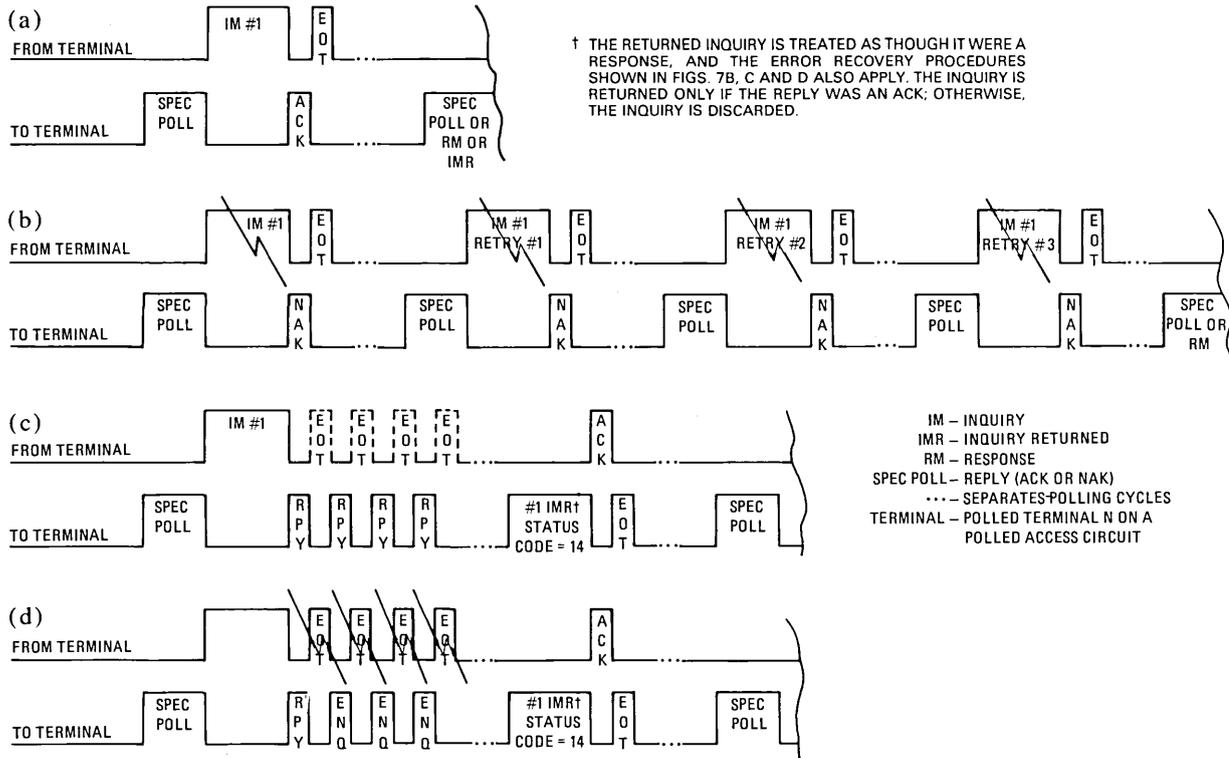
Fig. 6—(a) Normal inquiry transfer. (b) Garbled inquiry from the terminal. (c) Lost termination from the terminal. (d) Garbled termination from the terminal.
