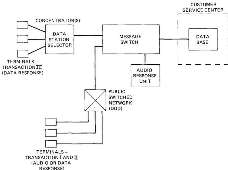
Fig. 4—Transaction network—another serving arrangement for transaction traffic.
