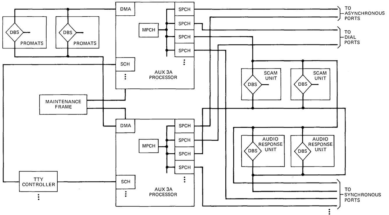
Fig. 1—Message switch common equipment.
