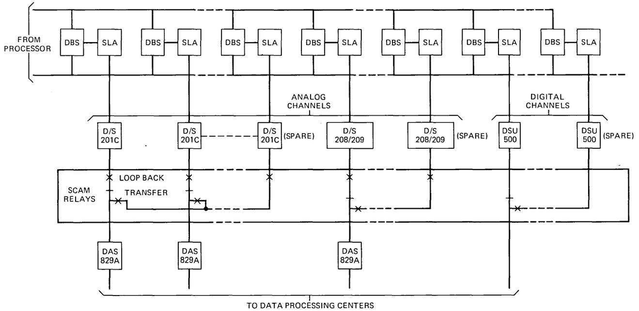
Fig. 5—Synchronous access configuration.
