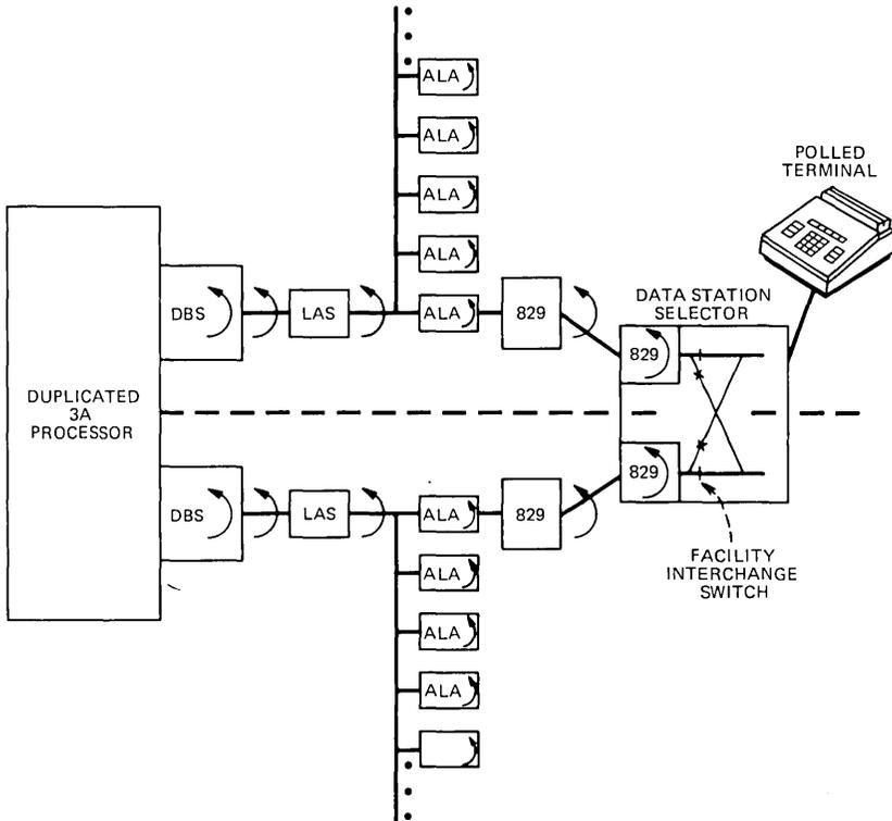
Fig. 11—Asynchronous polled access line loopbacks (Y).
