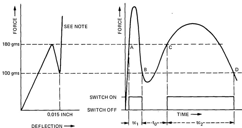
NOTE: AFTER THE DISK BOTTOMS ON THE CENTER STAPLE, THE SLOPE DEPENDS ON THE MANUAL ENTRY PAD SUPPORT.
