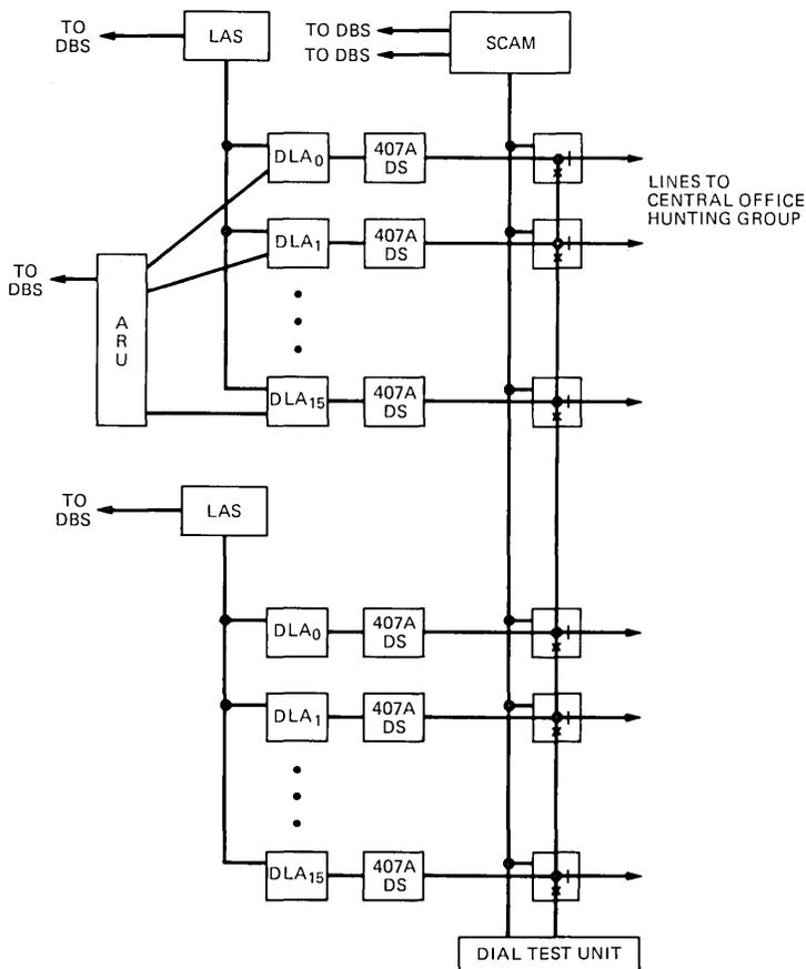
Fig. 7—Dial-in network configuration.
