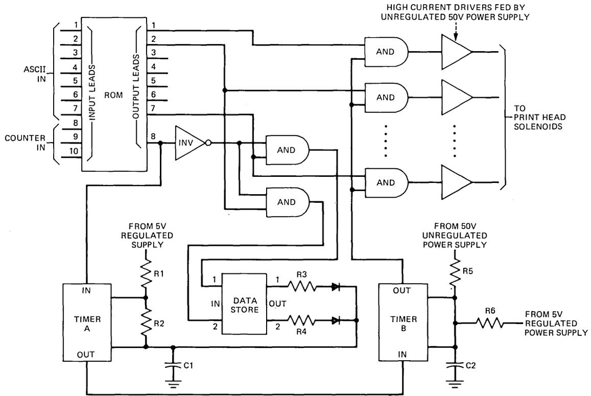
Fig. 5—Printer circuitry.
