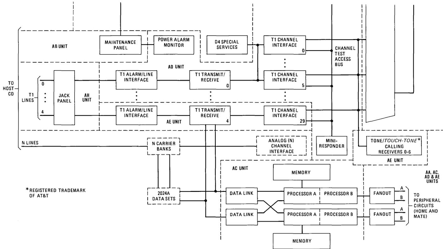
Fig. 11—No. 10A Remote Switching System block diagram (frame partitioning).
