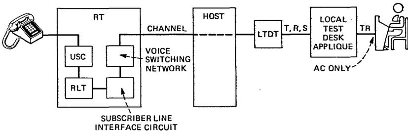
Fig. 27—Line test equipment using a telemetry path.
