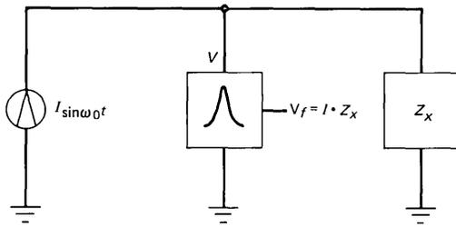
Fig. 9—Impedance measurement which reduces effects of noise.
