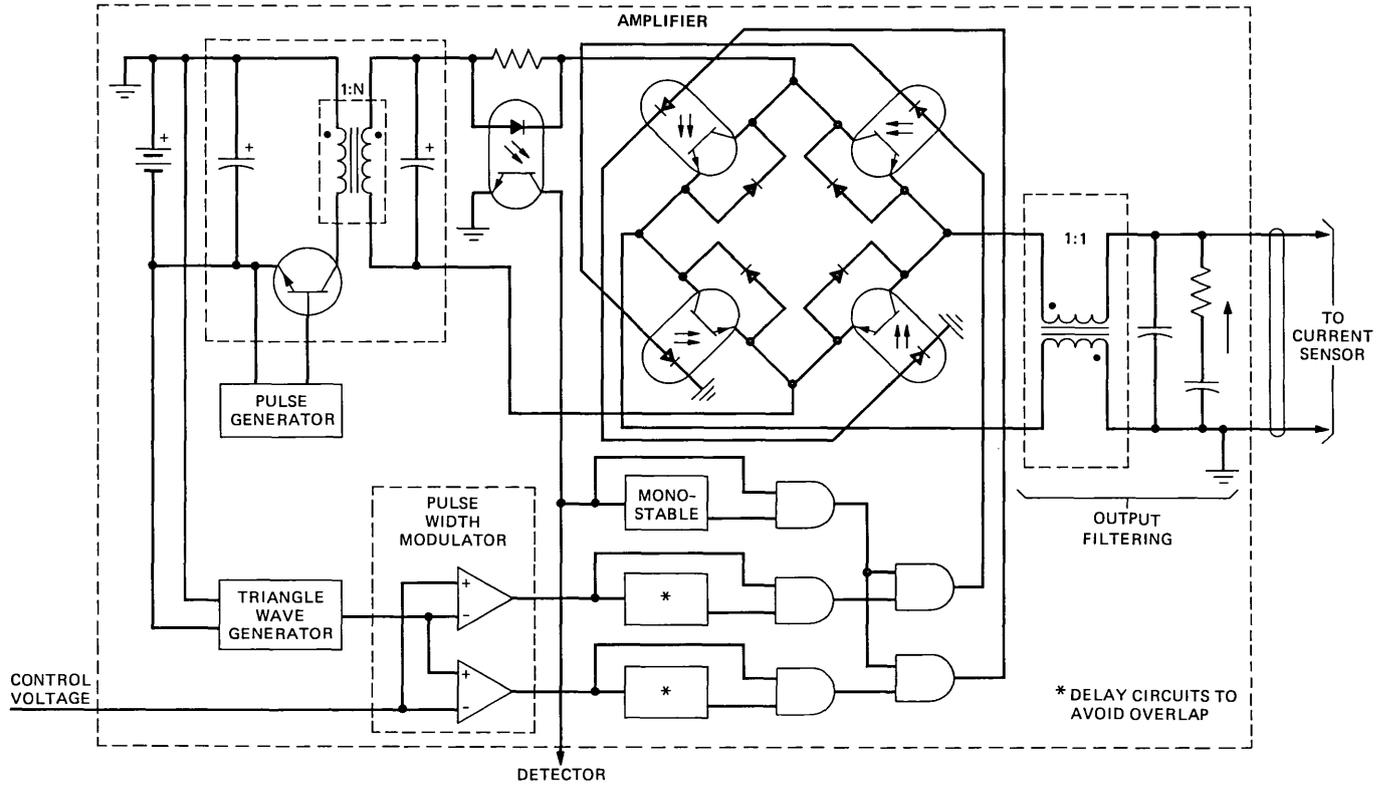
Fig. 17—Universal-level service circuit voltage source.
