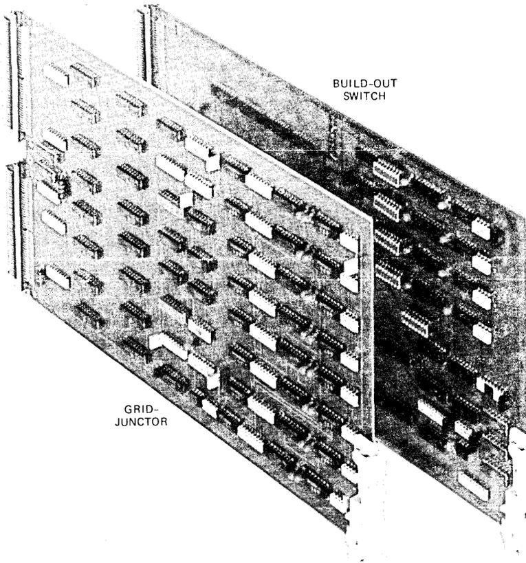
Fig. 14—PNPN network center-stage circuit packs.
