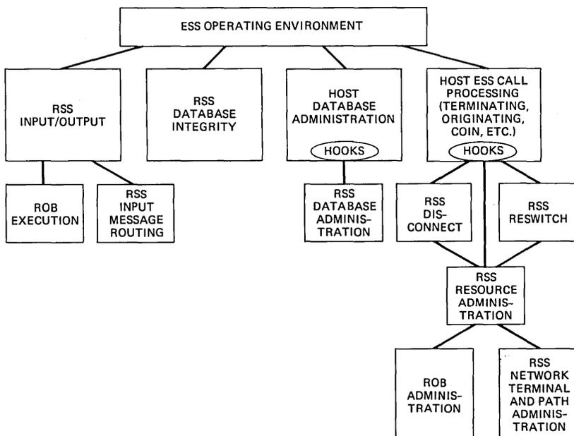
Fig. 2—Remote switching system host software architecture overview.
