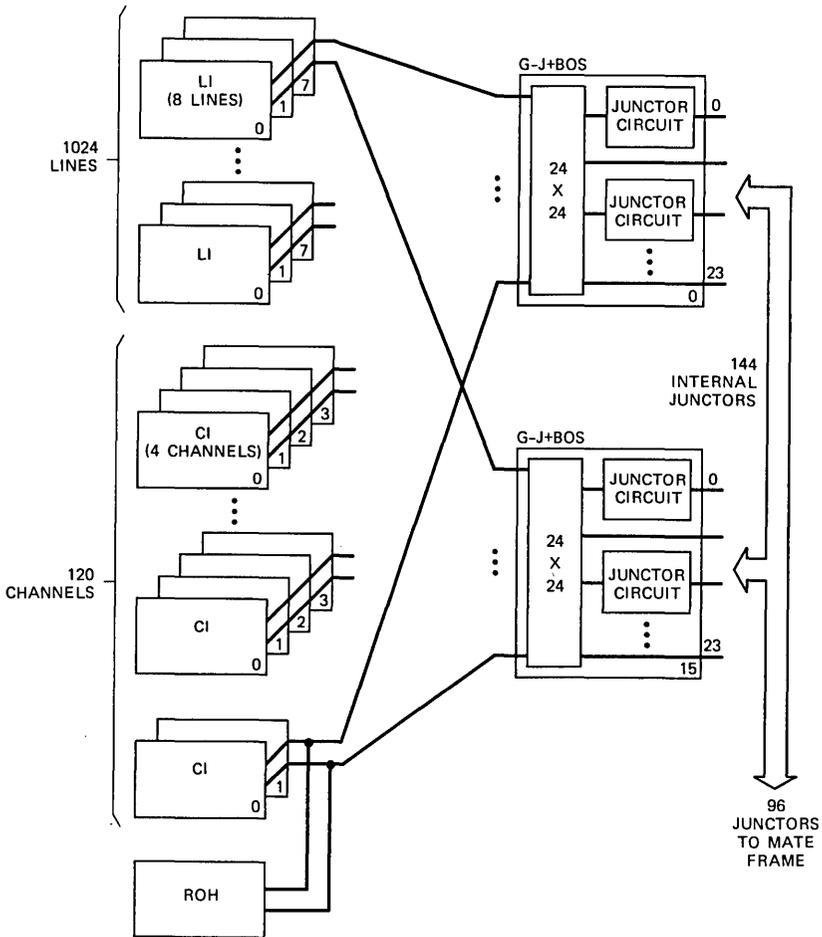
Fig. 11—Network configuration for up to 1024 lines and interconnect to optional mate frame.
