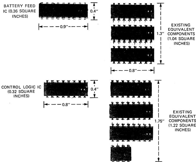
Fig. 2—Space savings of battery feed and control logic ICs.
