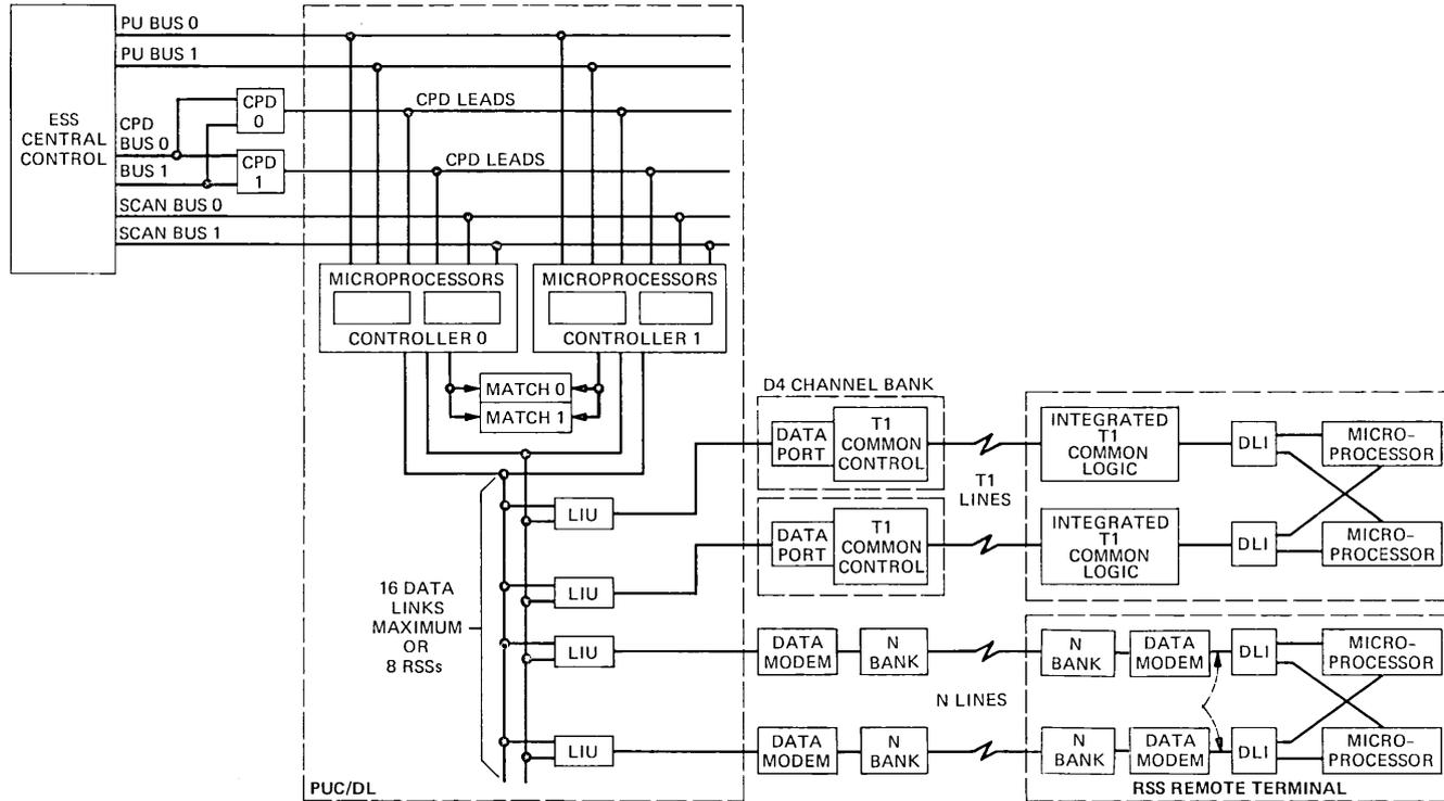
Fig. 3—Remote switching system data links.
