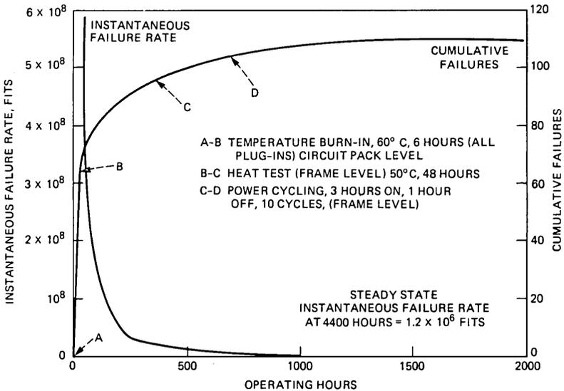
Fig. 26—Relationship between instantaneous failure rate, cumulative failures, and operating time.
