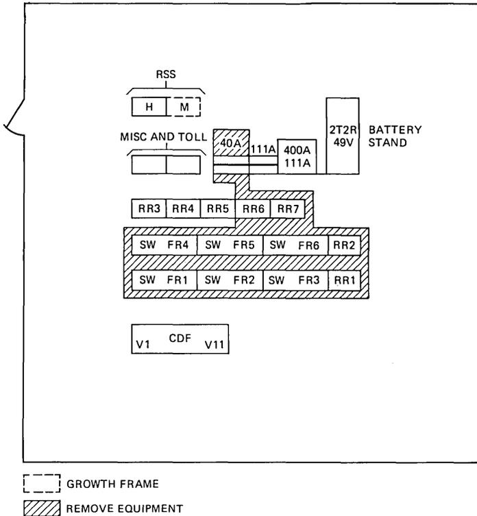
Fig. 20—Typical rss floor plan as a CDO replacement (800 lines step-by-step office).
