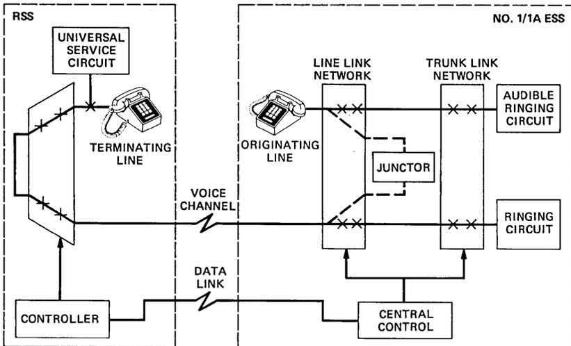
Fig. 13—Remote switching system terminating call.
