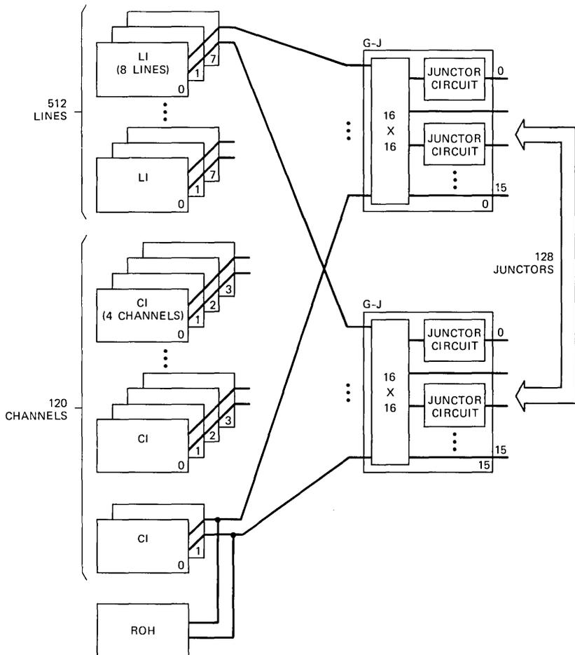
Fig. 10—Network configuration for up to 518 lines.
