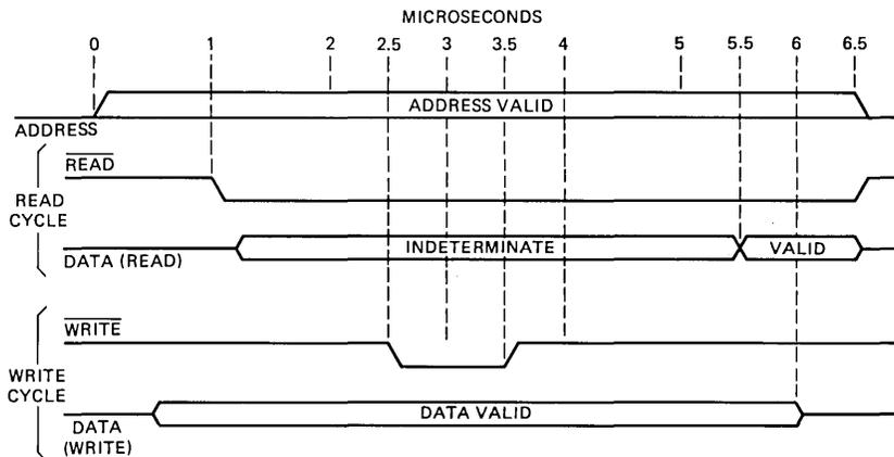
Fig. 11—Peripheral timing.
