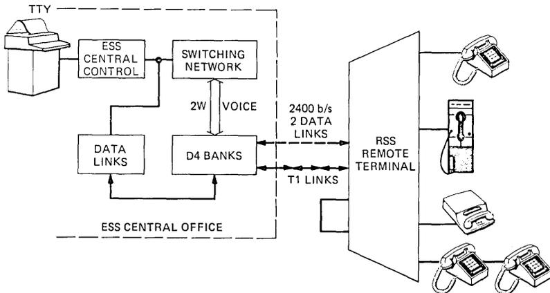
Fig. 1—Remote switching system block diagram (T carrier).
