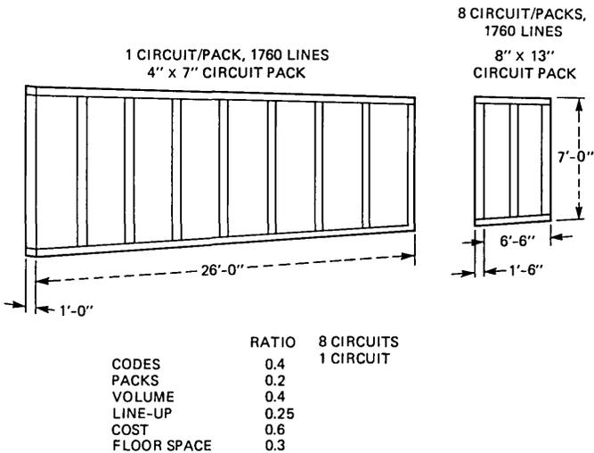
Fig. 4—Remote Switching System partitioning (one circuit per pack versus eight circuits per pack designs).
