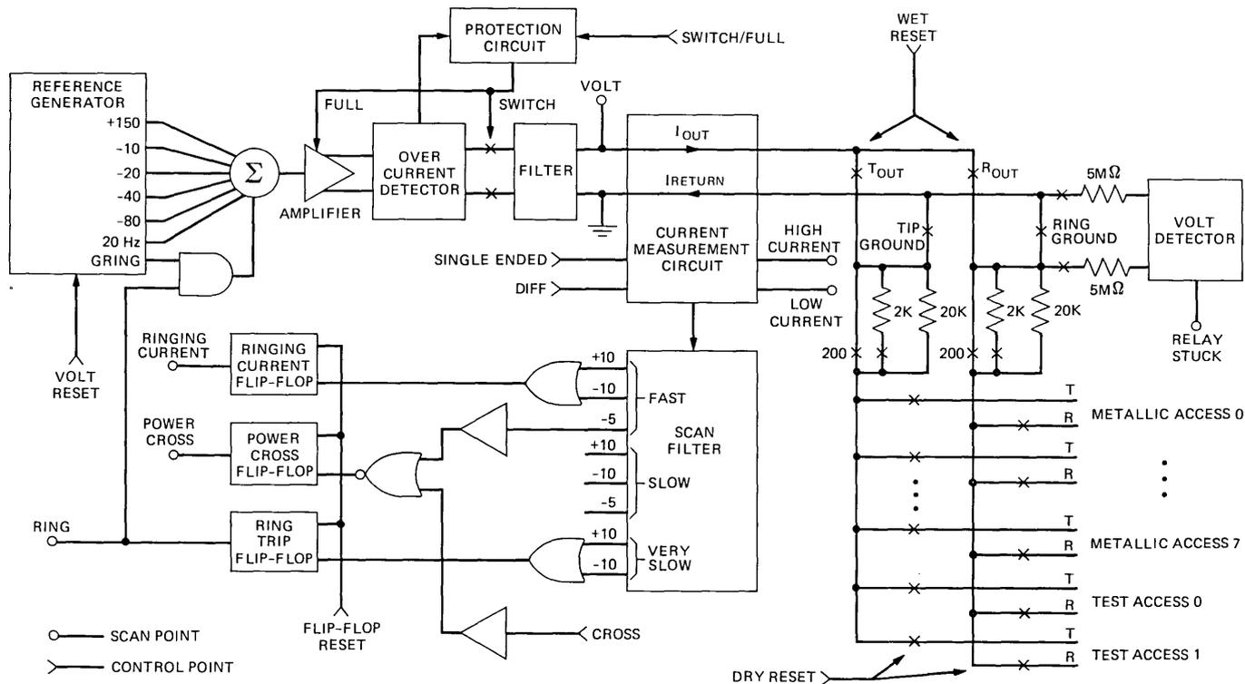
Fig. 16—Universal service circuit block diagram.
