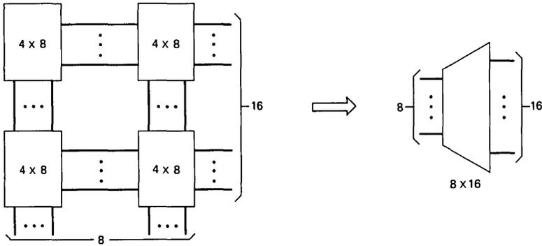
Fig. 8—Construction of line interface pack 8 x 16 switch.
