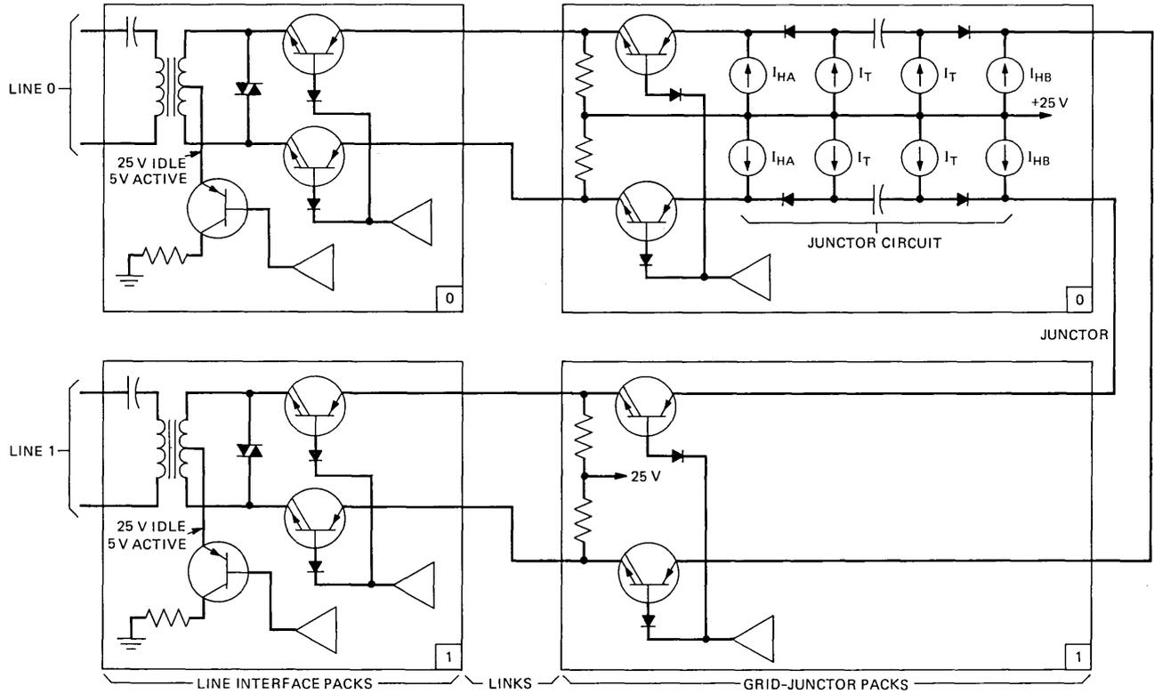
Fig. 13—A line-to-line network pass.
