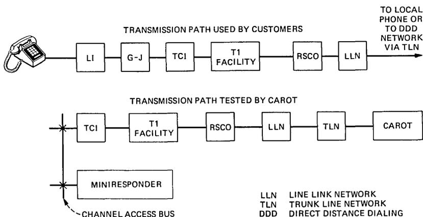
Fig. 29—Transmission testing.
