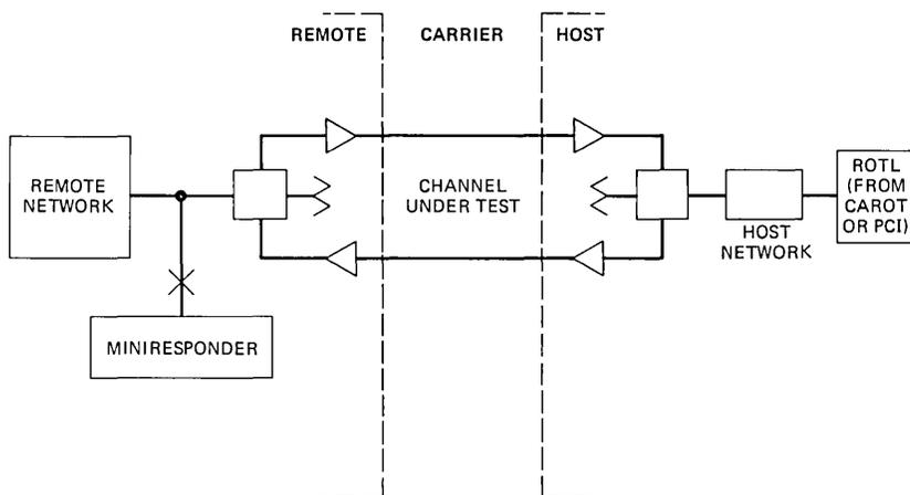
Fig. 3—Remote switching system channel testing.
