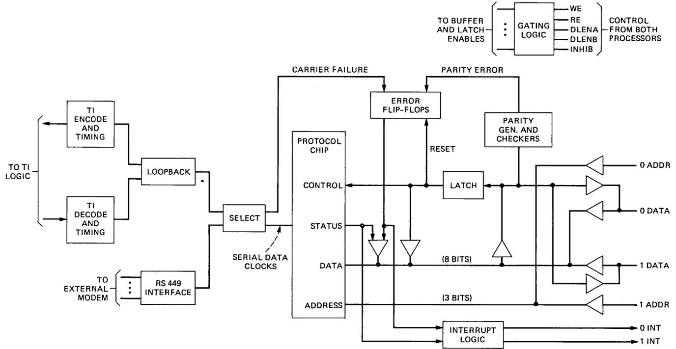
Fig. 8—Remote switching system data link interface functional block diagram.
