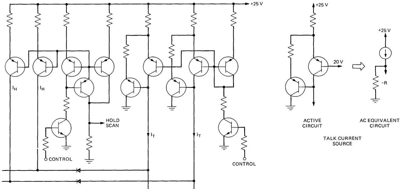
Fig. 14—Junction circuit diagram and implementation of negative resistance.
