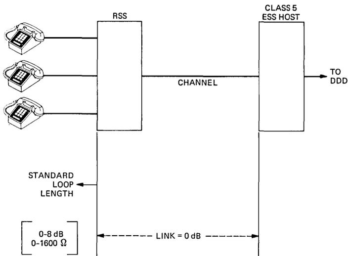
Fig. 1—Remote switching system transmission plan basic objective.
