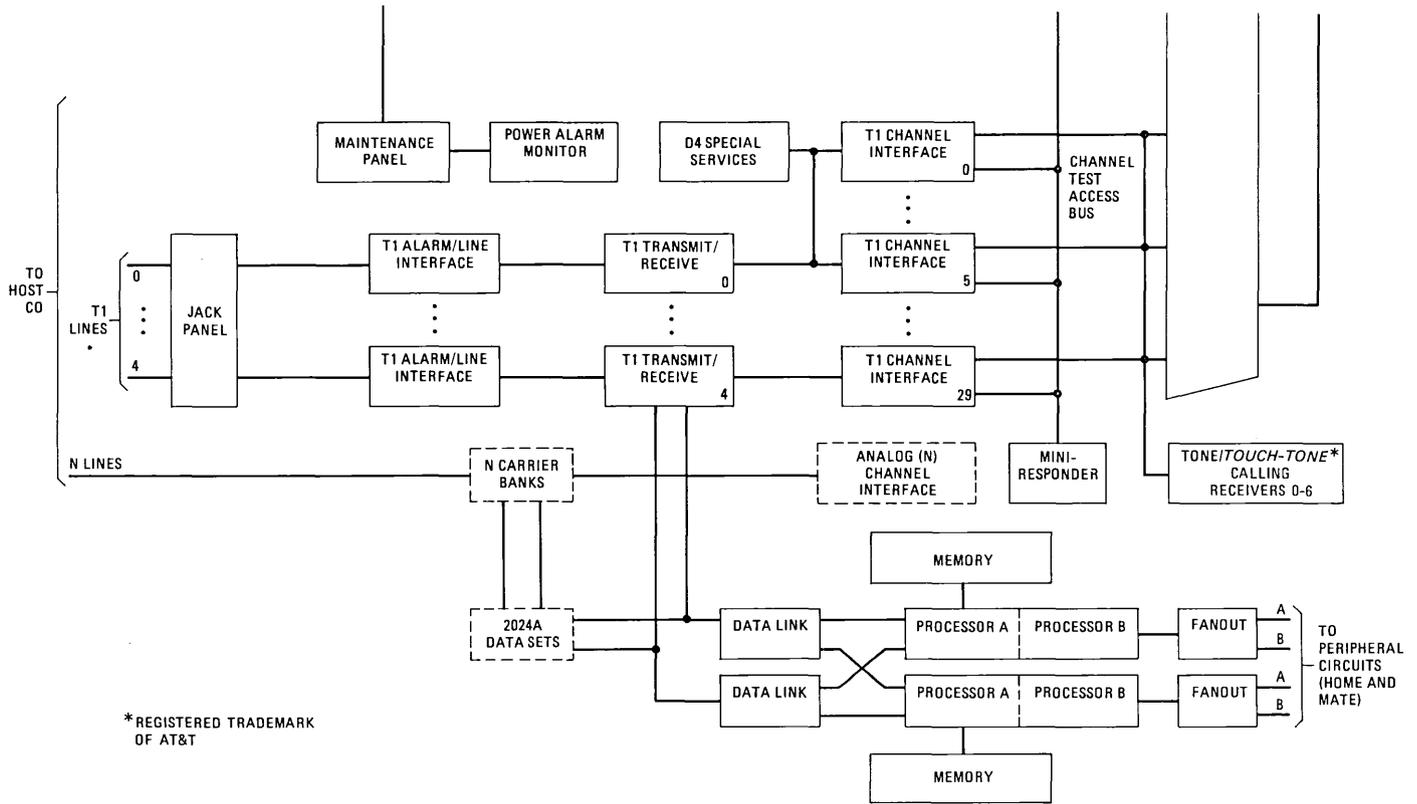
Fig. 10—No. 10A Remote Switching System block diagram.
