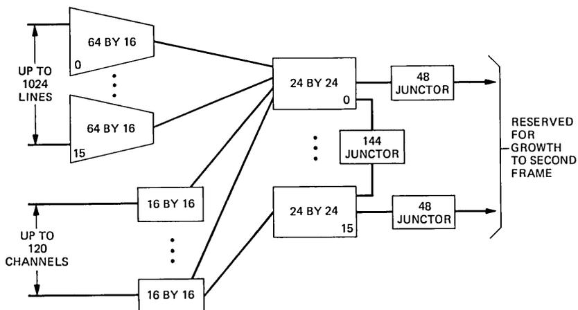
Fig. 6—No. 10A rss switching network, 512 to 1024 lines.
