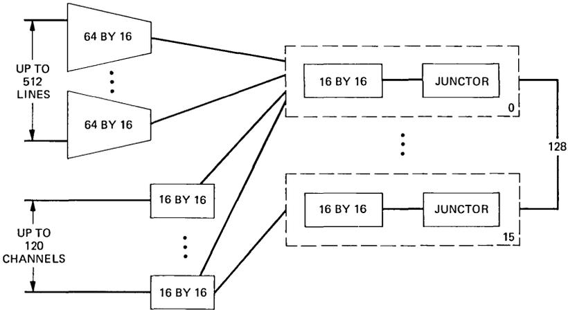
Fig. 5—No. 10A rss switching network, 0 to 512 lines.
