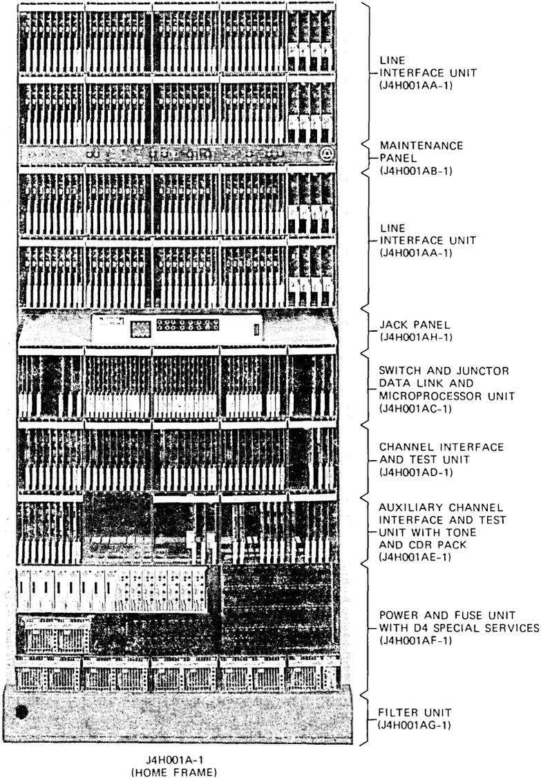
Fig. 9—No. 10A Remote Switching System (1024 lines/120 channels).
