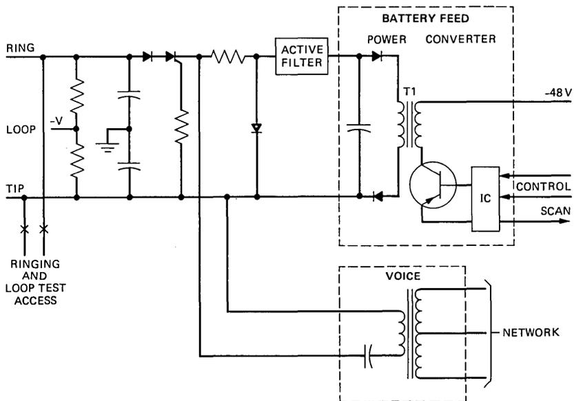
Fig. 3—Functional schematic of rss line interface circuit.
