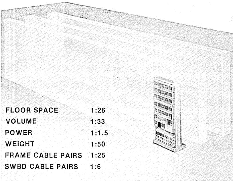
Fig. 2—Remote switching system versus step-by-step comparison (1,000-line offices).
