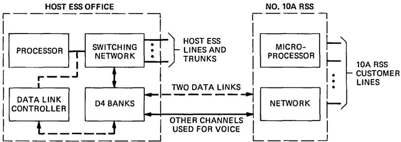
Fig. 1—Remote switching system configuration using digital carrier.
