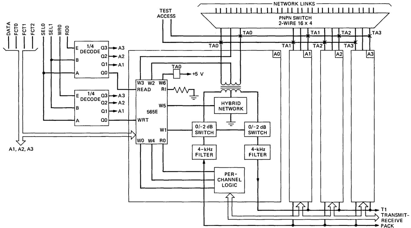
Fig. 23—No. 10A rss T1 carrier interface circuit pack.
