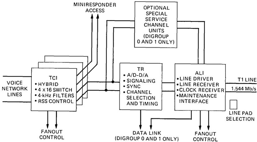
Fig. 22—No. 10A rssi internal T1 carrier interface.
