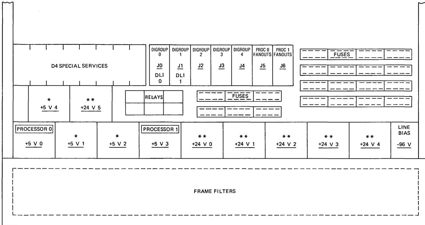
\* CONVERTERS +5 V 1, 2, 4 ARE CONNECTED IN PARALLEL TO A COMMON +5 V BUS.
