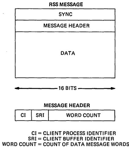
Fig. 7—Remote switching system message structure.
