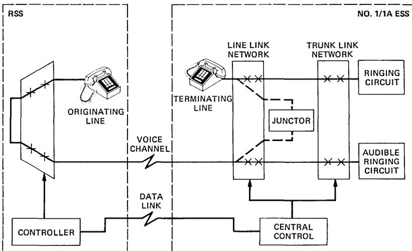
Fig. 12—Remote switching system originating call.
