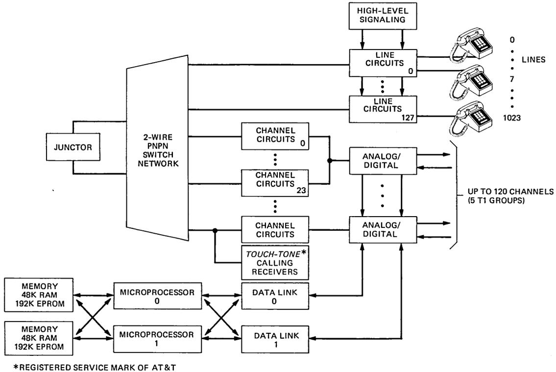
Fig. 4—No. 10A rss remote terminal hardware.
