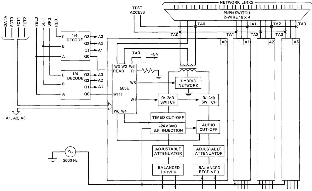
Fig. 25—No. 10A RSS analog carrier interface circuit pack.
