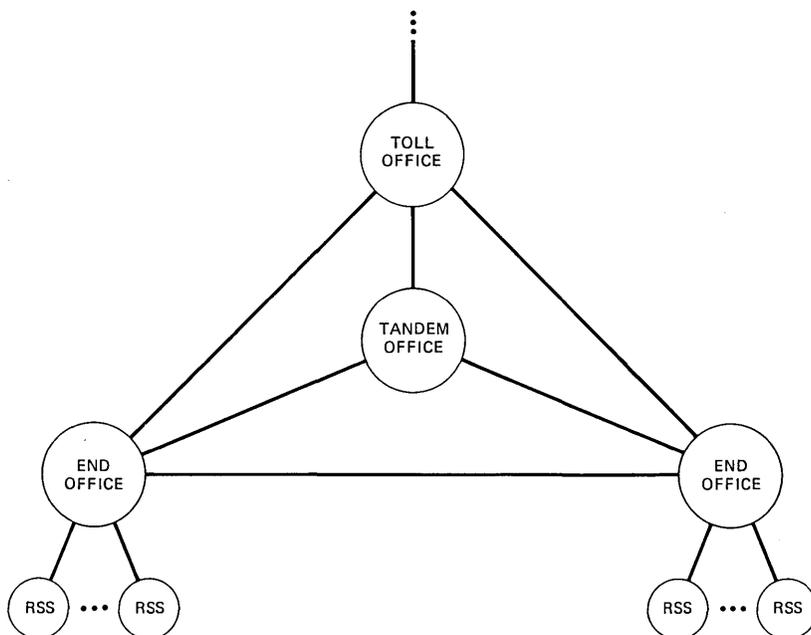
Fig. 9—Position in switching hierarchy.
