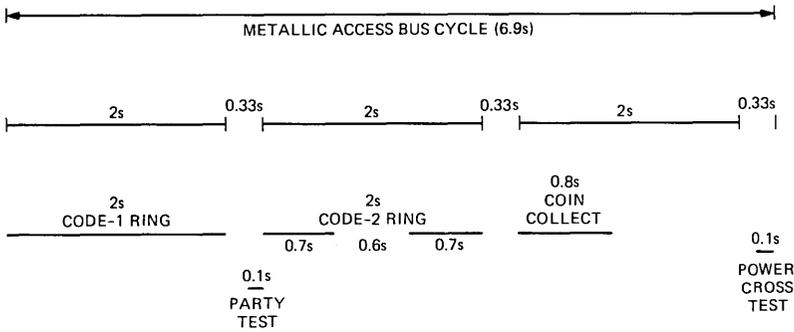
Fig. 20—Metallic access network timing.
