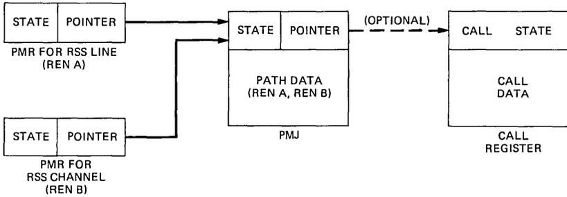
Fig. 3—Two-terminal RSS path memory configuration.
