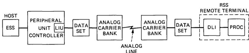
Fig. 7—Block diagram of analog carrier data link.
