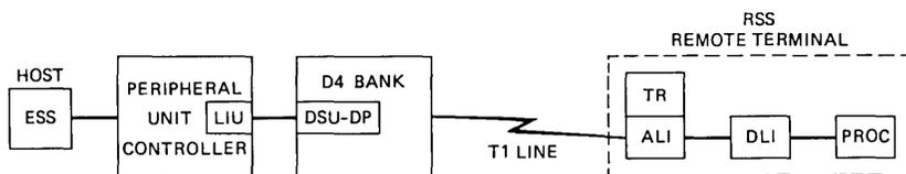
Fig. 6—Block diagram of digital carrier data link.
