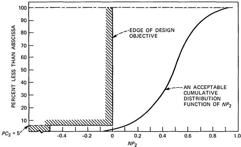
Fig. 12—Representative attenuation distortion design objective for an FX line.
