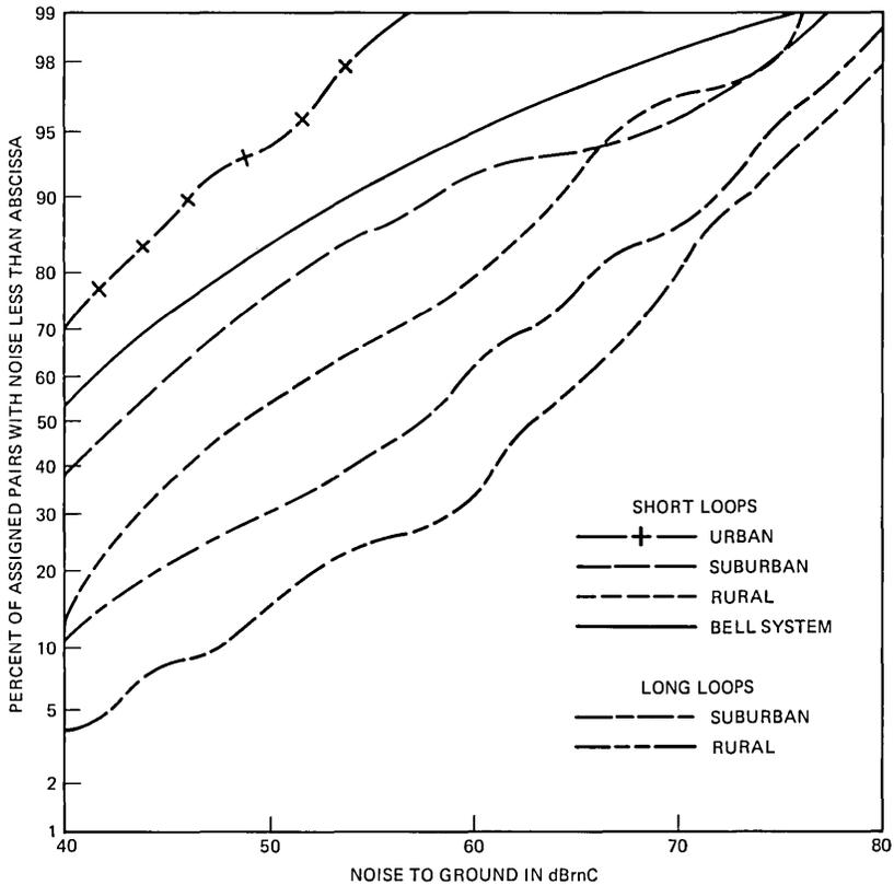
Fig. 5—Central office C-message weighted noise to ground for long (>20 kft) and short ( $\leq 20$  kft) loops.
