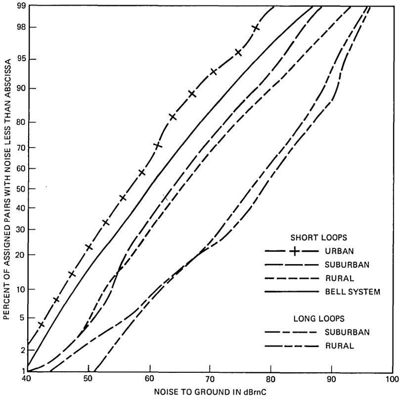
Fig. 17—Main station C-message weighted noise to ground for long (>20 kft) and short ( $\leq 20$  kft) loops.
