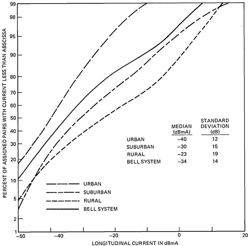
Fig. 8—Central office longitudinal current for urban, suburban, rural, and Bell System loop populations.
