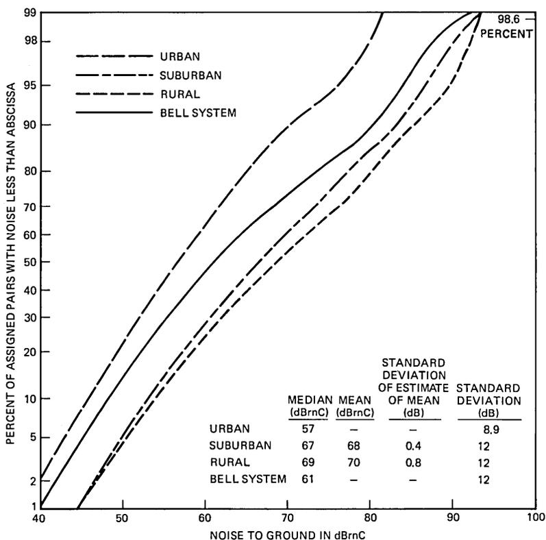
Fig. 16—Main station C-message weighted noise to ground for urban, suburban, rural, and Bell System loop populations.
