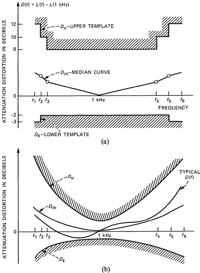
Fig. 7—Template and median curves for attenuation distortion objective: (a) Attenuation distortion objective; (b) smoothed attenuation distortion objective.
