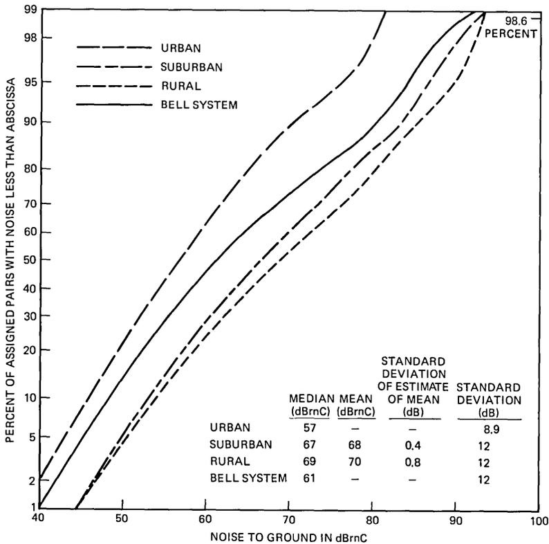
Fig. 29—Main station C-message weighted noise to ground for urban, suburban, rural, and Bell System loop populations.
