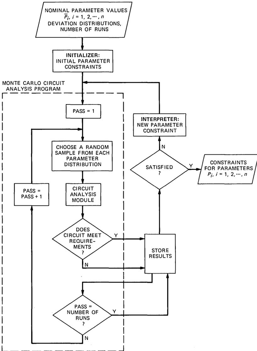
Fig. 13—Statistical analysis procedure.
