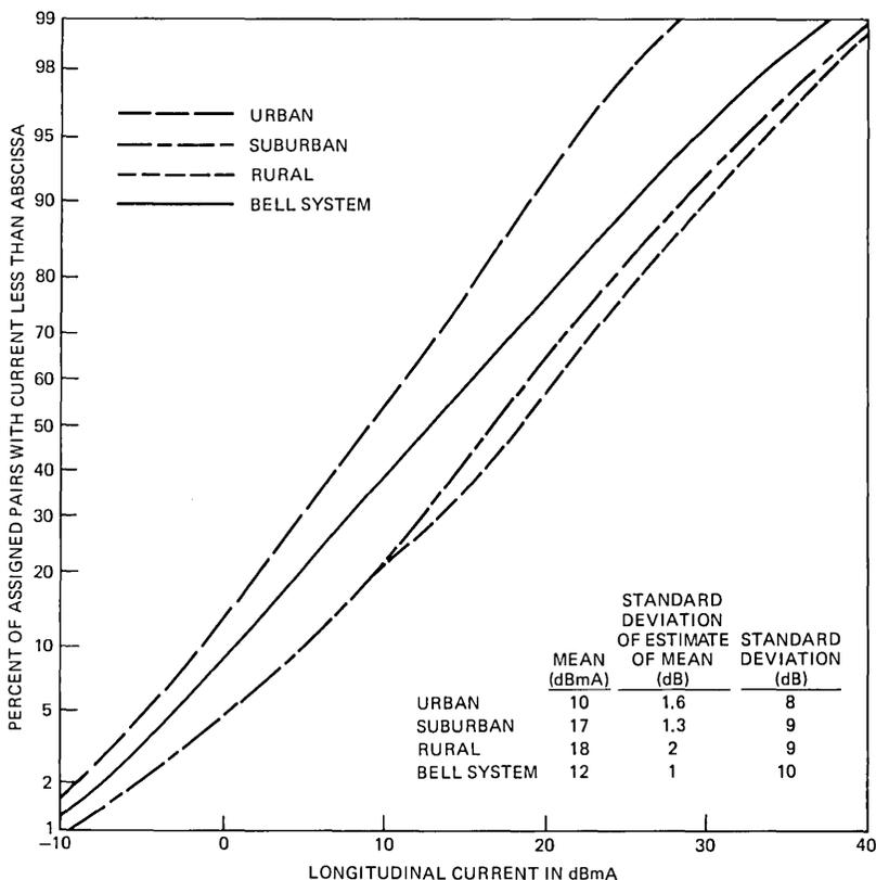
Fig. 21—Main station longitudinal current for urban, suburban, rural, and Bell System loop populations.
