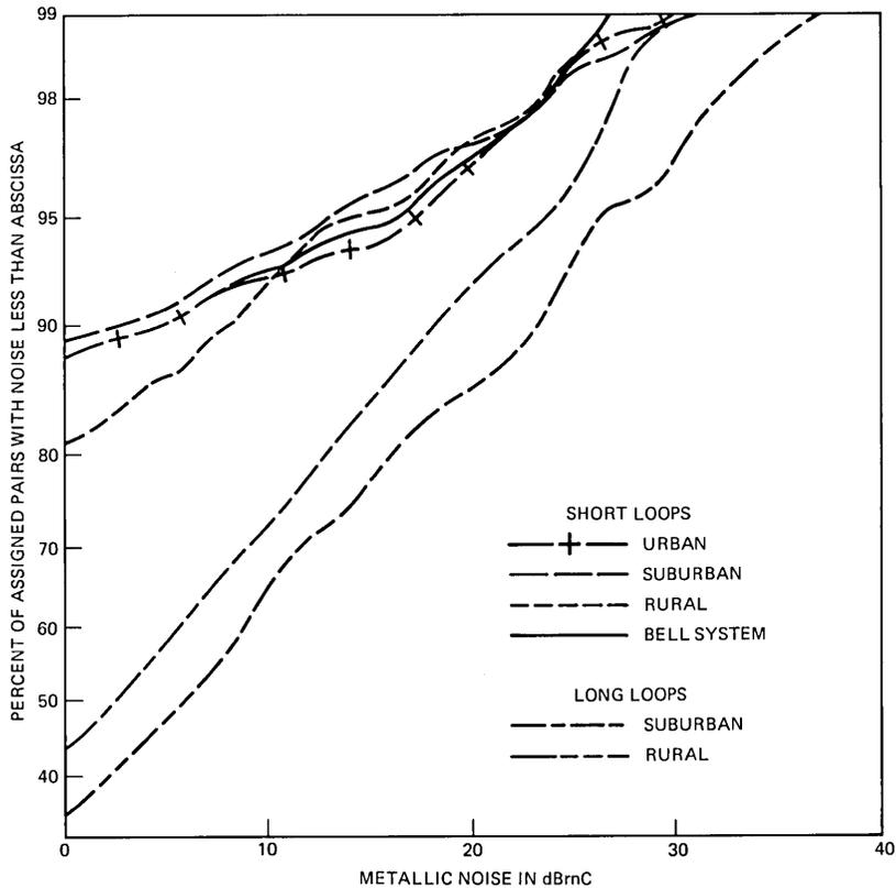
Fig. 23—Main station C-message weighted metallic noise as measured to main distributing frame for long (>20 kft) and short ( $\leq 20$  kft) loops.
