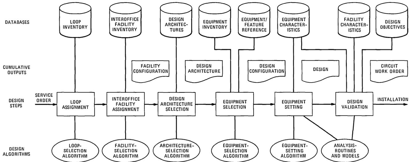
Fig. 2—Process flow in the provisioning of network services circuits.
