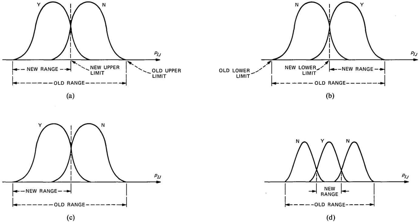
Fig. 15—Typical “Y” and “N” histograms for equipment parameter  $p_{IJ}$ . (a) One-sided parameter with upper limit. (b) One-sided parameter with lower limit. (c), (d) Two-sided parameter.
