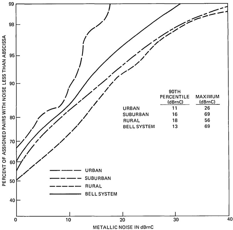
Fig. 24—Main station C-message weighted metallic noise as measured to quiet termination for urban, suburban, rural, and Bell System loop populations.
