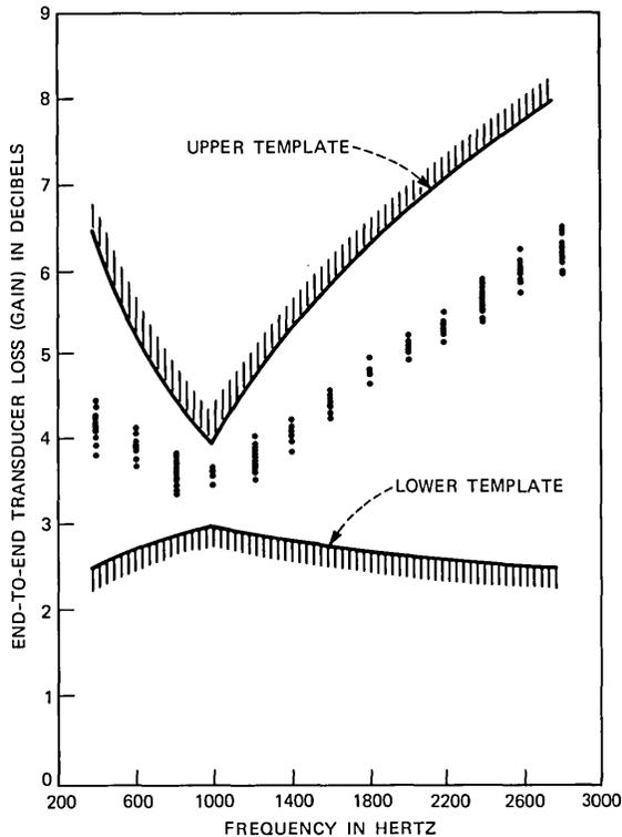
Fig. 8—Gain-frequency response with typical return-loss performance.
