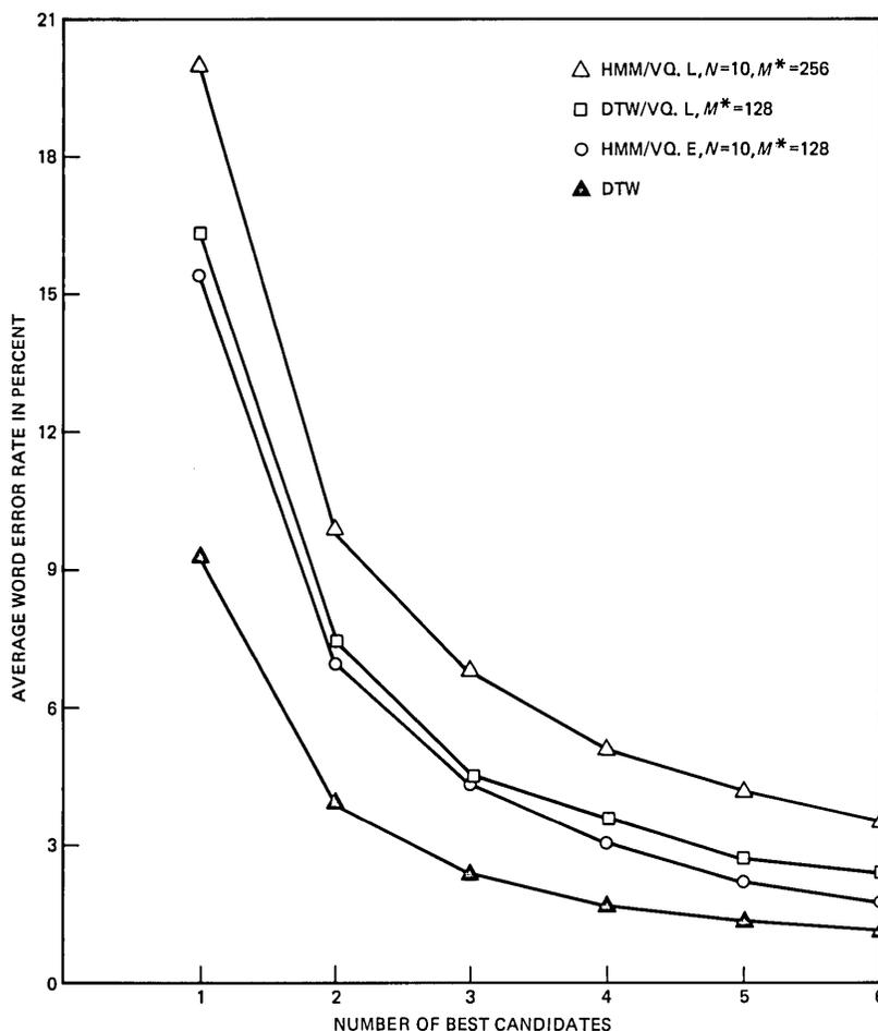
Fig. 4—Average word error rate in percent as a function of the number of best candidates for the airlines vocabulary for each of four recognition systems.
