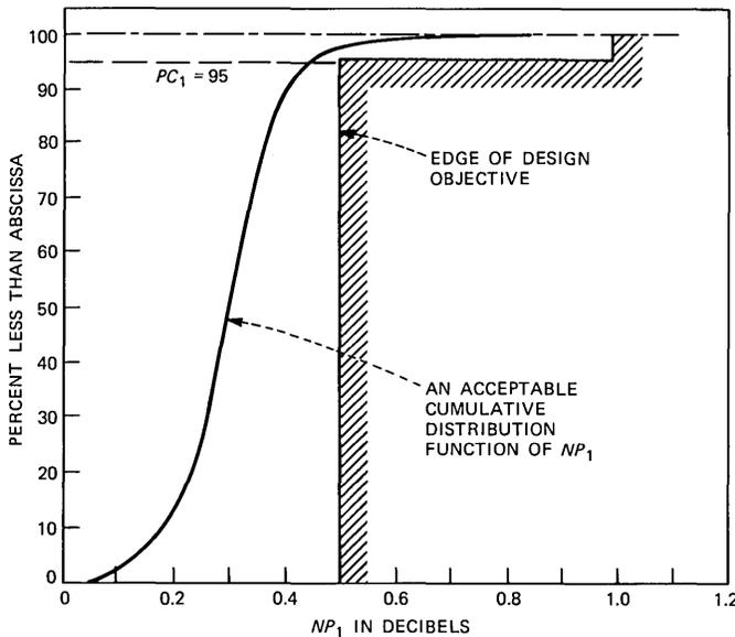
Fig. 10—Representative transducer-loss design objective for an FX line.
