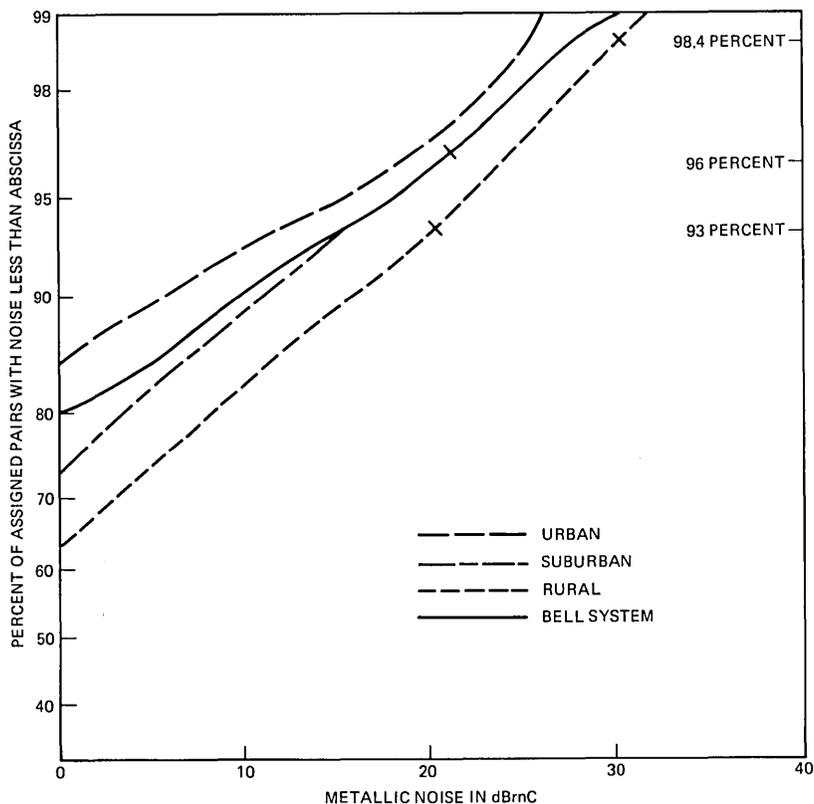
Fig. 22—Main station C-message weighted metallic noise as measured to main distributing frame for urban, suburban, rural, and Bell System loop populations.
