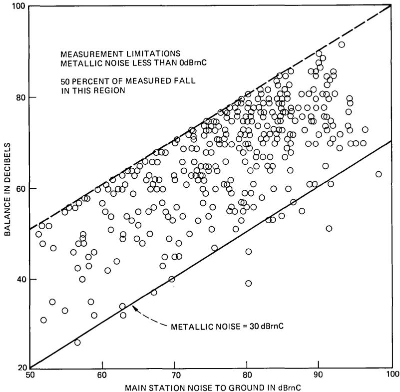
Fig. 26—Main station balance versus C-message weighted noise to ground.
