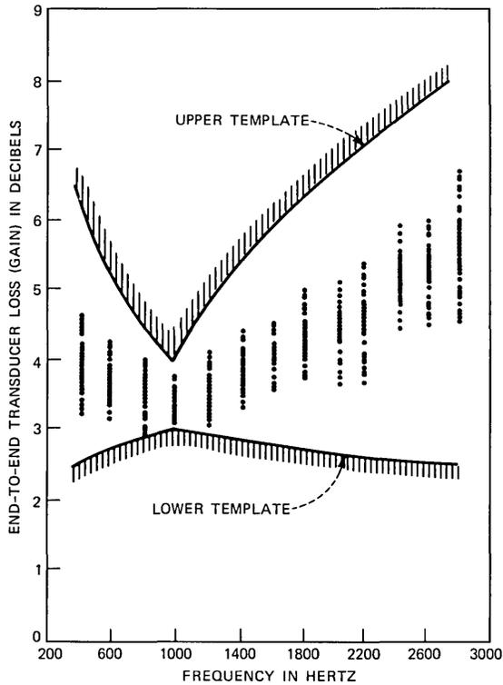
Fig. 9—Gain-frequency response with degraded return-loss performance.
