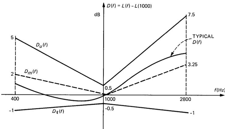
Fig. 11—Piecewise linear template and median curve for attenuation distortion design objective of an FX line.
