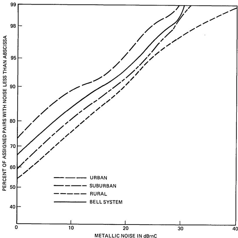
Fig. 12—Central office C-message weighted metallic noise to on-hook main station for urban, suburban, rural, and Bell System loop populations.
