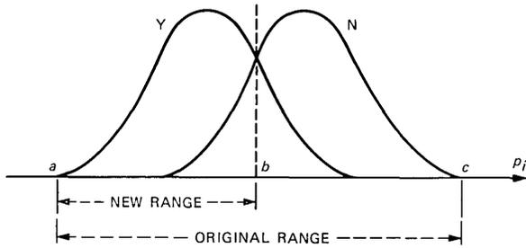
Fig. 16—Histograms of parameter  $p_i$  corresponding to circuits that meet the requirements “Y” or do not meet the requirements “N”.
