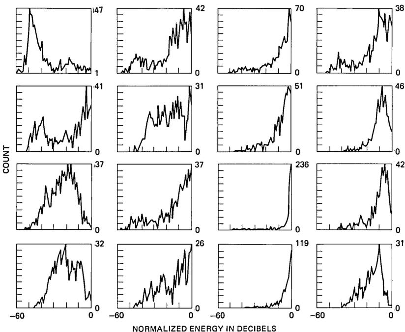
Fig. 2—Energy histograms of the 16 code words of an  $M^* = 16$  shape LPC vector quantizer.
