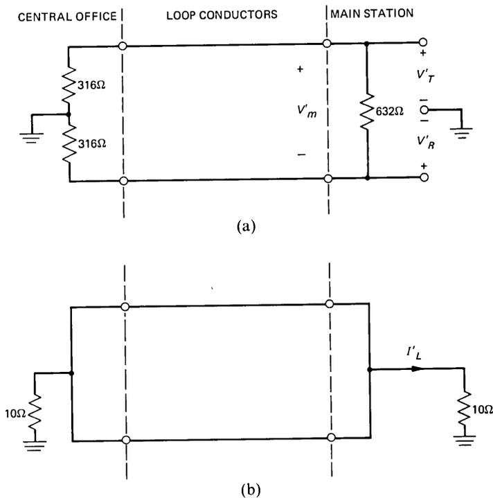
Fig. 15—Main station measurement configurations. (a) Metallic noise and noise to ground measurements. (b) Longitudinal current measurement.
