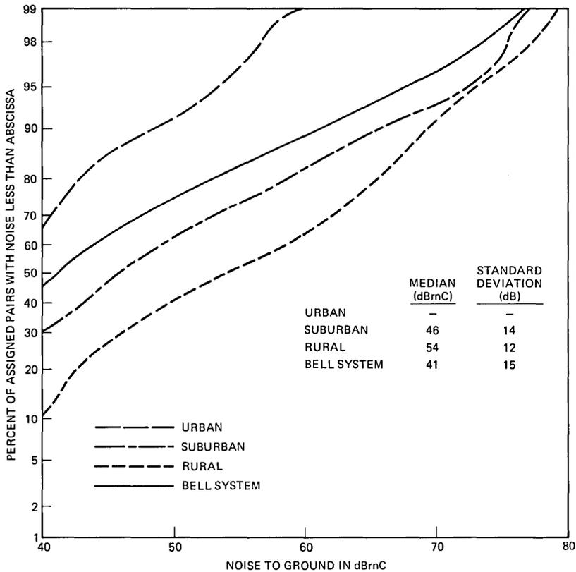
Fig. 4—Central office C-message weighted noise to ground for urban, suburban, rural, and Bell System loop populations.
