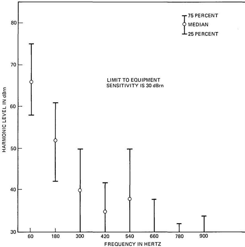
Fig. 7—Distributions of spectral levels of central office noise to ground.
