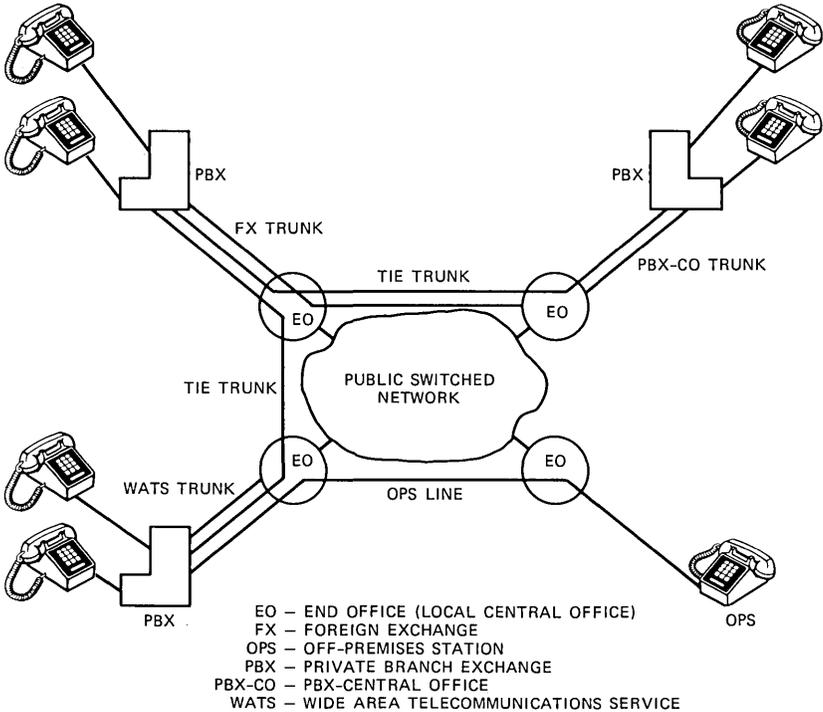
Fig. 1—Typical special services circuits.
