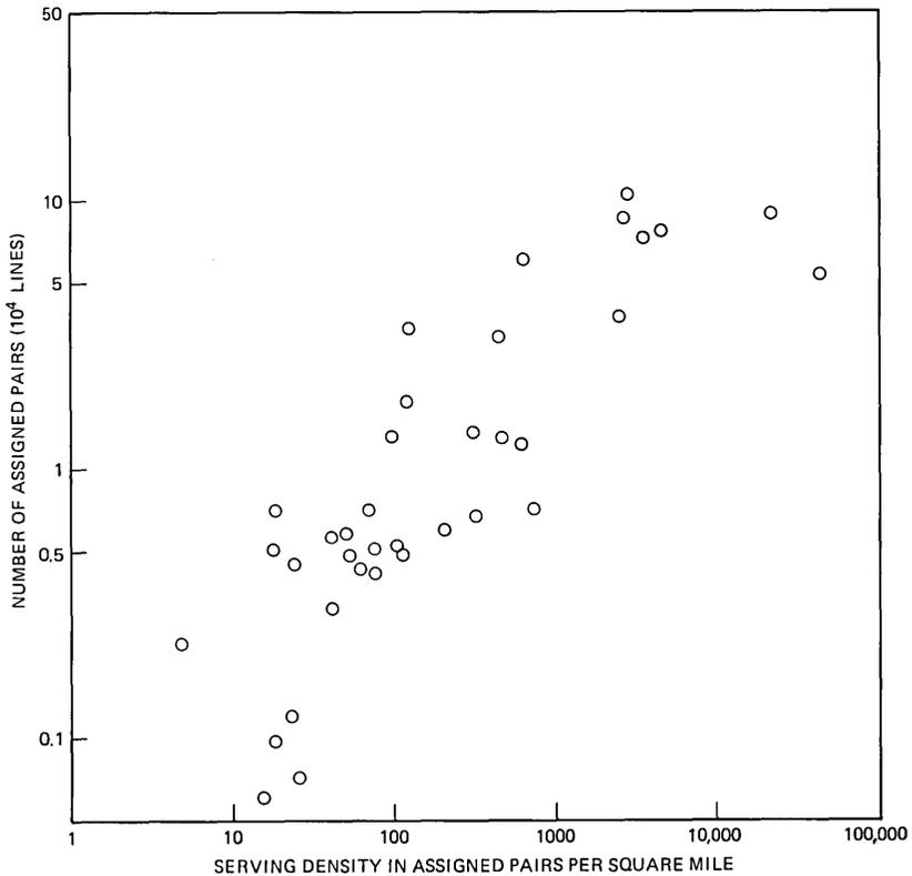
Fig. 27—Sampled wire center size versus serving density.
