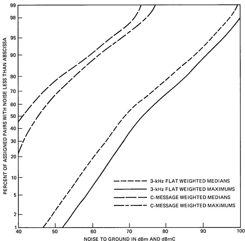
Fig. 6—Central office median and maximum noise to ground in a 24-hour period.
