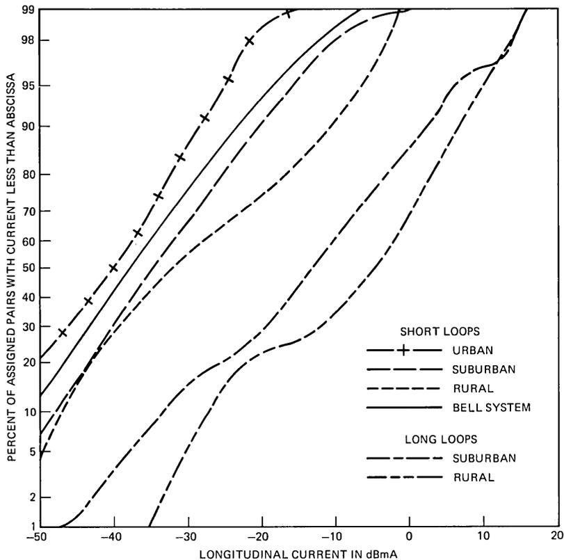
Fig. 10—Central office longitudinal current for long (>20 kft) and short ( $\leq 20$  kft) loops.
