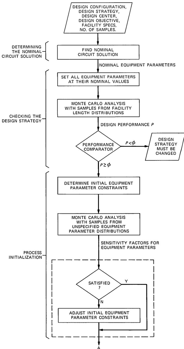
Fig. 14—Basic flowchart of the equipment requirement optimization process.
