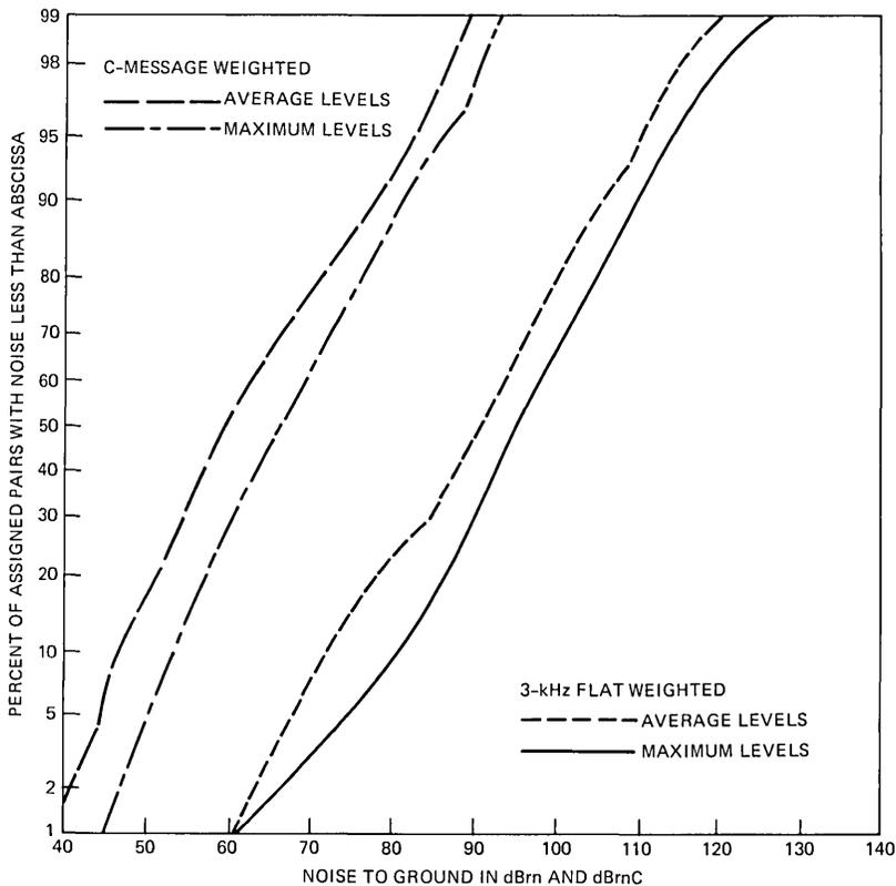
Fig. 19—Maximum and average main station noise to ground in a 24-hour period.
