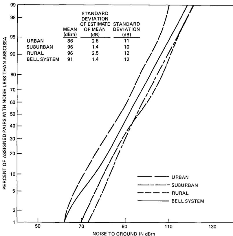
Fig. 18—Main station noise to ground for urban, suburban, rural, and Bell System loop populations.
