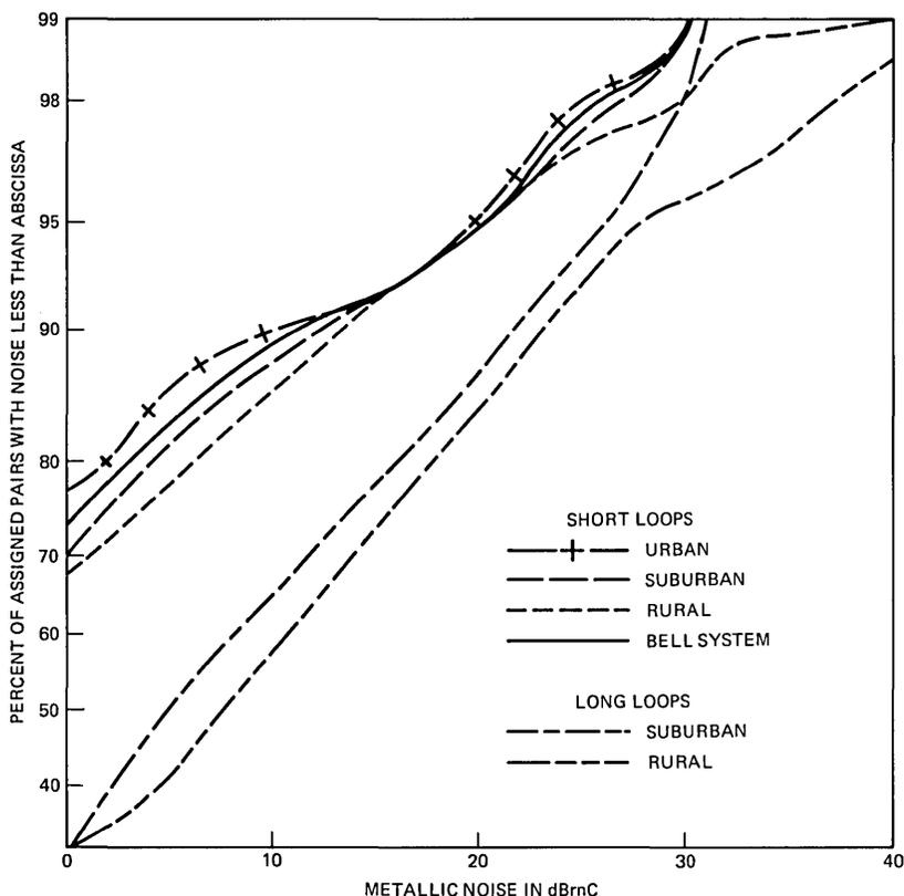
Fig. 14—Central office C-message weighted metallic noise to on-hook station for long (>20 kft) and short ( $\leq 20$  kft) loops.
