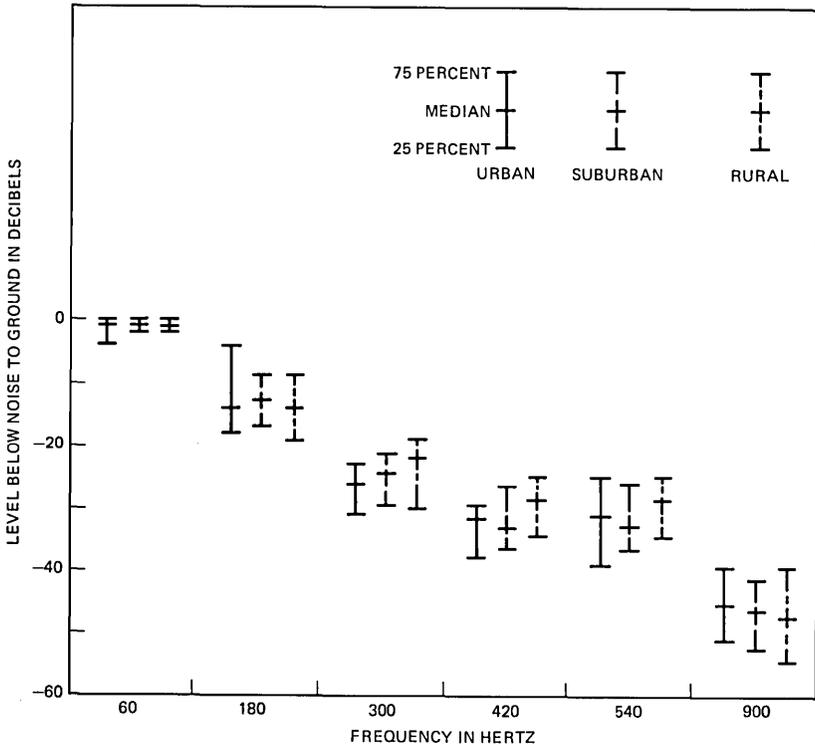
Fig. 20—Distributions of normalized spectral components of main station noise to ground.
