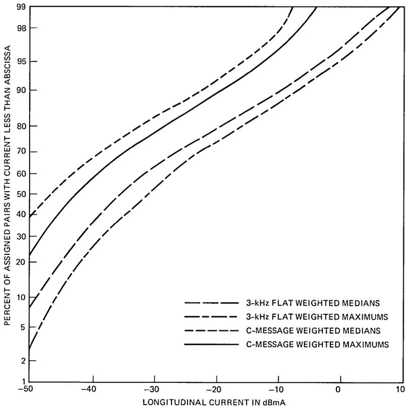
Fig. 11—Central office median and maximum longitudinal current in a 24-hour period.
