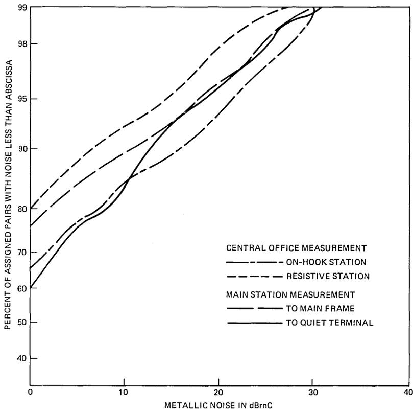
Fig. 25—Comparison of central office and main station metallic noise distributions.
