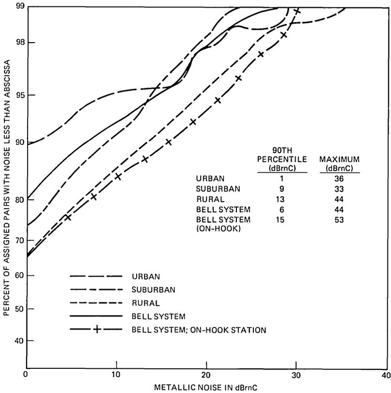
Fig. 13—Central office C-message weighted metallic noise to off-hook main station for urban, suburban, rural, and Bell System loop populations.
