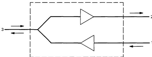
Fig. 5—A 4-wire to 2-wire (or 2-wire to 4-wire) generic segment.
