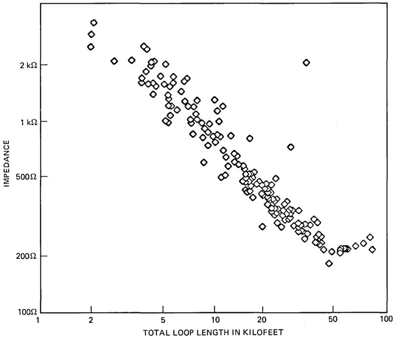
Fig. 9—Central office longitudinal impedance at 540 Hz versus total loop length.
