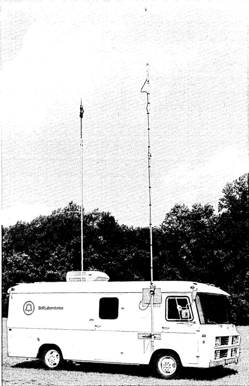
Fig. 2—The instrumentation van with the receiving antenna mast and the reference signal mast erected. The center of the four-element collinear receiving antenna is 27 feet above ground at the top of the mast mounted on the right side of the van near the front. The signal source is at the top of its reference mast mounted on the left side near the rear. The center of the signal-source dipole is also 27 feet above ground.
