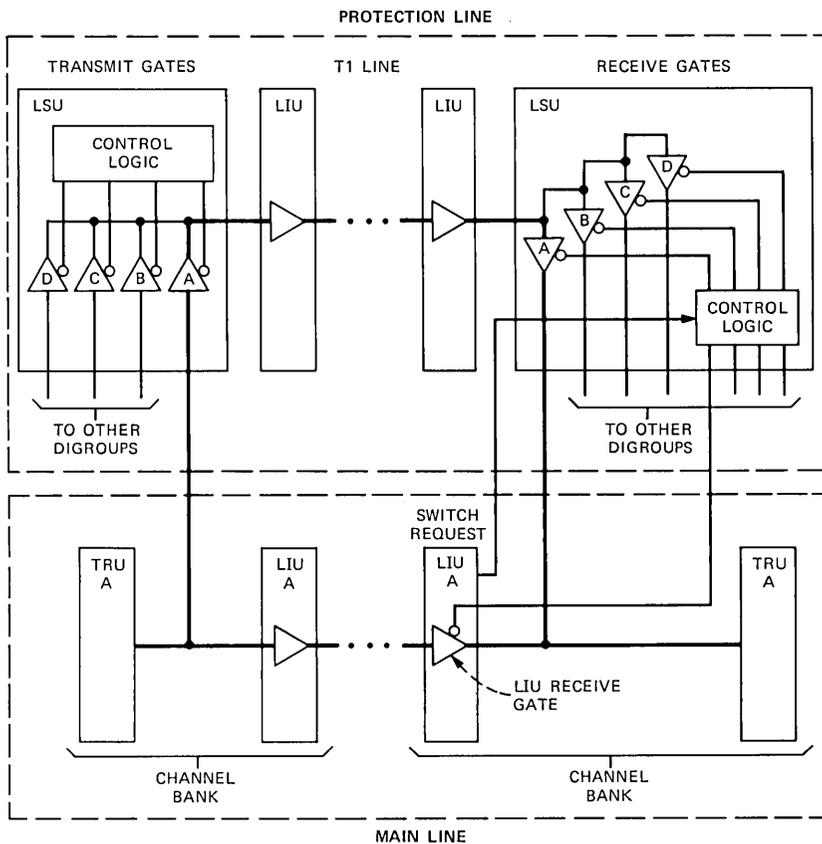
Fig. 12—Protection line switching with one direction shown.
