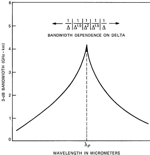
Fig. 7—Fiber spectral bandwidth for a narrow source.
