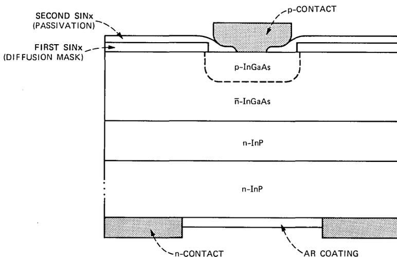
Fig. 4—Planar InGaAs PIN diode structure.
