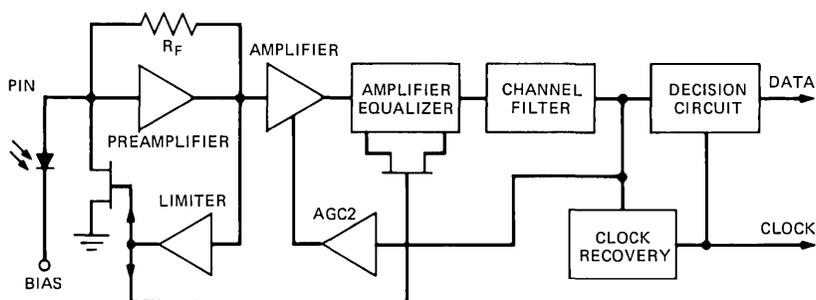
Fig. 12—Block diagram of an optical receiver.
