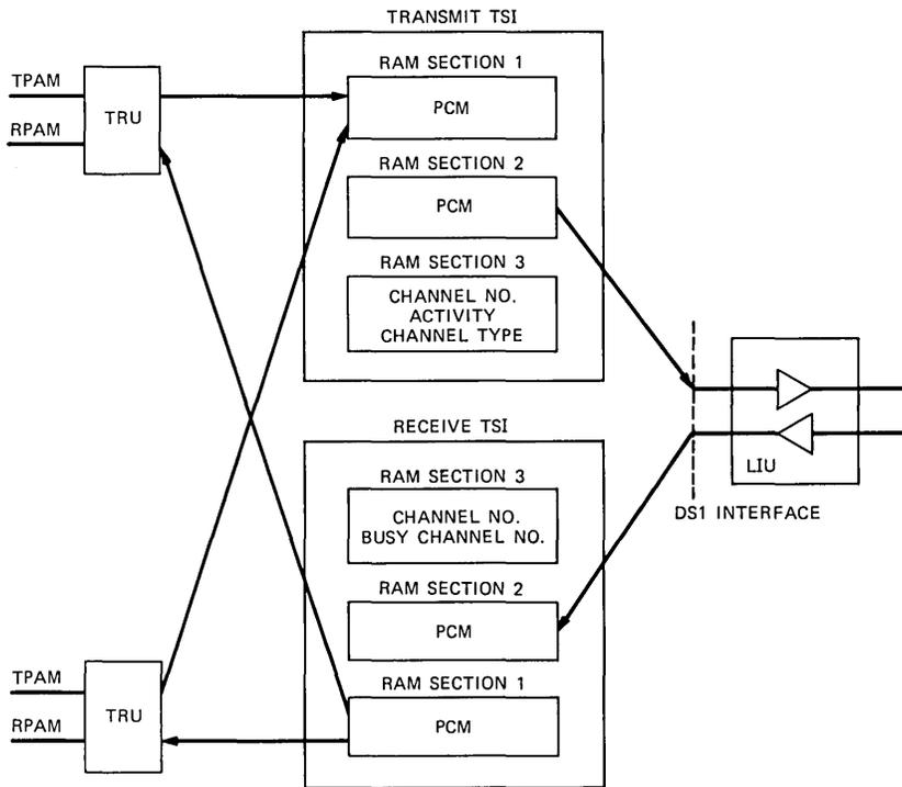
Fig. 8—Data flow through the time slot interchangers.
