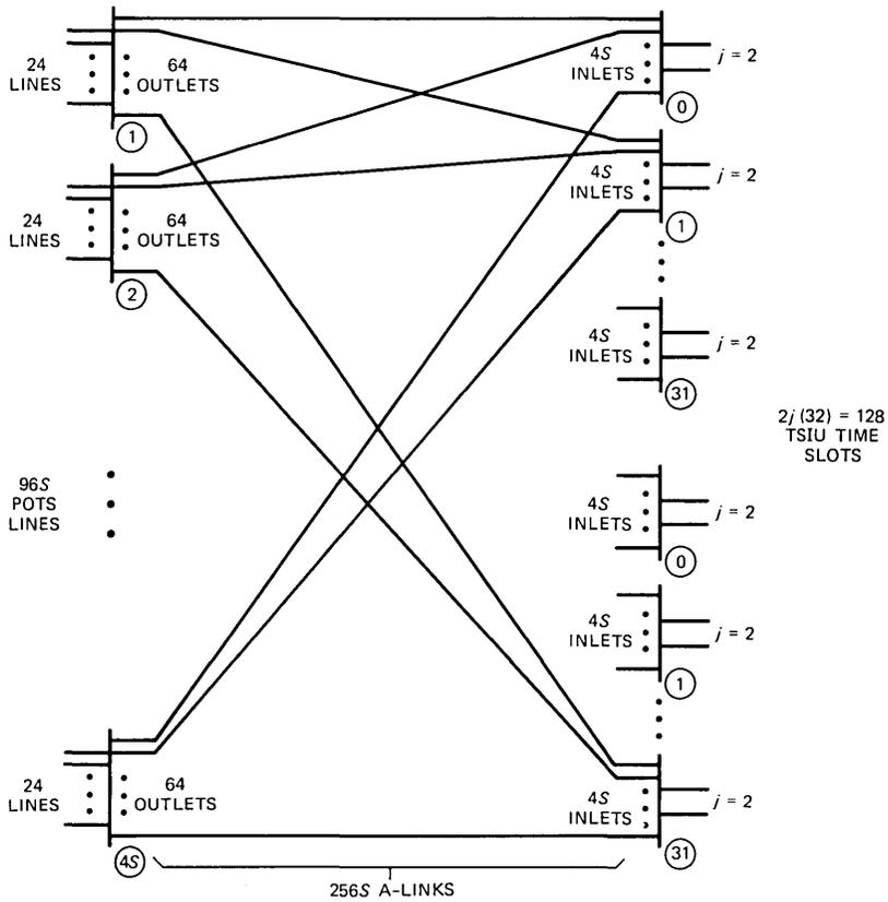
Fig. 9—DCLU switching network topology with  $S(1 \leq S \leq 6)$  Mode 1 RTs and  $j = 2$  PIDBs to TSIU from each data multiplexer.
