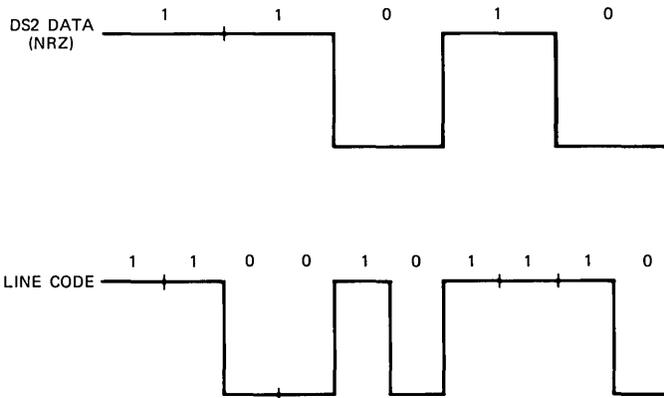
Fig. 9—Alternate dipulse coding.
