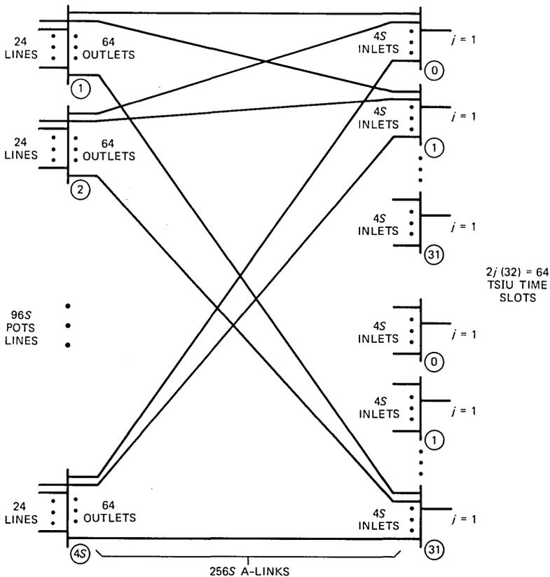
Fig. 8—DCLU switching network topology with  $S(1 \leq S \leq 6)$  Mode 1 RTs and  $j = 1$  PIDB to TSIU from each data multiplexer.
