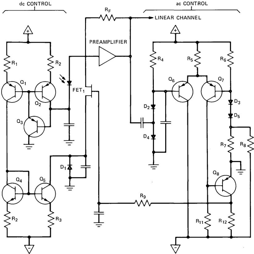
Fig. 13—Simplified circuit diagram of output limiter circuit used to increase the optical receiver dynamic range.
