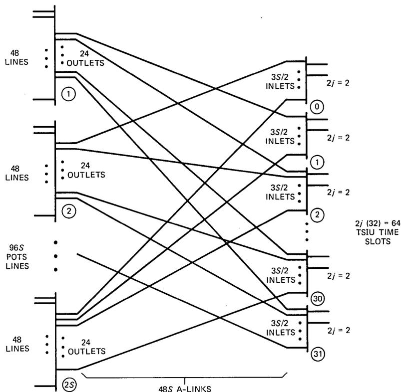
Fig. 6—RT and DCLU switching network topology with  $S(1 \leq S \leq 6)$  Mode 2 RTs and  $j = 1$  PIDB to TSIU from each data multiplexer.
