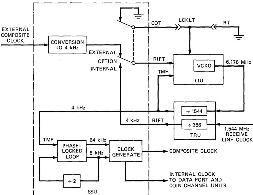
Fig. 17—System synchronization.
