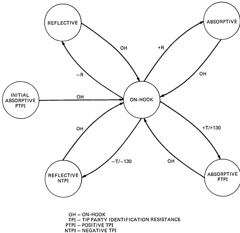
Fig. 7—State diagram for the remote terminal channel terminations.
