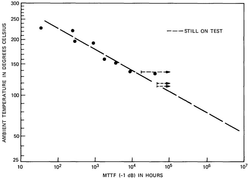
Fig. 2—Mean time to reach 1-dB degradation in output power as a function of ambient temperature. Junction temperature is 10 degrees higher than the ambient temperature.
