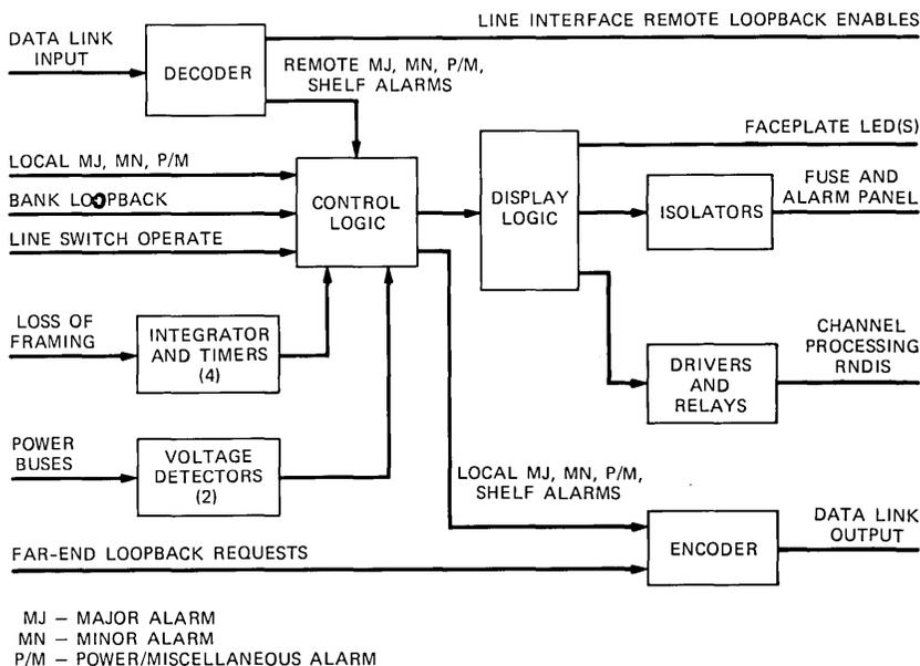
Fig. 14—Alarm control unit.
