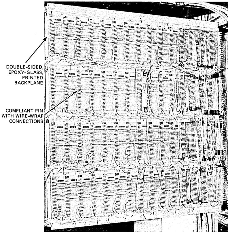
Fig. 6—SLC 96 backplane wiring.
