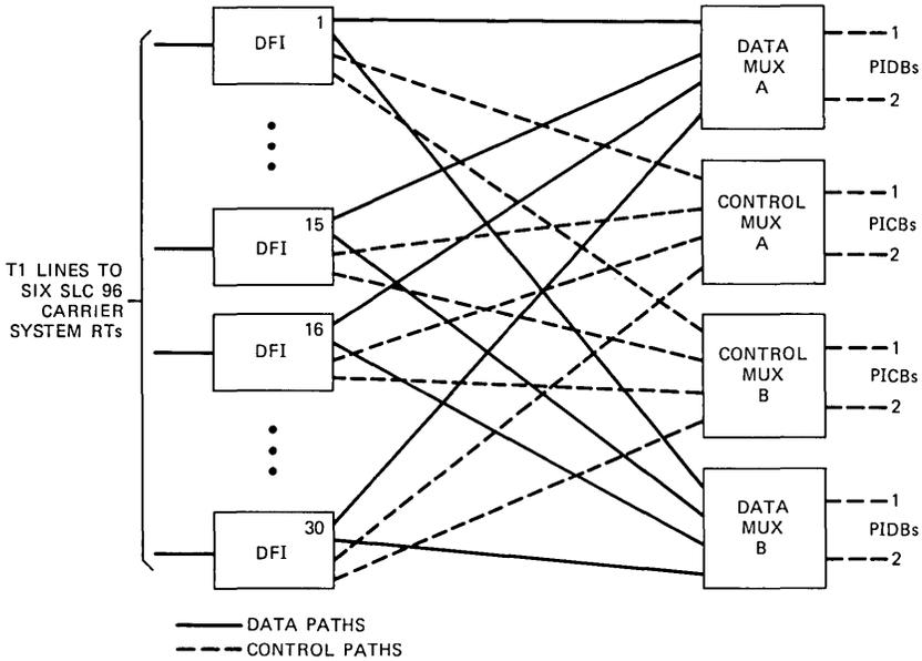
Fig. 2—5ESS switch digital carrier line unit.
