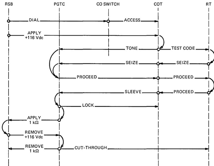
Fig. 4—Sequence to set up dc bypass path to customer's drop.
