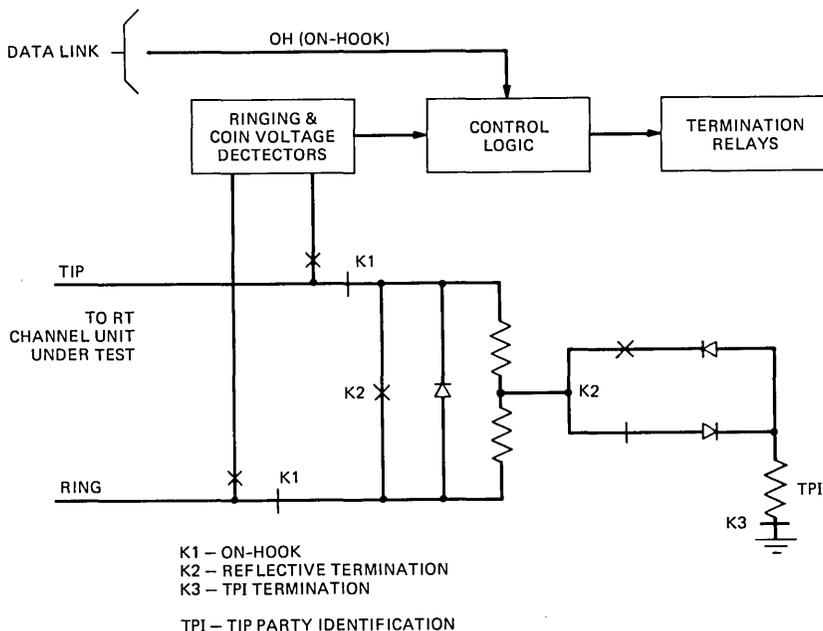
Fig. 6—Remote terminal termination circuit.
