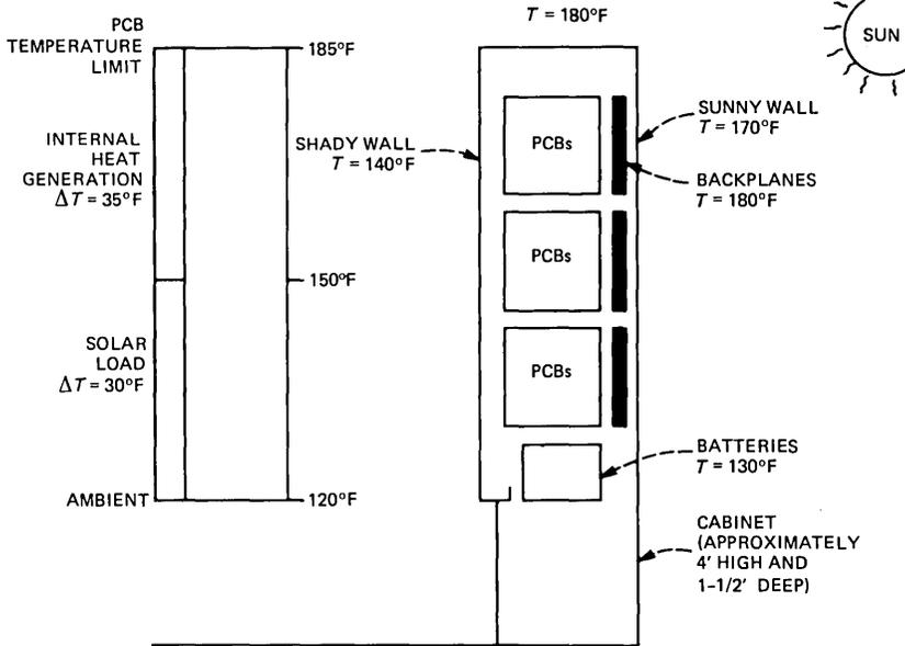
Fig. 22—Maximum temperature rises in a remote terminal cabinet.
