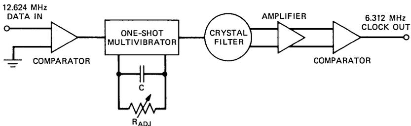
Fig. 16—Block diagram of clock recovery circuit.
