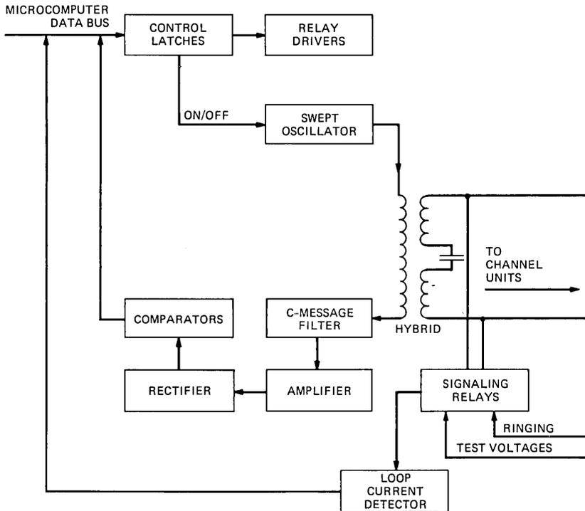
Fig. 5—The PGTC channel tester unit circuitry.
