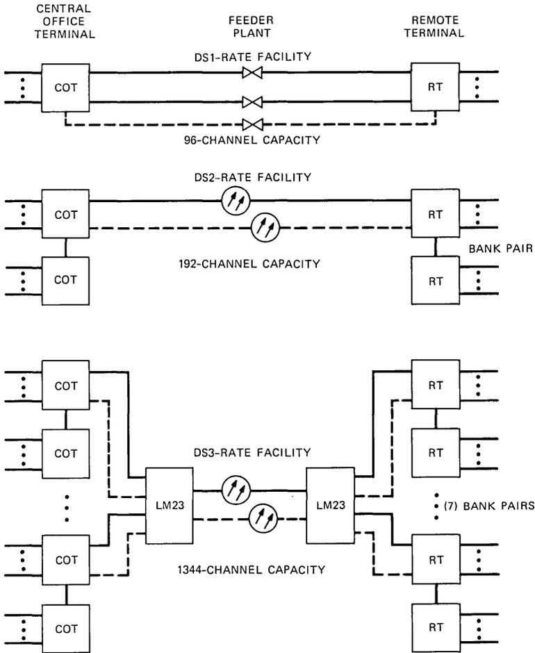
Fig. 4—SLC 96 carrier channel bank interfaces—Modes 2 and 3.
