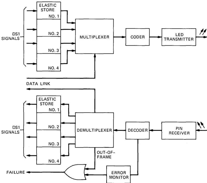
Fig. 8—Functional block diagram of the optical line interface unit.
