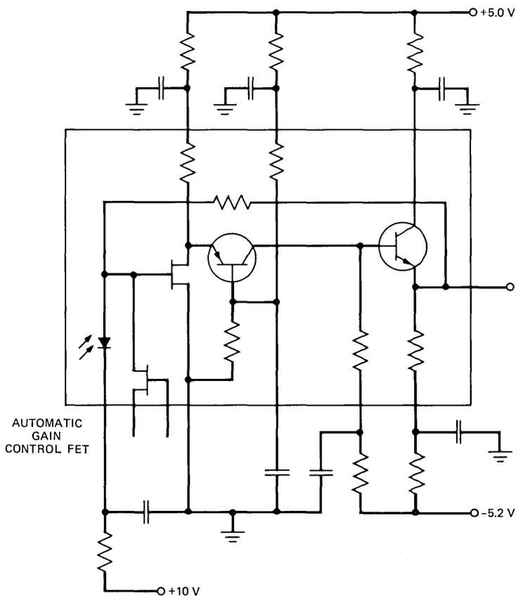
Fig. 5—1.3- $\mu\text{m}$  InGaAs PIN-GaAsFET receiver preamplifier.
