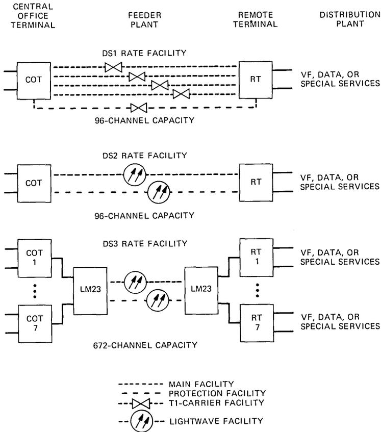
Fig. 3—Standard SLC 96 carrier channel bank interfaces.
