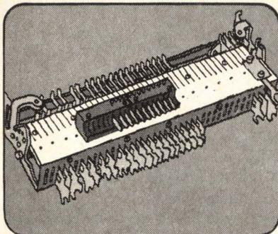
Basically, the stunt box does three things—mechanically initiates internal functions, electrically controls internal functions, and electrically controls external equipment.
