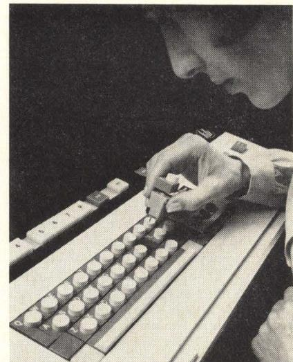
Micro Switch's KB line includes power switches (top row), alpha-numeric encoding switches (on keyboard), pushbars (bottom row), illuminated indicators (right of pushbar). All are available in a wide range of colors and shapes to permit complete design flexibility. Plug-in feature of all elements reduces assembly time and permits easy replacement.
