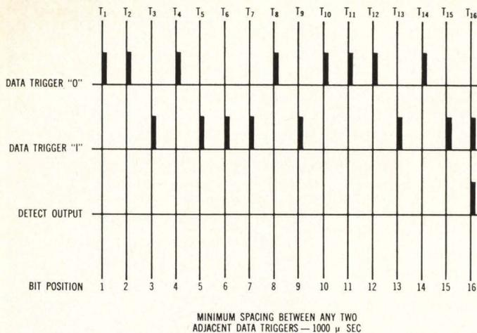
Fig. 3. Timing diagram for binary sequence detection.
