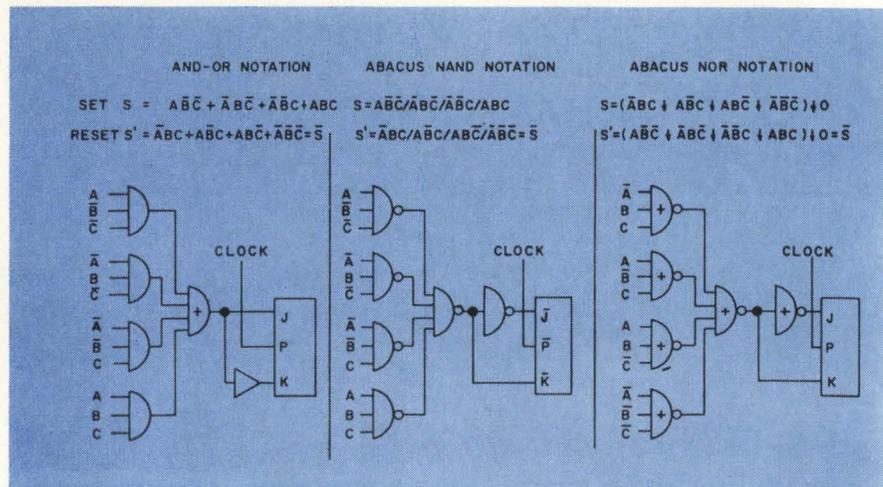
Fig. 3.5 Mechanization of a binary sum flip-flop using AND-OR, NAND, or NOR notation.
