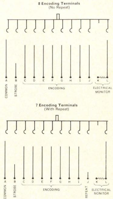
Circuit diagrams show the two types of KB encoding switches — one with 8 encoding terminals (top), the other with 7 encoding terminals plus a repeat circuit. Both types have a common terminal, a strobe terminal, and an electrical monitor circuit which can be used to determine if two switches have been pushed at the same time by mistake. The common and monitor circuits "make" first, followed by the bit outputs. The strobe circuit is delayed to eliminate bounce and noise from the output bits.
