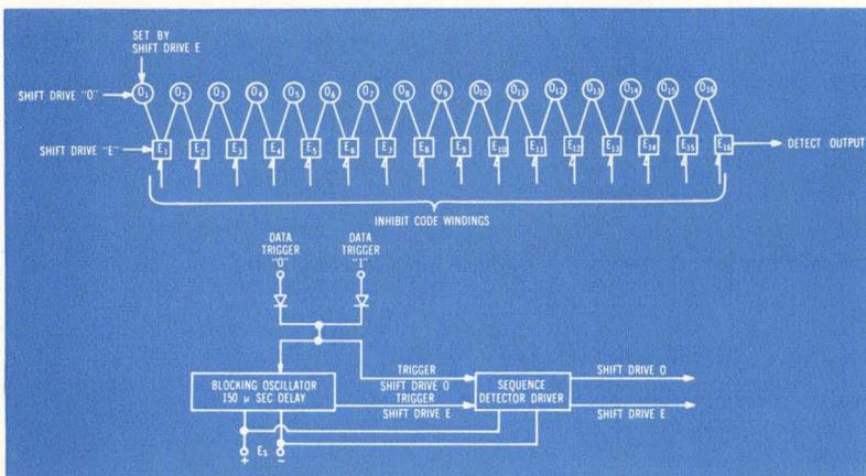
Fig. 1(b) Logic diagram for 16-bit code stream detector.
