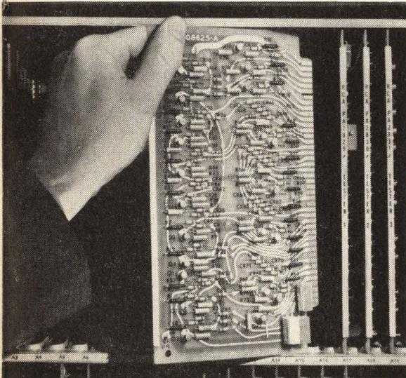
**EFFICIENT CIRCUIT BOARD DESIGN.** Vertical installation provides 86 connections per board, shorter current path.
