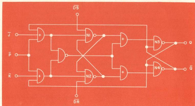
Fig. 3.3(b) Integrated circuit J-K flip-flop.
