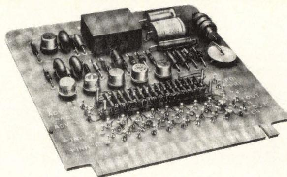
Fig. 4. The detector is mounted on a  $4\frac{1}{2} \times 5 \times \frac{3}{4}$  inch circuit board. Electrical specs include an input data rate from 0-1 kc, supply voltage from plus 24 vdc to plus 32 vdc, rise and fall times less than or equal to 0.5 usec., and signal-to-noise ratio greater than or equal to 5:1.
