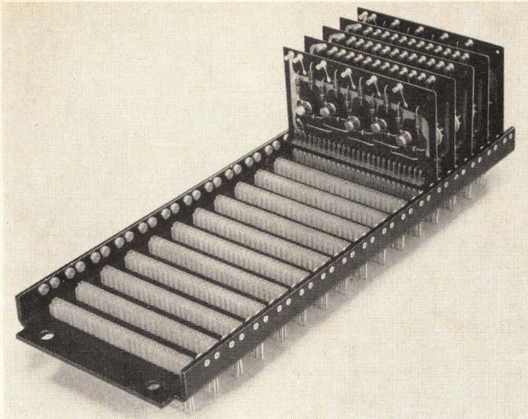
Fig. 3.2 Card cage holding I Series modules.
