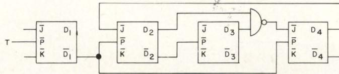
Fig. 3.6 Typical applications of the J-K flip-flop.
