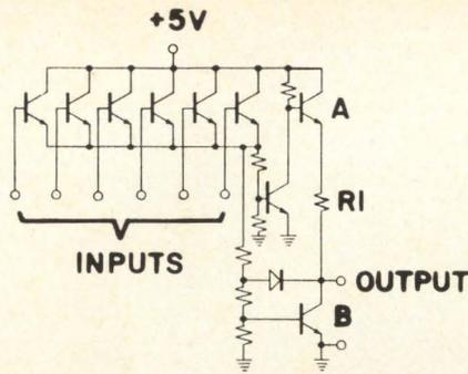
Fig. 3.3(a) The integrated circuit NAND gate made by Signetics (their Utilogic family) is used in the Abacus modules.
