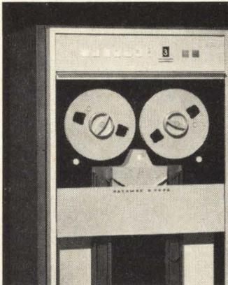
The **D 3030** writes and reads all three densities (800, 556 and 200 cpi) at 75 ips tape speed. Push-button selection of 60,000, 41,700 and 15,000 cps data transfer rates. Either 7-track or 9-track format. Vacuum column tape buffers, semi-automatic tape threading, front access to all electronics, and many other advanced features. Bi-directional start and stop times of 5 ms and 1½ ms, respectively.
