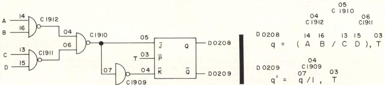
Fig. 3.7 Logic diagram and equations annotated with wiring information.
