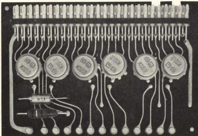
Fig. 3.1 A typical module of the Abacus I Series. This 2" x 3" module contains 6 integrated J-K clocked flip-flops or 12, 3-input NAND gates.
