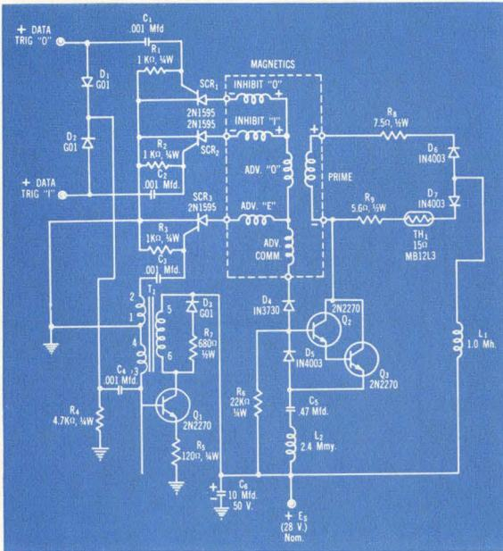
Fig. 1(a) Driver schematic for 16-bit code stream detector.
