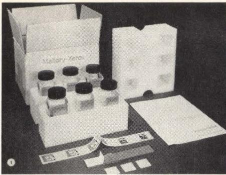
Production of a typical ac amplifier circuit using materials supplied in the new Mallory-Xerox Resistor Board Kit is shown. Photo 1 (upper left) is the complete kit which includes: three 1" x 1" thin-film resistor board wafers, a wafer mounting sheet, a set of three resistor and conductor pattern transfers, the necessary etchants and cleaners, and an instruction book. Photo 2 (center)
