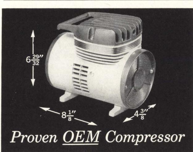
Need a compact, heavy-duty compressor or vacuum pump with a 40 p.s.i. capability in the .25 to 1.65 cfm range? Our Series 906 motor-driven diaphragm unit is a low-cost answer. Weighing only 9 pounds, it is available with a choice of 6 different curves and either a shaded pole or permanent split capacitor 115- or 230-volt, 50-60 cy. motor.
