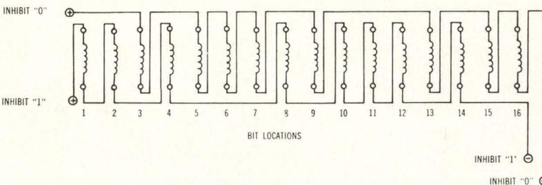
Fig. 2. Code wiring for detection of 0010111010001011.
