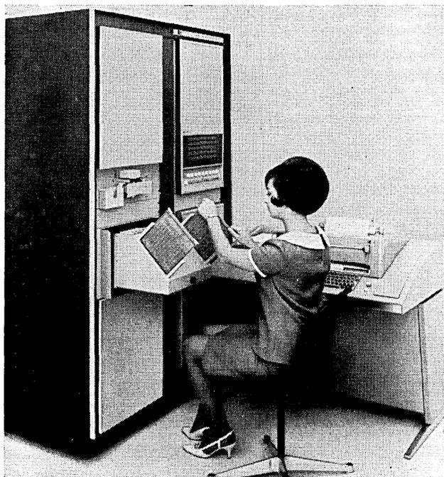
Operator compares unknown module with reference module at console of the digital logic module comparison test system.
