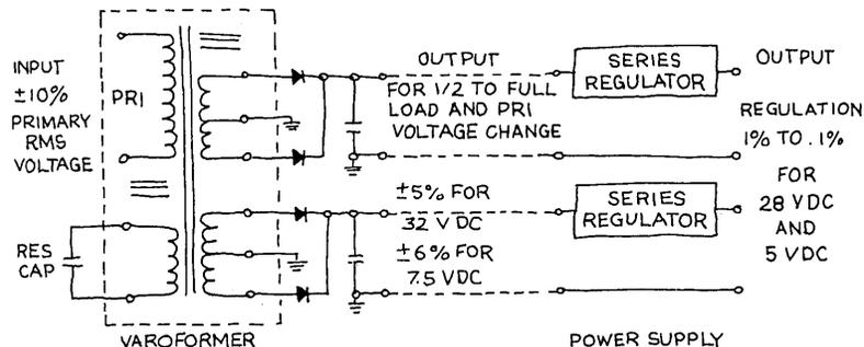
Starting with our basic Varoformer™ (constant voltage transformer) we can design power supplies to perform simple or complex functions by the addition of series regs.
