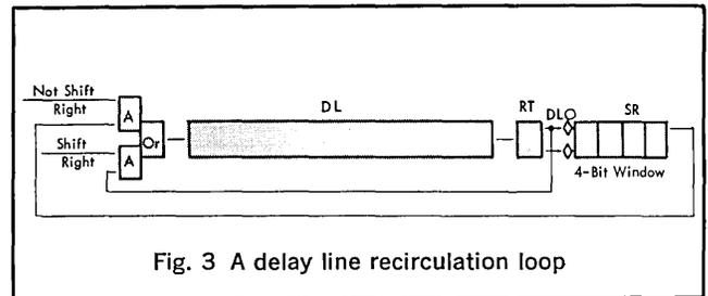
Fig. 3 A delay line recirculation loop
