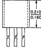
GET's package design conforms to TO-18 mounting patterns in existing PC boards. It's the ideal epoxy replacement for "hermetic devices" . . . no expensive redesign necessary.
