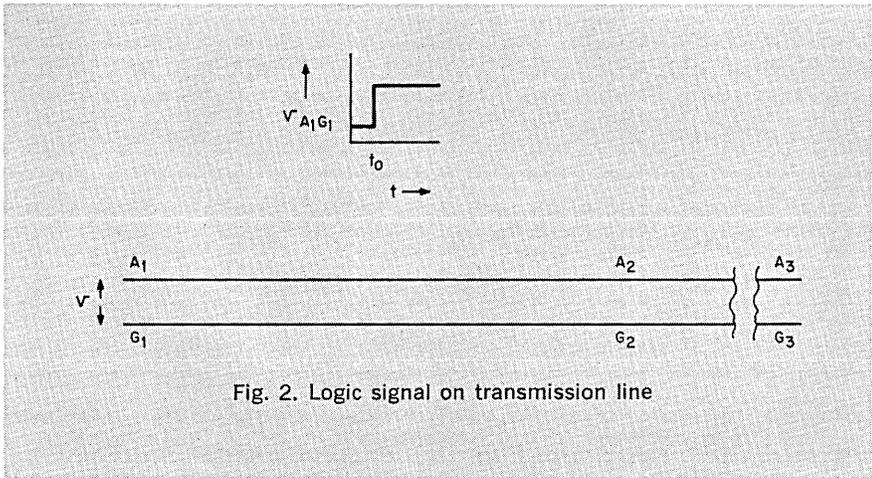
Fig. 2. Logic signal on transmission line
