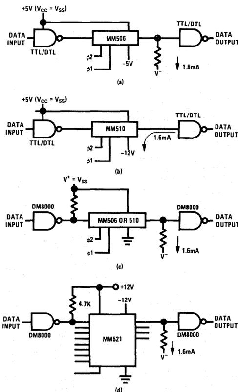
FIGURE 1. Typical TTL/MOS or DTL/MOS Interfaces.
