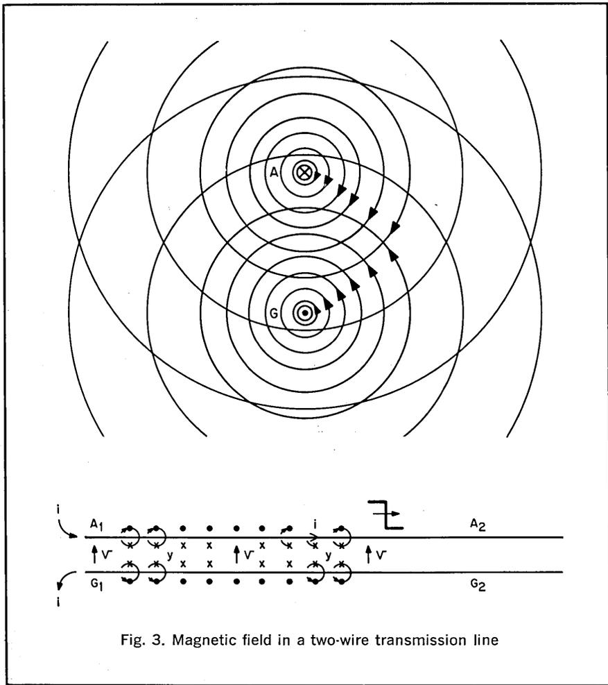
Fig. 3. Magnetic field in a two-wire transmission line
