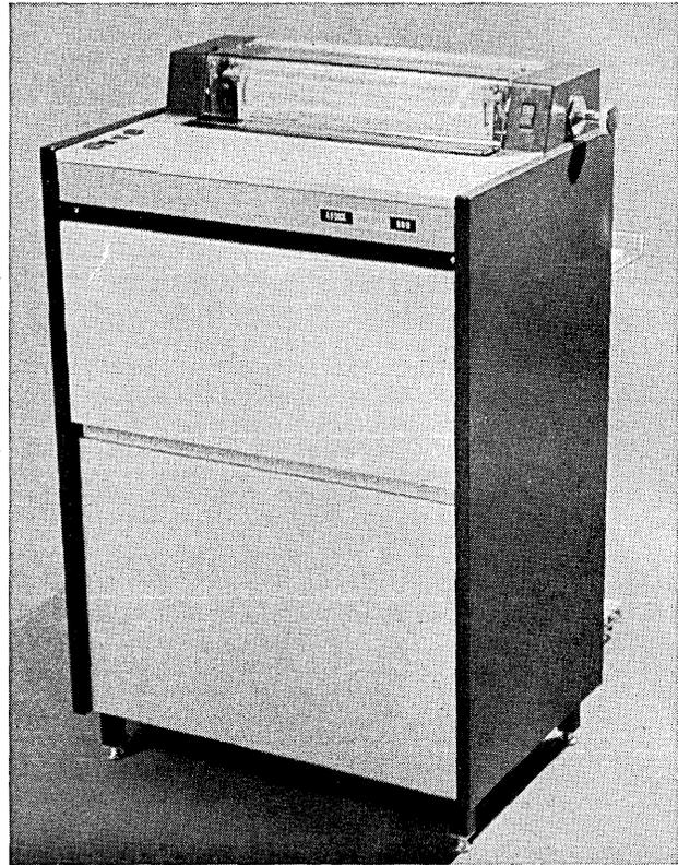
A quiet, high-speed communications printer built for remote printing via conventional voice-grade public-switched telephone lines has been developed by the A. B. Dick Company of Chicago.
