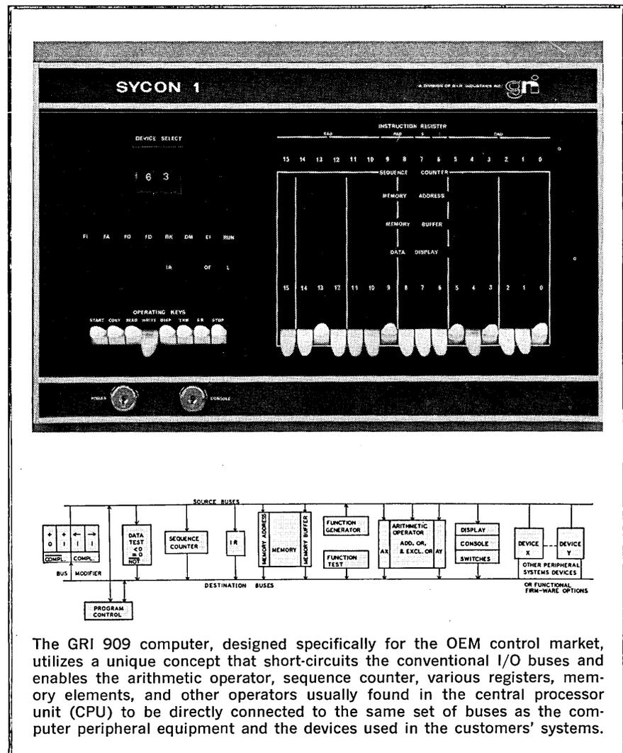
The GRI 909 computer, designed specifically for the OEM control market, utilizes a unique concept that short-circuits the conventional I/O buses and enables the arithmetic operator, sequence counter, various registers, memory elements, and other operators usually found in the central processor unit (CPU) to be directly connected to the same set of buses as the computer peripheral equipment and the devices used in the customers' systems.
