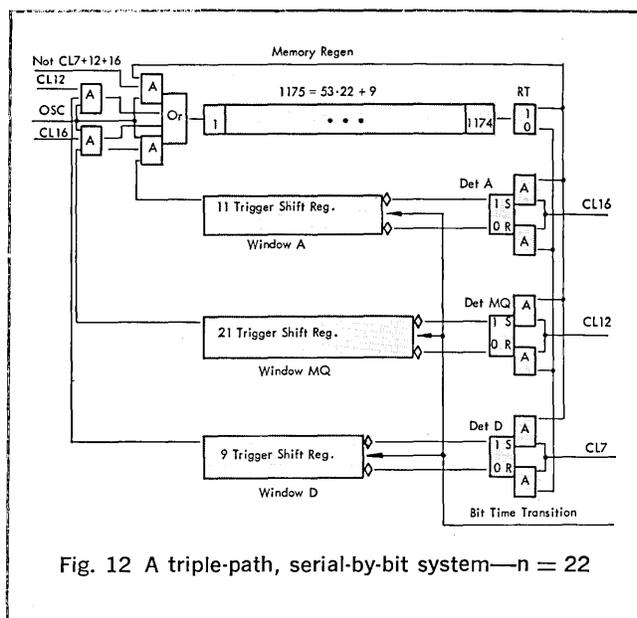
Fig. 12 A triple-path, serial-by-bit system— $n = 22$
