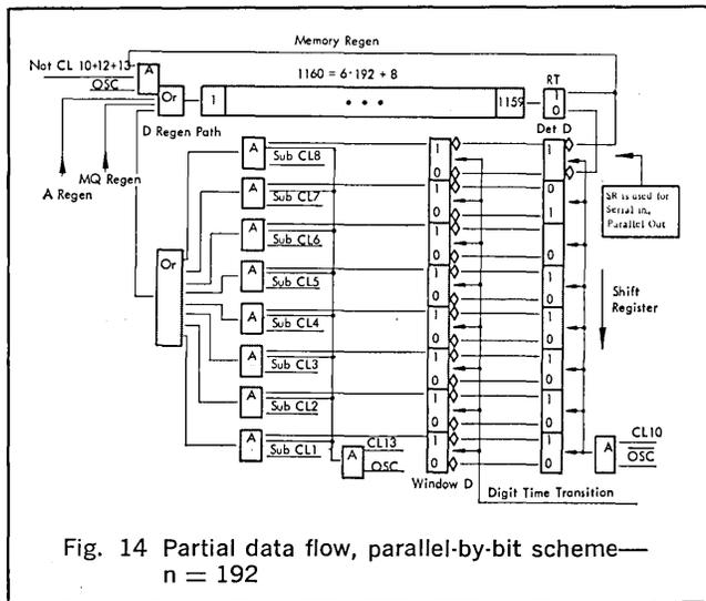
Fig. 14 Partial data flow, parallel-by-bit scheme— $n = 192$
