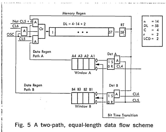
Fig. 5 A two-path, equal-length data flow scheme
