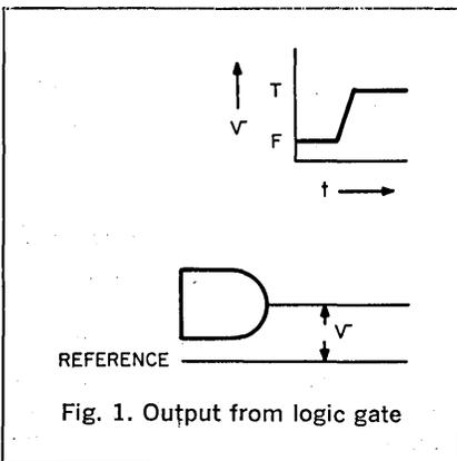
Fig. 1. Output from logic gate
