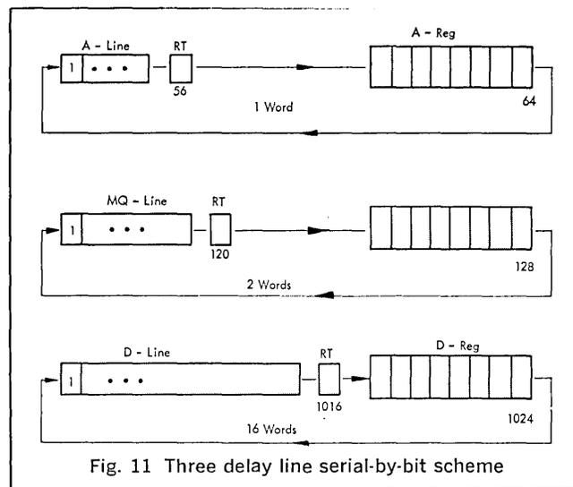
Fig. 11 Three delay-line serial-by-bit scheme
