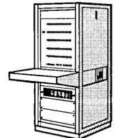
Beyond 190 I/O line pairs or 60 data bits, or where additional control section switches are required, a 72" high cabinet may be specified.
