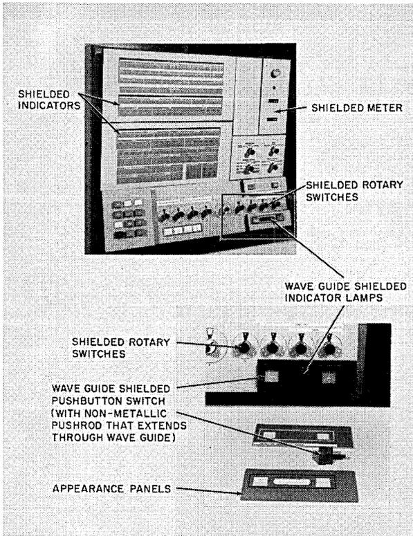
Fig. 4 EMC computer model with shielded treatment to controls and appearance panels
