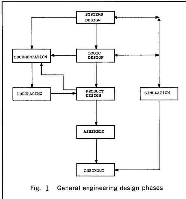
Fig. 1 General engineering design phases
