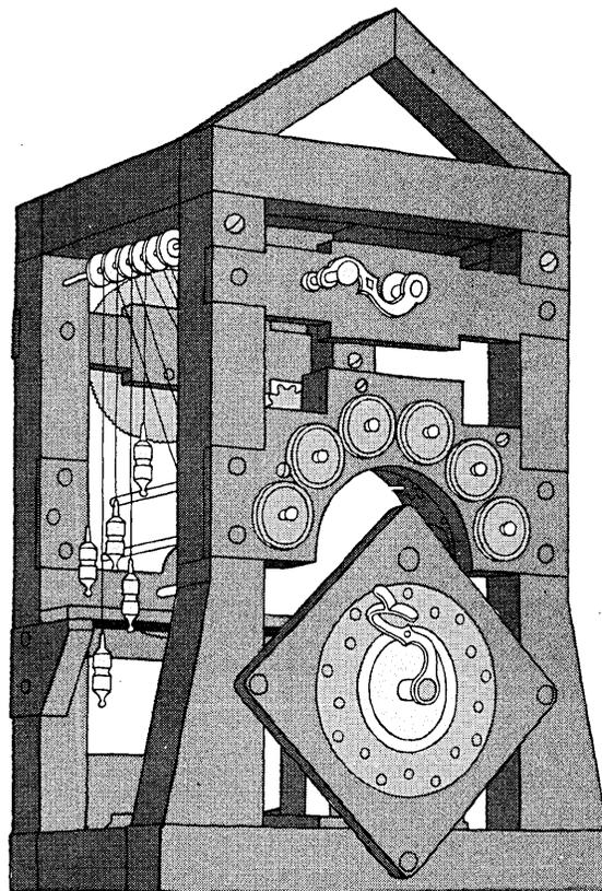
*Poleni's passion. Wind it up, and you could automatically compute the four fundamental arithmetic operations to three figures.*
