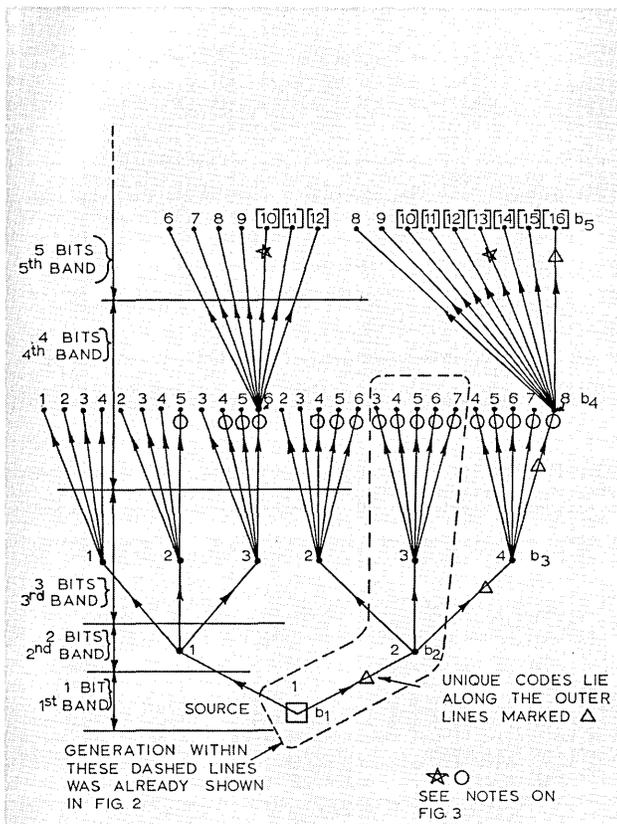
Fig. 3 Generation of all positive-bit-weight codes
