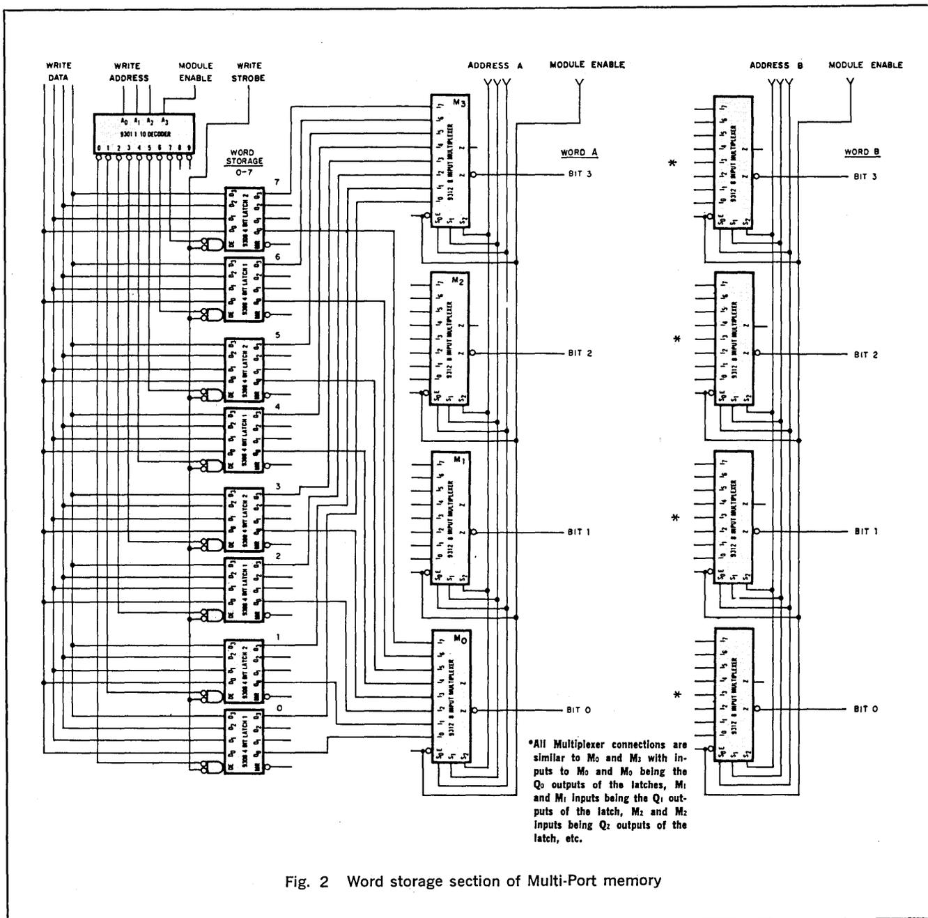
Fig. 2 Word storage section of Multi-Port memory
