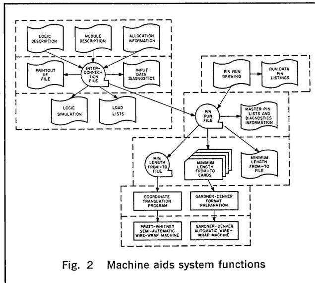
Fig. 2 Machine aids system functions
