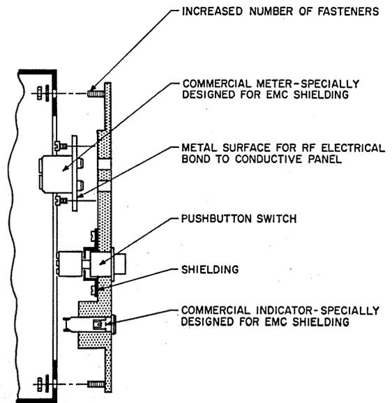
Fig. 7 Moderately treated EMC panel
