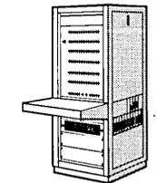
Where a Universal Interface is specified, two 64" high cabinets are usually required. Inclusion of this option increases the minimum cycle time from 100nsec to 150nsec.
