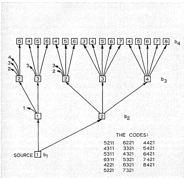
Fig. 4 4-bit code generation in the decimal system
