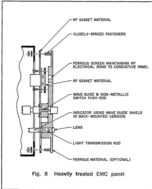
Fig. 8 Heavily treated EMC panel
