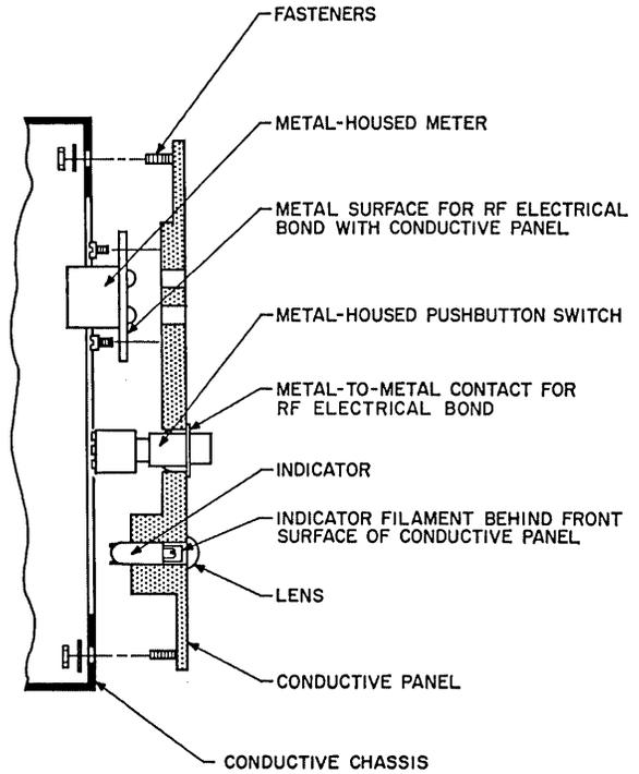
Fig. 6 Lightly shielded control mounting panel for EMC purposes
