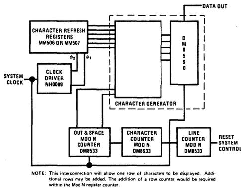
FIGURE 3. MOS/TTL System for Generation and Display Refresh.
