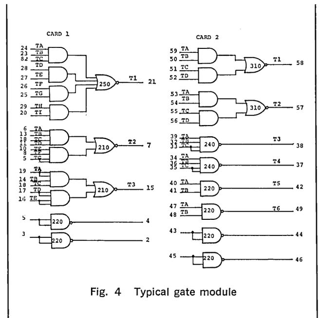
Fig. 4 Typical gate module
