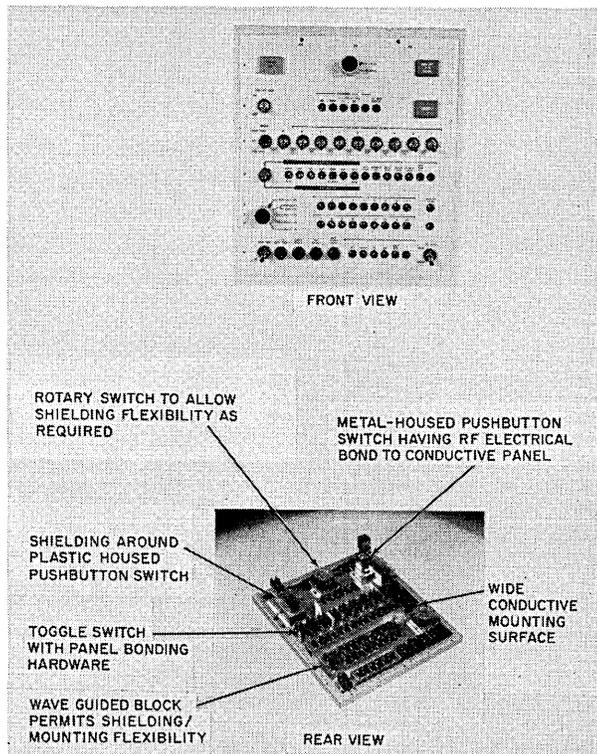
Fig. 5 EMC shielding, such as wave-guide blocks and housings (rear view) consume space for functional controls unless careful design is applied
