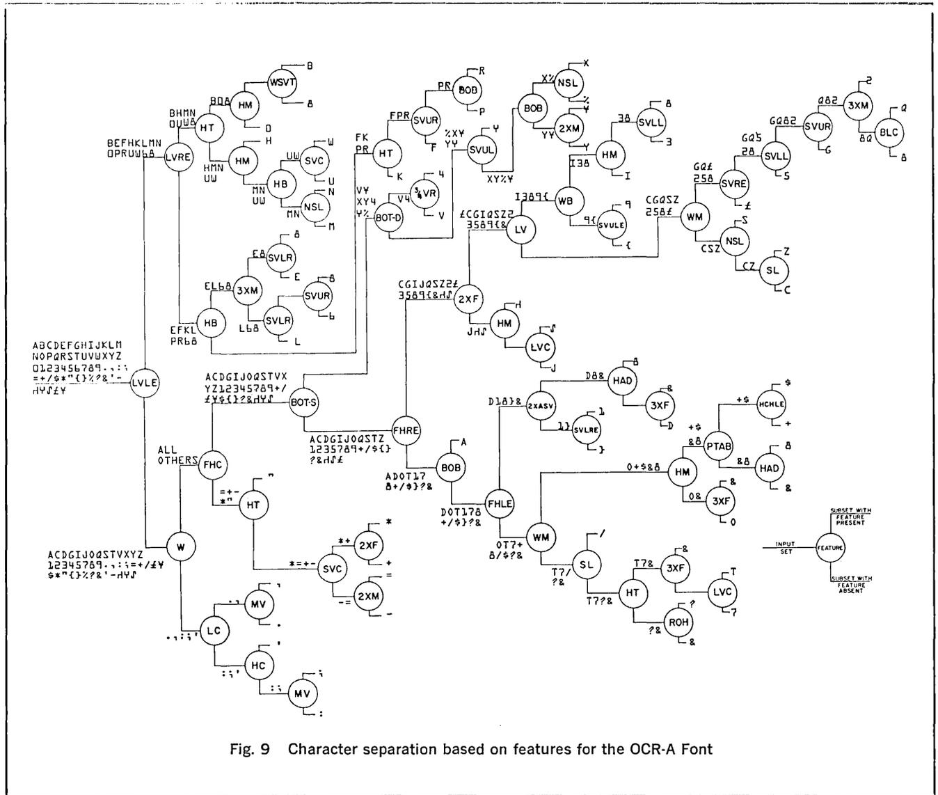
Fig. 9 Character separation based on features for the OCR-A Font
