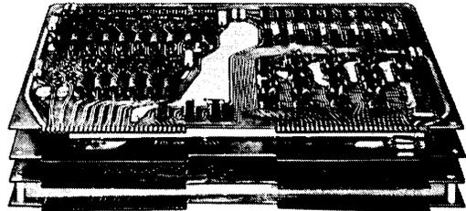
That's right, only \$2700 for up to 73,728 bits of information in an off-the-shelf memory system with 3 $\mu$ sec cycle time. Also standard in 4K by 12 or 16 bit words, and 2K by 12, 16 or 18 bit words ... In P.C. card sets, sub-chassis or rack mounted. DTL and TTL IC logic for maximum interface compatibility and optimum performance reliability.
