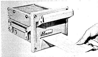
A 51 x 12 tab reader which supplies a full 612 bits from a standard 80 x 12 IBM punched card, is designed for data acquisition, process control and production control applications. The tab reader has an advanced contact system that eliminates unreliable thru-card contacts and prevents lint and dirt from impairing operation. The new design also does away with varying contact resistance caused by the accumulation of contaminants on conventional P.C. switch elements under a punched card.
