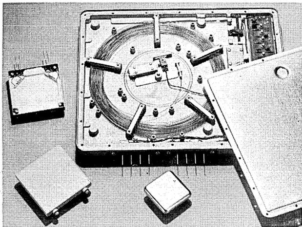
Group of digital stores. Largest unit is wire-sonic type with 17,000 bit storage capacity at cost of approximately ½ cent per bit. Input transducer in center converts electrical signal to sonic energy which propagates through wire (coiled into multi-layer helix) until it reaches output transducer which reconverts the energy. Remaining stores contain glass. Unit with cover removed is 2,000 bit store.
