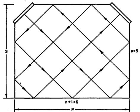
**Wave propagation patterns in two typical digital glass delay line stores.**
