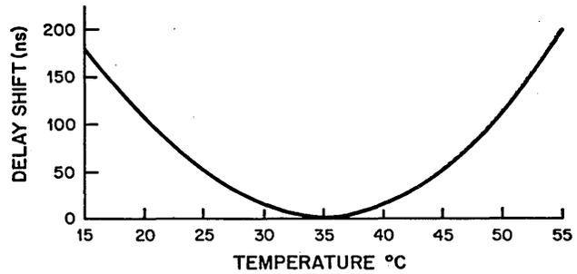
Fig. 1 Typical delay shift vs. temperature curve for a 10,000 foot  $\mu\text{sec}$  wire-sonic delay line.
