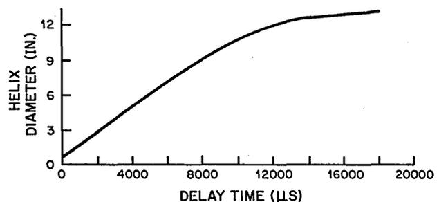
Fig. 2 Minimum helix diameter vs. delay time curve for wire-sonic delay lines.
