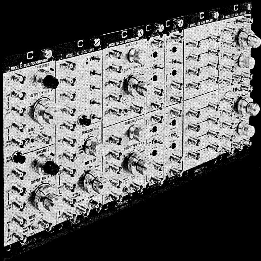
**Nanologic 150: Simultaneous, Automatic Measurement of Output Amplitude • Width • Propagation Delay • Rise Time • Fall Time • With 1 mV Accuracy and Picosecond Timing On a Single-Bit Sample. Plus . . .**
