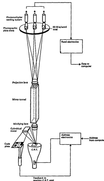
Fig. 1 Block diagram of the optical fixed store.
