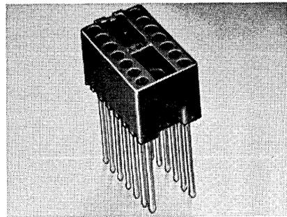
channel shaped. Designed in accordance with MIL-STD-1130, this four-corner channel shaped post of spring hardness delivers unusual advantages for wrapped terminations. The contact post plating is hard gold-over-nickel, but tin plating is optional. Other features include the availability of bridging contacts which make direct contact between a post and printed circuitry on the front or back panel. AMP Inc., Harrisburg, Pa.
