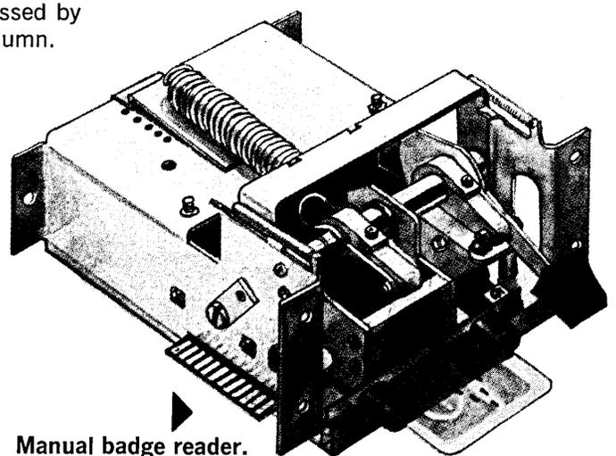
**Manual badge reader. Model 361.** Cross-matrix or individual outputs. Takes 15-, 20- or 22-column badge up to 0.040" thick. One-hand operation. Up to 264 switches. Designed for one million cycles.
