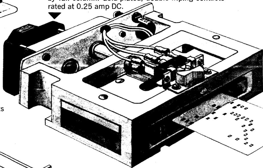
**Behind-panel reader.** Model 2981A. Industrial full 80-column card reader. Complete alphanumeric coding and 160 six-bit word capability with only 160 diodes. Can be bussed by column, by split column, or by row. Gold-plated contacts take 0.25 amp.
