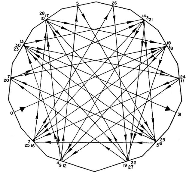
**Wave propagation pattern in polygonal quartz delay line serial store.**
