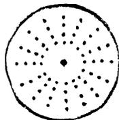
Diagram of the versatile multiple switch, which can be assembled to make any switch combinations from 16 decks of 2 positions, 10 decks of 3 positions, etc., to 2 decks of 16 positions.
