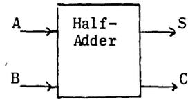
This circuit expresses in hardware a part of the functions necessary for binary addition. The letter S stands for "sum without carry"; the letter C stands for "carry". With two half-adders, and another circuit properly transferring the carry from one column to the next column, a circuit which will perform binary addition can be constructed.
