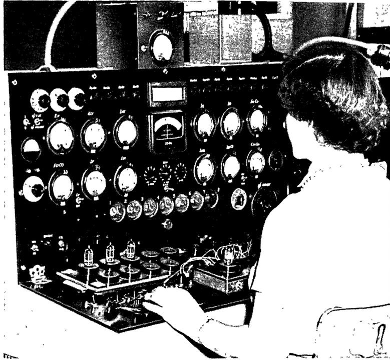
▲ **CHECKED FOR COMPUTER-SERVICE CHARACTERISTICS!** G-E computer tubes are specifically tested for those electrical qualities that closely affect tube operation in computer circuits. Among the characteristics checked are zero-bias plate current . . . cut-off performance . . . difference in cut-off between both triode sections.
