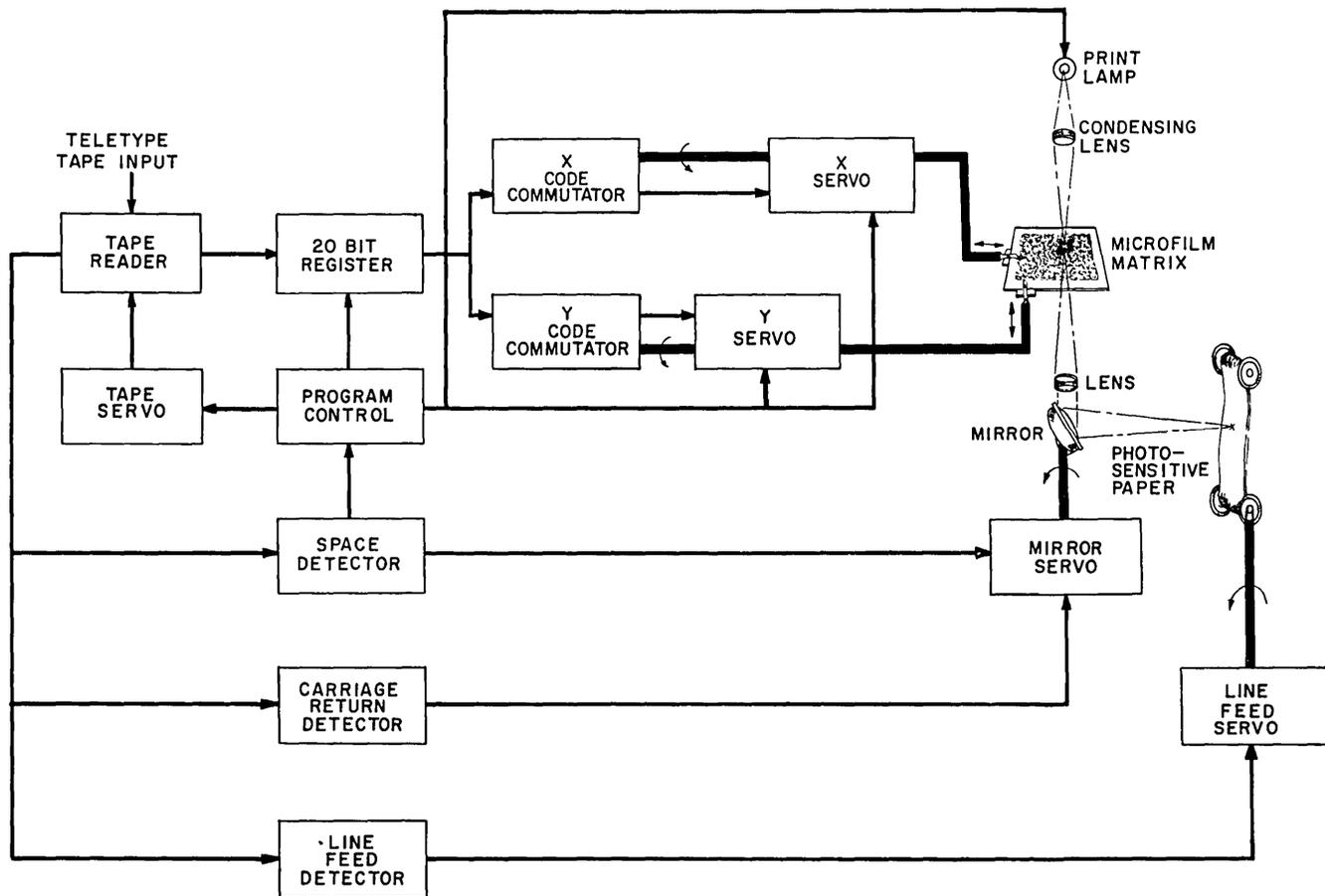
DIGITAL AUTOMATIC MICROFILM SELECTOR AND PRINTER
